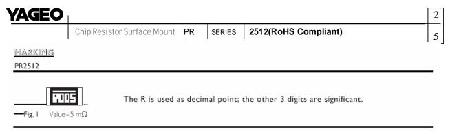
For marking codes, please see EIA-marking code rules in data sheet "Chip resistors marking".
