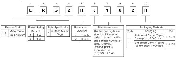
The above example 2 shows a metal oxide film resistor SMD type, 2 W power rating, resistance value of 1.0 kΩ, tolerance ±5 %, and embossed taping.
