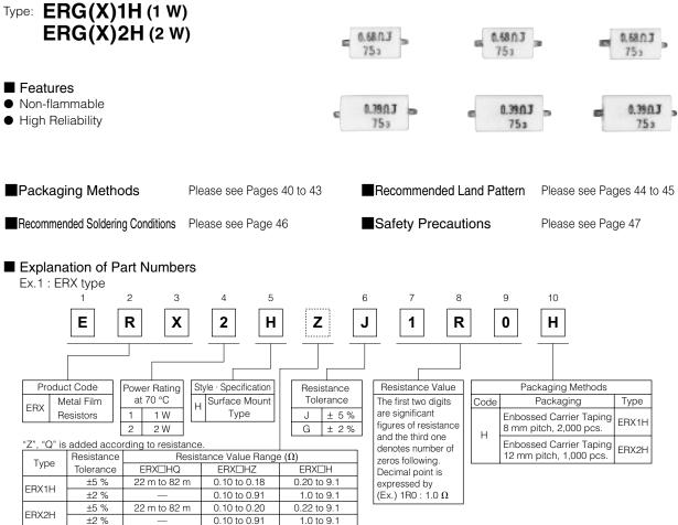
The above example 1 shows a metal film resistor SMD type, 2 W power rating, resistance value of 1.0 Ω, tolerance ±5 %, and embossed taping.
