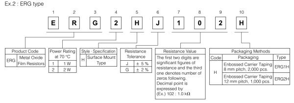
The above example 2 shows a metal oxide film resistor SMD type, 2 W power rating, resistance value of 1.0 kΩ, tolerance ±5 %, and embossed taping.
