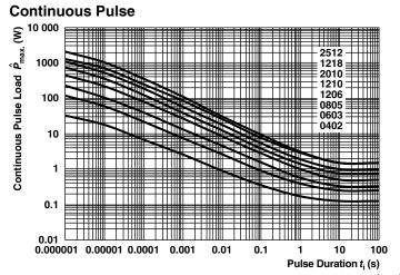
Maximum pulse load, continuous pulses; applicable if  $\overline{P} \leq P(\vartheta_{amb})$  and  $\hat{U} \leq \hat{U}_{max}$ ; for permissible resistance change equivalent to 8000 h operation
