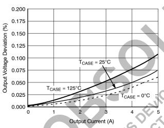
Figure 4. Load Regulation vs.
