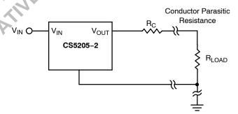
Figure 8. Conductor Parasitic Resistance Effects
