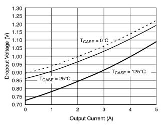
Figure 2. Dropout Voltage vs. Output Current
