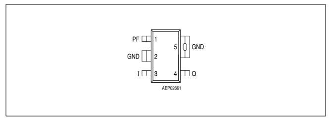
Figure 1 Pin Configuration (top view)
