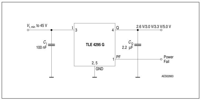
Figure 3 Application Circuit
