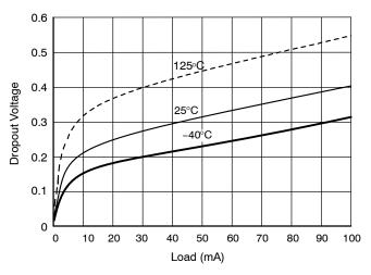
Figure 2. CS8101 Dropout Voltage vs. Load Over Temperature
