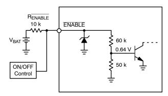
Figure 7. Using the ENABLE pin with V<sub>BAT</sub>
