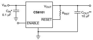
\*C<sub>IN</sub> required if regulator is located far from the power supply filter.
