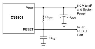
Figure 5. RC Network for RESET Delay
