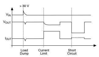
Figure 3. Typical Circuit Waveforms for Output Stage Protection
