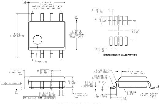
CONTROLLING DIMENSION IS MILLIMETER VALUES IN [ ] ARE INCHES
