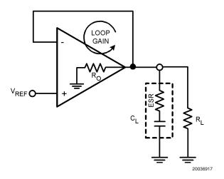
FIGURE 3. Simplified Model of Regulator Loop Gain Components
