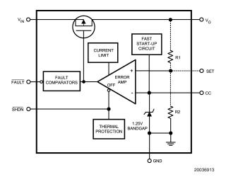
FIGURE 1. Functional Block Diagram for the LP3982
