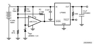
FIGURE 6. Minimum Battery Detector that Disconnects the Load Via the SHDN Pin of the LP3982
