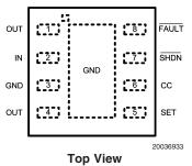
Note: The SET pin is internally disconnected for the fixed versions.
