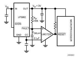
FIGURE 5. Power on Delayed Reset Application
