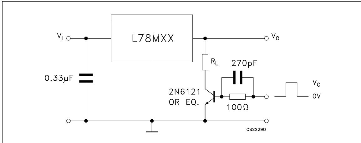
**Figure 7. Ripple rejection**
