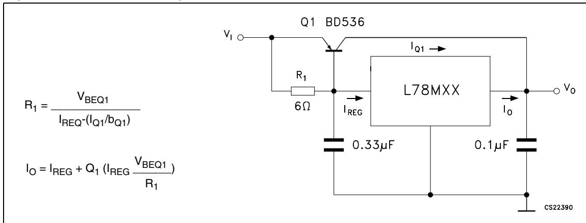
**Figure 20. Short-circuit protection**
