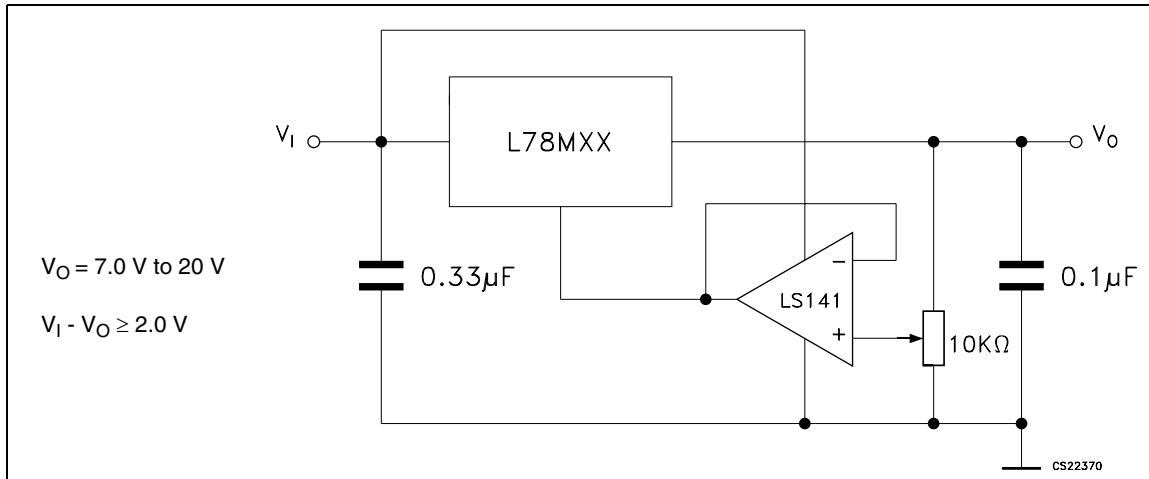
**Figure 19. Current boost regulator**
