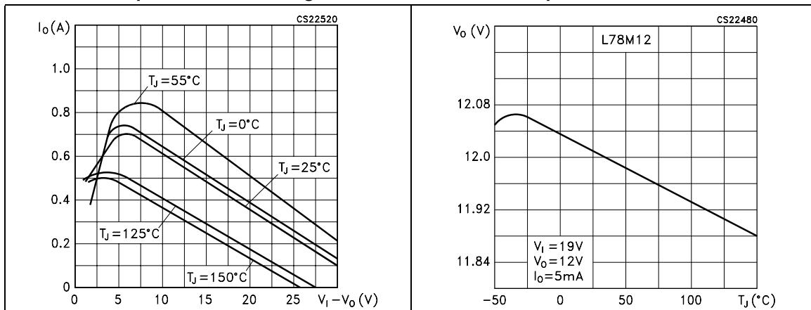
**Figure 11. Output voltage vs. junction temperature**
