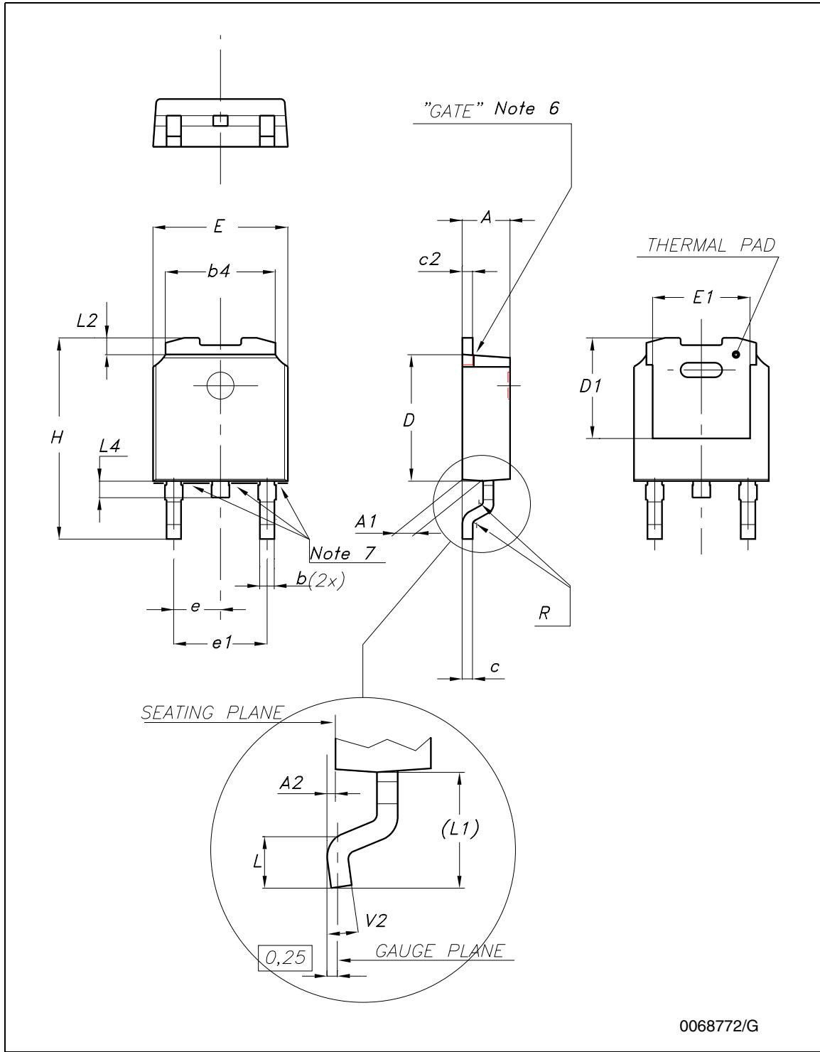
**Figure 22.** Drawing dimension DPAK type FUJITSU-subcon
