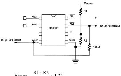
$$V_{\text{SENSE}} = \frac{R1 + R2}{R2} \times 1.25$$
