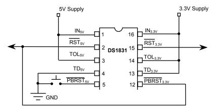
NOTE: The  $\overline{\text{RST}}_{5V}$  output is connected to the IN<sub>3.3V</sub> via a 100 k $\Omega$  resistor in the push-button input and therefore does not require a pull-up resistor (an addition pull up can be used to accelerate responses). If an external pull up is used in this example it must be connected to the 3.3V power supply.
