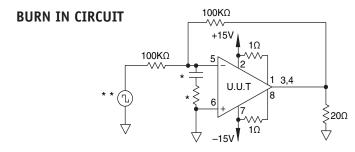
\* These components are used to stabilize device due to poor high frequency characteristics of burn in board.
