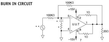
\* These components are used to stabilize device due to poor high frequency characteristics of burn in board.
