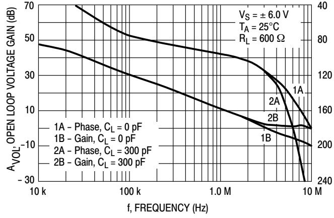
**Figure 18.** Voltage Gain and Phase versus Frequency
