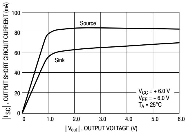
Figure 13. Output Short Circuit Current
