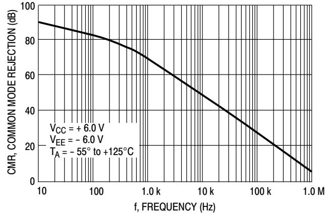
Figure 11. Common Mode Rejection
