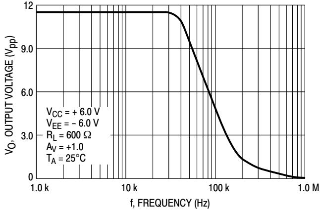
Figure 10. Output Voltage
