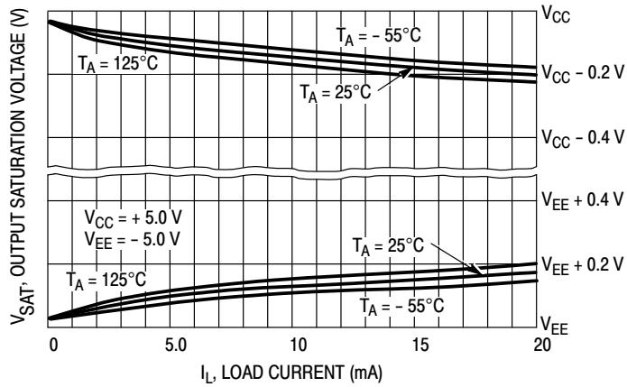
Figure 9. Output Saturation Voltage
