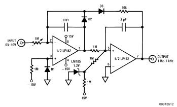
Trim 1M pot for 1 kHz full-scale output 15 mW power drain No integrator reset FET required Mount D1 and D2 in close proximity 1% linearity to 1 kHz
