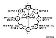
Pin 4 connected to case
