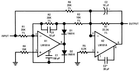
Note 1: Feedforward compensation can be used to make a fast full wave rectifier without a filter.
