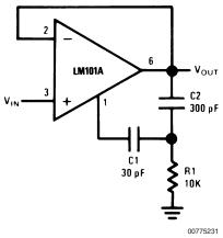
Power Bandwidth: 15 kHz Slew Rate: 1V/µs
