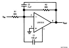
Power Bandwidth: 250 kHz Small Signal Bandwiidth: 3.5 MHz
