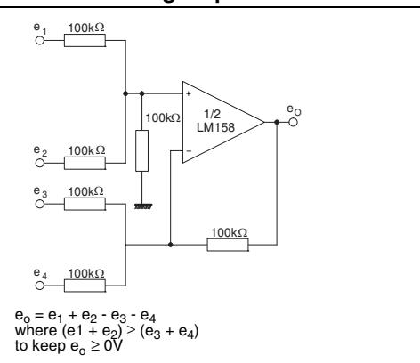
**Figure 22. High input Z, DC differential amplifier**
