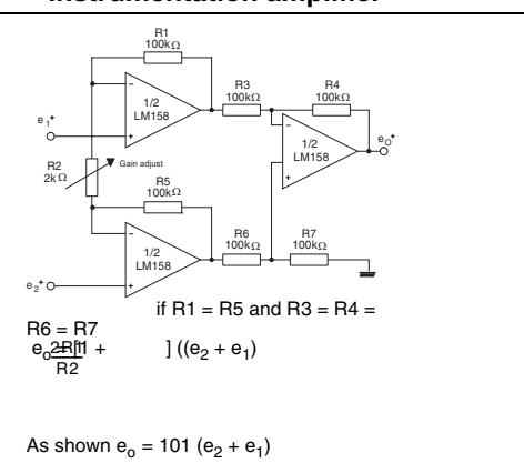
**Figure 24.** Using symmetrical amplifiers to reduce input current
