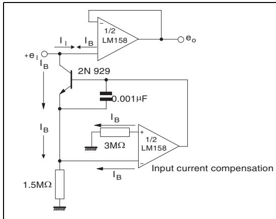
**Figure 25.** Low drift peak detector
