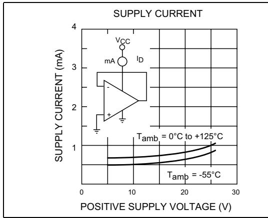
**Figure 13. Input current**
