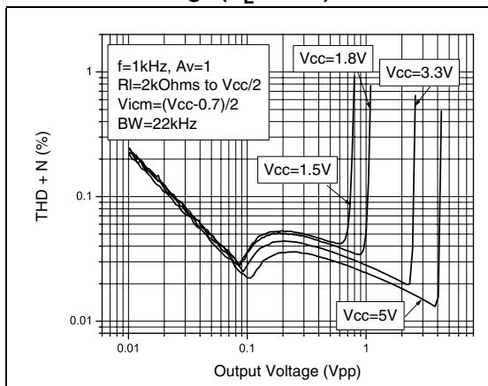
**Figure 12. Distortion + noise vs. output voltage ( $R_L = 100 \text{ k}\Omega$ )**
