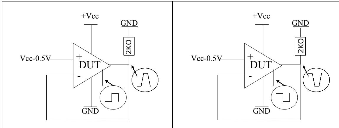
**Figure 20.** Turn-on time,  $\text{V}_{\text{CC}} = 5 \text{ V}$ ,
