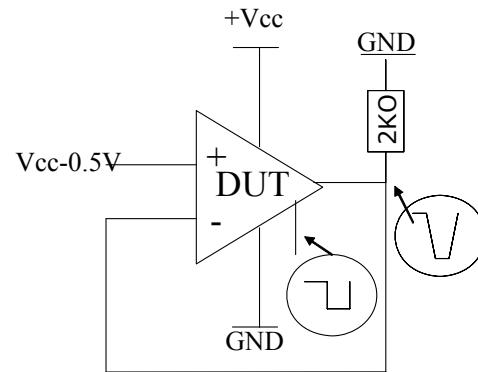
**Figure 21.** Turn-off time,  $\text{V}_{\text{CC}} = 5 \text{ V}$ ,
