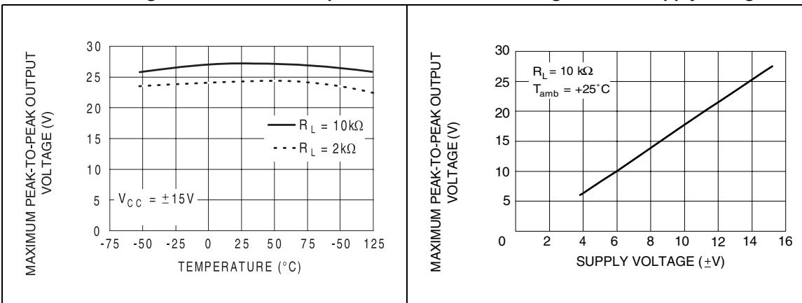
**Figure 7. Maximum peak-to-peak output voltage versus supply voltage**
