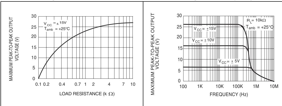
**Figure 5. Maximum peak-to-peak output voltage versus frequency**
