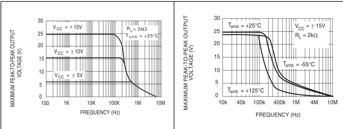
**Figure 3. Maximum peak-to-peak output voltage versus frequency**
