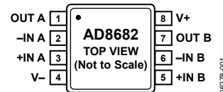
Figure 1. 8-Lead SOIC_N and 8-Lead MSOP
