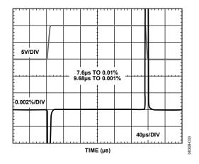
Figure 33. Large-Signal Pulse Response and Settling Time, 10 V Step,  $V_S = \pm 15 \text{ V}, G = 2$
