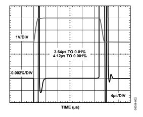
Figure 32. Large-Signal Pulse Response and Settling Time, 2 V Step,  $V_S = 2.7 \, V, \, G = \frac{1}{2}$
