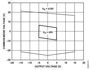
Figure 13. Input Common-Mode Voltage vs. Output Voltage,  $\pm 15 \text{ V}$  and  $\pm 5 \text{ V}$  Supplies, G = 2
