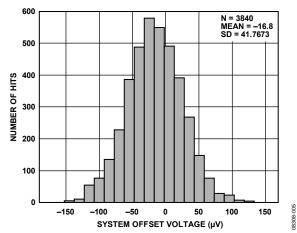
Figure 5. Distribution of Typical System Offset Voltage, G = 2
