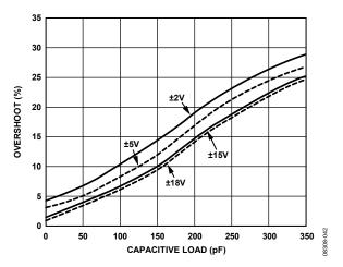
Figure 42. Small-Signal Overshoot vs. Capacitive Load,  $R_L \ge 2 k\Omega$ , G = 2
