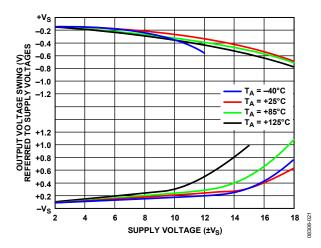
Figure 21. Output Voltage Swing vs. Supply Voltage and Temperature,  $R_l = 2 k\Omega$
