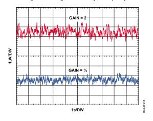
Figure 44. 0.1 Hz to 10 Hz Voltage Noise
