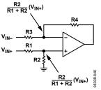
Figure 46. Voltage Division in the Difference Amplifier Configuration
