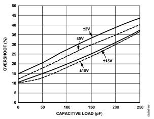
Figure 41. Small-Signal Overshoot vs. Capacitive Load,  $R_L \ge 2 \ k\Omega$ ,  $G = \frac{1}{2}$
