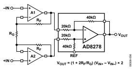
Figure 56. Low Power Precision Instrumentation Amplifier
