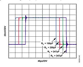
Figure 40. Small-Signal Step Response for Various Capacitive Loads, G = 2
