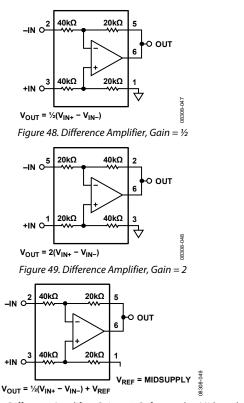
Figure 50. Difference Amplifier, Gain =  $\frac{1}{2}$ , Referenced to Midsupply
