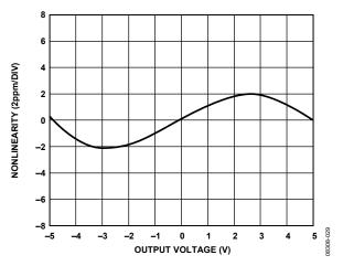
Figure 29. Gain Nonlinearity,  $V_S = \pm 15 \text{ V}$ ,  $R_L \ge 2 \text{ k}\Omega$ ,  $G = \frac{1}{2}$
