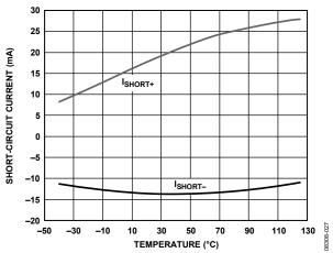
Figure 27. Short-Circuit Current vs. Temperature
