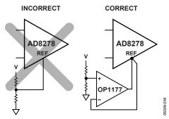
Figure 55. Driving the Reference Pin
