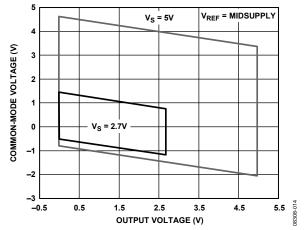
Figure 14. Input Common-Mode Voltage vs. Output Voltage, 5 V and 2.7 V Supplies,  $V_{REF} = Midsupply$ , G = 2
