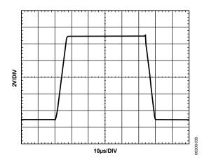
Figure 35. Large-Signal Step Response,  $G = \frac{1}{2}$
