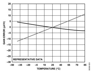
Figure 9. Gain Error vs. Temperature, Normalized at 25°C,  $G = \frac{1}{2}$
