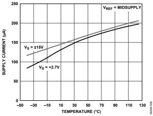
Figure 26. Supply Current vs. Temperature
