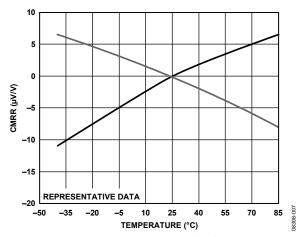
Figure 7. CMRR vs. Temperature, Normalized at 25°C,  $G = \frac{1}{2}$
