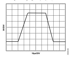
Figure 36. Large-Signal Step Response, G = 2
