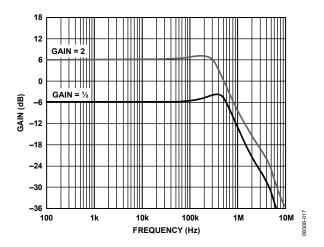
Figure 17. Gain vs. Frequency, +2.7 V Single Supply
