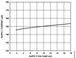
Figure 24. Supply Current vs. Dual-Supply Voltage,  $V_{IN} = 0 V$
