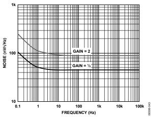
Figure 43. Voltage Noise Density vs. Frequency
