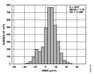
Figure 6. Distribution of Typical Common-Mode Rejection, G = 2
