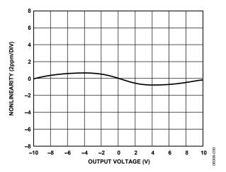
Figure 30. Gain Nonlinearity,  $V_S = \pm 15 \text{ V}$ ,  $R_L \ge 2 \text{ k}\Omega$ , G = 2
