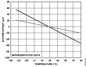
Figure 8. System Offset vs. Temperature, Normalized at 25°,  $G = \frac{1}{2}$
