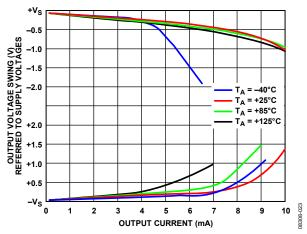
Figure 23. Output Voltage Swing vs.  $I_{OUT}$  and Temperature,  $V_S = \pm 15 \text{ V}$
