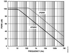
Figure 19. PSRR vs. Frequency
