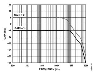
Figure 16. Gain vs. Frequency, ±15 V Supplies
