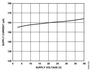
Figure 25. Supply Current vs. Single-Supply Voltage,  $V_{IN} = 0 V$ ,  $V_{REF} = 0 V$
