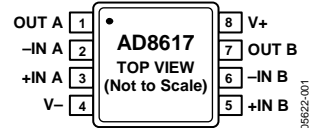
Figure 2. 8-Lead MSOP and 8-Lead SOIC_N
