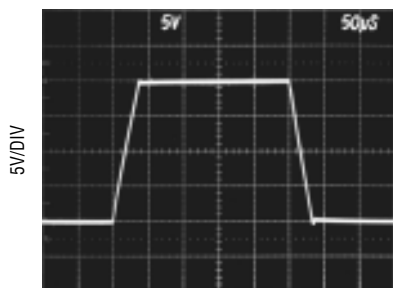
Large-Signal Transient Response
