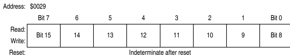
Figure 18-15. TIM Channel 1 Register High (TCH1H)
