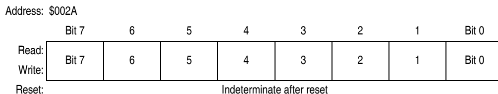
Figure 18-16. TIM Channel 1 Register Low (TCH1L)
