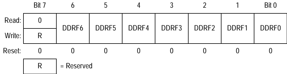
Figure 20-18. Data Direction Register F (DDRF)
