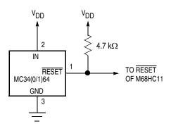
Figure 1-7. External Reset Circuit
