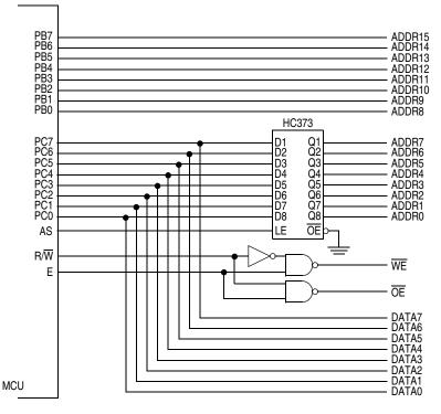
Figure 2-1. Address/Data Demultiplexing
