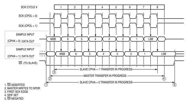
Figure 8-2. SPI Transfer Format
