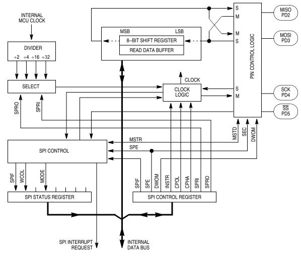
Figure 8-1. SPI Block Diagram
