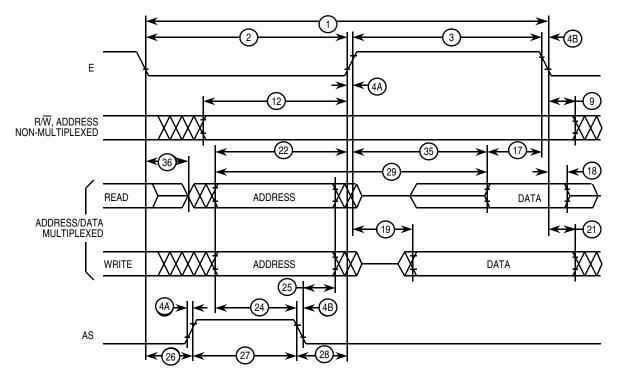
Note: Measurement points shown are 20% and 70% of V<sub>DD</sub>.
