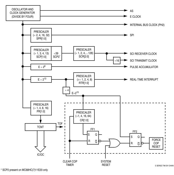
Figure 9-1. Timer Clock Divider Chains
