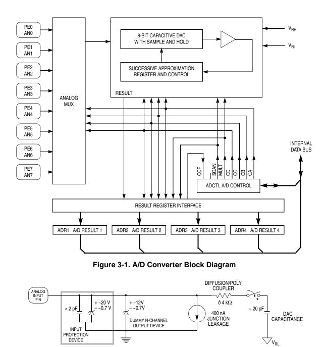
\* THIS ANALOG SWITCH IS CLOSED ONLY DURING THE 12-CYCLE SAMPLE TIME.
