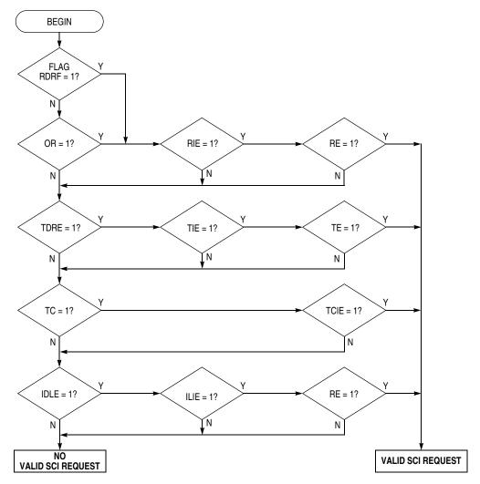
Figure 5-7. Interrupt Source Resolution Within SCI
