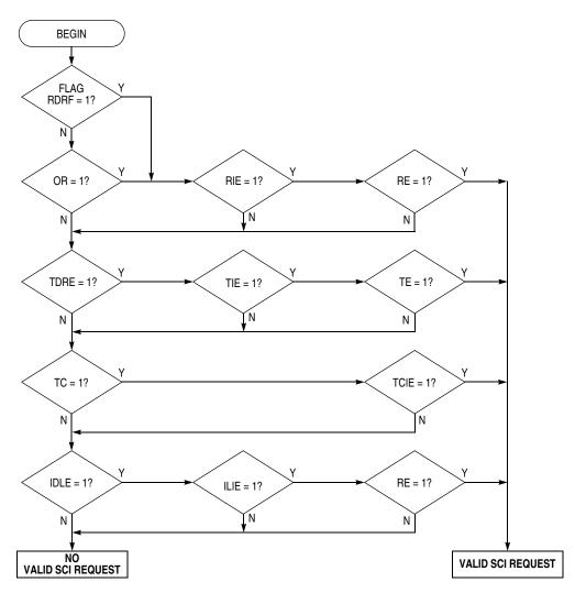
Figure 7-10. Interrupt Source Resolution Within SCI
