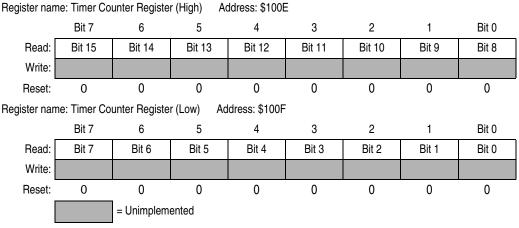
Figure 9-15. Timer Counter Register (TCNT)
