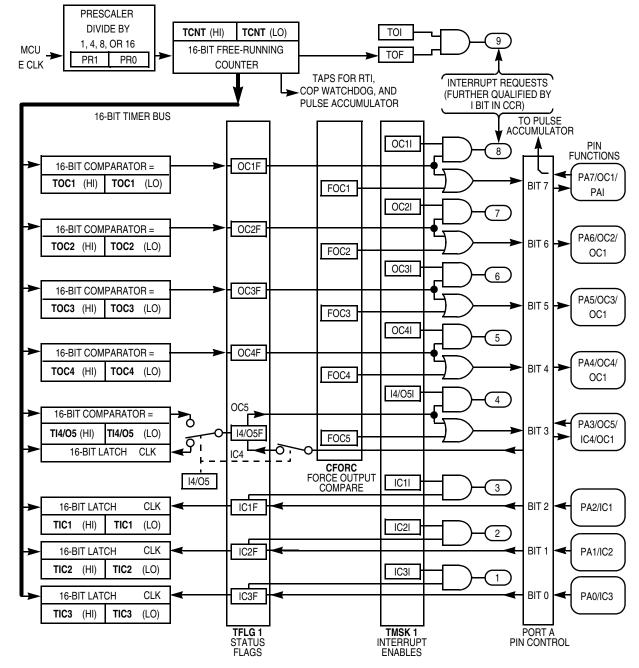
Figure 9-2. Capture/Compare Block Diagram
