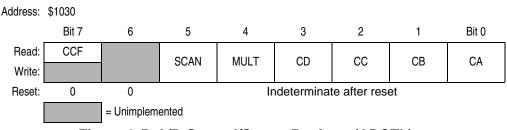
Figure 3-5. A/D Control/Status Register (ADCTL)
