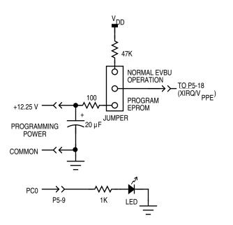
Figure 8. PC-to-MCU Programming Circuit
