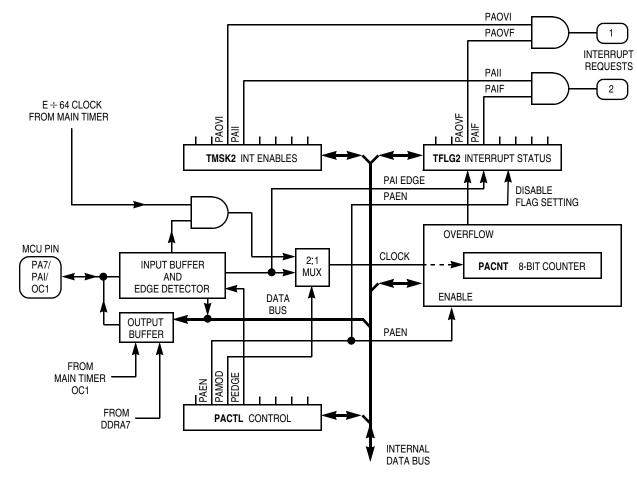
Figure 9-24. Pulse Accumulator
