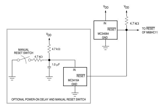
Figure 1-8. External Reset Circuit with Delay
