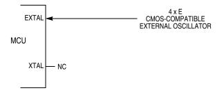
Figure 1-10. External Oscillator Connections
