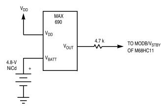
Figure 2-8. RAM Standby MODB/V<sub>STBY</sub> Connections
