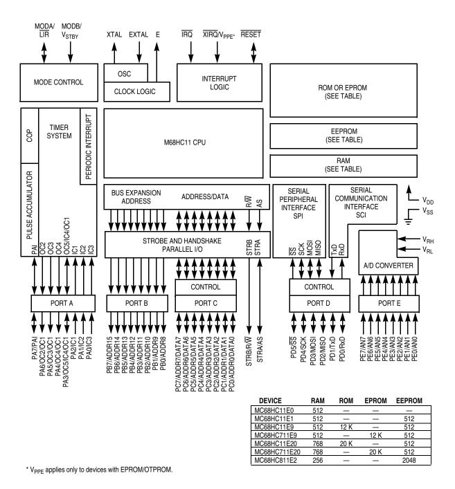
Figure 1-1. M68HC11 E-Series Block Diagram
