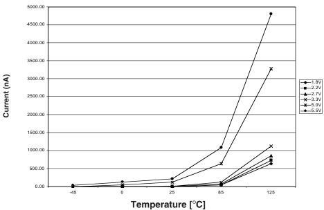
**Figure 9: IDLE Mode Current**
