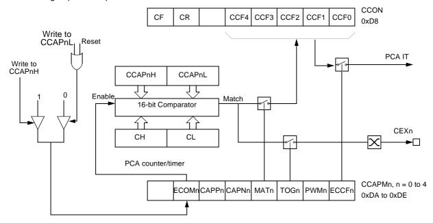
Before enabling ECOM bit, CCAPnL and CCAPnH should be set with a non zero value, otherwise an unwanted match could happen.
