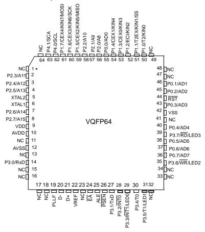
Figure 2. AT89C5131 64-pin VQFP Pinout
