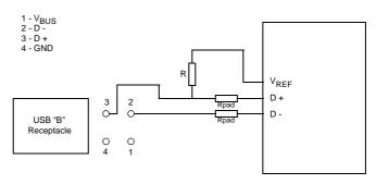
$R = 1.5 \text{ k}\Omega$  $R_{\text{pad}} = 27\Omega$
