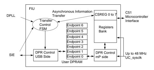
Figure 56. Minimum Intervention from the USB Device Firmware
