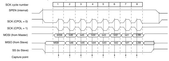
Figure 43. Data Transmission Format (CPHA = 1)
