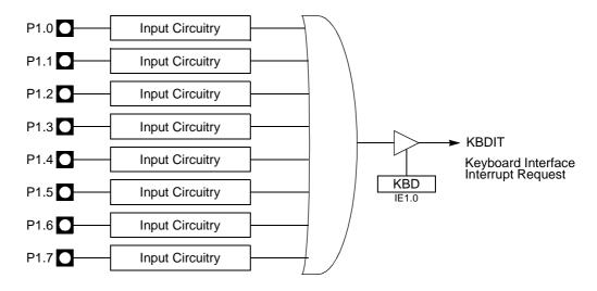
Figure 38. Keyboard Input Circuitry
