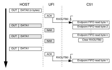
An endpoint will be first enabled and configured before being able to receive Bulk or Interrupt packets.
