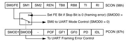
When this feature is enabled, the receiver checks each incoming data frame for a valid stop bit. An invalid stop bit may result from noise on the serial lines or from simultaneous transmission by two CPUs. If a valid stop bit is not found, the Framing Error bit (FE) in SCON register (See Table 57) bit is set.
