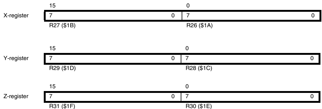
Figure 7. X-, Y-, and Z-registers
