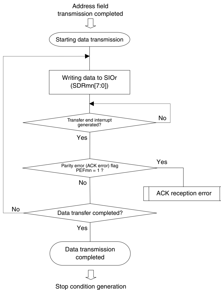
Figure 14-94. Flowchart of Data Transmission
