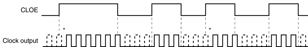
Figure 11-4. Clock Output Application Example
