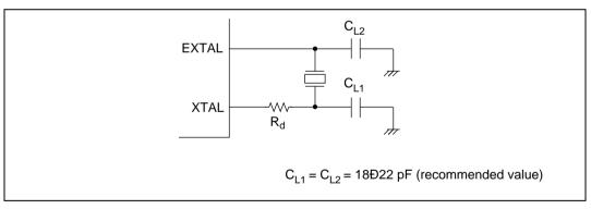
Figure 4.2 Connection of the Crystal Oscillator (Example)
