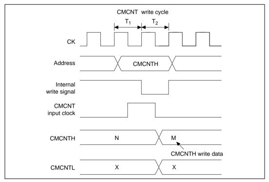
Figure 15.8 CMCNT Byte Write and Increment Contention
