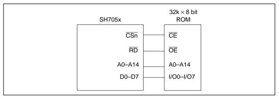
Figure 8.10 8-Bit Data Bus Width ROM Connection
