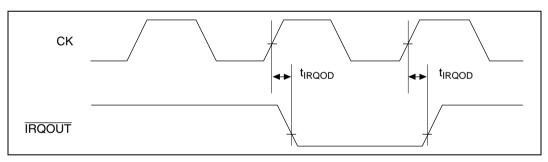
Figure 22.6 Interrupt Signal Output Timing
