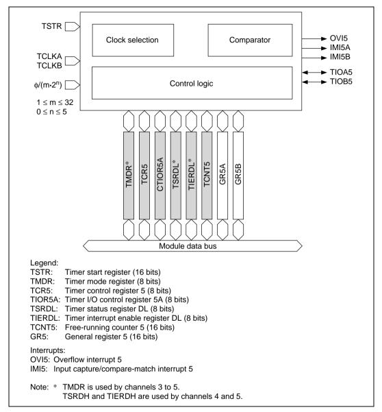
Figure 10.6 Block Diagram of Channel 5
