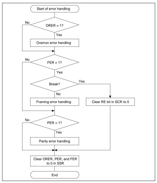
Figure 13.8 Sample Flowchart for Receiving Serial Data (2)
