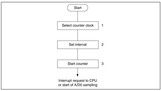
Figure 10.50 Sample Setup Procedure for Interval Timer Operation
