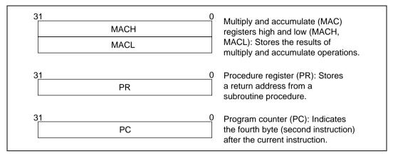
Figure 2.3 System Register Configuration
