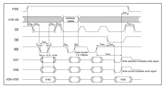
Figure 18.18 Auto-Program Mode Timing Waveforms
