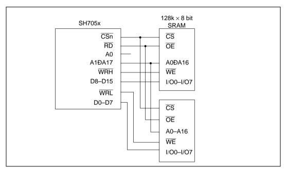
Figure 8.13 16-Bit Data Bus Width SRAM Connection
