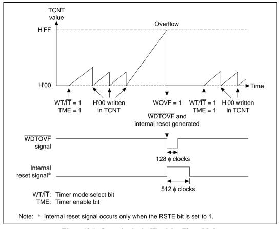
Figure 12.4 Operation in the Watchdog Timer Mode
