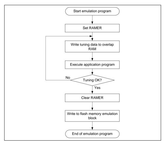
Figure 19.10 Flowchart for Flash Memory Emulation in RAM
