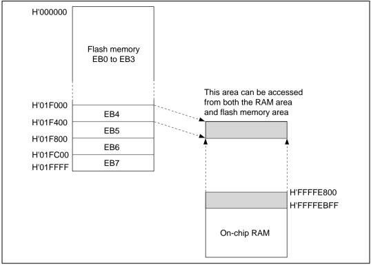
Figure 18.11 Example of RAM Overlap Operation
