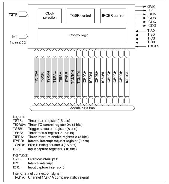
Figure 10.2 Block Diagram of Channel 0
