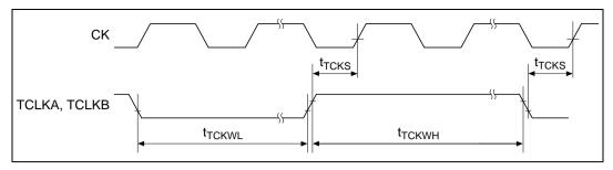
Figure 22.15 ATU Clock Input Timing
