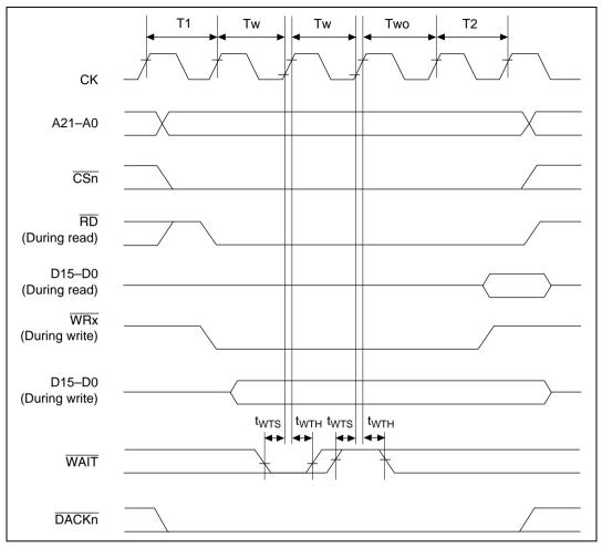
Figure 22.10 Basic Cycle (2 Software Waits + Wait due to WAIT Signal)
