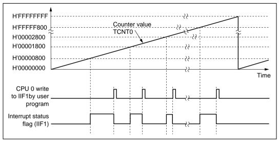
Figure 10.18 Example of Interval Timer Operation
