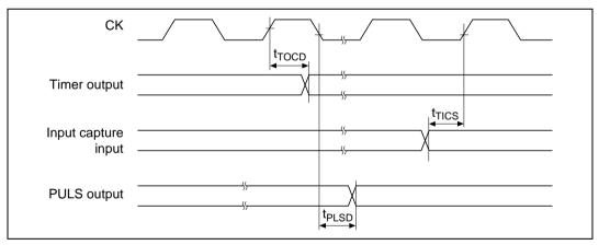
Figure 22.14 ATU I/O Timing
