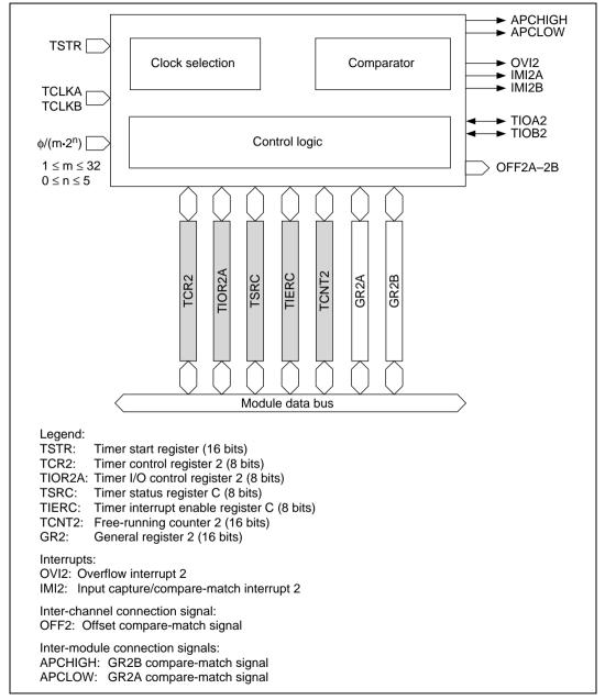
Figure 10.4 Block Diagram of Channel 2
