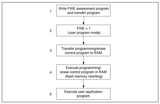
Figure 18.6 User Program Mode Execution Procedure
