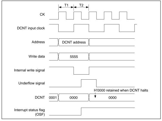
Figure 10.63 Contention between DCNT Write and Underflow
