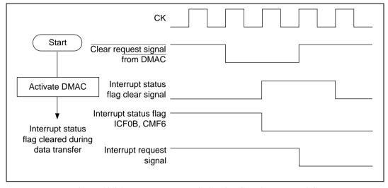
Figure 10.36 Procedure and Timing for Clearing by DMAC
