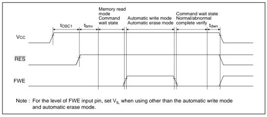
Figure 19.21 Oscillation Stabilization Time, Boot Program Transfer Time, and Power-Down Sequence
