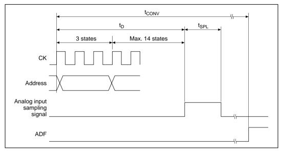
Figure 22.21 Analog Conversion Timing
