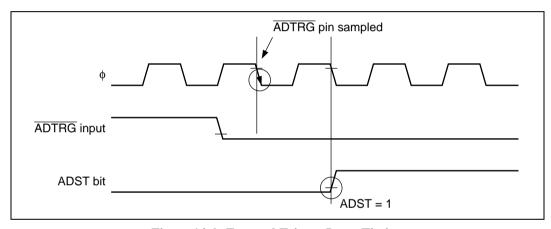
Figure 14.6 External Trigger Input Timing
