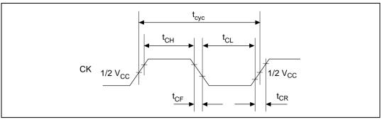
Figure 22.1 System Clock Timing
