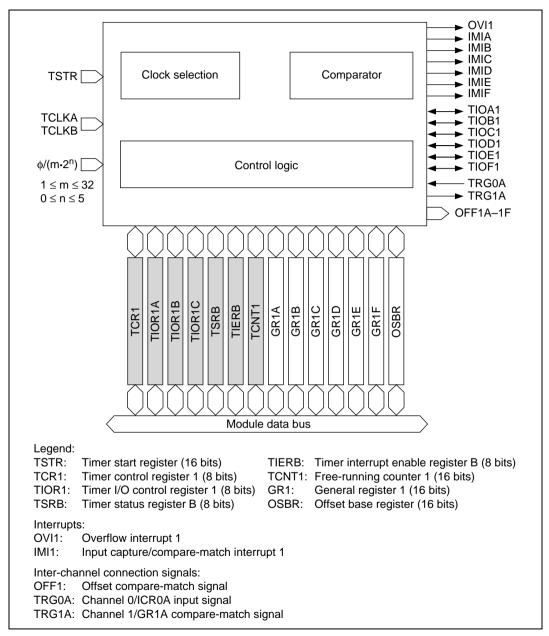
Figure 10.3 Block Diagram of Channel 1
