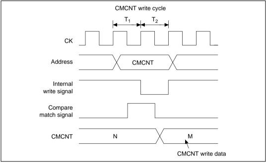
Figure 15.7 CMCNT Word Write and Increment Contention
