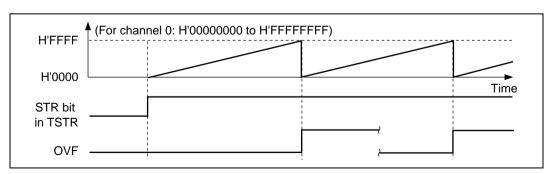
Figure 10.11 Free-Running Counter Operation
