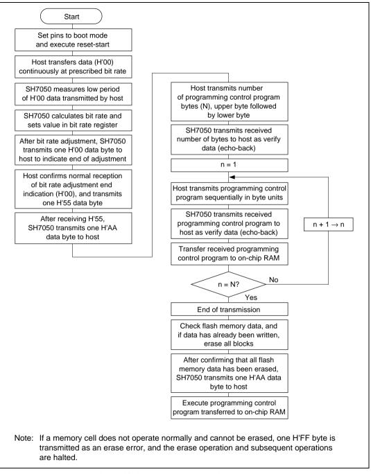
Figure 18.4 Boot Mode Execution Procedure
