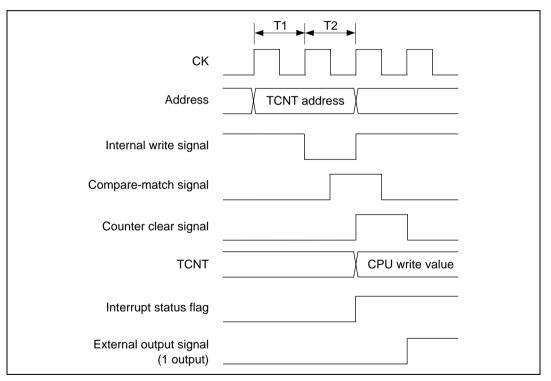
Figure 10.53 Contention between TCNT Write and Clear
