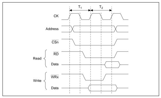
Figure 8.3 Basic Timing of Ordinary Space Access
