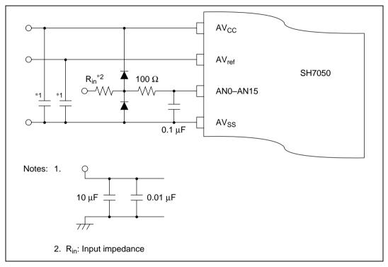
Figure 14.8 Example of Analog Input Pin Protection Circuit
