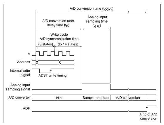
Figure 14.5 A/D Conversion Timing
