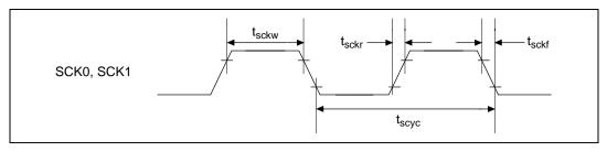
Figure 22.18 Input Clock Timing
