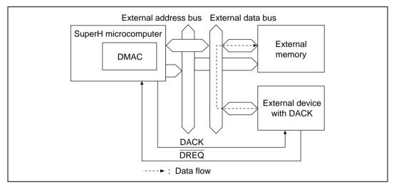
Figure 9.5 Data Flow in Single Address Mode
