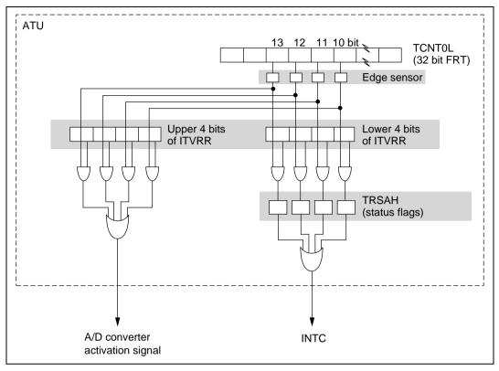
Figure 10.17 Schematic Diagram of Interval Timer
