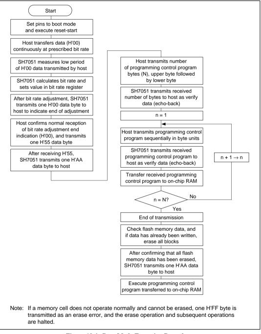
Figure 19.4 Boot Mode Execution Procedure
