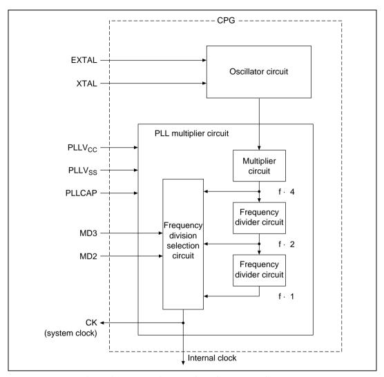
Figure 4.1 Block Diagram of the Clock Pulse Generator
