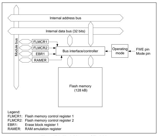
Figure 18.1 Block Diagram of Flash Memory
