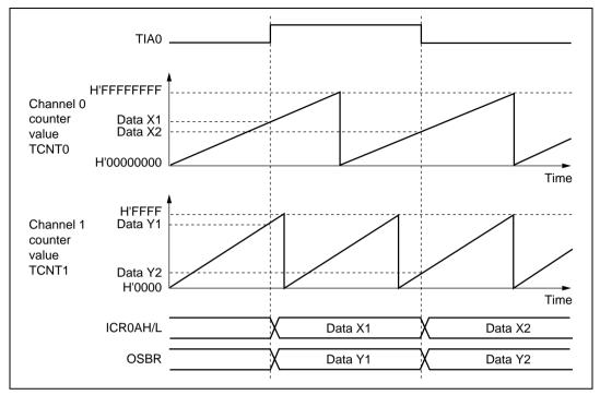
Figure 10.19 Example of Twin-Capture Operation
