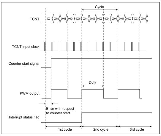
Figure 10.28 Channel 6 to 9 PWM Output Waveform
