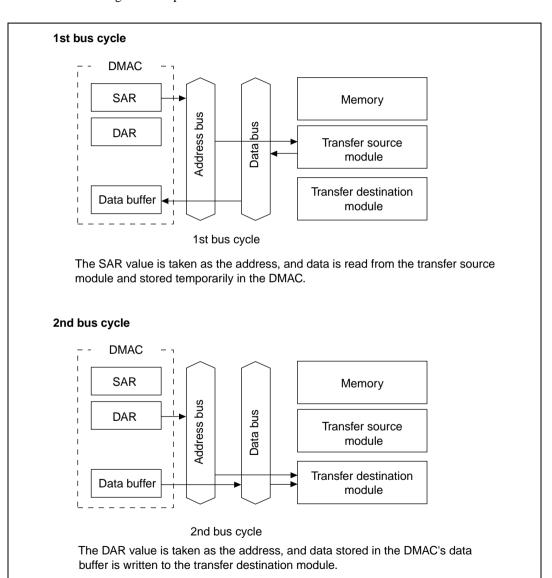
Figure 9.7 Direct Address Operation during Dual Address Mode
