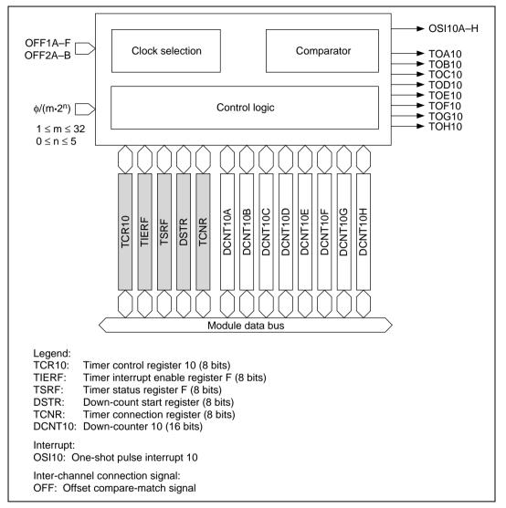
Figure 10.8 Block Diagram of Channel 10
