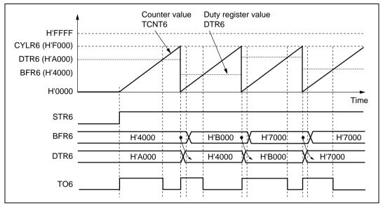
Figure 10.22 Example of Buffered PWM Waveform Output Operation
