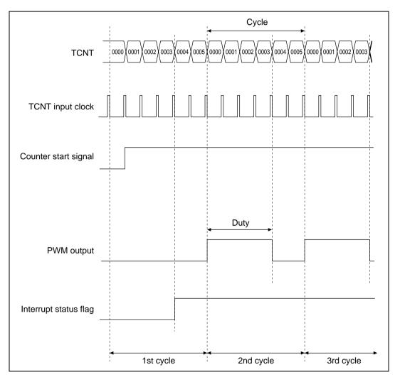
Figure 10.27 Channel 3 to 5 PWM Output Waveform
