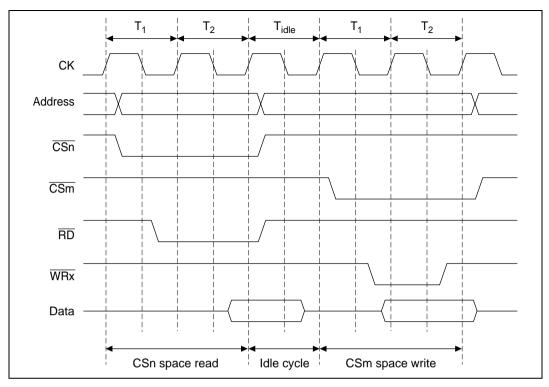
Figure 8.7 Idle Cycle Insertion Example
