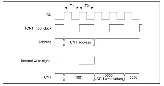
Figure 10.55 Contention between TCNT Write and Increment
