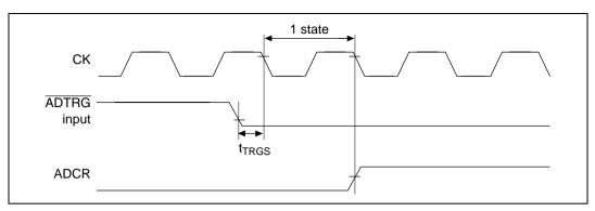
Figure 22.20 External Trigger Input Timing
