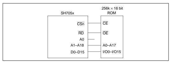
Figure 8.11 16-Bit Data Bus Width ROM Connection
