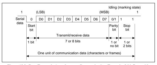
Figure 13.2 Data Format in Asynchronous Communication (Example: 8-bit Data with Parity and Two Stop Bits)
