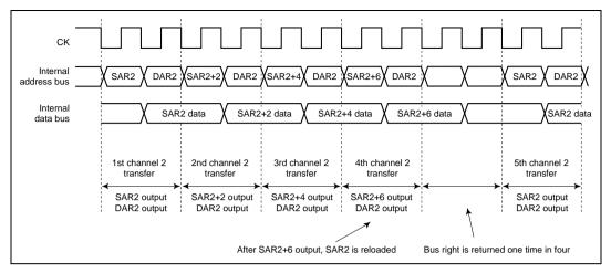
Figure 9.26 Source Address Reload Function Timing Chart
