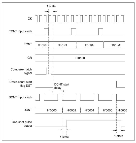
Figure 10.24 Offset One-Shot Pulse Function Pulse Output Timing
