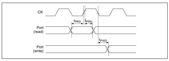
Figure 22.16 I/O Port I/O Timing
