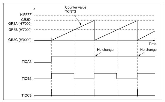
Figure 10.21 Example of PWM Waveform Output Operation
