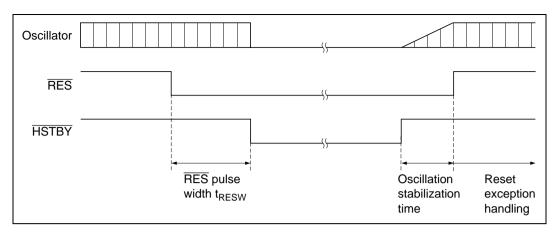
Figure 21.1 Hardware Standby Mode Timing
