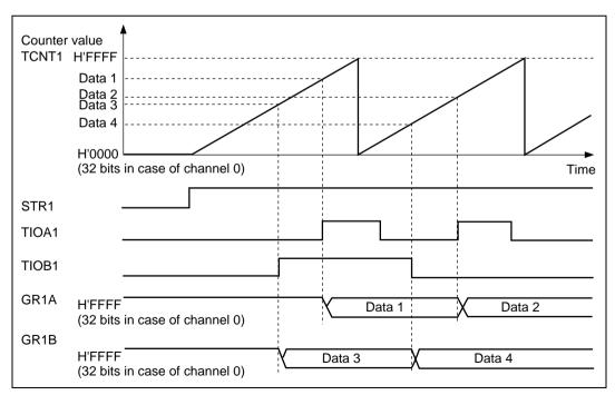
Figure 10.14 Example of Input Capture Operation
