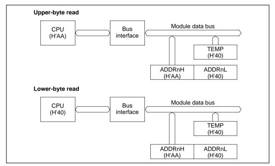
Figure 14.2 A/D Data Register Access Operation (Reading H'AA40)
