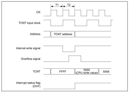
Figure 10.56 Contention between TCNT Write and Overflow
