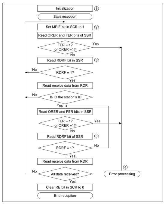
Figure 13.13 Sample Flowchart for Receiving Multiprocessor Serial Data
