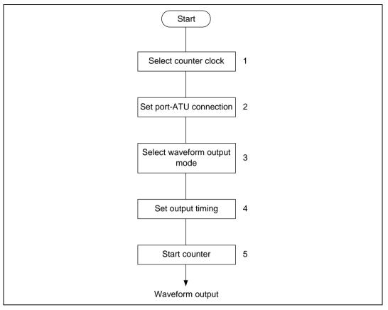
Figure 10.46 Sample Setup Procedure for Waveform Output by Output Compare-Match
