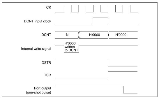
Figure 10.60 Halting of a Down-Counter by the CPU
