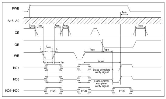
Figure 19.19 Auto-Erase Mode Timing Waveforms
