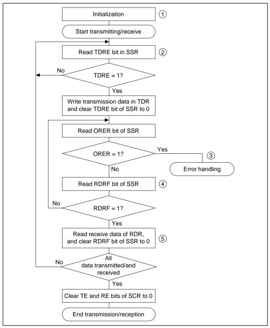
Figure 13.22 Sample Flowchart for Serial Transmission
