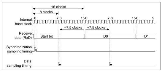
Figure 13.23 Receive Data Sampling Timing in Asynchronous Mode
