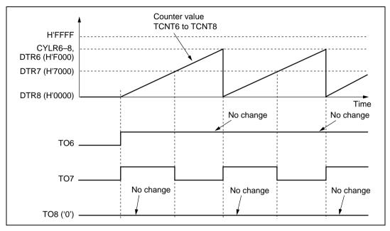
Figure 10.20 Example of PWM Waveform Output Operation
