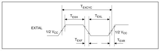
Figure 22.2 EXTAL Clock Input Timing
