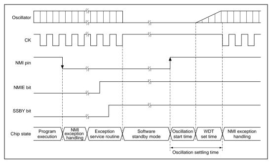
Figure 21.2 Standby Mode NMI Timing (Application Example)
