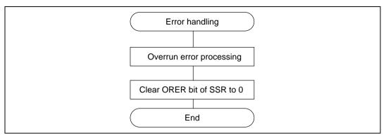
Figure 13.20 Sample Flowchart for Serial Receiving (cont)
