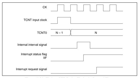
Figure 10.34 Timing of IIF Setting Timing by Interval Timer
