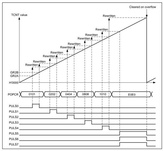
Figure 11.4 Example of Advanced Pulse Controller Output Operation
