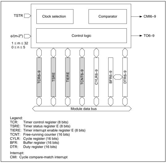
Figure 10.7 Block Diagram of Channels 6 to 9
