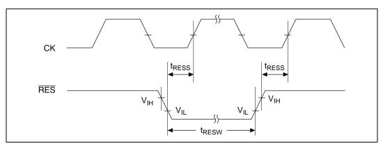
Figure 22.4 Reset Input Timing
