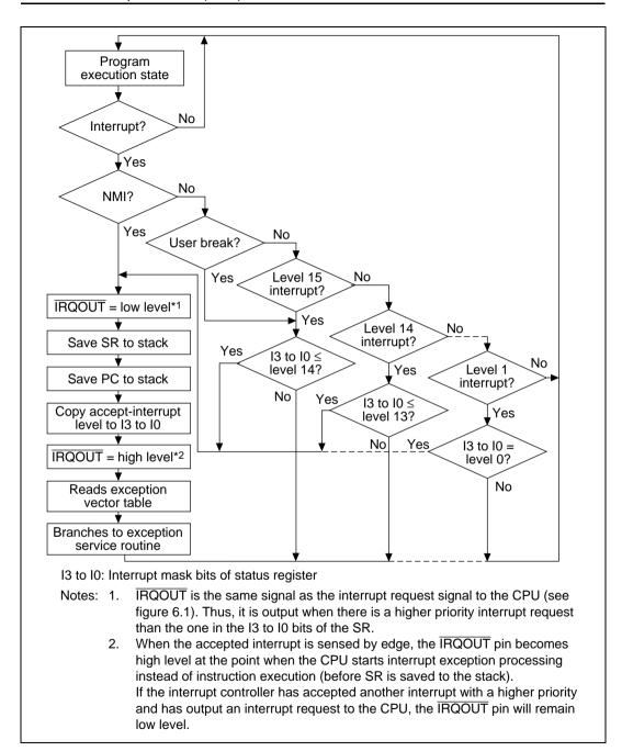
Figure 6.3 Interrupt Sequence Flowchart
