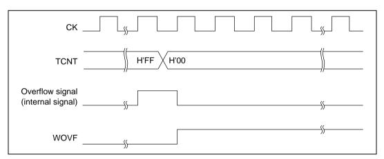
Figure 12.7 Timing of Setting the WOVF Bit
