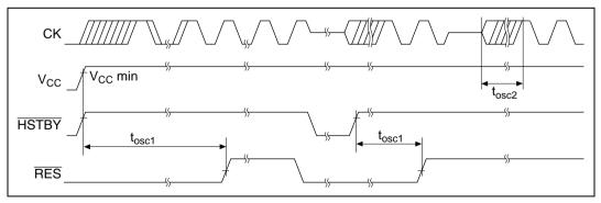
Figure 22.3 Oscillation Settling Time
