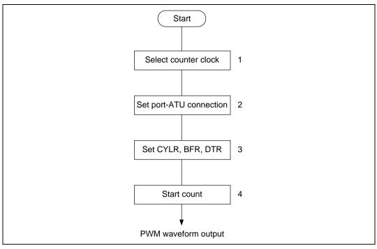
Figure 10.52 Sample Setup Procedure for PWM Timer Operation (Channels 6 to 9)
