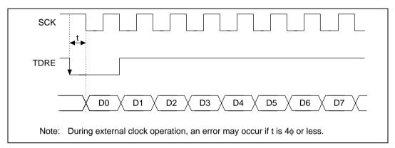
Figure 13.24 Example of Clock Synchronous Transmission with DMAC
