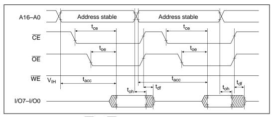
Figure 18.17  $\overline{\text{CE}}$  and  $\overline{\text{OE}}$  Clock System Read Timing Waveforms
