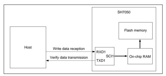
Figure 18.3 System Configuration in Boot Mode
