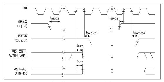
Figure 22.7 Bus Right Release Timing
