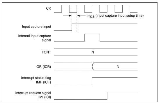
Figure 10.30 IMF (ICF) Setting Timing in Input Capture
