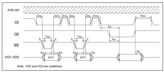
Figure 18.20 Status Read Mode Timing Waveforms
