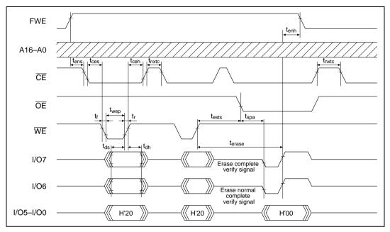
Figure 18.19 Auto-Erase Mode Timing Waveforms
