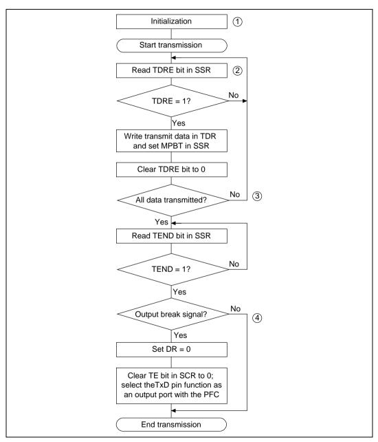
Figure 13.11 Sample Flowchart for Transmitting Multiprocessor Serial Data
