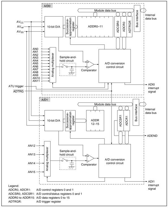
Figure 14.1 A/D Converter Block Diagram
