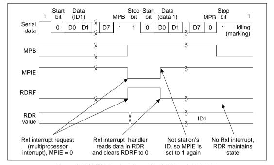
Figure 13.14 SCI Receive Operation (ID Does Not Match)
