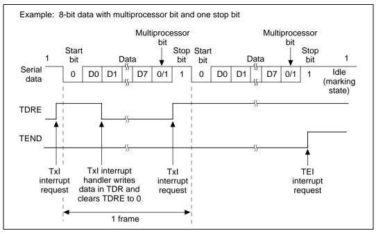
Figure 13.12 SCI Multiprocessor Transmit Operation
