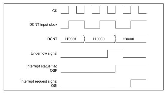
Figure 10.33 OSF Setting Timing in Underflow
