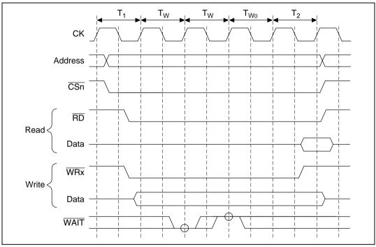
Figure 8.5 Wait State Timing of Ordinary Space Access (Wait States from Software Wait 2 State + WAIT Signal)
