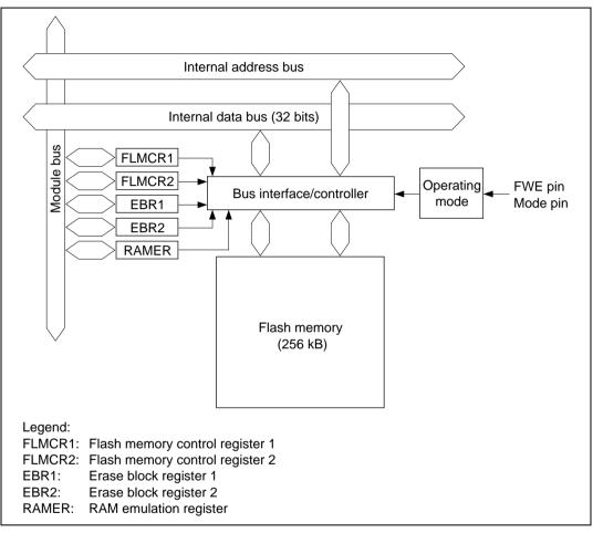
Figure 19.1 Block Diagram of Flash Memory
