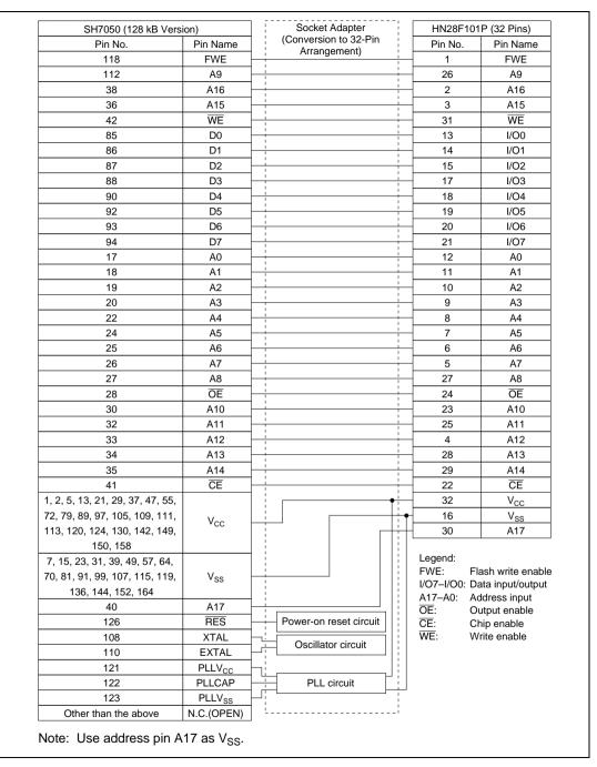
Figure 18.13 Socket Adapter Pin Correspondence Diagram
