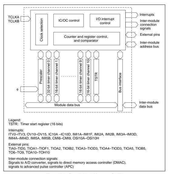
Figure 10.1 Overall Block Diagram of ATU
