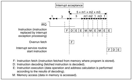
Figure 6.5 Pipeline when an IRQ Interrupt is Accepted
