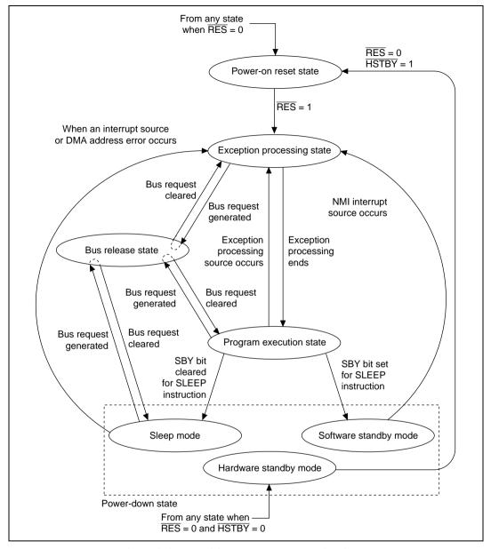
Figure 2.6 Transitions between Processing States
