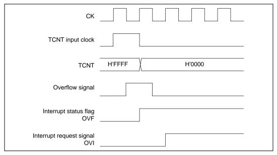
Figure 10.32 OVF Setting Timing in Overflow
