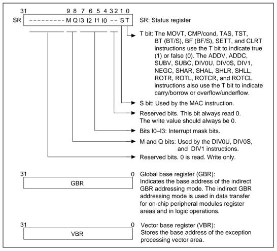
Figure 2.2 Control Register Configuration
