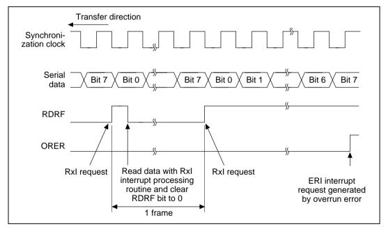
Figure 13.21 Example of SCI Receive Operation
