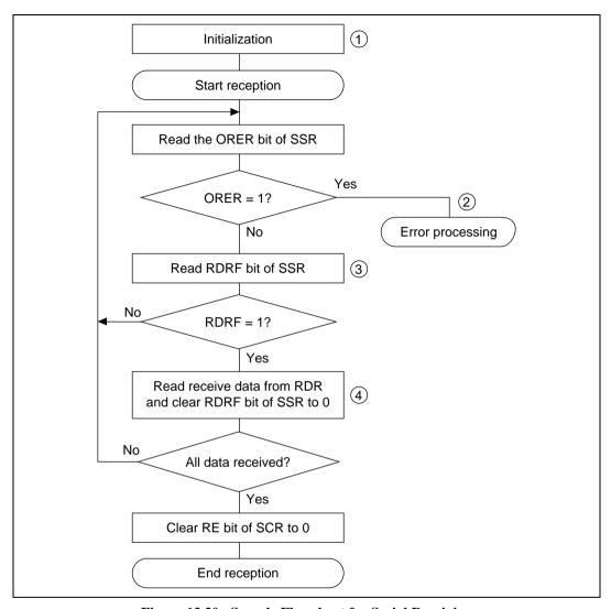
Figure 13.20 Sample Flowchart for Serial Receiving
