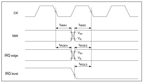
Figure 22.5 Interrupt Signal Input Timing
