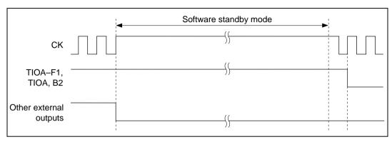
Figure 10.65 External Output Value Transition Points in Relation to Software Standby Mode
