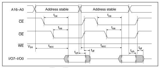
Figure 19.17  $\overline{\text{CE}}$  and  $\overline{\text{OE}}$  Clock System Read Timing Waveforms
