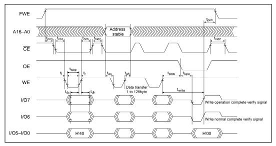
Figure 19.18 Auto-Program Mode Timing Waveforms
