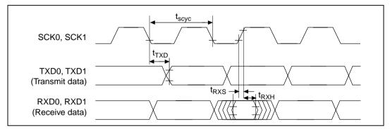
Figure 22.19 SCI I/O Timing (Clock Sync Mode)
