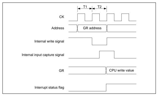
Figure 10.54 Contention between GR Write and Data Transfer by Input Capture
