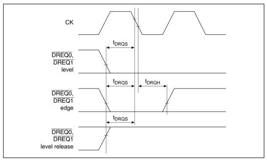
Figure 22.11 DREQ0 and DREQ1 Input Timing (1)
