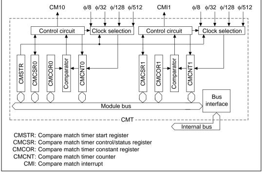
Figure 15.1 CMT Block Diagram
