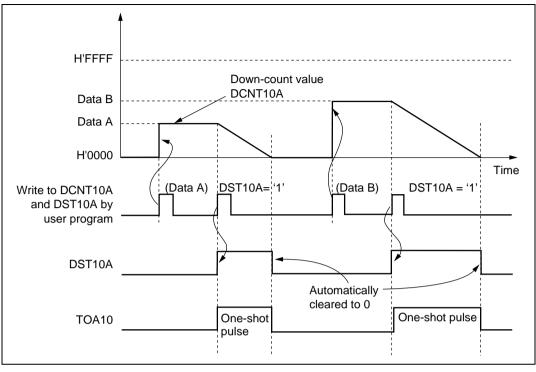
Figure 10.15 Example of One-Shot Pulse Operation
