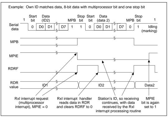
Figure 13.15 Example of SCI Receive Operation (ID Matches)
