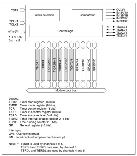
Figure 10.5 Block Diagram of Channels 3 and 4
