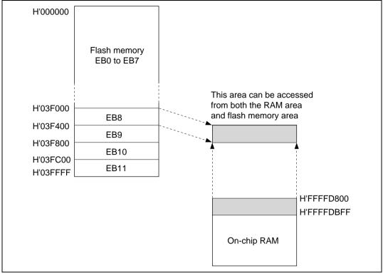
Figure 19.11 Example of RAM Overlap Operation
