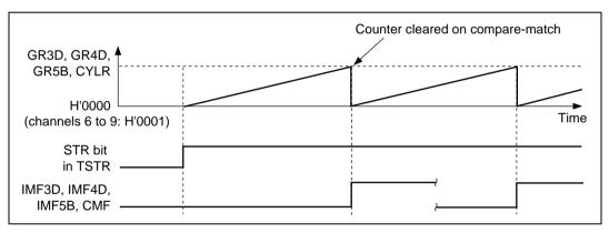
Figure 10.12 Cyclic Counter Operation
