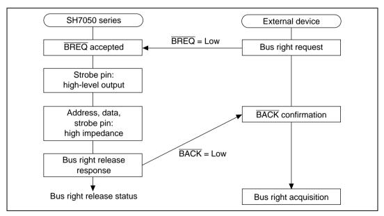
Figure 8.9 Bus Right Release Procedure
