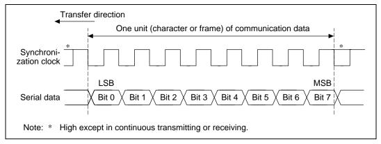
Figure 13.16 Data Format in Clock Synchronous Communication
