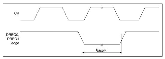
Figure 22.12 DREQ0 and DREQ1 Input Timing (2)
