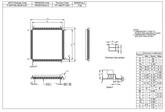
Figure D.1 Package Dimensions
