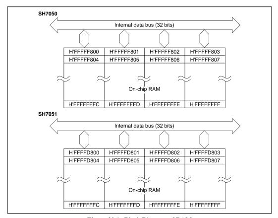
Figure 20.1 Block Diagram of RAM
