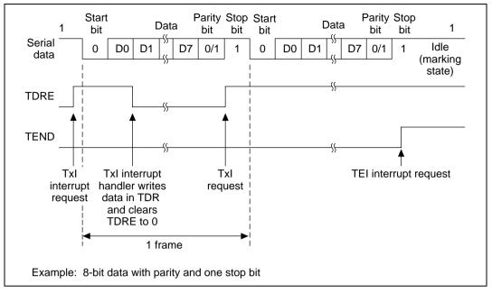
Figure 13.6 SCI Transmit Operation in Asynchronous Mode
