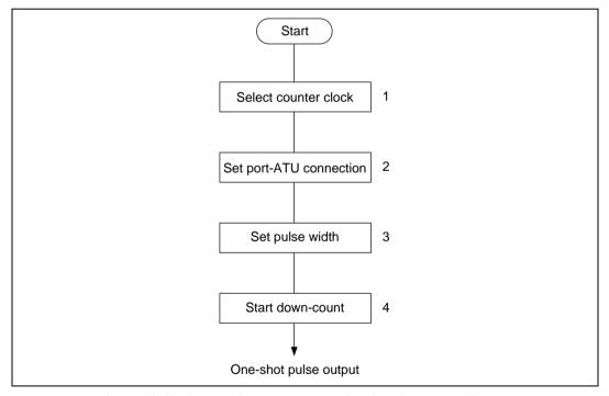
Figure 10.48 Sample Setup Procedure for One-Shot Pulse Output
