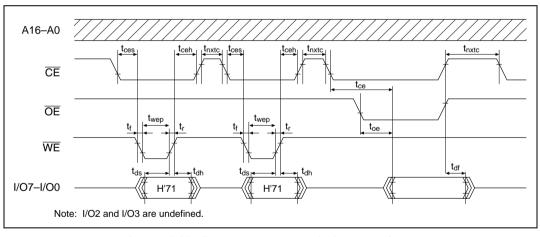
Figure 19.20 Status Read Mode Timing Waveforms
