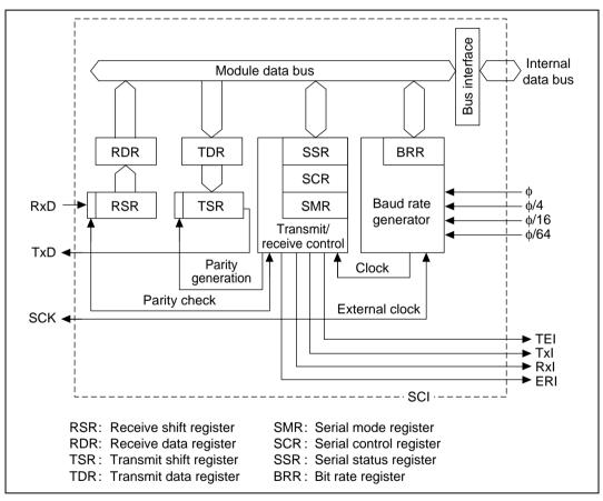
Figure 13.1 SCI Block Diagram
