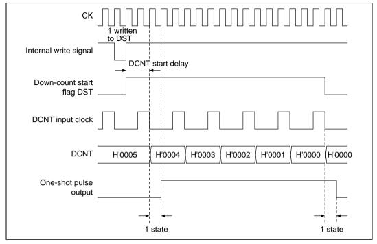
Figure 10.23 One-Shot Pulse Function Pulse Output Timing
