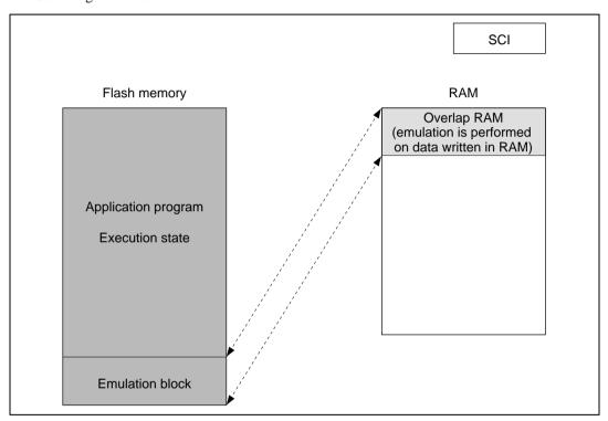
When overlap RAM data is confirmed, the RAMS bit is cleared, RAM overlap is released, and writes should actually be performed to the flash memory.
