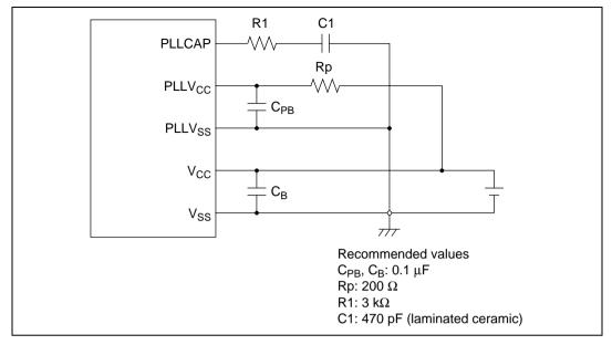
Figure 4.6 Points for Caution in PLL Power Supply Connection
