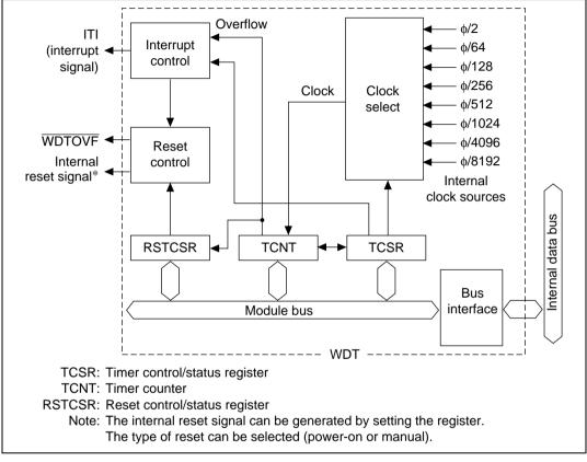
Figure 12.1 WDT Block Diagram
