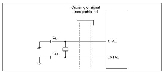
Figure 4.5 Cautions for Oscillator Circuit System Board Design
