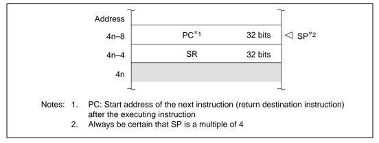
Figure 6.4 Stack after Interrupt Exception Processing
