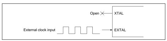
Figure 4.4 External Clock Input Method (Example)
