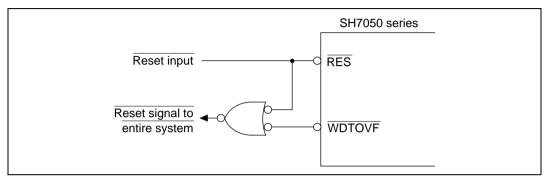
Figure 12.9 Example of a System Reset Circuit with a WDTOVF Signal
