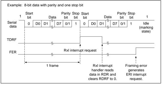
Figure 13.9 SCI Receive Operation
