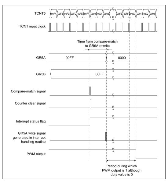
Figure 10.26 Channel 5 Waveform when Duty Changes from 100% to 0%
