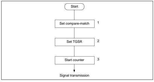
Figure 10.47 Sample Setup Procedure for Compare-Match Signal Transmission
