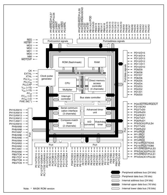
Figure 1.1 Block Diagram
