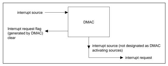
Figure 6.6 Block Diagram of Interrupt Controller
