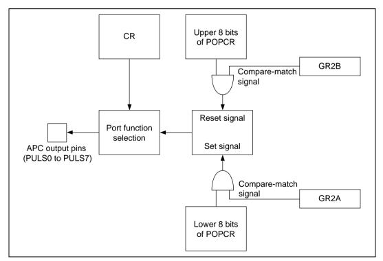
Figure 11.2 Advanced Pulse Controller Output Operation
