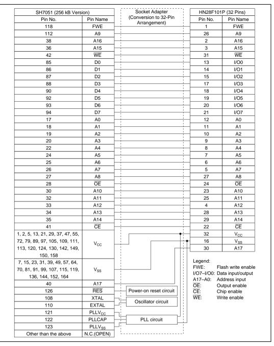
Figure 19.13 Socket Adapter Pin Correspondence Diagram
