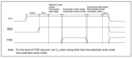
Figure 18.21 Oscillation Stabilization Time, Boot Program Transfer Time, and Power-Down Sequence
