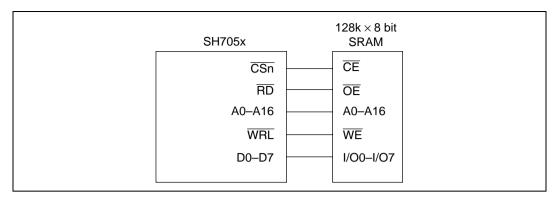
Figure 8.12 8-Bit Data Bus Width SRAM Connection
