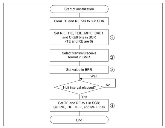
Figure 13.17 Sample Flowchart for SCI Initialization
