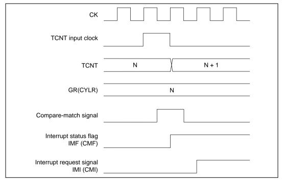
Figure 10.31 IMF (CMF) Setting Timing in Compare-Match
