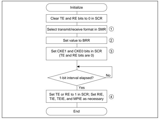
Figure 13.4 Sample Flowchart for SCI Initialization
