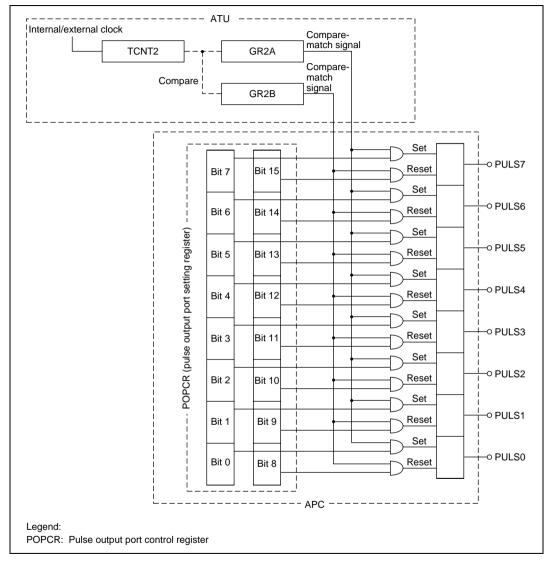
Figure 11.1 Advanced Pulse Controller Block Diagram
