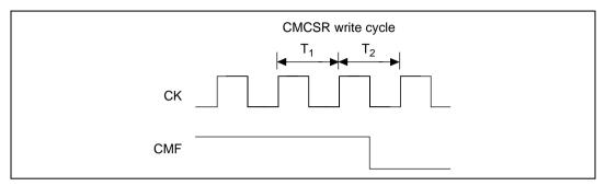
Figure 15.5 Timing of CMF Clear by the CPU
