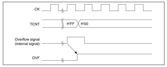
Figure 12.6 Timing of Setting the OVF
