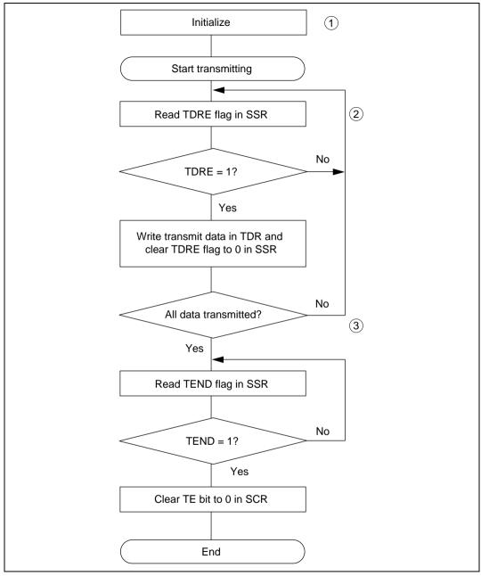
Figure 13.18 Sample Flowchart for Serial Transmitting
