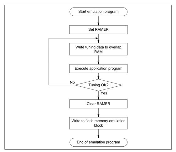
Figure 18.10 Flowchart for Flash Memory Emulation in RAM
