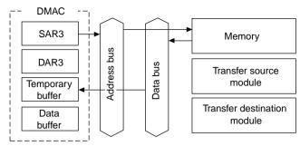
The SAR value is taken as the address, memory data is read, and the value is stored in the temporary buffer. Since the value read at this time is used as the address, it must be 32 bits.
