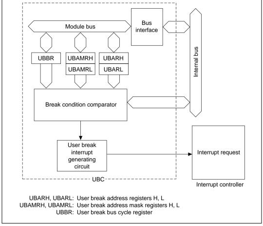
Figure 7.1 User Break Controller Block Diagram
