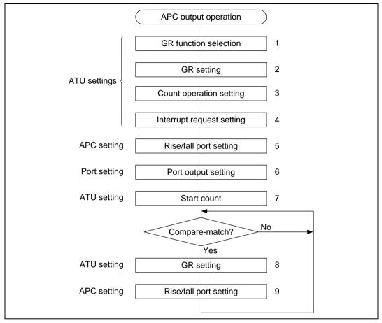
Figure 11.3 Example of Setting Procedure for Advanced Pulse Controller Output
