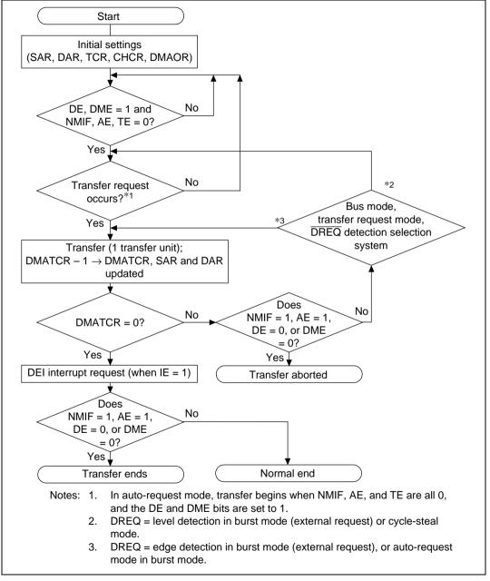
Figure 9.2 DMAC Transfer Flowchart
