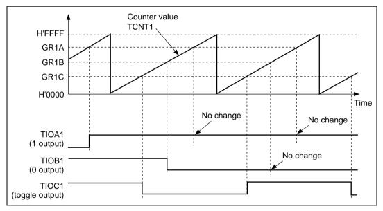
Figure 10.13 Example of Output Compare-Match Operation
