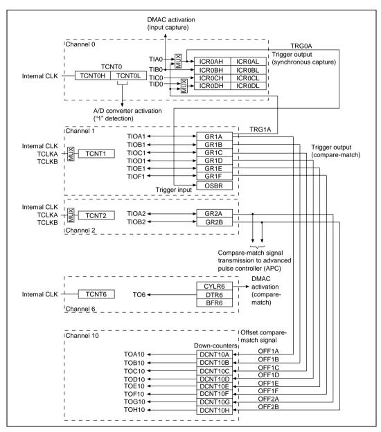
Figure 10.9 Inter-Channel and Inter-Module Signal Connection Diagram
