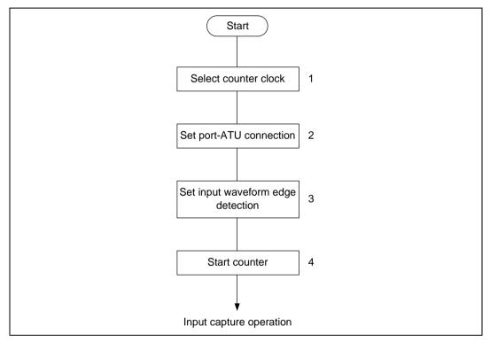
Figure 10.45 Sample Setup Procedure for Input Capture
