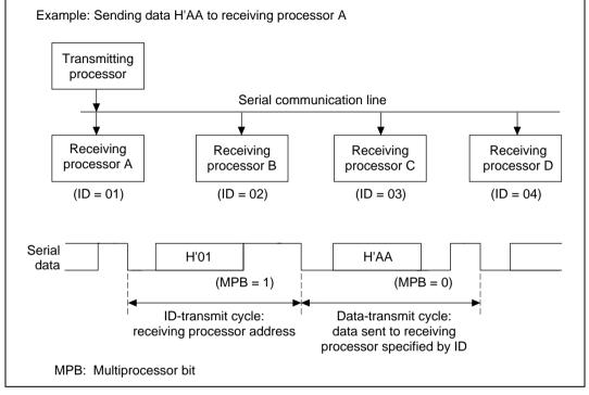
Figure 13.10 Communication Among Processors Using Multiprocessor Format
