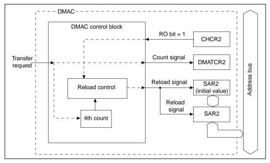
Figure 9.25 Source Address Reload Function
