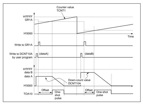
Figure 10.16 Example of Offset One-Shot Pulse Operation
