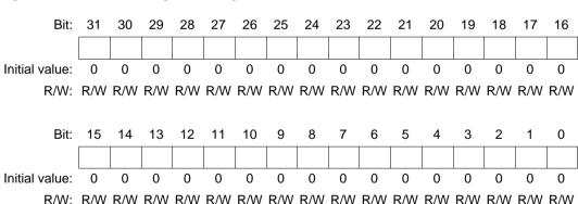
When TCNT0 overflows (from H'FFFFFFF to H'00000000), the OVF0 overflow flag in the timer status register (TSR) is set to 1.
