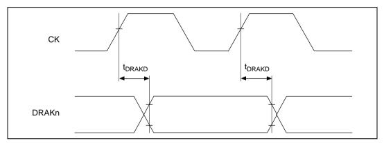
Figure 22.13 DRAK Output Delay Time
