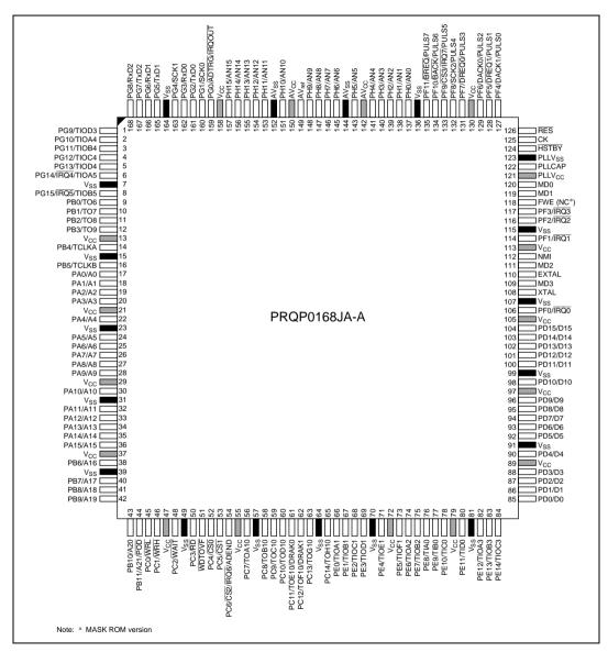
Figure 1.2 Pin Arrangement
