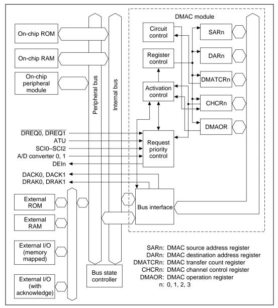
Figure 9.1 DMAC Block Diagram
