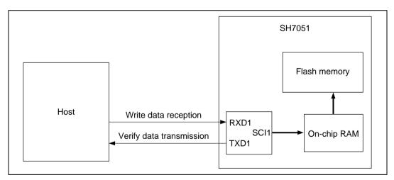
Figure 19.3 System Configuration in Boot Mode
