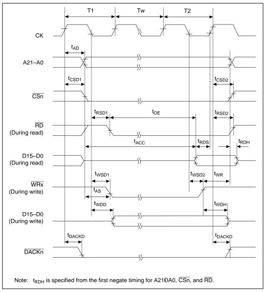
Figure 22.9 Basic Cycle (Software Waits)
