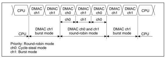
Figure 9.14 Bus Handling when Multiple Channels Are Operating
