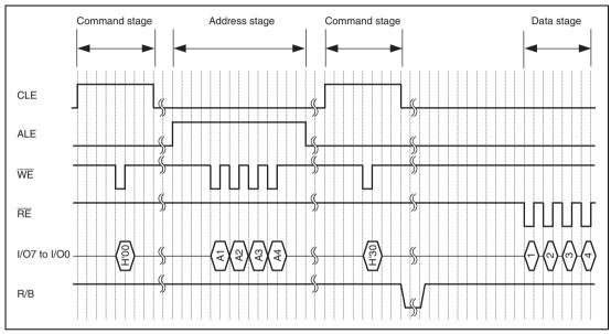
Figure 27.5 Reading Operation Timing for NAND-Type Flash Memory
