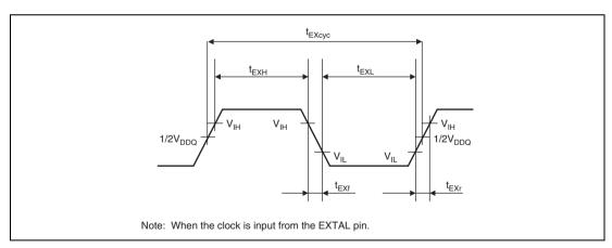
Figure 32.1 EXTAL Clock Input Timing
