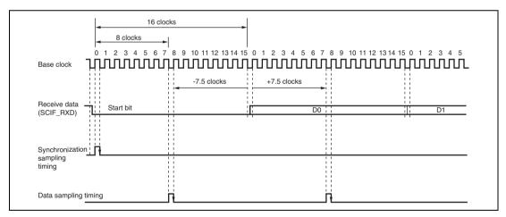
Figure 21.22 Receive Data Sampling Timing in Asynchronous Mode
