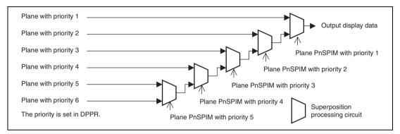
Figure 19.5 Plane Processing Sequence in α Blending and EOR Operation
