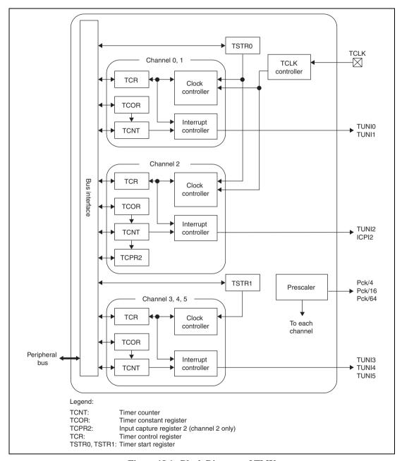
Figure 18.1 Block Diagram of TMU
