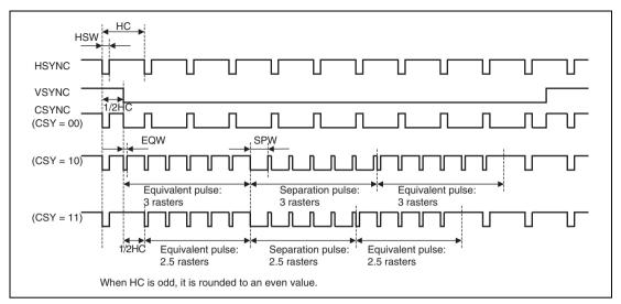
Figure 19.15 CSYNC Timing Chart (Last Half of Interlace Frame)
