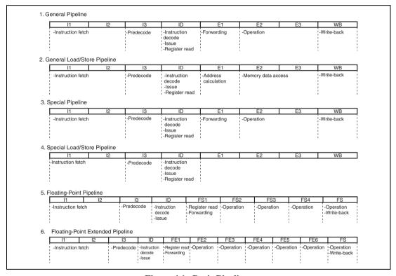
Figure 4.1 Basic Pipelines
