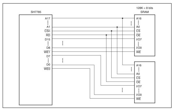
Figure 11.7 Example of 16-Bit Data Width SRAM Connection
