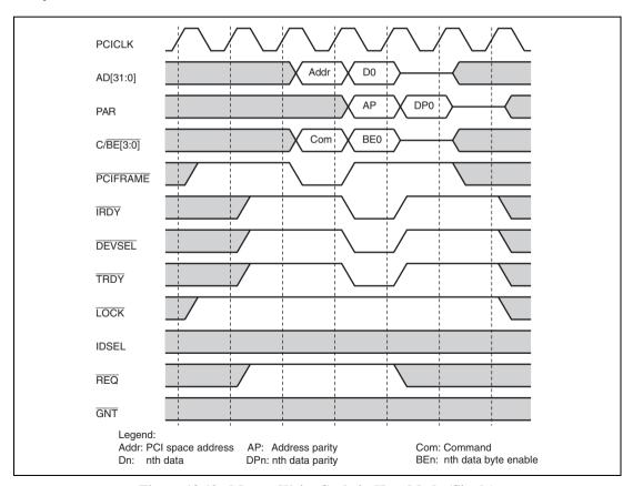
Figure 13.19 Master Write Cycle in Host Mode (Single)
