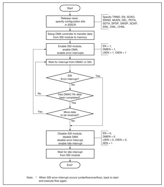
Figure 26.23 Reception Using DMA Controller
