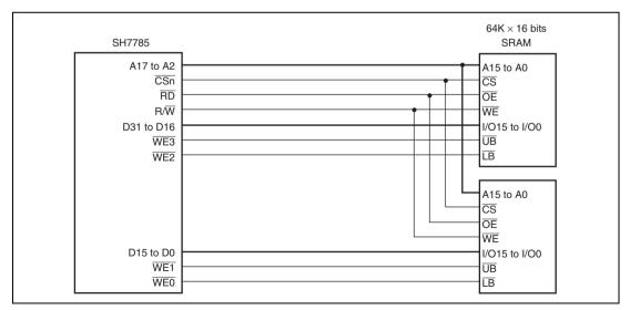
Figure 11.36 Example of Byte Control SRAM with 32-Bit Data Width
