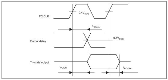
Figure 32.38 PCI Output Signal Timing
