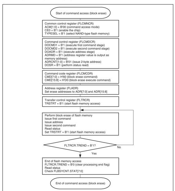
Figure 27.11 NAND Command Access (Block Erase)
