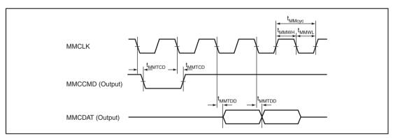
Figure 32.56 MMCIF Transmission Timing
