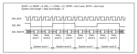
Figure 26.6 Multi-channel Format (4 Channels, No Padding)
