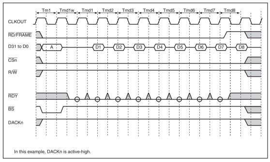
Figure 11.32 MPX Interface Timing 9 (Burst Read Cycle, IW = 0000, No External Wait, 32-Bit Bus Width, 32-Byte Data Transfer)
