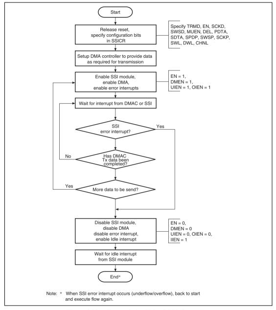
Figure 26.21 Transmission Using DMA Controller
