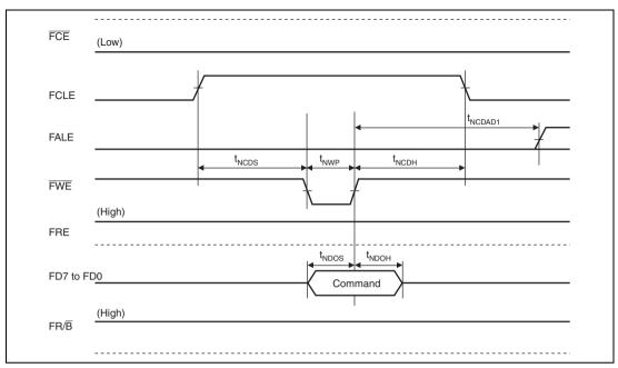
Figure 32.67 Command Issue Timing of NAND-Type Flash Memory
