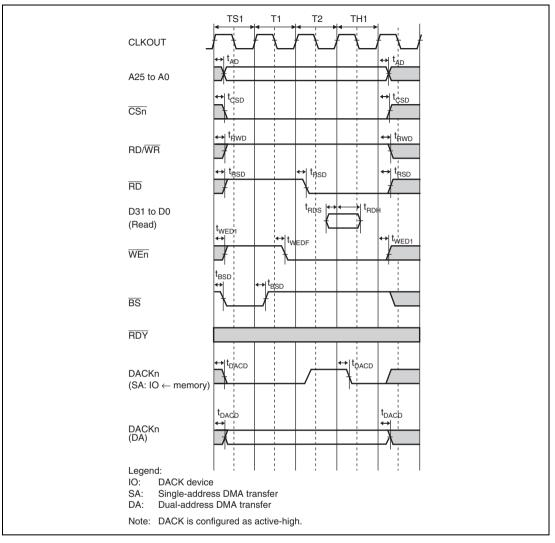
Figure 32.25 Memory Byte Control SRAM Bus Cycle: Basic Read Cycle (CSnWCR.IW = 0000, CSnWCR.RDS = 001, CSnWCR.WTS = 001, CSnWCR.RDH = 001, CSnWCR.WTH = 001)
