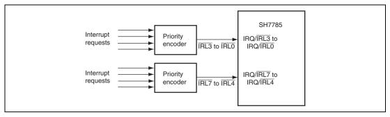
Figure 10.3 Example of IRL Interrupt Connection
