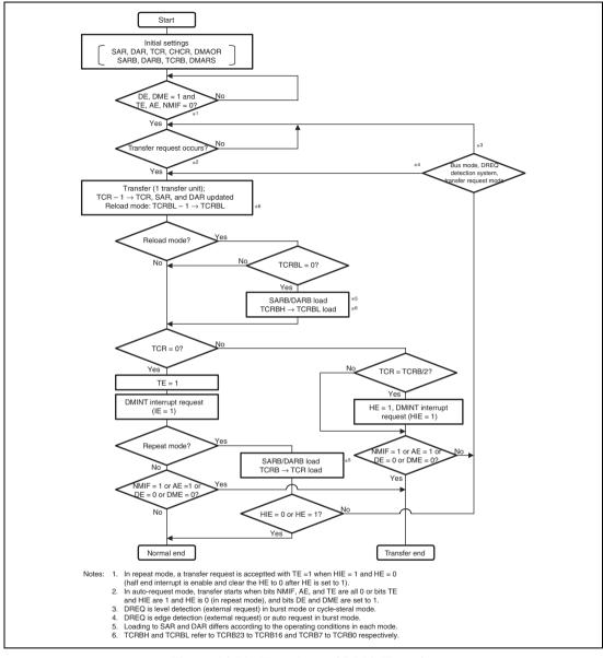
Figure 14.11 Flowchart of DMA Transfer
