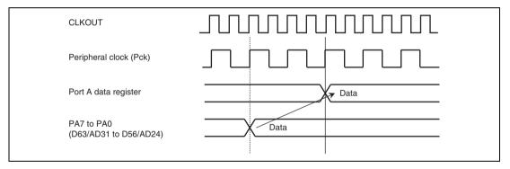
Figure 28.2 Port A Data Input Timing Diagram
