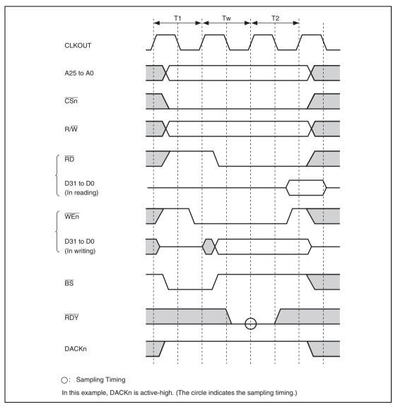
Figure 11.9 SRAM Interface Wait Timing (Software Wait Only)
