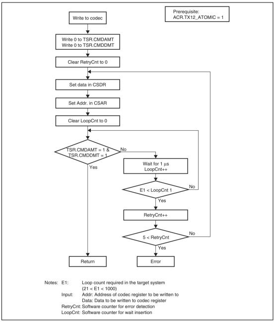
Figure 25.4 Sample Flowchart for Off-Chip Codec Register Write
