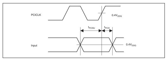
Figure 32.39 PCI Input Signal Timing
