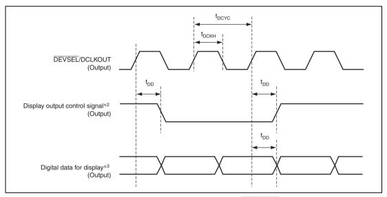
Figure 32.74 Display Timing (with Respect to DEVSEL/DCLKOUT)
