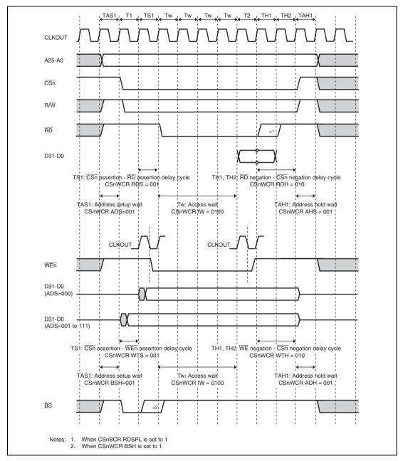
Figure 11.11 SRAM Interface Wait Timing (Read-Strobe/Write-Strobe Timing Setting)
