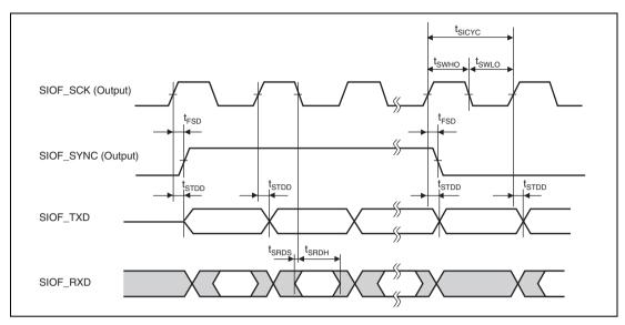
Figure 32.53 SIOF Transmission/Reception Timing (Master Mode 2, Sampling on Falling Edges)
