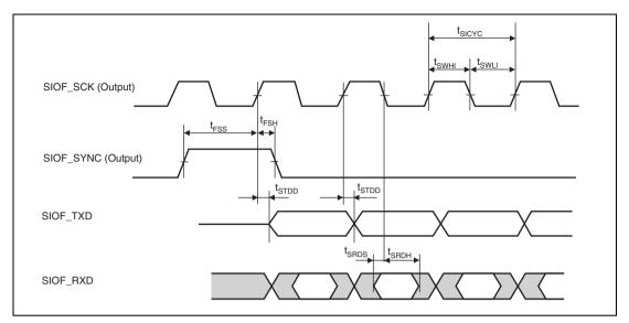
Figure 32.55 SIOF Transmission/Reception Timing (Slave Mode 1, Slave Mode 2)
