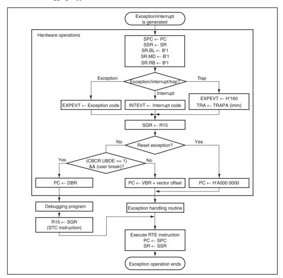
Figure 29.2 Flowchart of User Break Debugging Support Function
