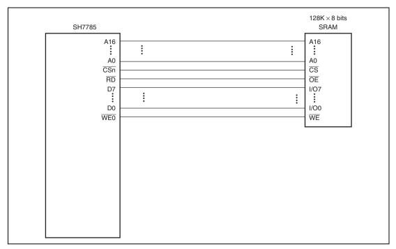
Figure 11.8 Example of 8-Bit Data Width SRAM Connection
