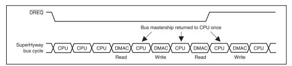
Figure 14.7 DMA Transfer Timing Example in Cycle Steal Normal Mode 2 (DREQ Low Level Detection)
