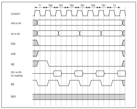
Figure 11.12 Burst ROM Basic Timing
