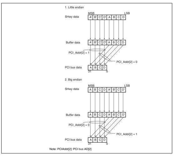
Figure 13.7 Endian Conversion from SuperHyway Bus to PCI Bus (Non-Byte Swapping: TBS = 0)
