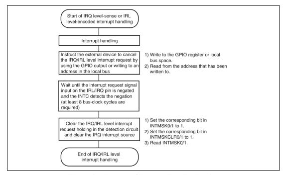
Figure 10.6 Example of Interrupt Handling Routine
