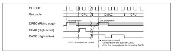
Figure 14.14 Example 2 of DREQ Input Detection in Cycle Steal Mode Edge Detection (Word Transfer in 8-Bit Bus Width, Longword Transfer in 8/16-Bit Bus Width, 16/32-Byte Transfer in 8/16/32/64-Bit Bus Width: DACK of DMA1 Transfer Divided)
