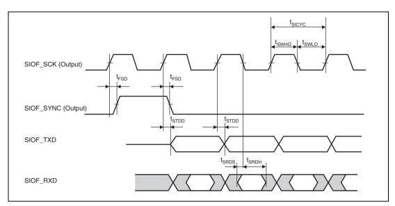
Figure 32.51 SIOF Transmission/Reception Timing (Master Mode 1, Sampling on Falling Edges)
