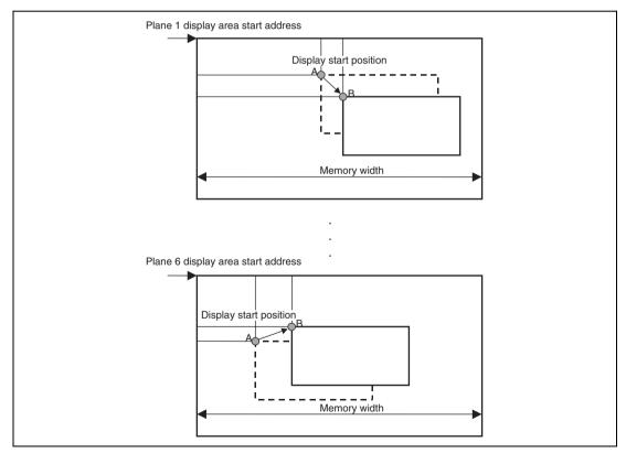
Figure 19.9 Schematic Diagram of Scroll Display
