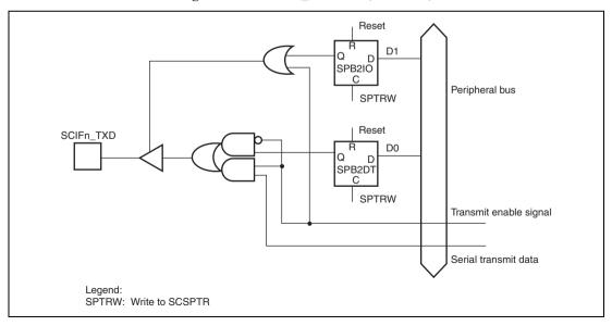
Figure 21.5 SCIFn\_TXD Pin (n = 0 to 5)
