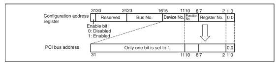
Figure 13.17 Address Generation for Type 0 Configuration Access
