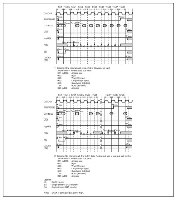
Figure 32.22 MPX Bus Cycle (Burst Read)
