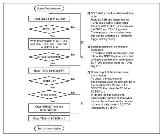
Figure 21.9 Sample Serial Transmission Flowchart
