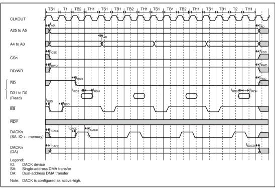
Figure 32.15 Burst ROM Bus Cycle (CSnWCR.IW = 0000, CSnWCR.RDS = 001, CSnWCR.WTS = 001, CSnWCR.RDH = 001, CSnWCR.WTH = 001)
