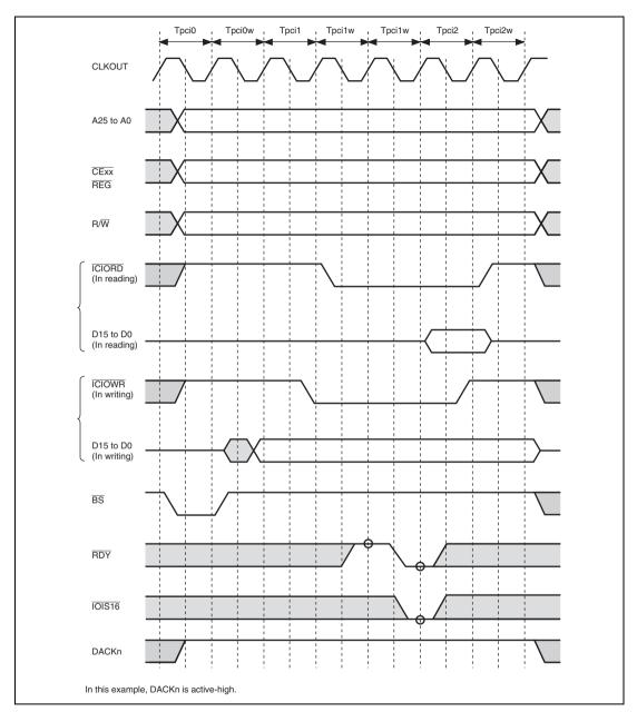
Figure 11.20 Wait Timing for PCMCIA I/O Card Interface
