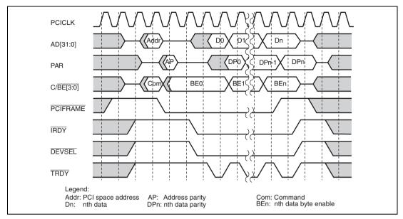
Figure 13.28 Target Memory Read Cycle in Host Bus Bridge Mode (Burst, with Stepping)
