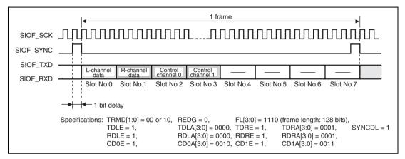
Figure 22.18 Transmit and Receive Timing (16-Bit Stereo Data (3))
