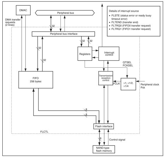
Figure 27.1 Block Diagram of FLCTL
