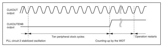
Figure 15.3 End of the Change of the Bus Clock Frequency
