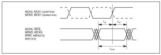
Figure 32.27 Command Signal and MCK Output Clock
