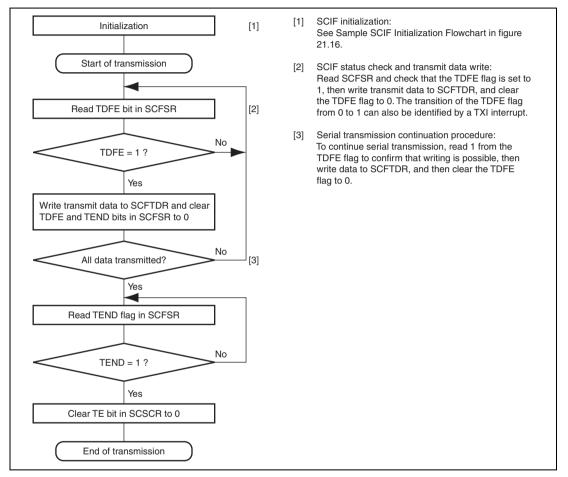
Figure 21.17 Sample Serial Transmission Flowchart
