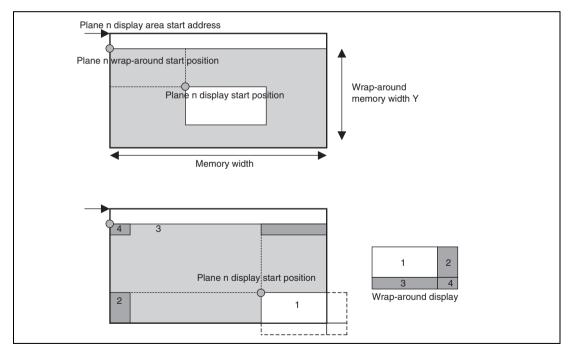
Figure 19.10 Schematic Diagram of Wraparound Display
