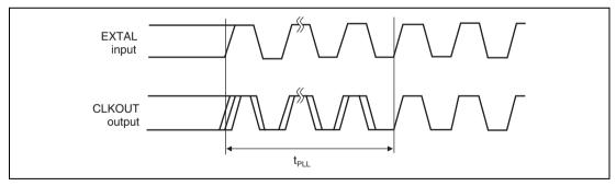
Figure 32.5 PLL Synchronization Settling Time
