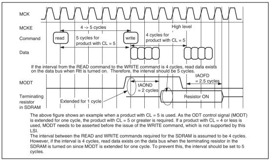
Figure 12.22 Important Information on One-Cycle Extension of ODT Control Signal
