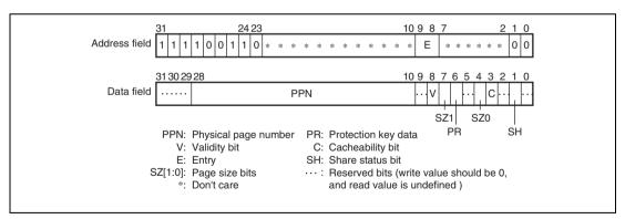
Figure 7.19 Memory-Mapped ITLB Data Array (TLB Compatible Mode)
