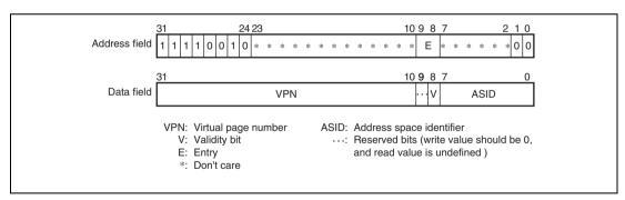
Figure 7.18 Memory-Mapped ITLB Address Array
