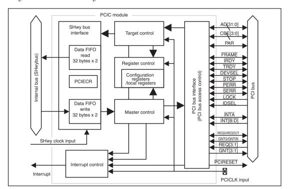
Figure 13.1 shows a block diagram of the PCIC.
