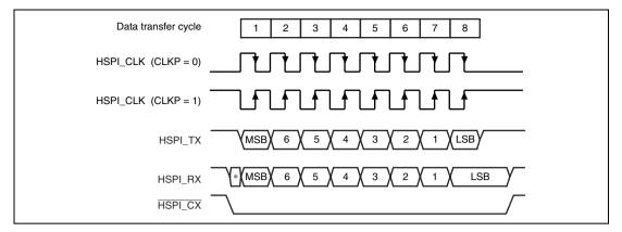
Figure 23.5 Timing Conditions when FBS = 1
