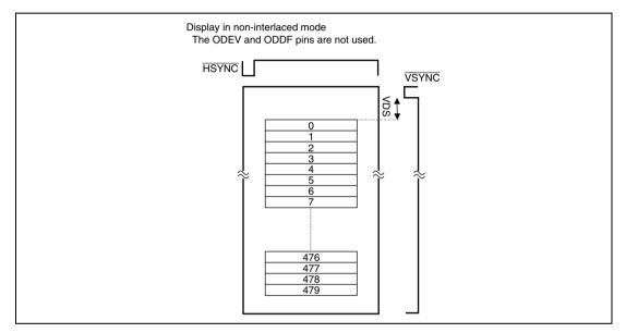
Figure 19.17 Display in Non-Interlaced Method
