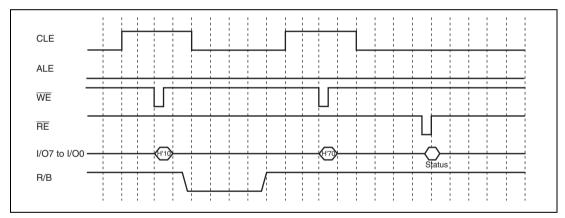
Figure 27.4 Status Read Operation Timing for NAND-Type Flash Memory
