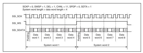
Figure 26.8 Multi-channel Format (8 Channels, Serial Data First, Followed by Padding Bits, with Padding)
