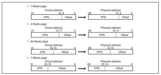
Figure 7.7 Relationship between Page Size and Address Format (TLB Compatible Mode)
