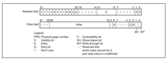
Figure 7.24 Memory-Mapped UTLB Data Array 1 (TLB Extended Mode)
