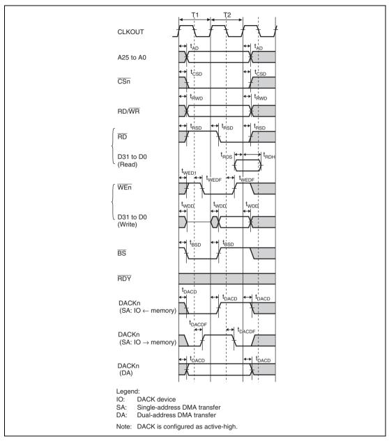
Figure 32.9 SRAM Bus Cycle: Basic Bus Cycle (No Wait)
