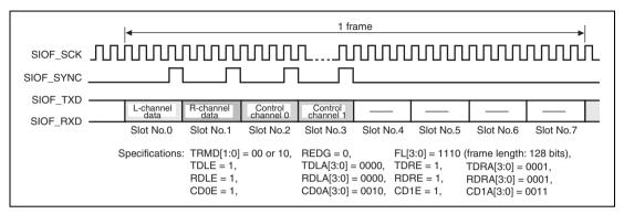
Figure 22.20 Transmit and Receive Timing (16-Bit Stereo Data)
