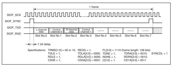
Figure 22.19 Transmit and Receive Timing (16-Bit Stereo Data (4))
