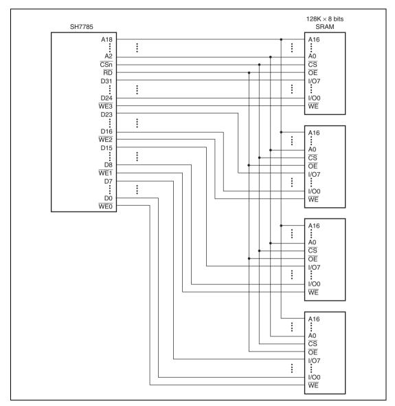
Figure 11.6 Example of 32-Bit Data Width SRAM Connection
