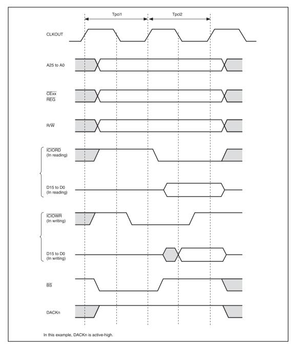
Figure 11.19 Basic Timing for PCMCIA I/O Card Interface
