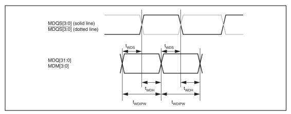
Figure 32.32 MDQS and MDQ/MDM Output Waveform (Write)
