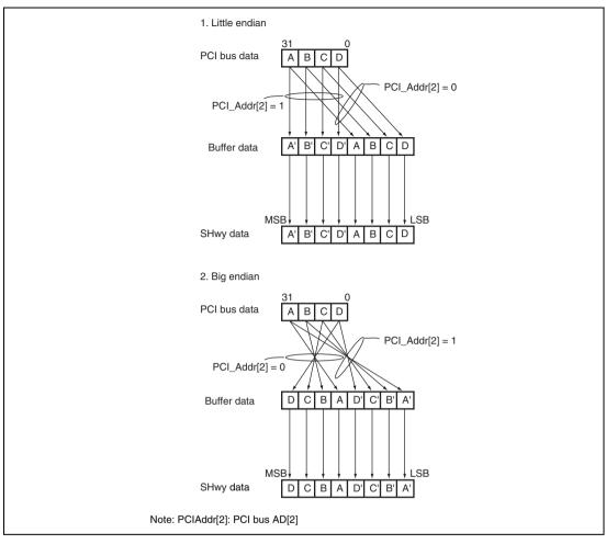
Figure 13.14 Endian Conversion from PCI Bus to SuperHyway Bus (Byte Swapping: TBS = 1)
