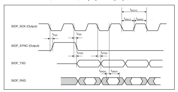
Figure 32.52 SIOF Transmission/Reception Timing (Master Mode 1, Sampling on Rising Edges)
