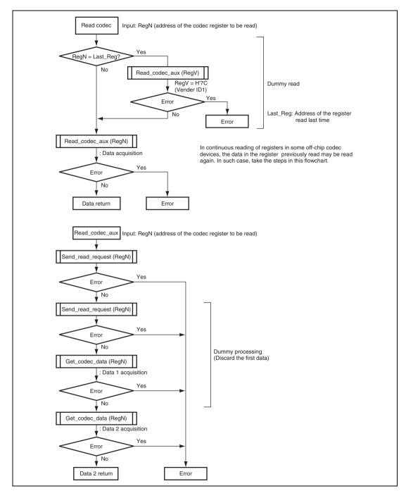
Figure 25.5 Sample Flowchart for Off-Chip Codec Register Read (1)
