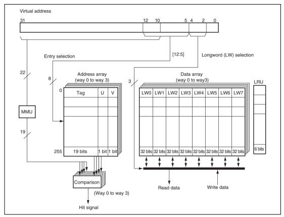
Figure 8.1 Configuration of Operand Cache (Cache size = 32 Kbytes)
