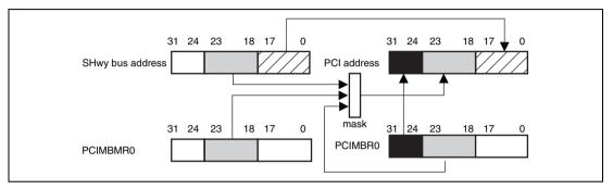
Figure 13.3 Access from SuperHyway Bus to PCI Memory (PCI Bus) (PCI Memory Space 0)
