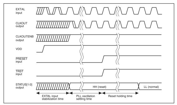
Figure 16.3 STATUS Output when Power Is Turned On
