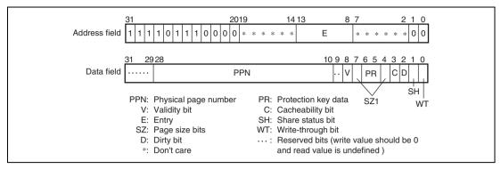
Figure 7.23 Memory-Mapped UTLB Data Array (TLB Compatible Mode)
