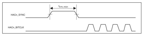
Figure 32.59 HAC Warm Reset Timing
