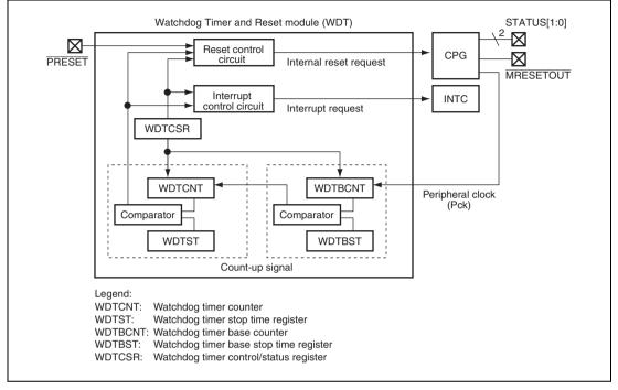
Figure 16.1 Block Diagram of WDT
