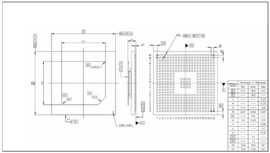
Figure A.1 Package Dimensions (436-Pin BGA)
