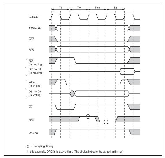
Figure 11.10 SRAM Interface Wait Timing (Wait Cycle Insertion by RDY Signal, RDY Signal Is Synchronous Input)
