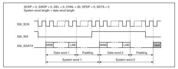
Figure 26.3 Philips Format (with Padding)
