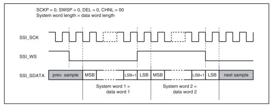
Figure 26.2 Philips Format (with No Padding)
