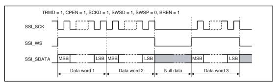
Figure 26.19 Compressed Data Format, Master Transmitter, and Burst Mode Enabled
