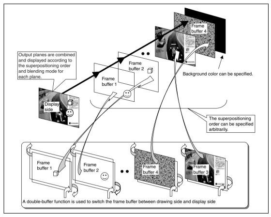
Figure 19.2 Block Diagram of Plane Configuration and Superpositioning
