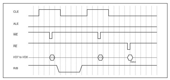
Figure 27.7 Status Read Operation Timing for NAND-Type Flash Memory
