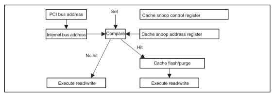
Figure 13.16 Cache Flush/Purge Execution Flow from PCI Bus to SuperHyway Bus
