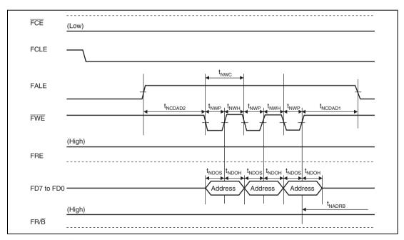
Figure 32.68 Address Issue Timing of NAND-Type Flash Memory
