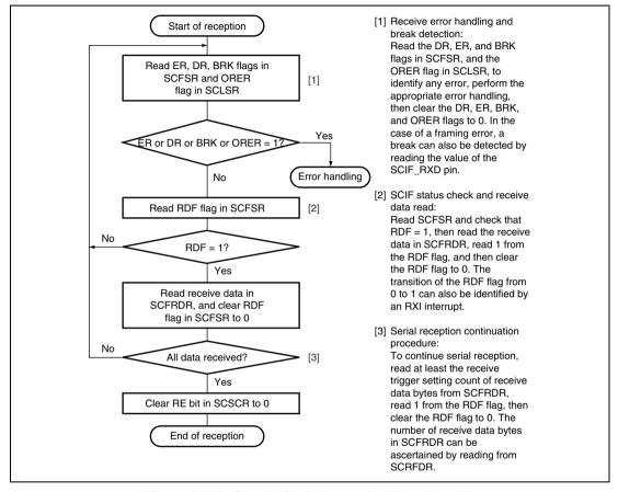
Figure 21.12 Sample Serial Reception Flowchart (1)
