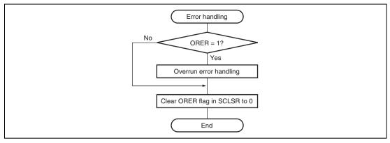
Figure 21.19 Sample Serial Reception Flowchart (2)
