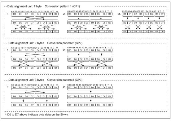
Figure 20.8 Data Alignment Conversion Pattern
