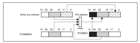
Figure 13.5 Access from SuperHyway Bus to PCI Memory (PCI Bus) (PCI Memory Space 2)
