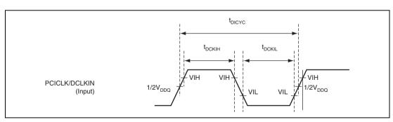
Figure 32.72 PCICLK/DCLKIN Clock Input Timing
