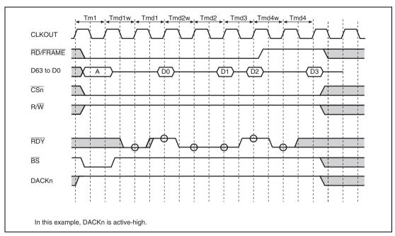
Figure 11.29 MPX Interface Timing 6 (Burst Read Cycle, IW = 0000, External Wait Control, 64-Bit Bus Width, 32-Byte Data Transfer)
