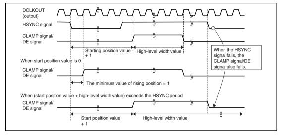
Figure 19.20 CLAMP Signal and DE Signal
