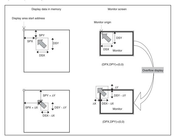
Figure 19.11 Schematic Diagram of Upper-Left Overflow Display
