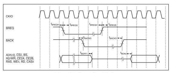
Figure 32.7 Control Signal Timing
