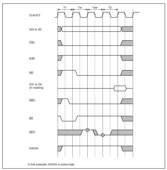
Figure 11.40 Wait State Timing of Byte Control SRAM (One Internal Wait + One External Wait)
