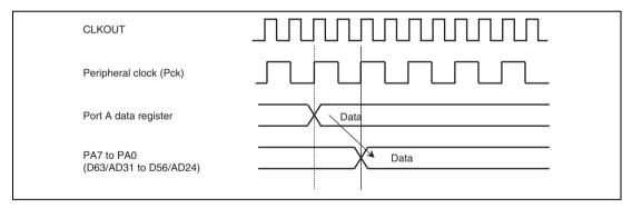
Figure 28.1 Port A Data Output Timing Diagram
