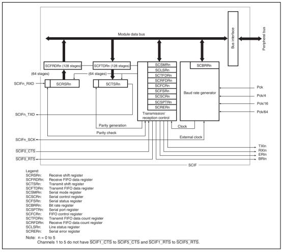
Figure 21.1 Block Diagram of SCIF
