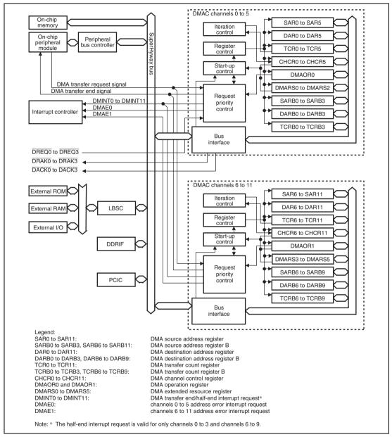
Figure 14.1 Block Diagram of DMAC
