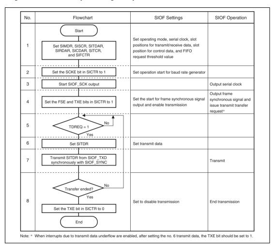
Figure 22.9 Example of Transmit Operation in Master Mode
