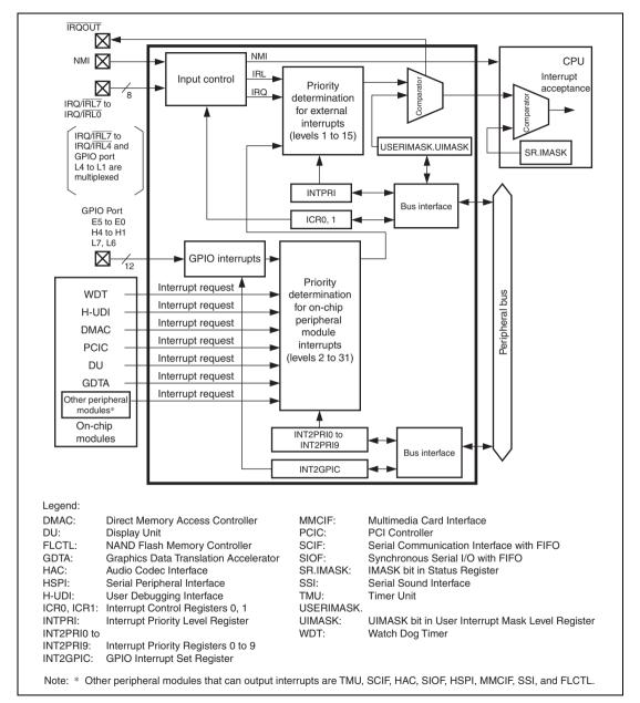
Figure 10.1 Block Diagram of INTC
