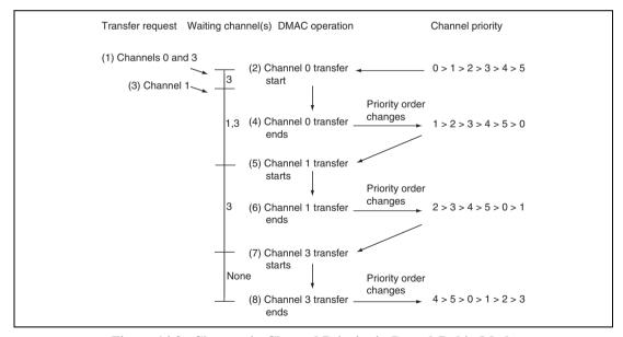
Figure 14.3 Changes in Channel Priority in Round-Robin Mode (Example of Channels 0 to 5)
