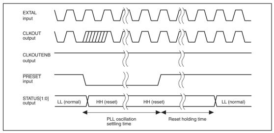
Figure 16.4 STATUS Output by Power-On Reset Caused by PRESET Input during Normal Operation
