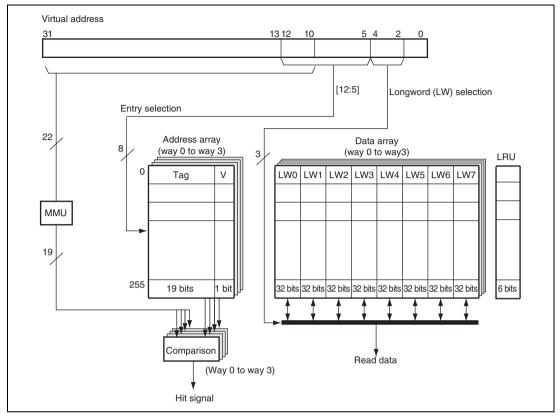
Figure 8.2 Configuration of Instruction Cache (Cache size = 32 Kbytes)
