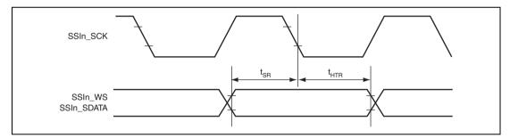
Figure 32.66 SSI Reception Timing (2)
