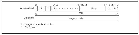
Figure 8.8 Memory-Mapped OC Data Array (Cache size = 32 Kbytes)
