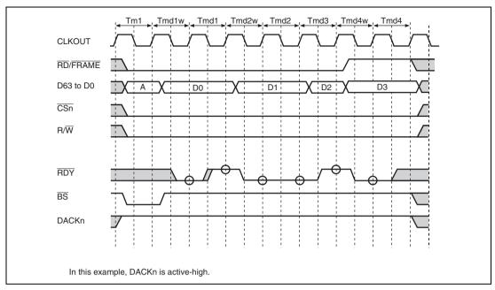
Figure 11.31 MPX Interface Timing 8 (Burst Write Cycle, IW = 0001, External Wait Control, 32-Bit Bus Width, 32-Byte Data Transfer)
