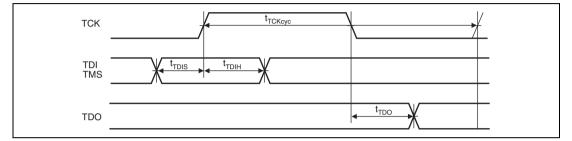
Figure 32.46 H-UDI Data Transfer Timing
