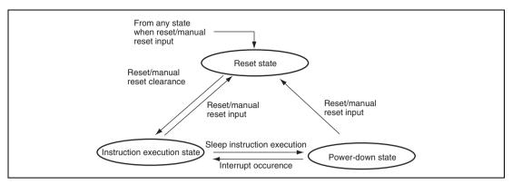
Figure 2.8 Processing State Transitions
