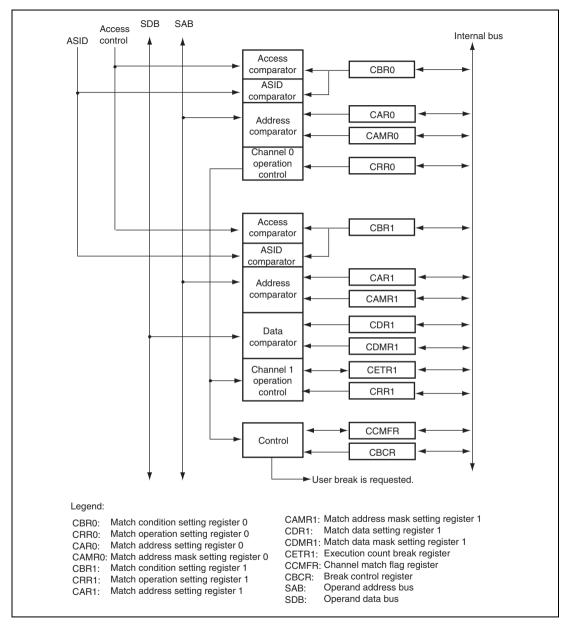
Figure 29.1 Block Diagram of UBC
