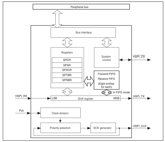
Figure 23.1 Block Diagram of HSPI
