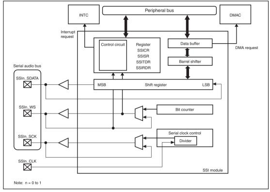
Figure 26.1 Block Diagram of SSI Module
