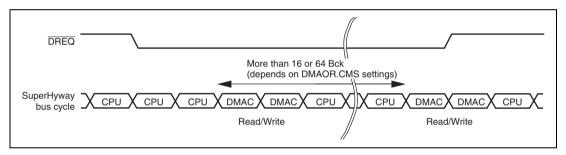
Figure 14.8 Example e of DMA Transfer Timing in Cycle Steal Intermittent Mode (DREQ Low Level Detection)
