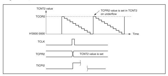
Figure 18.6 Operation Timing when Using Input Capture Function
