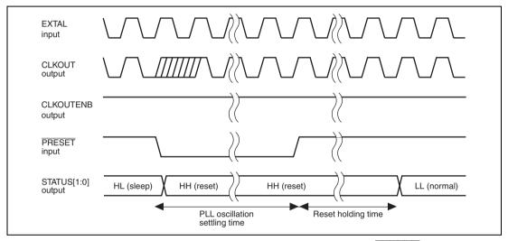
Figure 16.5 STATUS Output by Power-On Reset Caused by PRESET Input in Sleep Mode
