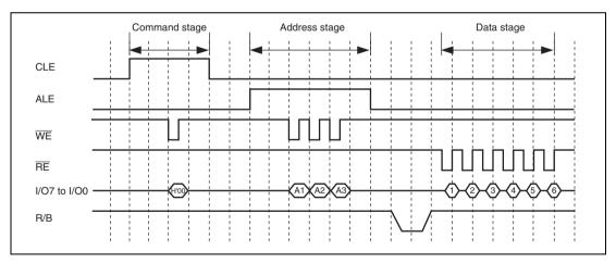
Figure 27.2 Reading Operation Timing for NAND-Type Flash Memory
