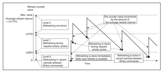
Figure 12.7 Relation between Auto-Refresh Operation and Threshold Values
