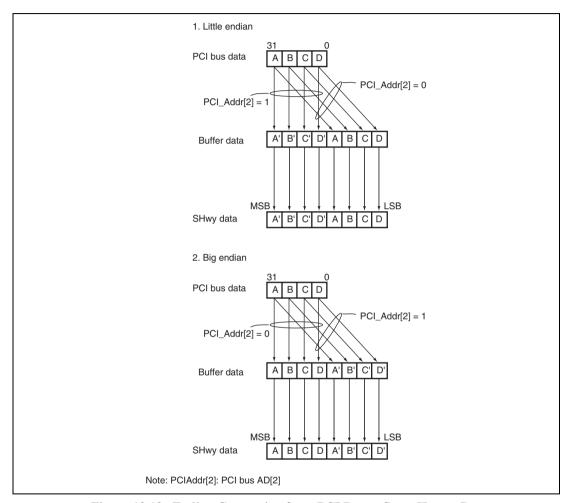
Figure 13.13 Endian Conversion from PCI Bus to SuperHyway Bus (Non-Byte Swapping: TBS = 0)
