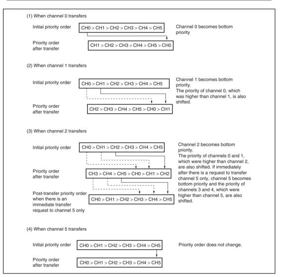
Figure 14.2 Round-Robin Mode (Example of Channels 0 to 5)
