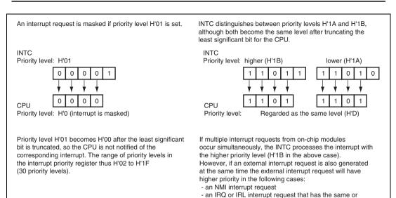
Figure 10.4 Priority of On-Chip Peripheral Module Interrupts
