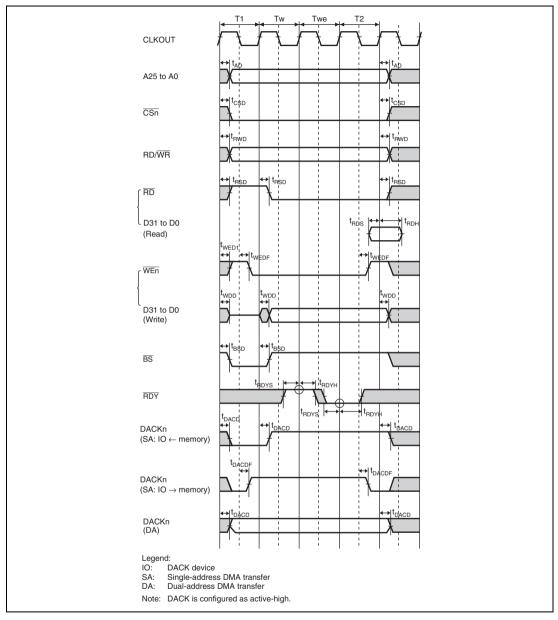
Figure 32.11 SRAM Bus Cycle: Basic Bus Cycle (One Internal Wait Cycle + One External Wait Cycle)
