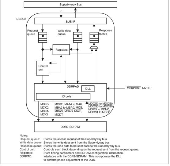
Figure 12.1 Block Diagram of the DBSC2
