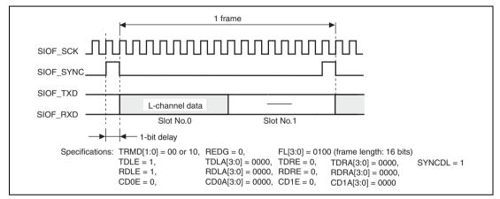
Figure 22.14 Transmit and Receive Timing (8-Bit Monaural Data (2))
