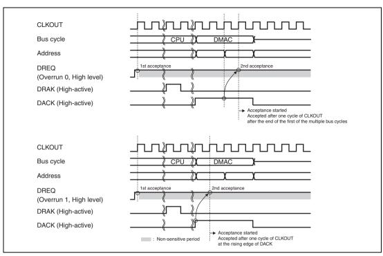
Figure 14.22 Example 3 of DREQ Input Detection in Burst Mode Level Detection (Word Transfer in 8-Bit Bus Width, Longword Transfer in 8/16-Bit Bus Width, or 16/32-Byte Transfer in 8/16/32/64-Bit Bus Width: DACK of DMA1 Transfer Is Connected)
