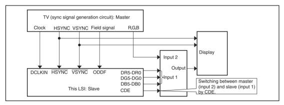
Figure 19.12 Signal Flow in TV Sync Mode
