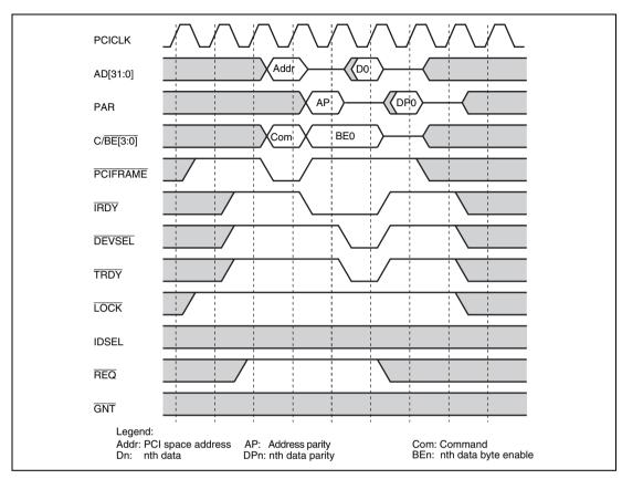
Figure 13.20 Master Read Cycle in Host Mode (Single)
