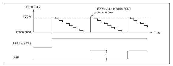
Figure 18.3 TCNT Auto-Reload Operation
