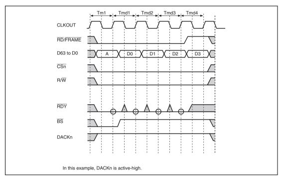
Figure 11.30 MPX Interface Timing 7 (Burst Write Cycle, IW = 0000, No External Wait, 64-Bit Width, 32-Byte Data Transfer)
