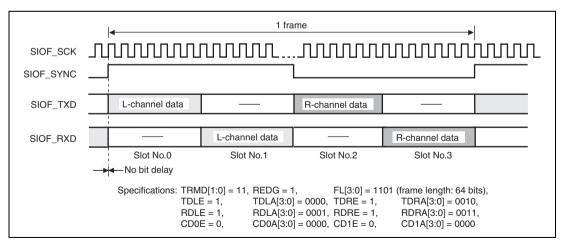
Figure 22.17 Transmit and Receive Timing (16-Bit Stereo Data (2))
