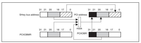
Figure 13.6 Access from SuperHyway Bus to PCI I/O Space (PCI Bus)
