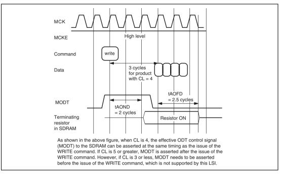
Figure 12.21 ODT Control Signal when CL = 4
