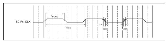
Figure 32.42 SCIFn\_CLK Input Clock Timing
