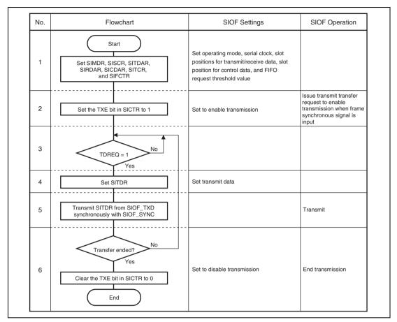
Figure 22.11 Example of Transmit Operation in Slave Mode
