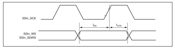
Figure 32.65 SSI Reception Timing (1)
