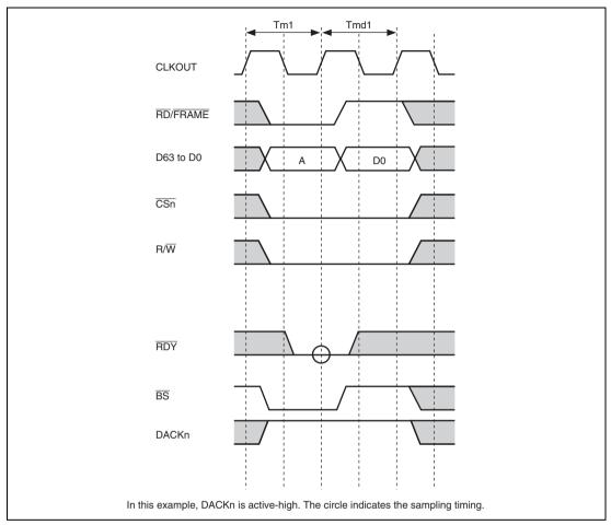
Figure 11.26 MPX Interface Timing 3 (Single Write Cycle, IW = 0000, No External Wait, 64-Bit Bus Width)
