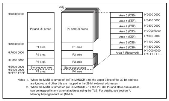
Figure 11.2 Correspondence between Virtual Address Space and Local Bus Memory Space
