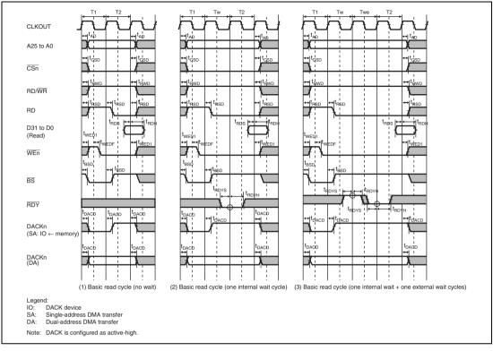
Figure 32.24 Memory Byte Control SRAM Bus Cycle
