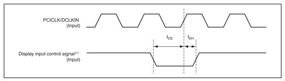
Figure 32.73 Display Timing (with Respect to PCICLK/DCLKIN)
