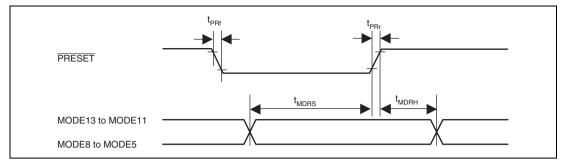
Figure 32.6 MODE Pin Setup/Hold Timing
