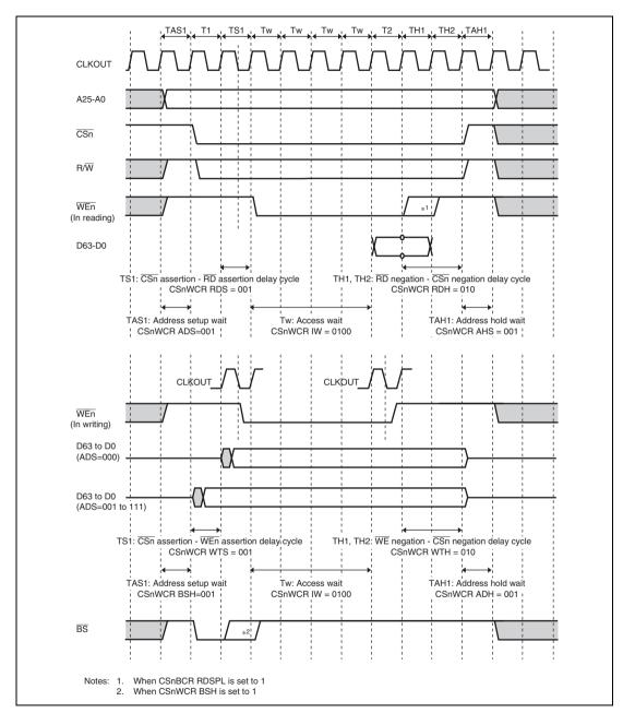
Figure 11.39 Wait State Timing of Byte Control SRAM
