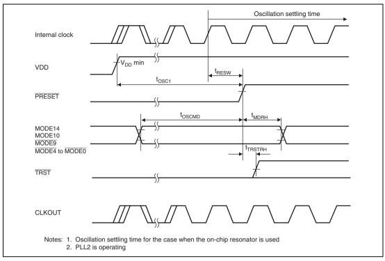
Figure 32.4 Power-On Oscillation Settling Time
