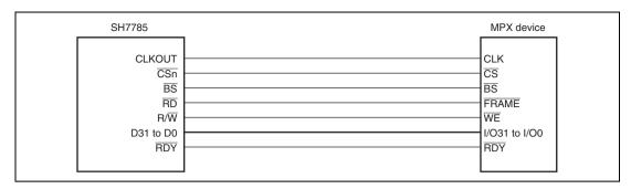
Figure 11.22 Example of 32-Bit Data Width MPX Connection
