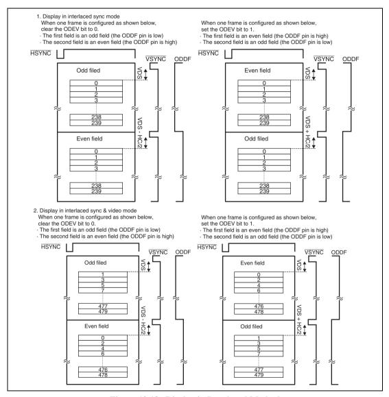
Figure 19.18 Display in Interlaced Method
