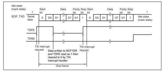
Figure 21.10 Example of SCIF Transmission Operation (Example with 8-Bit Data, Parity, One Stop Bit)
