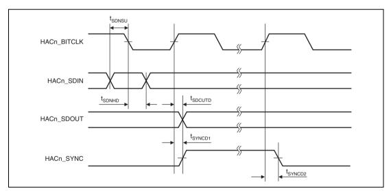
Figure 32.61 HAC Interface Module Signal Timing
