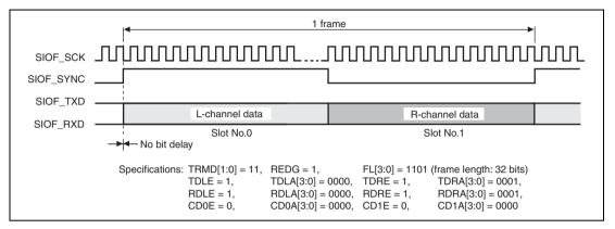
Figure 22.16 Transmit and Receive Timing (16-Bit Stereo Data (1))
