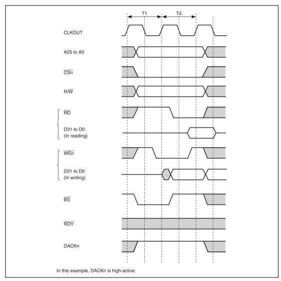
Figure 11.5 Basic Timing of SRAM Interface
