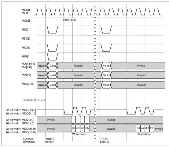
Figure 12.2 Burst Access Operation
