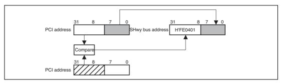
Figure 13.12 I/O Access from PCI Bus to SuperHyway Bus
