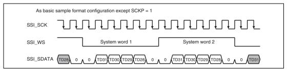
Figure 26.10 Inverted Clock
