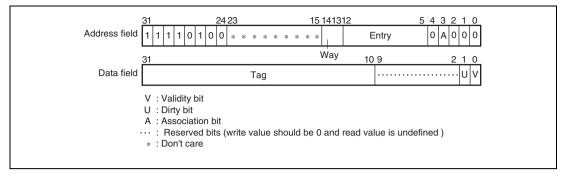
Figure 8.7 Memory-Mapped OC Address Array (Cache size = 32 Kbytes)
