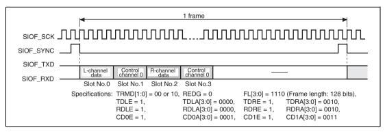
Figure 22.7 Control Data Interface (Slot Position)
