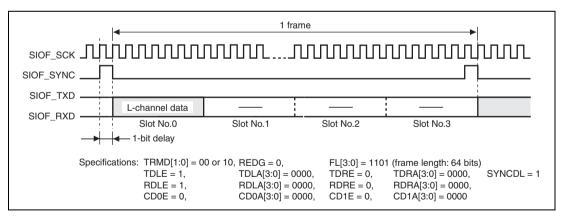
Figure 22.15 Transmit and Receive Timing (16-Bit Monaural Data)
