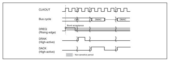
Figure 14.19 Example of DREQ Input Detection in Burst Mode Edge Detection
