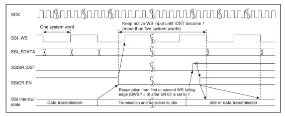
Figure 26.25 SSI Transfer Termination and Resumption Timing in Slave Mode
