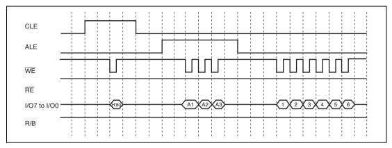
Figure 27.3 Writing Operation Timing for NAND-Type Flash Memory
