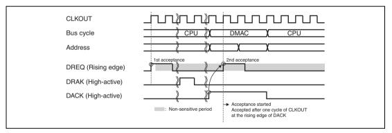
Figure 14.15 Example 3 of DREQ Input Detection in Cycle Steal Mode Edge Detection (Word Transfer in 8-Bit Bus Width, Longword Transfer in 8/16-Bit Bus Width, or 16/32-Byte Transfer in 8/16/32/64-Bit Bus Width: DACK of DMA1 Transfer Is Connected)
