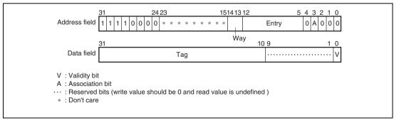
Figure 8.5 Memory-Mapped IC Address Array (Cache size = 32 Kbytes)
