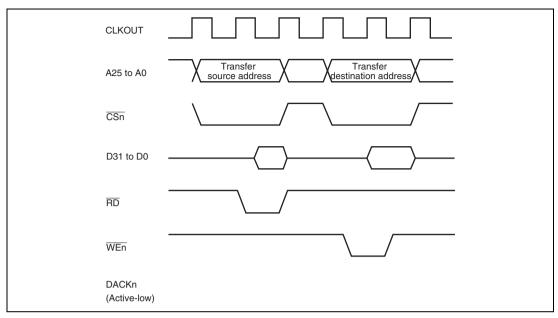
Figure 14.5 Example of DMA Transfer Timing in Dual Address Mode (Source: SRAM, Destination: DDR-SDRAM)
