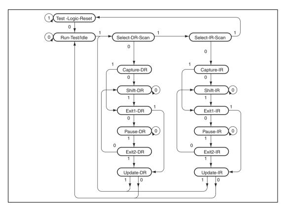
Figure 30.3 Diagram of Transitions of TAP Controller State
