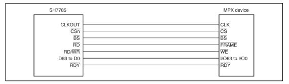
Figure 11.23 Example of 64-Bit Data Width MPX Connection
