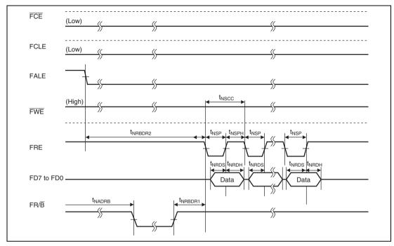
Figure 32.69 Data Read Timing of NAND-Type Flash Memory
