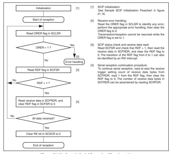
Figure 21.19 Sample Serial Reception Flowchart (1)
