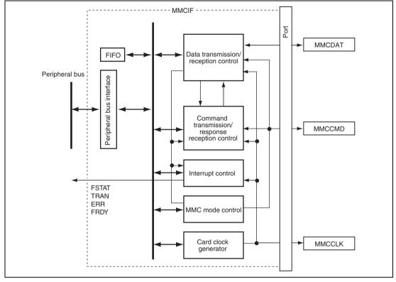
Figure 24.1 Block Diagram of MMCIF
