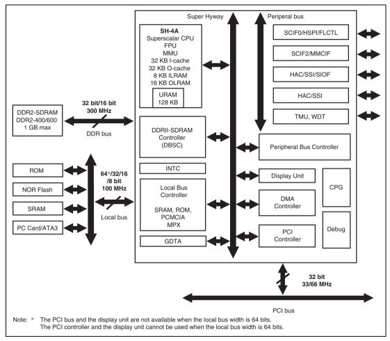
Figure 1.1 SH7785 Block Diagram
