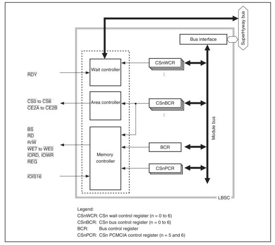
Figure 11.1 Block Diagram of LBSC
