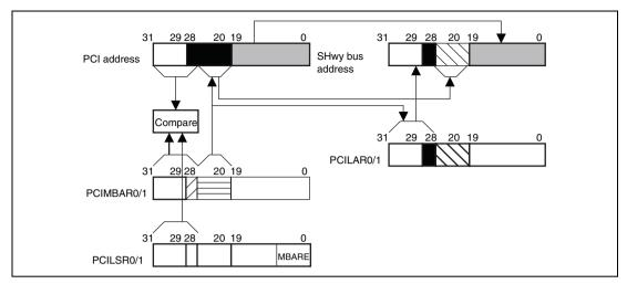
Figure 13.11 PCI Bus to SuperHyway Bus Address Translation
