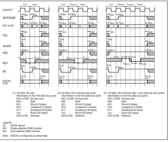
Figure 32.21 MPX Basic Bus Cycle (Write)
