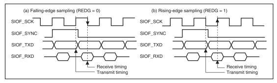
Figure 22.4 SIOF Transmit/Receive Timing
