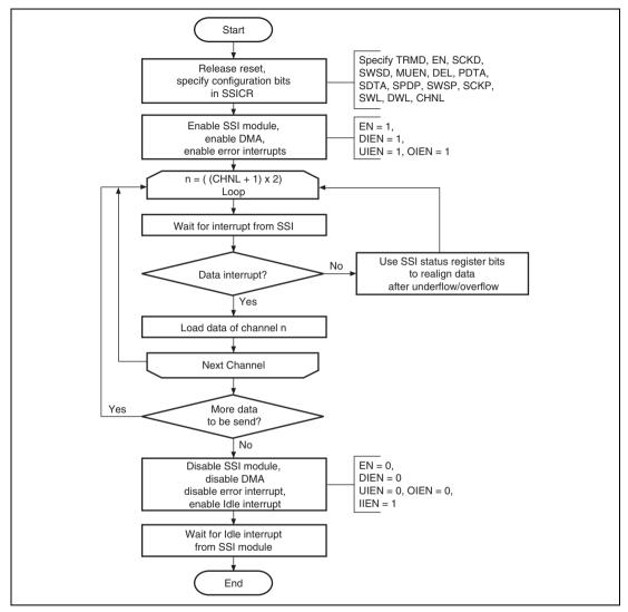
Figure 26.22 Transmission Using Interrupt Data Flow Control
