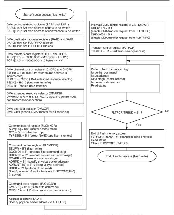
Figure 27.12 NAND Sector Access (Flash Write) Using DMAC
