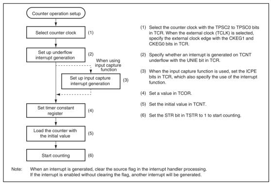
Figure 18.2 Example of Count Operation Setting Procedure
