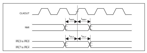
Figure 32.34 Interrupt Signal Input Timing (1)
