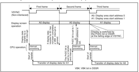
**Auto Display Change Mode:** For information on the auto display change mode, refer to section 19.4.11, Blinking.
