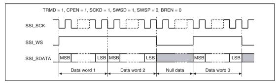
Figure 26.18 Compressed Data Format, Master Transmitter, Burst Mode Disabled
