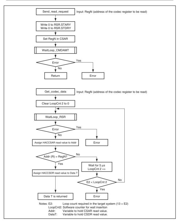
Figure 25.6 Sample Flowchart for Off-Chip Codec Register Read (2)
