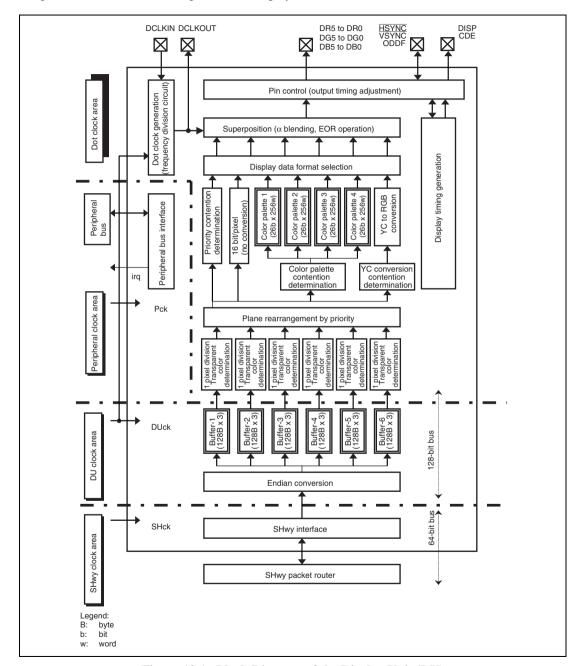
Figure 19.1 Block Diagram of the Display Unit (DU)
