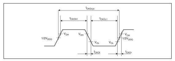
Figure 32.2 CLKOUT Clock Output Timing (1)
