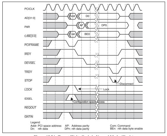
Figure 13.24 Target Write Cycle in Normal Mode (Single)
