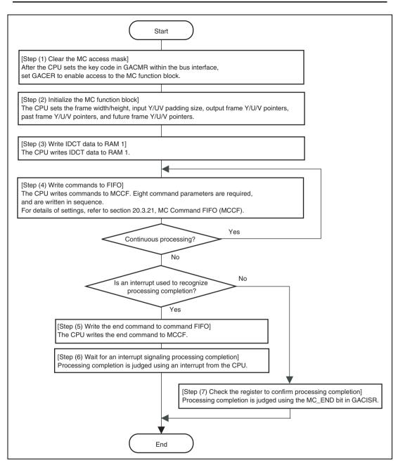
Figure 20.7 MC Processing Procedure
