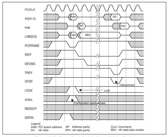
Figure 13.23 Target Read Cycle in Normal Mode (Single)
