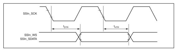
Figure 32.64 SSI Transmission Timing (2)
