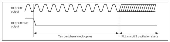
Figure 15.2 Beginning of the Change of the Bus Clock Frequency
