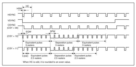
Figure 19.14 CSYNC Timing Chart (Non-Interlaced Mode, First Half of Interlace Frame)
