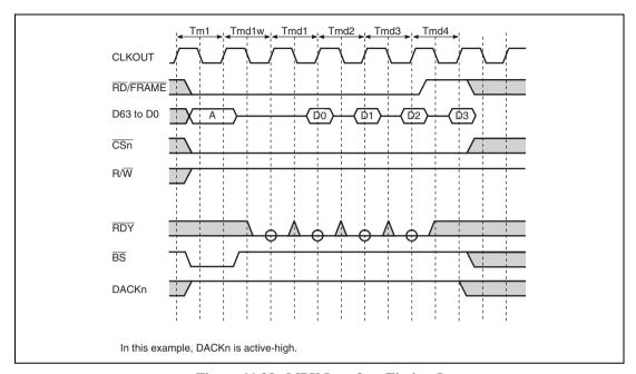
Figure 11.28 MPX Interface Timing 5 (Burst Read Cycle, IW = 0000, No External Wait, 64-Bit Bus Width, 32-Byte Data Transfer)
