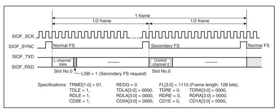
Figure 22.8 Control Data Interface (Secondary FS)
