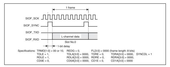
Figure 22.13 Transmit and Receive Timing (8-Bit Monaural Data (1))
