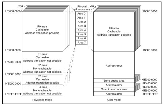
Figure 7.3 Virtual Address Space (AT in MMUCR = 1)
