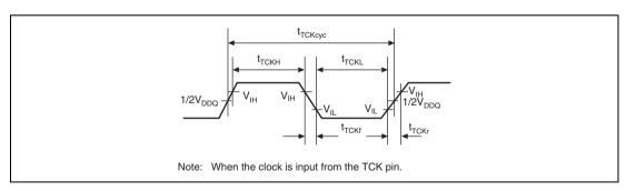
Figure 32.44 TCK Input Timing
