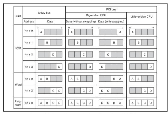
Figure 13.9 Data Alignments for SuperHyway Bus and PCI Bus
