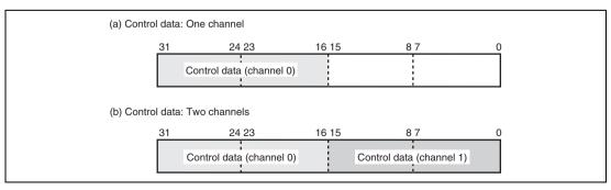
Figure 22.6 Control Data Bit Alignment
