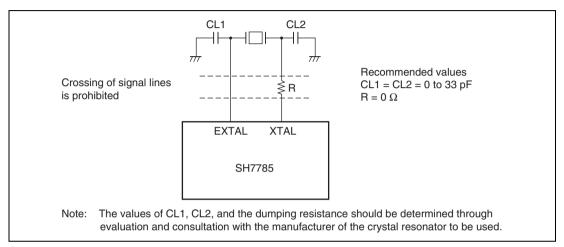
Figure 15.4 Note on Using a Crystal Resonator
