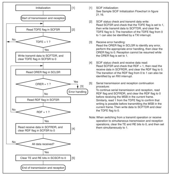
Figure 21.21 Sample Flowchart for Transmitting/Receiving Serial Data
