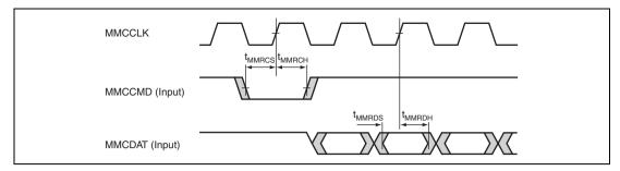
Figure 32.57 MMCIF Reception Timing (Sampling on Rising Edges)
