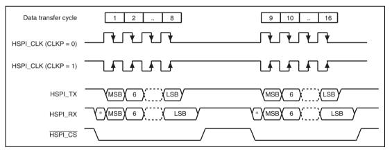
Figure 23.6 Timing Conditions when FBS = 1 (Continuous Transfer)
