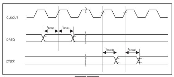
Figure 32.40 DREQ/DRAK Signal Timing
