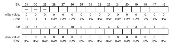
Table 10.10 shows the correspondence between bits in INT2MSKCR and interrupt masking that are cleared.
