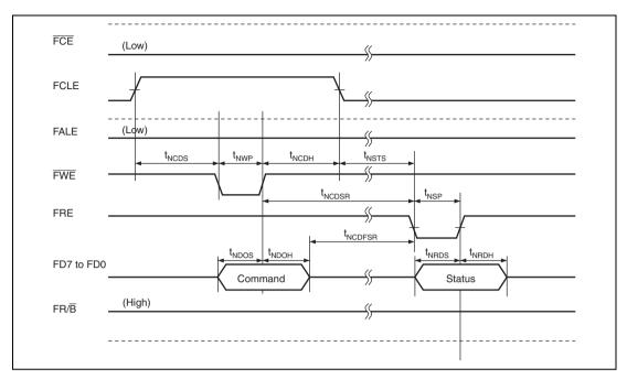
Figure 32.71 Status Read Timing of NAND-Type Flash Memory
