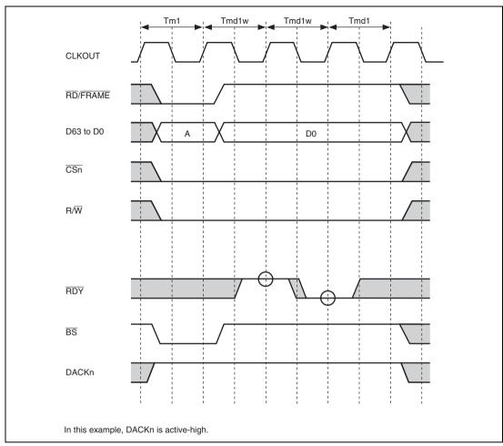
Figure 11.27 MPX Interface Timing 4 (Single Write Cycle, IW = 0001, One External Wait Inserted, 64-Bit Bus Width)
