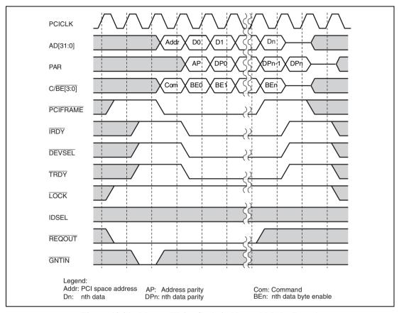
Figure 13.21 Master Write Cycle in Normal Mode (Burst)
