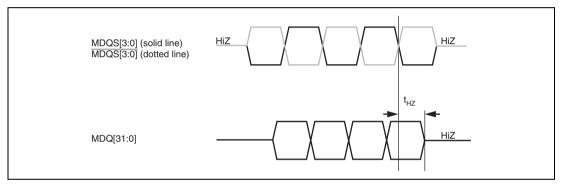
Figure 32.33 MDQ High-Impedance Time from MDQS (Write)
