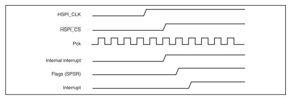
Figure 23.7 Flags and Interrupt Timing
