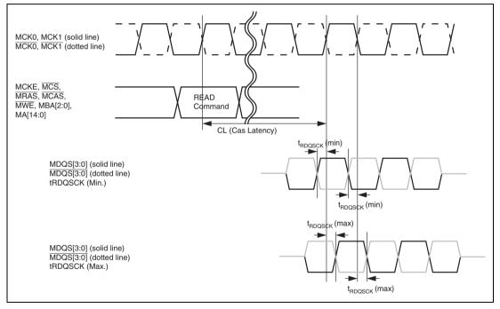
Figure 32.28 MDQS Input Timing at Data Read
