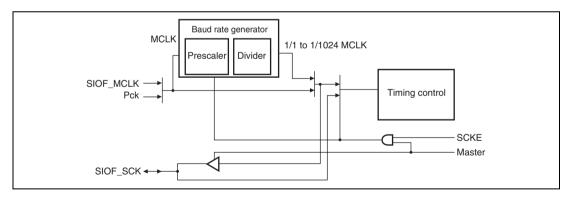
Figure 22.2 Serial Clock Supply
