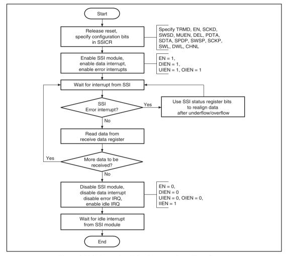
Figure 26.24 Reception Using Interrupt Data Flow Control
