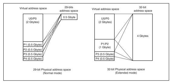
Figure 7.26 Physical Address Space (32-Bit Address Extended Mode)
