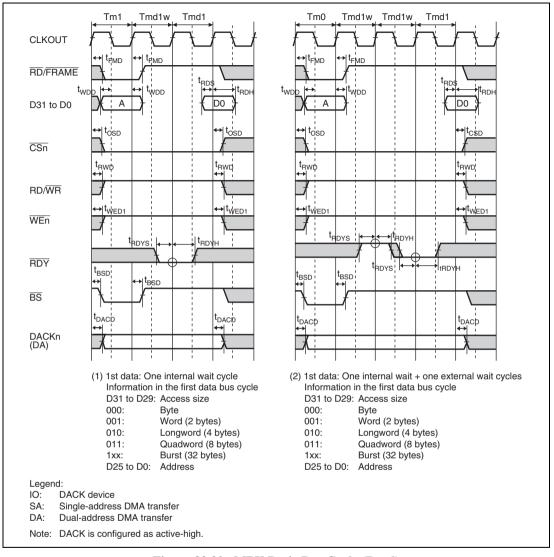
Figure 32.20 MPX Basic Bus Cycle (Read)
