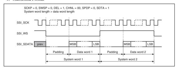
Figure 26.5 Matsushita Format (with Padding Bits First, Followed by Serial Data)
