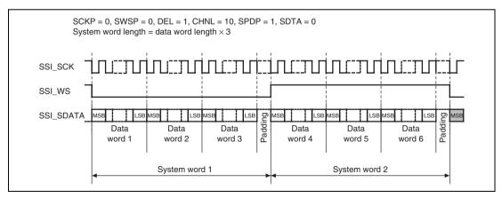
Figure 26.7 Multi-channel Format (6 Channels with High Padding)
