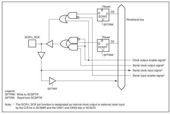
Figure 21.4 SCIFn\_SCK Pin (n = 0 to 5)
