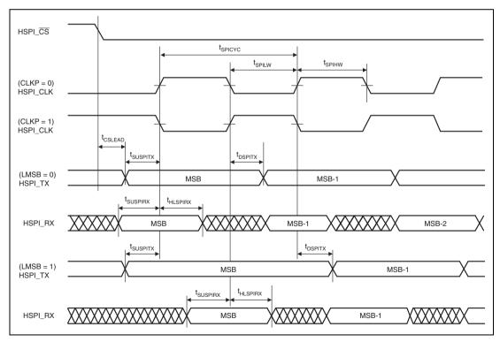
Figure 32.49 HSPI Data Output/Input Timing
