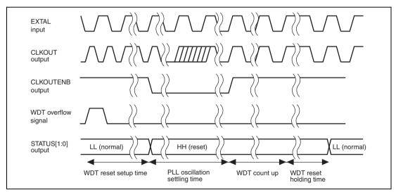
Figure 16.6 STATUS Output by Power-On Reset Caused by WDT Overflow during Normal Operation
