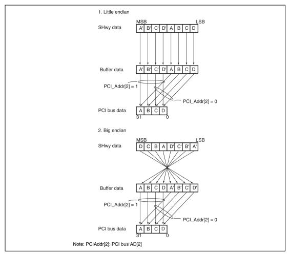
Figure 13.8 Endian Conversion from SuperHyway Bus to PCI Local Bus (Byte Swapping: TBS = 1)
