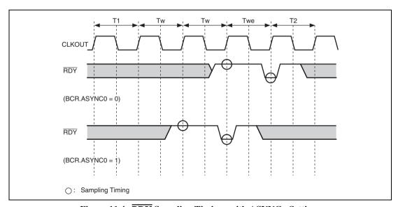
Figure 11.4 RDY Sampling Timings with ASYNCn Settings (Two Wait Cycles Inserted by CSnWCR.)
