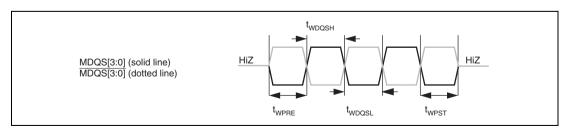
Figure 32.31 MDQS Output Waveform (Write)
