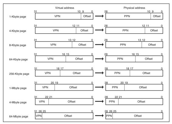
Figure 7.12 Relationship between Page Size and Address Format (TLB Extended Mode)
