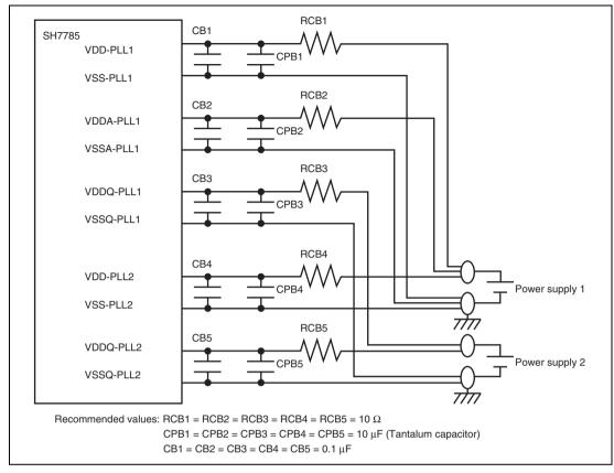
Figure 15.5 Note on Using a PLL Oscillator Circuit
