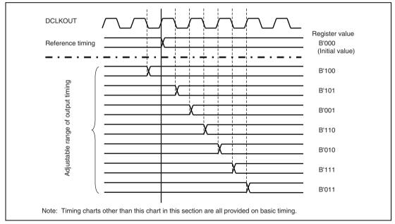
Figure 19.19 Adjustable Range of Output Timing
