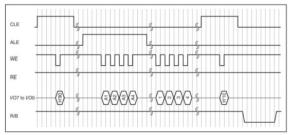
Figure 27.6 Writing Operation Timing for NAND-Type Flash Memory
