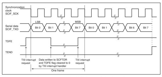
Figure 21.18 Example of SCIF Transmission Operation
