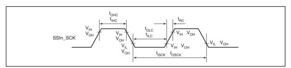
Figure 32.62 SSI Clock Input/Output Timing
