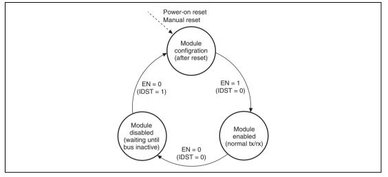
Figure 26.20 Transition Diagram between Operation Modes
