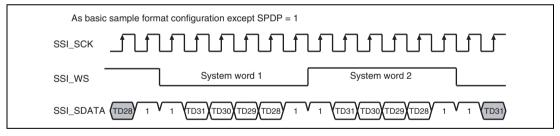
Figure 26.12 Inverted Padding Polarity
