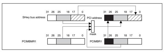
Figure 13.4 Access from SuperHyway Bus to PCI Memory (PCI Bus) (PCI Memory Space 1)
