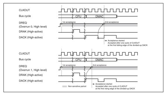
Figure 14.21 Example 2 of DREQ Input Detection in Burst Mode Level Detection (Word Transfer in 8-Bit Bus Width, Longword Transfer in 8/16-Bit Bus Width, 16/32-Byte Transfer in 8/16/32/64-Bit Bus Width: DACK of DMA1 Transfer Divided)
