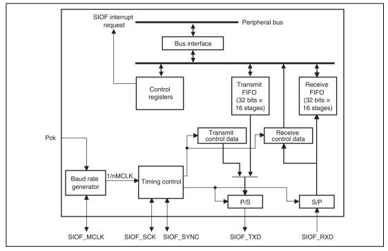
Figure 22.1 Block Diagram of SIOF
