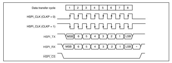
Figure 23.3 Timing Conditions when FBS = 0
