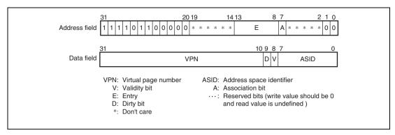
Figure 7.22 Memory-Mapped UTLB Address Array
