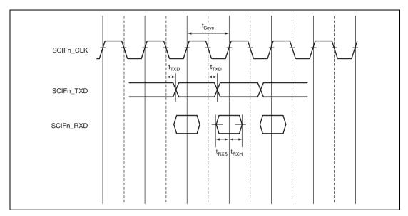
Figure 32.43 Clock Timing in SCIF I/O Synchronous Mode
