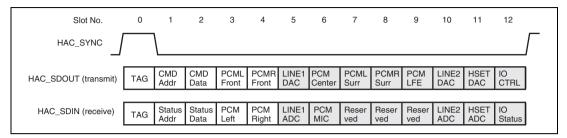
Figure 25.2 AC97 Frame Slot Structure
