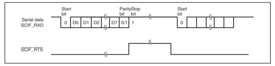
Figure 21.14 Example of Operation Using Modem Control (SCIF\_RTS)
