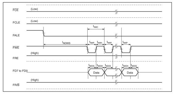
Figure 32.70 Data Write Timing of NAND-Type Flash Memory
