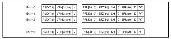
Figure 7.11 UTLB Configuration (TLB Extended Mode)
