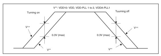
Figure D.3 Sequence of Turning On and Off VDD10 Power Supply Series
