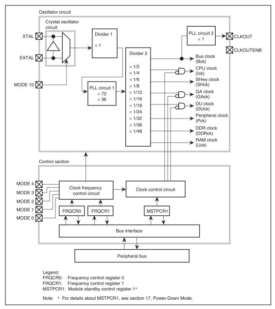
Figure 15.1 Block Diagram of the CPG
