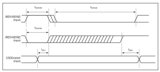
Figure 32.75 Display Timing in TV Synchronous Mode
