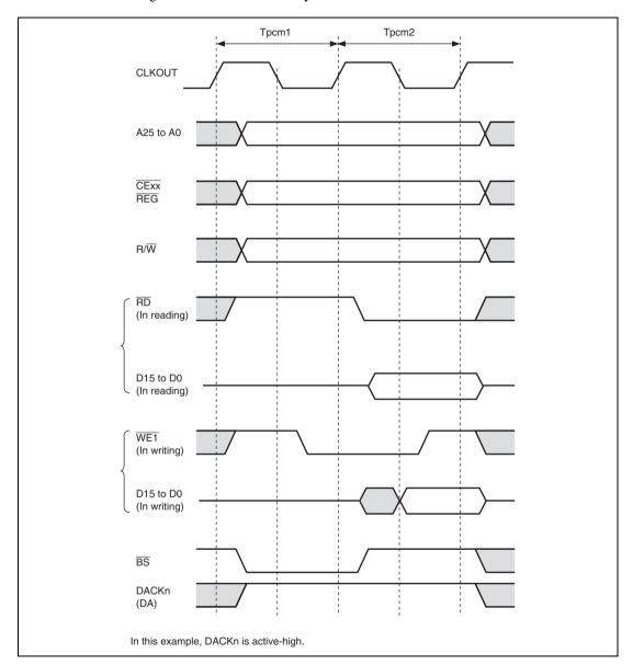
Figure 11.17 Basic Timing for PCMCIA Memory Card Interface
