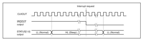
Figure 17.1 Status Pins Output when an Interrupt Occurs in Sleep Mode
