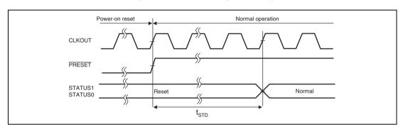
Figure 32.8 STATUS Pin Output Timing at Power-On Reset
