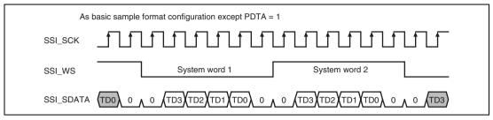
Figure 26.16 Parallel Right Aligned with Delay
