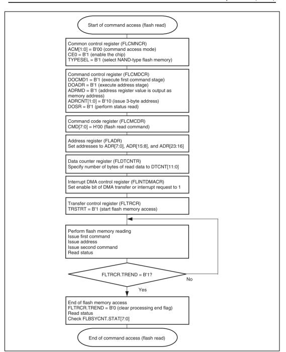
Figure 27.13 NAND Command Access (Flash Read)
