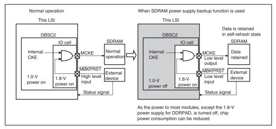
Figure 12.23 SDRAM Power Supply Backup Function
