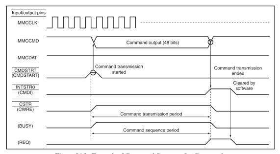
Figure 24.3 Example of Command Sequence for Commands
