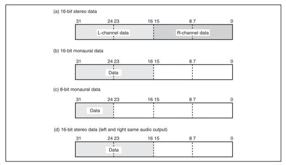
Figure 22.5 Transmit/Receive Data Bit Alignment
