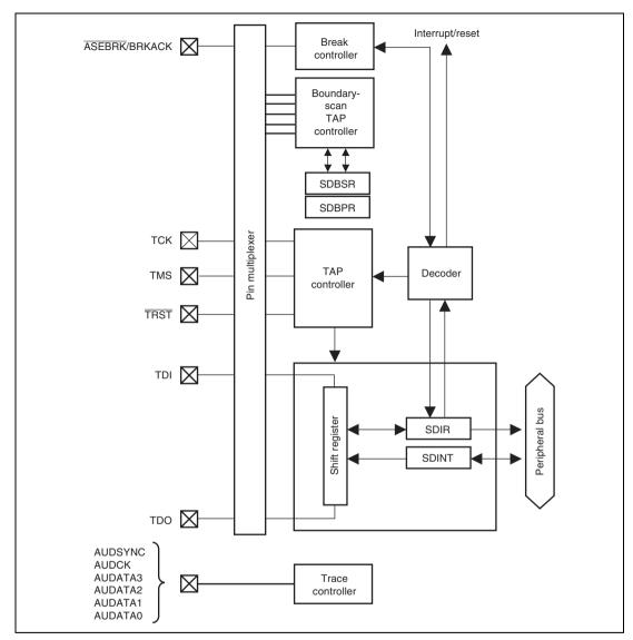
Figure 30.1 Block Diagram of H-UDI
