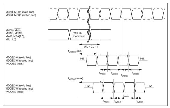
Figure 32.30 MDQS Output Waveform to MCK (Write)
