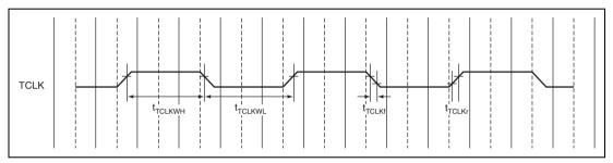
Figure 32.41 TCLK Input Timing
