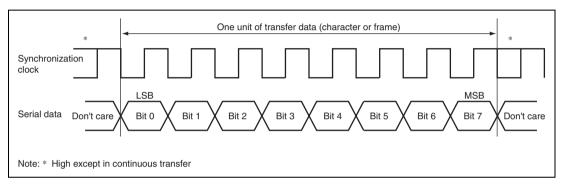
Figure 21.15 Data Format in Clocked Synchronous Communication
