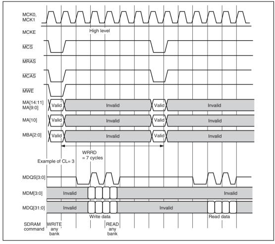
Figure 12.19 WRITE-READ Minimum Time
