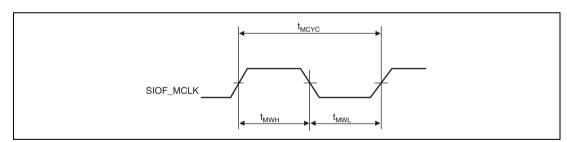
Figure 32.50 SIOF\_MCLK Input Timing
