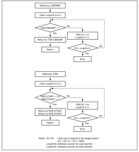
Figure 25.7 Sample Flowchart for Off-Chip Codec Register Read (3)
