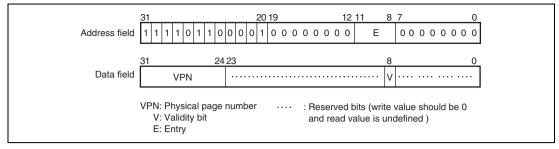
Figure 7.28 Memory-Mapped PMB Address Array
