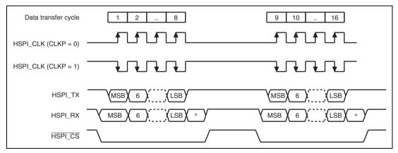
Figure 23.4 Timing Conditions when FBS = 0 (Continuous Transfer)
