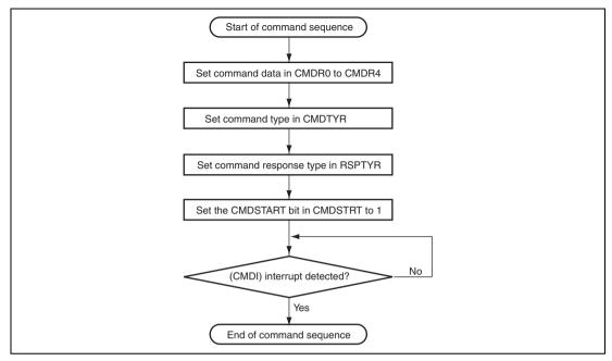
Figure 24.4 Example of Operational Flow for Commands
