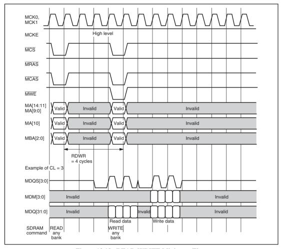
Figure 12.18 READ-WRITE Minimum Time
