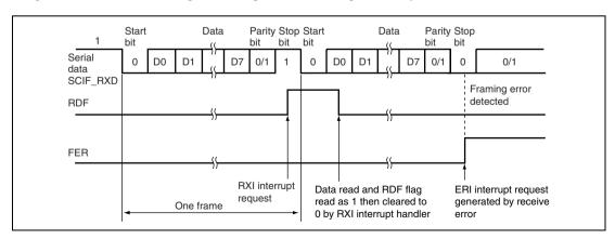
Figure 21.13 Example of SCIF Receive Operation (Example with 8-Bit Data, Parity, One Stop Bit)
