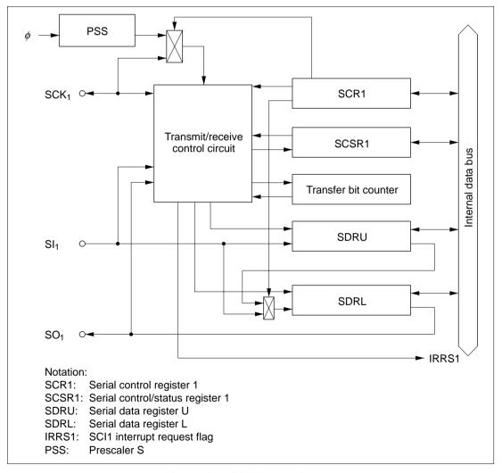
Figure 10.1 SCI1 Block Diagram
