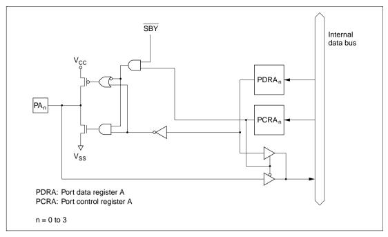
Figure C.10 Port A Block Diagram
