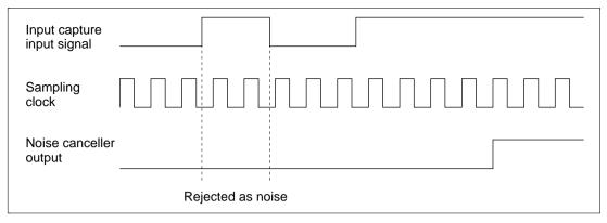
Figure 9.10 Noise Canceller Circuit Timing (Example)
