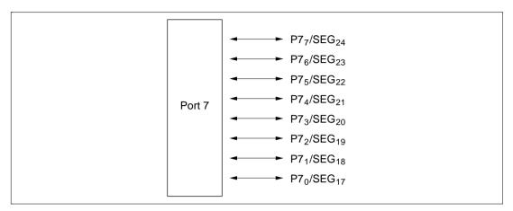
Figure 8.7 Port 7 Pin Configuration
