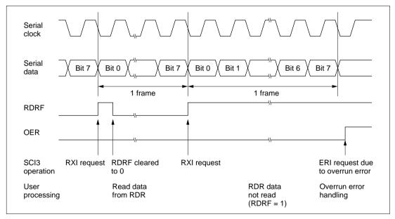
Figure 10.20 Typical Receive Operation in Synchronous Mode
