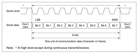
Figure 10.16 Data Format in Synchronous Communication Mode
