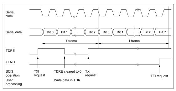
Figure 10.18 Typical SCI3 Transmit Operation in Synchronous Mode
