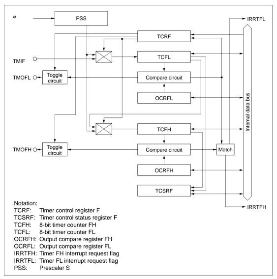
Figure 9.4 Block Diagram of Timer F
