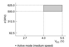
3. Analog power supply voltage vs. A/D converter operating range of H8/3835, H8/3836 and H8/3837
