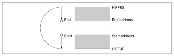
Figure 10.6 Operation When End Address is Smaller than Start Address
