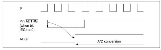
Figure 12.2 External Trigger Input Timing
