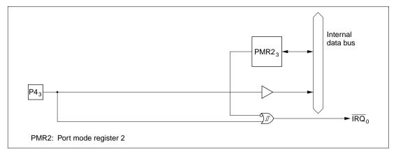
Figure C.4 (a) Port 4 Block Diagram (Pin P4<sub>3</sub>)
