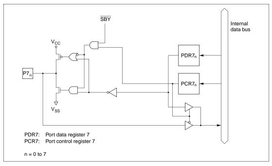
Figure C.7 Port 7 Block Diagram
