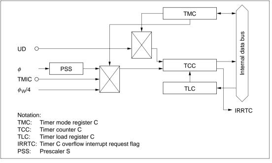
Figure 9.3 Block Diagram of Timer C
