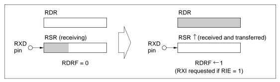
Figure 10.8 (a) RDRF Setting and RXI Interrupt
