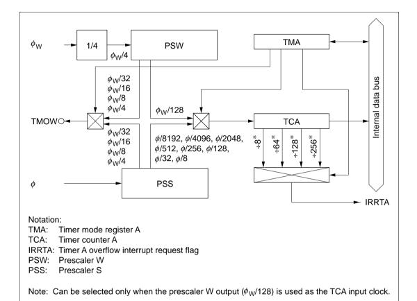
Figure 9.1 Block Diagram of Timer A
