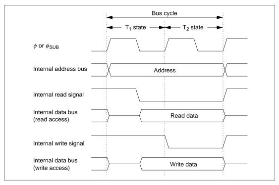
Figure 2.11 On-Chip Memory Access Cycle
