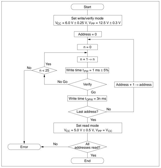
Figure 6.4 High-Performance Programming Flowchart
