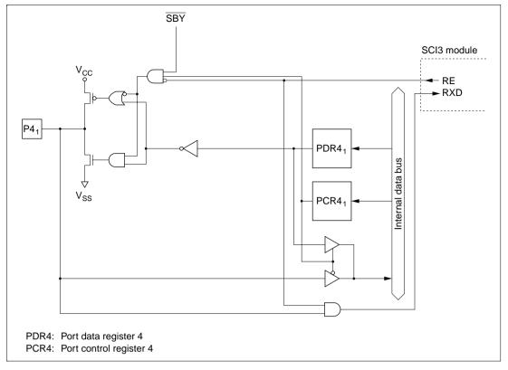
Figure C.4 (c) Port 4 Block Diagram (Pin P4<sub>1</sub>)
