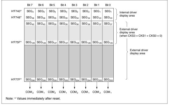
Figure 13.9 LCD RAM Map: External Segment Expansion (1/2 Duty)
