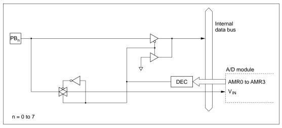
Figure C.11 Port B Block Diagram
