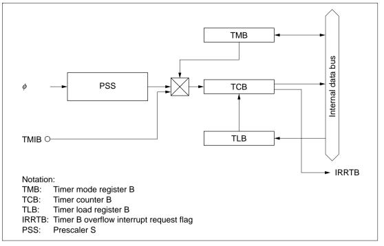
Figure 9.2 Block Diagram of Timer B
