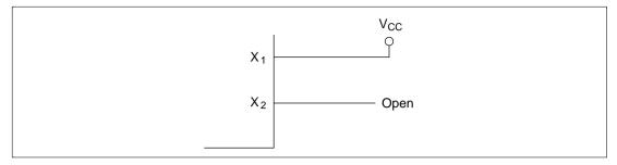
Figure 4.9 Pin Connection when Not Using Subclock
