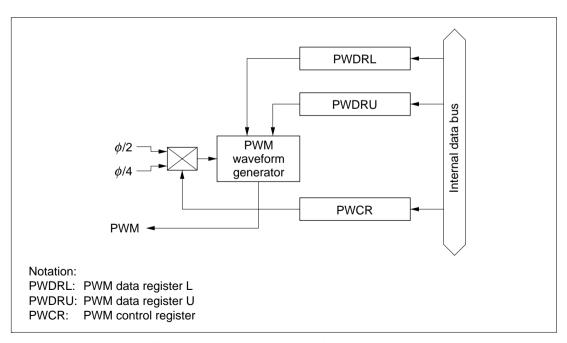
Figure 11.1 Block Diagram of the 14 bit PWM
