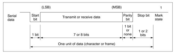
Figure 10.9 Data Format in Asynchronous Serial Communication Mode
