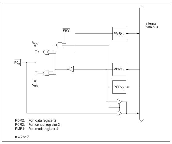
Figure C.2 (a) Port 2 Block Diagram (Pins P2, to P2,)
