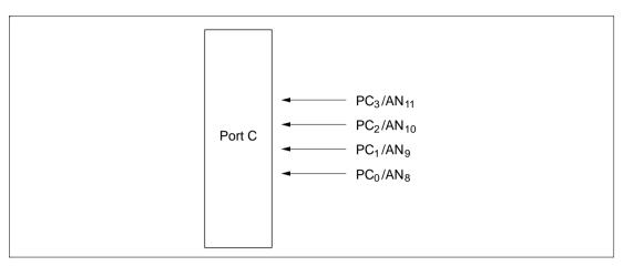
Figure 8.12 Port C Pin Configuration
