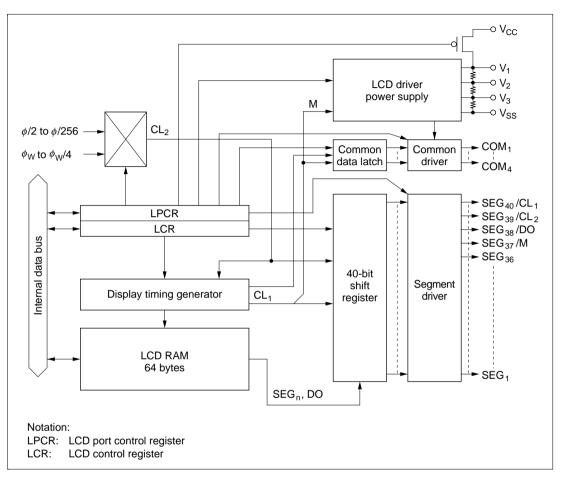
Figure 13.1 LCD Controller/Driver Block Diagram
