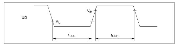
Figure 14.4 UD Pin Minimum Transition Width Timing
