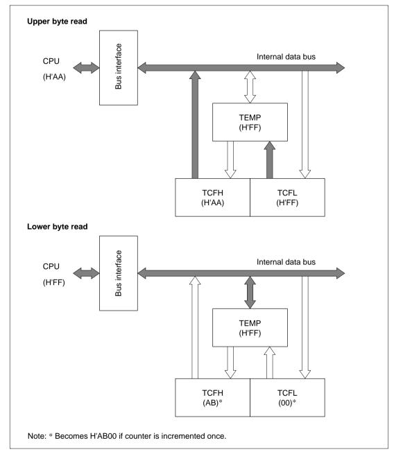
Figure 9.6 TCF Read Operation (TCF  $\rightarrow$  CPU)
