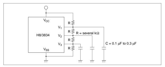
Figure 13.14 Connecting an External Resistive Voltage Divider
