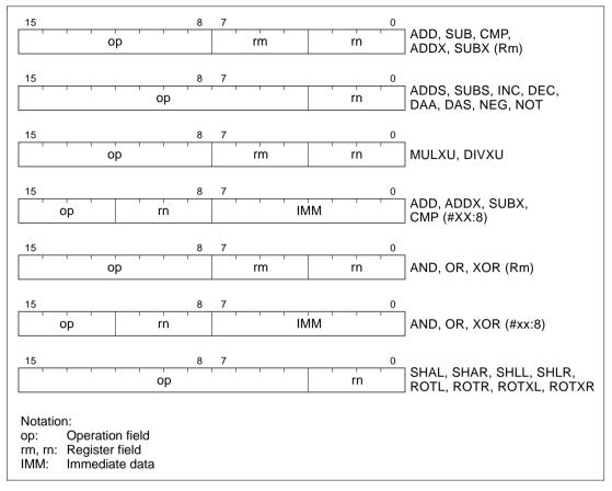
Figure 2.6 Arithmetic, Logic, and Shift Instruction Codes
