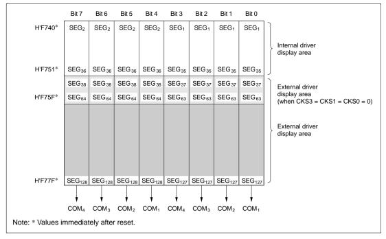
Figure 13.7 LCD RAM Map: External Segment Expansion (1/4 Duty)
