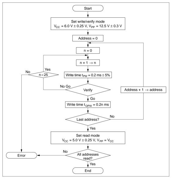
Figure 6.8 High-Speed, High-Reliability Programming Flow Chart
