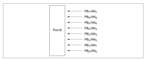
Figure 8.11 Port B Pin Configuration
