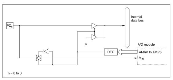
Figure C-12 Port C Block Diagram
