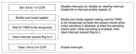
Figure 9.15 Procedure for Modifying Port Mode Register and Clearing Interrupt Request Flag
