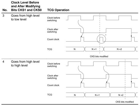
Note: \* The switchover is seen as a falling edge of the clock pulse, and TCG is incremented.
