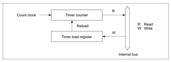
Figure 2.23 Timer Configuration Example
