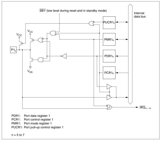
Figure C.1 (a) Port 1 Block Diagram (Pins P1, to P1,
