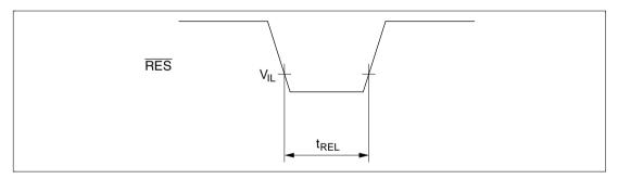
Figure 14.2 RES Low Width Timing
