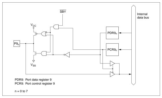
Figure C.9 Port 9 Block Diagram
