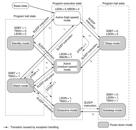
A transition between different modes cannot be made to occur simply because an interrupt request is generated. Make sure that the interrupt is accepted and interrupt handling is performed. Details on the mode transition conditions are given in the explanations of each mode, in sections 5.2 through 5.8.
