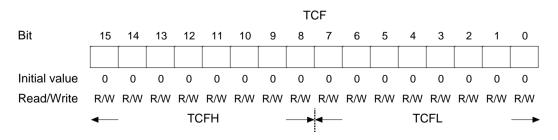
TCF is a 16-bit read/write up-counter consisting of two cascaded 8-bit timer counters, TCFH and TCFL. TCF can be used as a 16-bit counter, with TCFH as the upper 8 bits and TCFL as the lower 8 bits of the counter, or TCFH and TCFL can be used as independent 8-bit counters.
