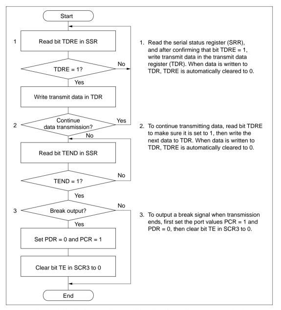
Figure 10.12 Typical Data Transmission Flow Chart (Asynchronous Mode)
