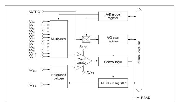
Figure 12.1 Block Diagram of the A/D Converter
