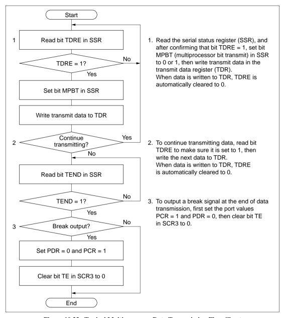
Figure 10.23 Typical Multiprocessor Data Transmission Flow Chart
