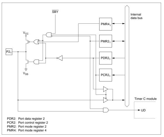
Figure C.2 (b) Port 2 Block Diagram (Pin P2<sub>1</sub>)
