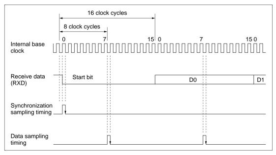
Figure 10.27 Receive Data Sampling Timing in Asynchronous Mode
