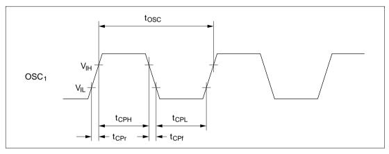
Figure 14.1 System Clock Input Timing
