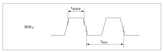
Figure 14.7 SCK<sub>3</sub> Input Clock Timing
