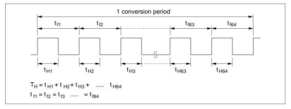
Figure 11.2 PWM Output Waveform
