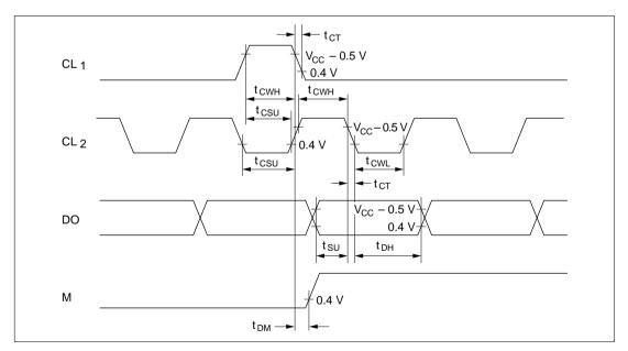
Figure 14.9 Segment Expansion Signal Timing
