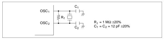
Figure 4.2 Typical Connection to Crystal Oscillator
