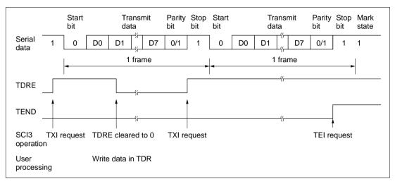
Figure 10.13 Typical Transmit Operation in Asynchronous Mode (8-Bit Data, Parity Bit Added, and 1 Stop Bit)
