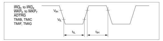
Figure 14.3 Input Timing
