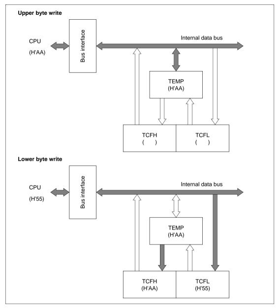
Figure 9.5 TCF Write Operation (CPU  $\rightarrow$  TCF)
