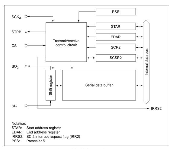
Figure 10.3 SCI2 Block Diagram
