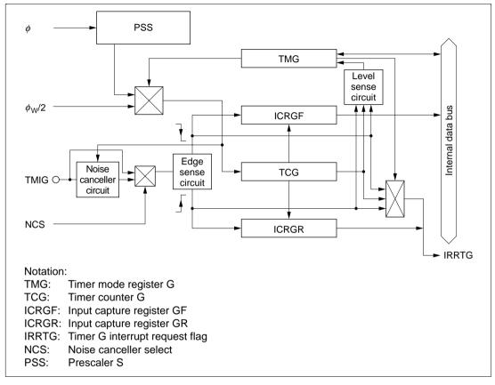
Figure 9.8 Block Diagram of Timer G
