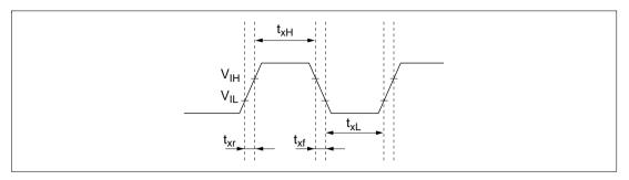
Figure 4.10 External Subclock Timing
