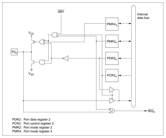
Figure C.2 (c) Port 2 Block Diagram (Pin P2<sub>0</sub>)
