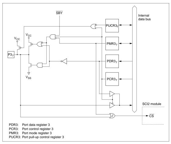
Figure C.3 (a) Port 3 Block Diagram (Pin P3<sub>7</sub>)
