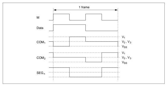
Figure 13.13 (c) Waveforms at 1/2 Duty
