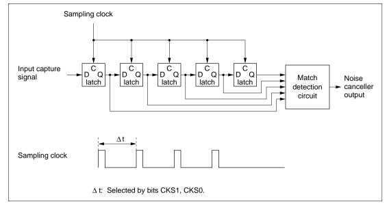
Figure 9.9 Block Diagram of Noise Canceller Circuit
