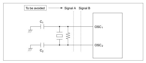
Figure 4.5 Board Design of Oscillator Circuit
