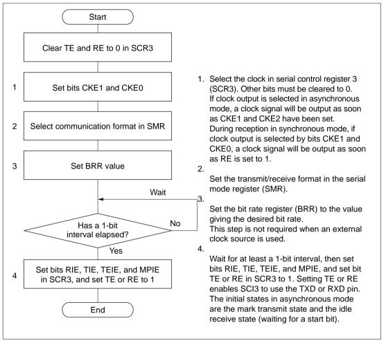
Figure 10.11 Typical Flow Chart when SCI3 Is Initialized
