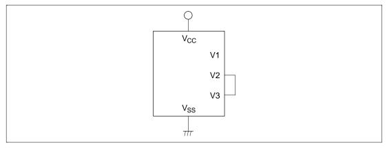
Figure 13.2 LCD Driver Power Supply Processing at 1/2 Duty
