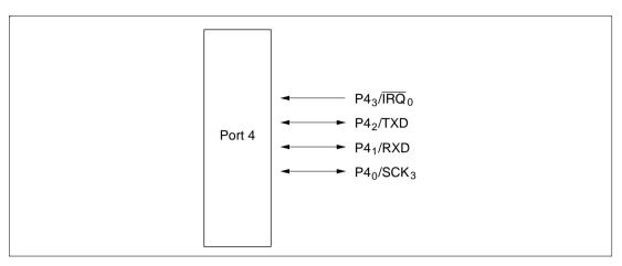
Figure 8.4 Port 4 Pin Configuration
