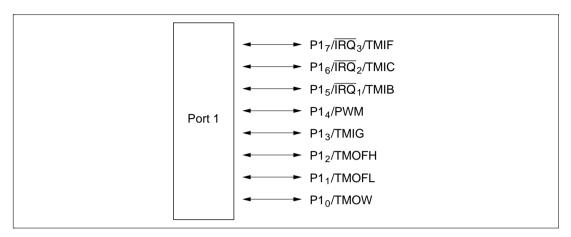
Figure 8.1 Port 1 Pin Configuration
