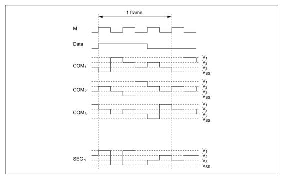
Figure 13.13 (b) Waveforms at 1/3 Duty
