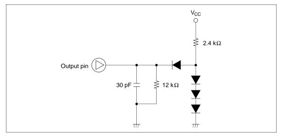
Figure 14.10 Output Load Condition
