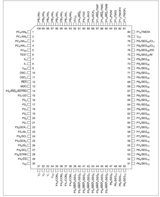
Figure 1.3 Pin Arrangement (FP-100A: Top View)
