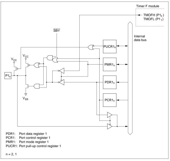
Figure C.1 (d) Port 1 Block Diagram (Pins P1<sub>2</sub> and P1<sub>1</sub>)
