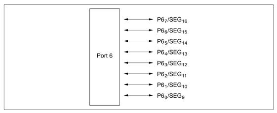
Figure 8.6 Port 6 Pin Configuration
