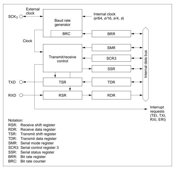
Figure 10.7 SCI3 Block Diagram
