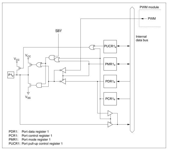
Figure C.1 (b) Port 1 Block Diagram (Pin P1<sub>4</sub>)
