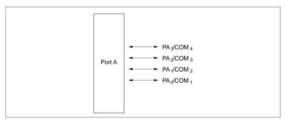
Figure 8.10 Port A Pin Configuration
