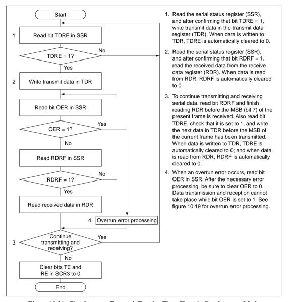
Figure 10.21 Simultaneous Transmit/Receive Flow Chart in Synchronous Mode
