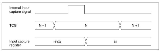
Figure 9.13 Input Capture Timing
