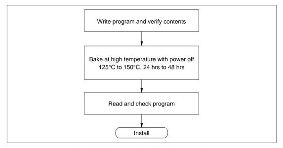
Figure 6.10 Recommended Screening Procedure
