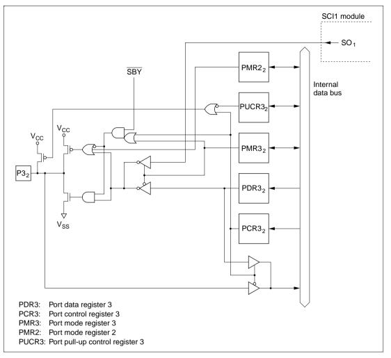
Figure C.3 (f) Port 3 Block Diagram (Pin P3<sub>2</sub>)
