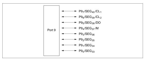
Figure 8.9 Port 9 Pin Configuration
