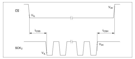
Figure 14.6 Serial Interface 2 Chip Select Timing
