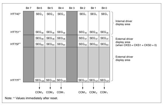
Figure 13.8 LCD RAM Map: External Segment Expansion (1/3 Duty)
