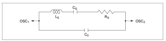
Figure 4.3 Equivalent Circuit of Crystal Oscillator
