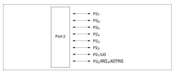
Figure 8.2 Port 2 Pin Configuration
