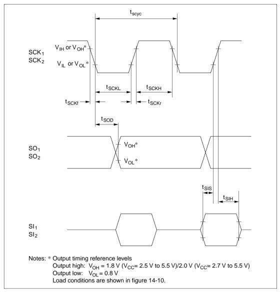
Figure 14.5 Serial Interface 1 and 2 Input/Output Timing
