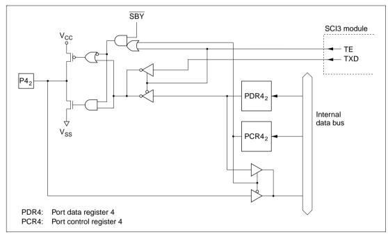
Figure C.4 (b) Port 4 Block Diagram (Pin P4<sub>2</sub>)
