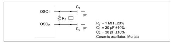
Figure 4.4 Typical Connection to Ceramic Oscillator
