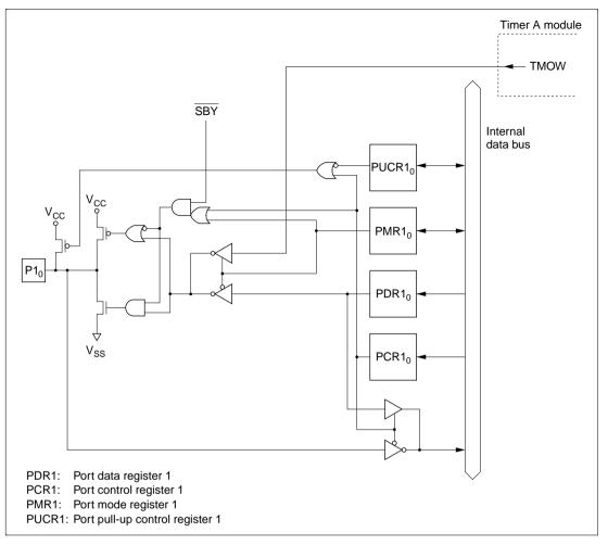
Figure C.1 (e) Port 1 Block Diagram (Pin  $P1_0$ )
