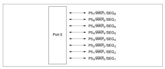
Figure 8.5 Port 5 Pin Configuration
