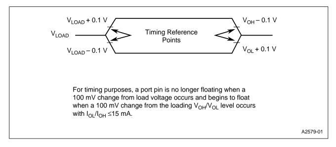
Figure 14. Float Waveforms
