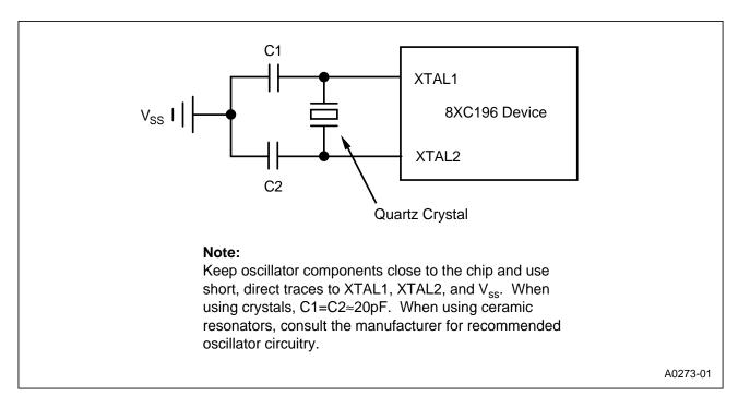
Figure 12. External Crystal Connections
