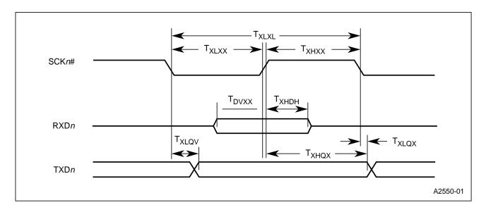
Figure 16. Serial Port Waveform — Mode 4
