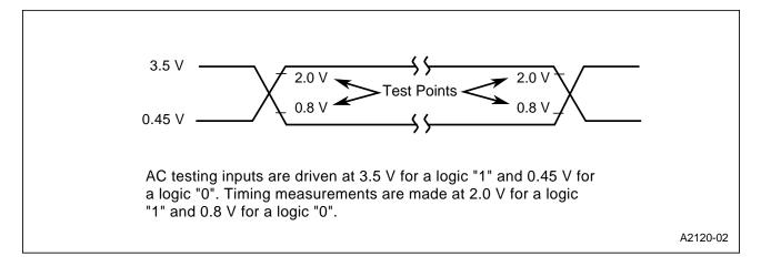
Figure 13. AC Testing Input, Output Waveforms
