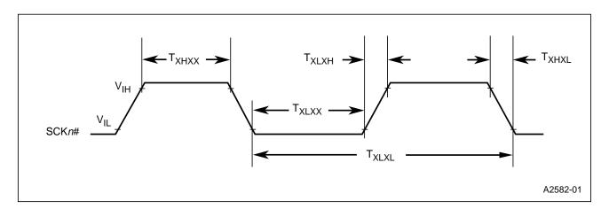
Figure 17. Serial Port Waveform — Clock Drive (DIR = 1)
