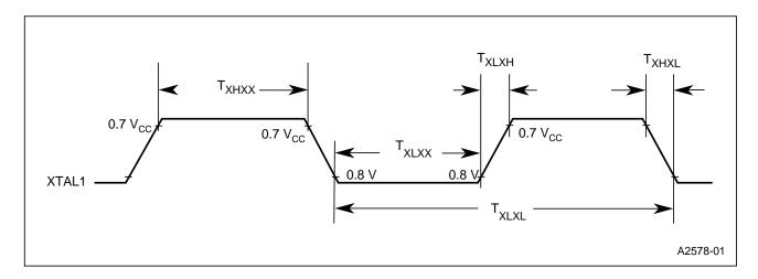
Figure 10. External Clock Drive Waveforms
