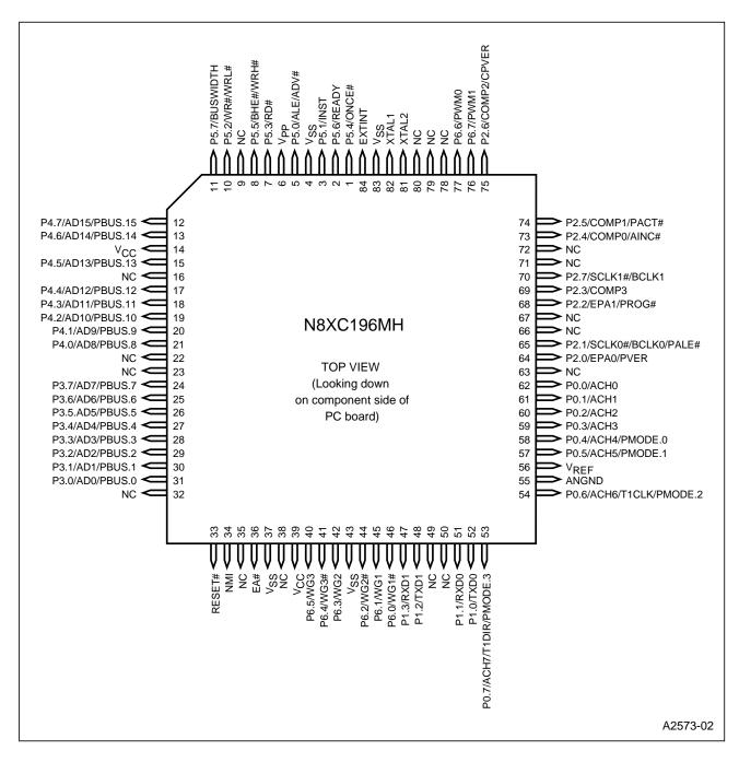
Figure 4. 8XC196MH 84-lead PLCC Package
