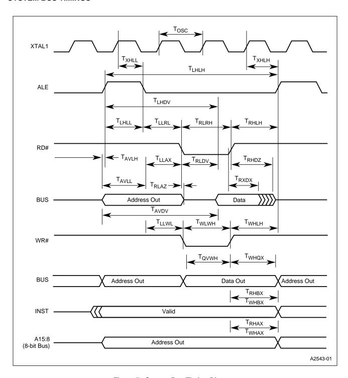
Figure 7. System Bus Timing Diagram
