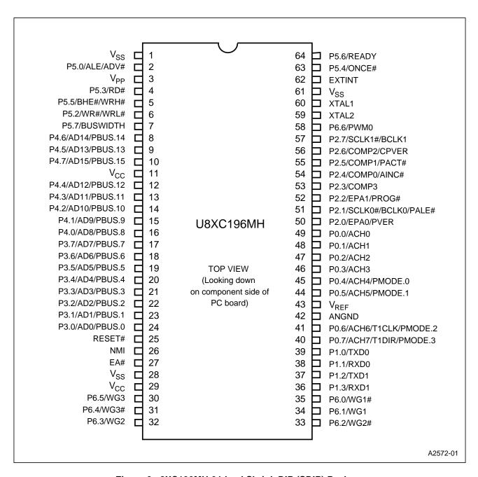
Figure 3. 8XC196MH 64-lead Shrink DIP (SDIP) Package
