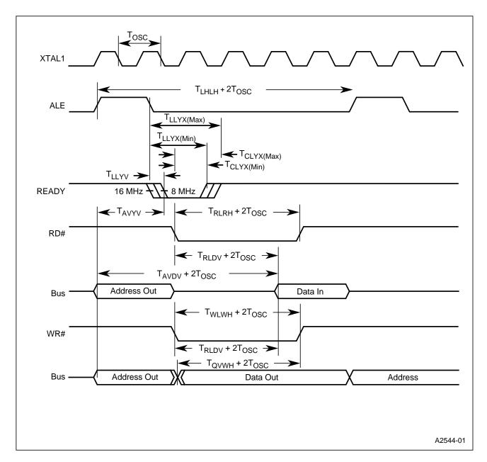
Figure 8. READY Timing Diagram (One Wait State)
