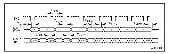
Figure 15. Serial Port Waveform — Shift Register Mode (Mode 0)
