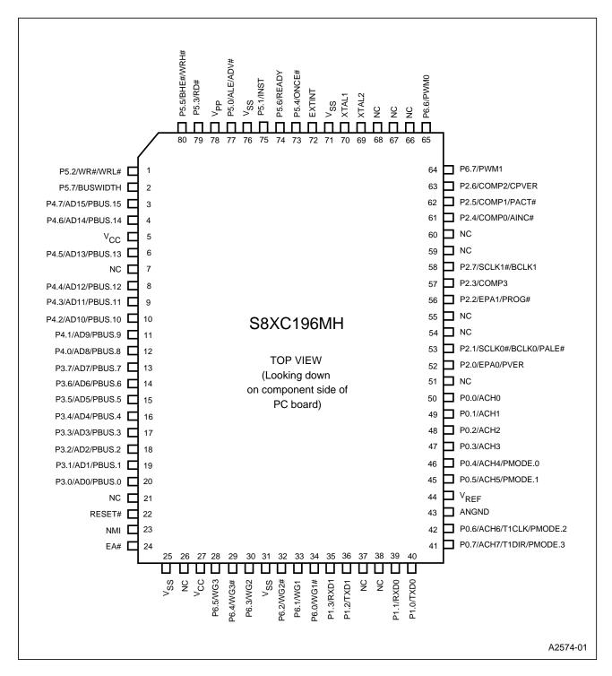
Figure 5. 8XC196MH 80-lead Shrink EIAJ/QFP Package
