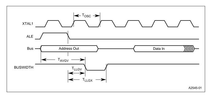
Figure 9. BUSWIDTH Timing Diagram
