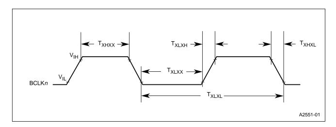
Figure 18. Baud-Rate Clock Drive Waveforms
