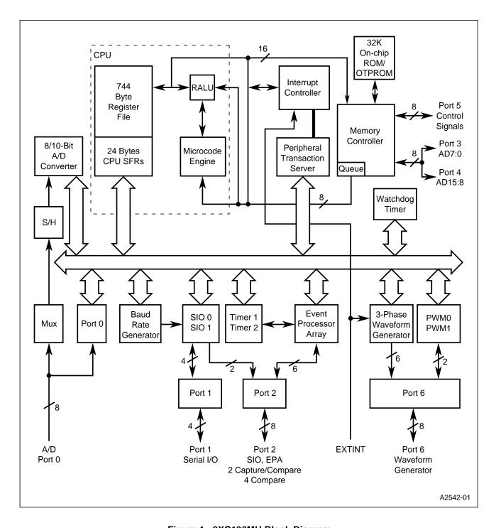
Figure 1. 8XC196MH Block Diagram
