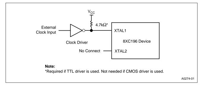
Figure 11. External Clock Connections
