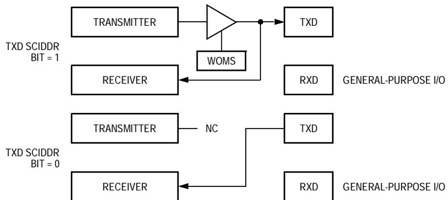
Figure 16-25. Single-Wire Operation (LOOPS = 1, RSRC = 1)
