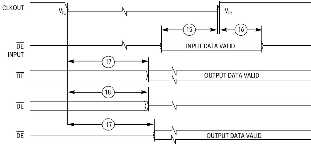
Figure 22-13. Debug Event Pin Timing
