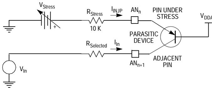
Figure 18-52. Input Pin Subjected to Positive Stress
