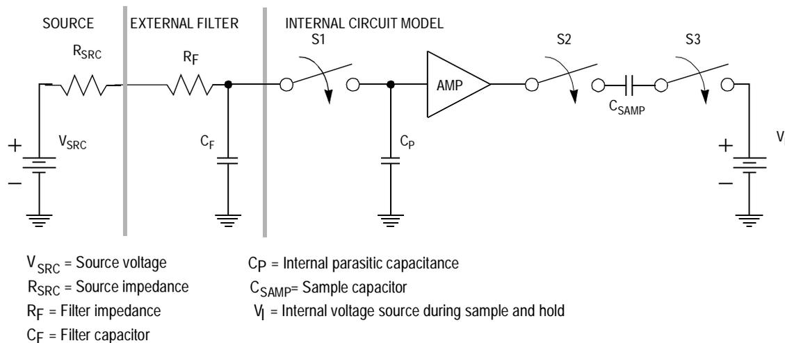
**Figure 18-54. Electrical Model of an A/D Input Pin**
