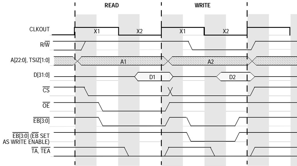
Figure 19-3. Master Mode — 1-Clock Read and Write Cycle
