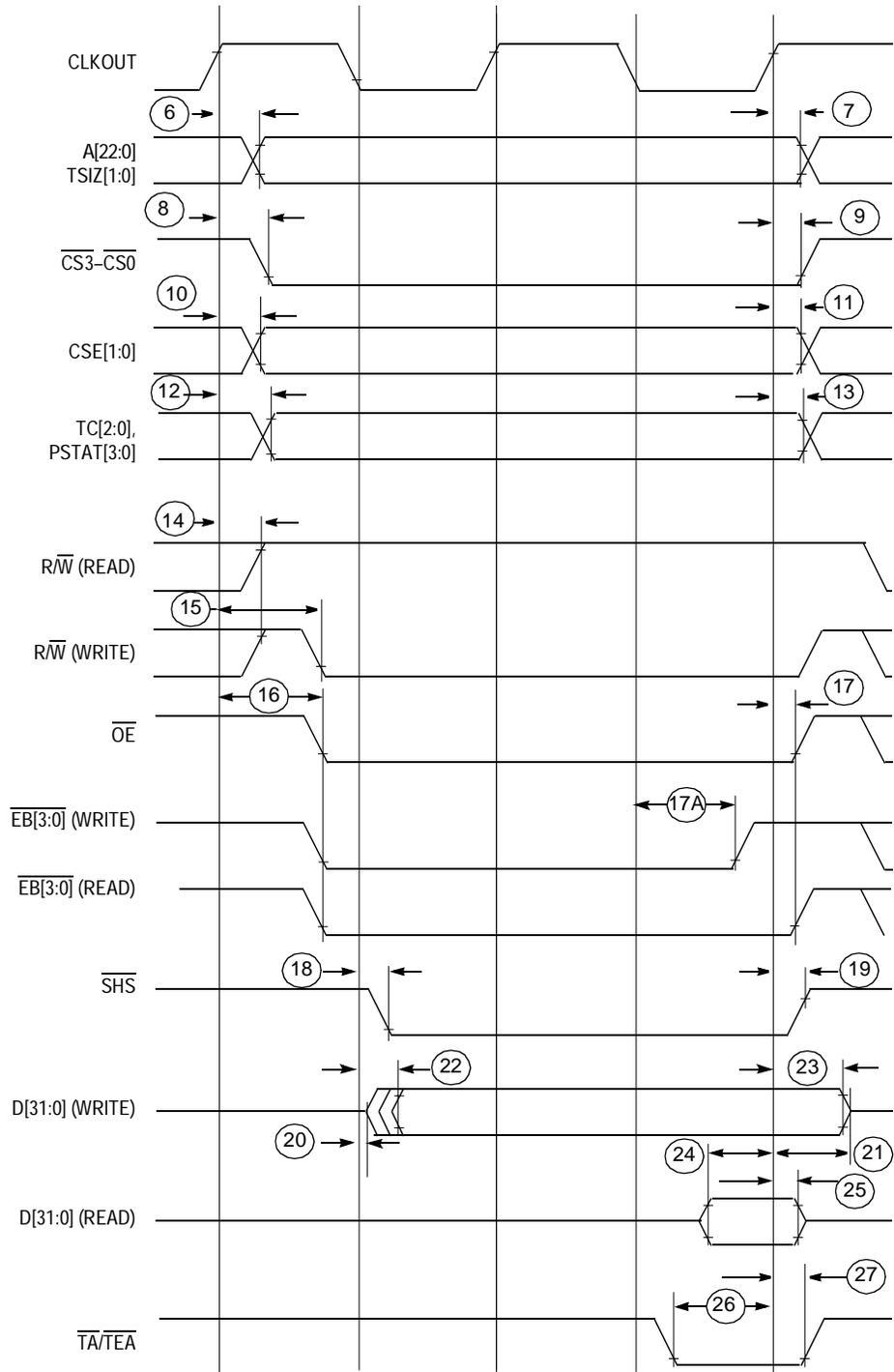
Figure 22-5. Read/Write Cycle Timing with Wait States
