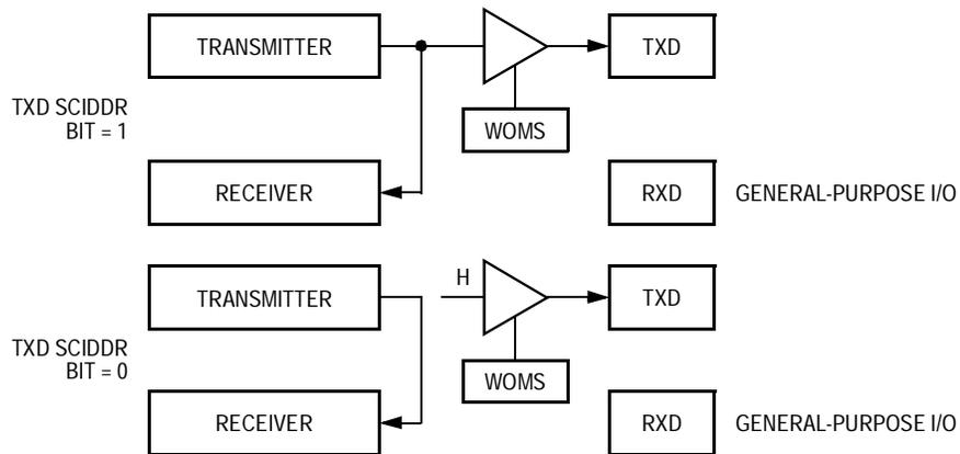
**Figure 16-26. Loop Operation (LOOPS = 1, RSRC = 0)**
