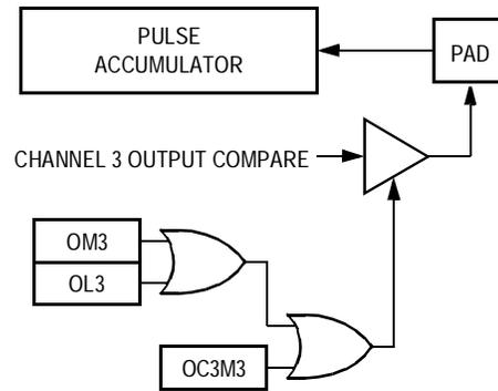
Figure 15-26. Channel 3 Output Compare/Pulse Accumulator Logic
