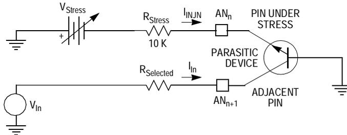
Figure 18-51. Input Pin Subjected to Negative Stress
