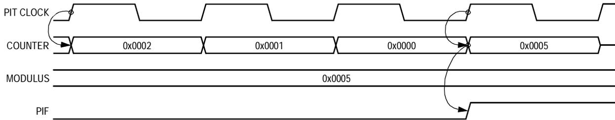
Figure 14-5. Counter Reloading from the Modulus Latch
