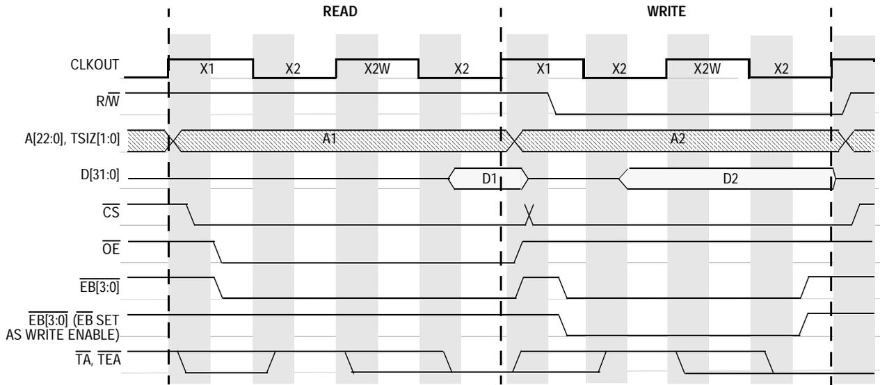
Figure 19-4. Master Mode — 2-Clock Read and Write Cycle
