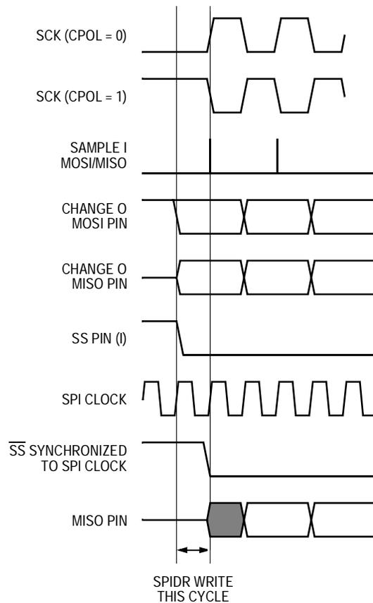
Figure 17-13. Transmission Error Due to Master/Slave Clock Skew
