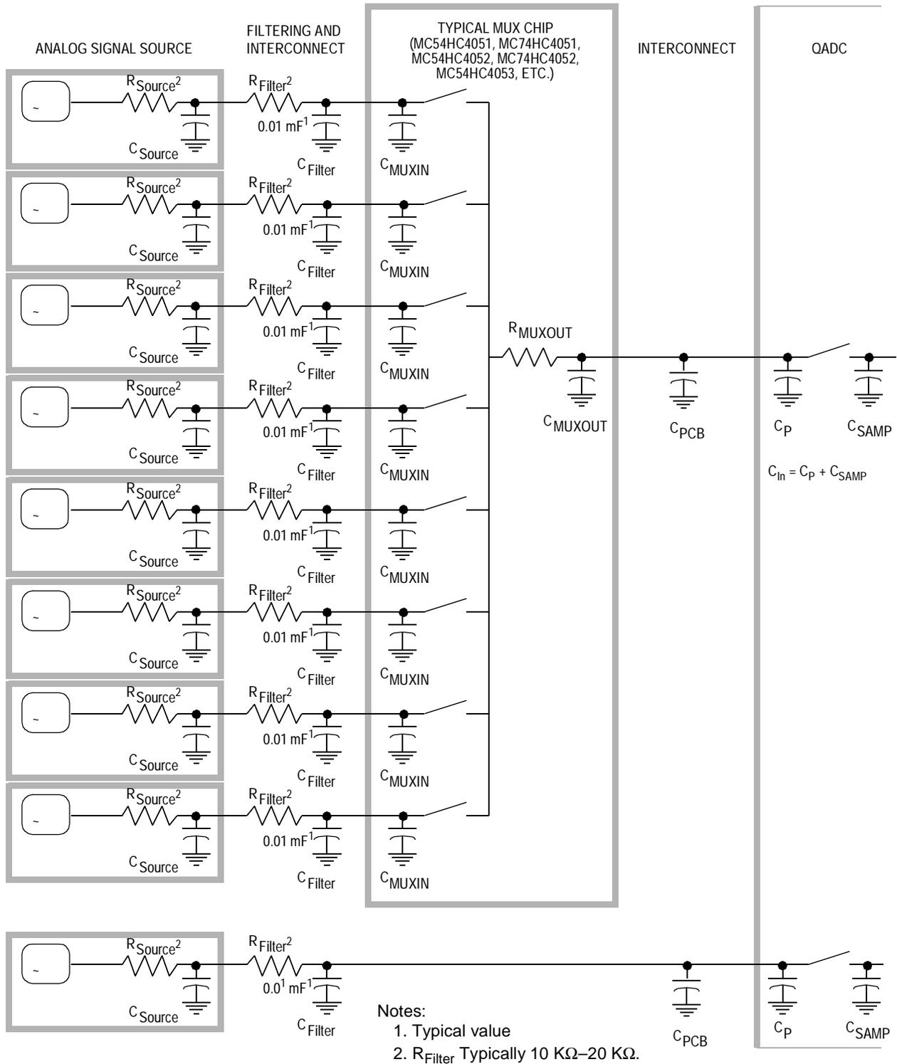
Figure 18-53. External Multiplexing of Analog Signal Sources
