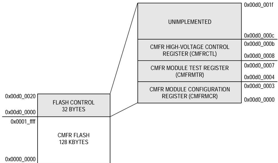
**Figure 9-2. CMFR Array and Control Register Addressing**
