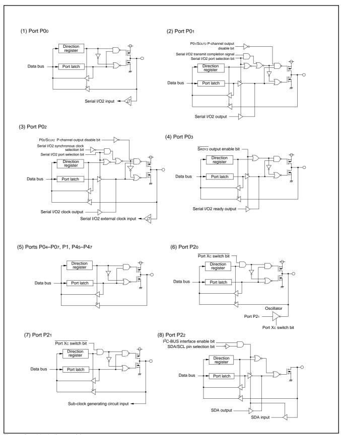
Fig. 10 Port block diagram (1)
