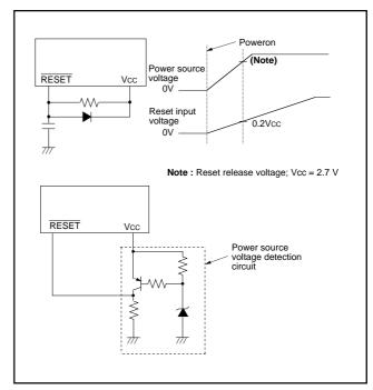
Fig. 49 Reset circuit example
