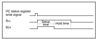
Fig. 34 START condition generating timing diagram
