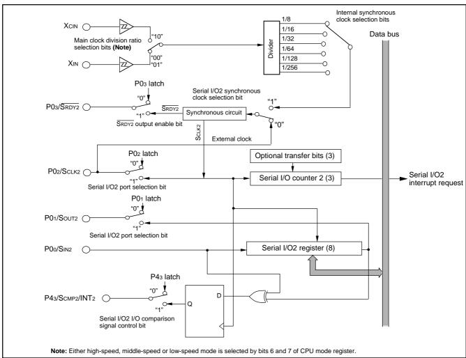
Fig. 24 Block diagram of Serial I/O2
