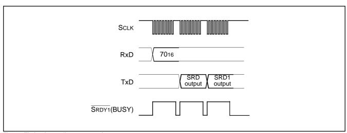
Fig. 67 Timing for reading status register
