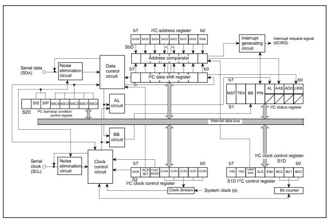
Fig. 27 Block diagram of multi-master I<sup>2</sup>C-BUS interface
