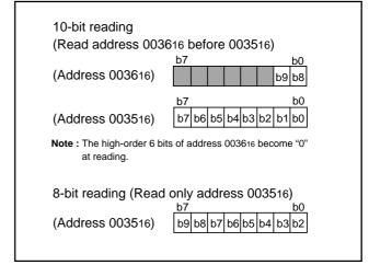
Fig. 45 Structure of A-D conversion registers
