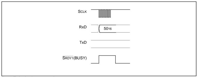
Fig. 68 Timing for clear status register
