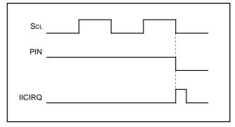
Fig. 33 Interrupt request signal generating timing
