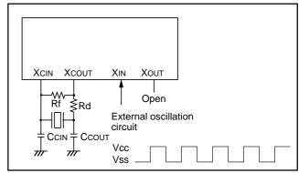
Fig. 53 External clock input circuit
