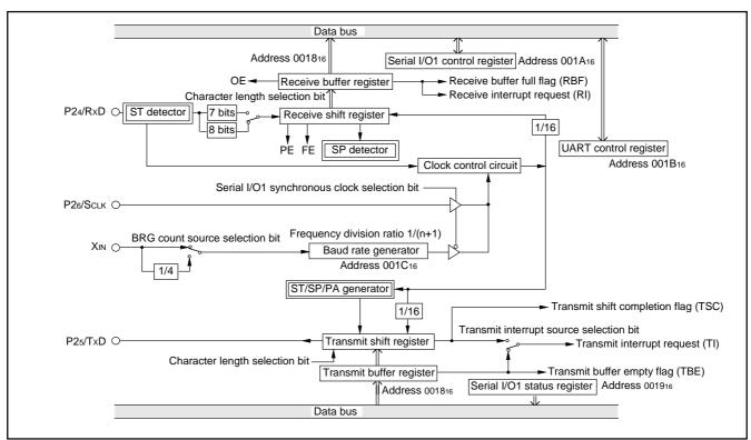
Fig. 20 Block diagram of UART serial I/O1
