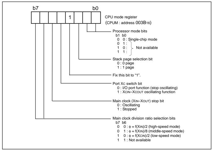
Fig. 7 Structure of CPU mode register
