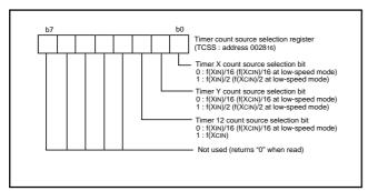
Fig. 16 Structure of timer count source selection register
