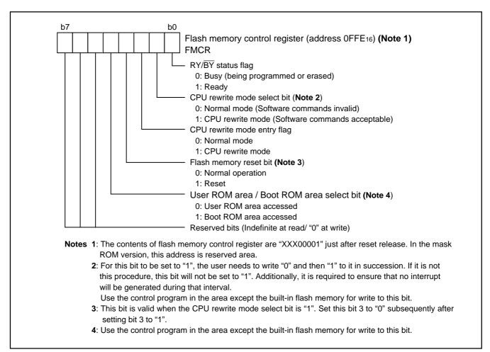
Fig. 58 Structure of flash memory control register
