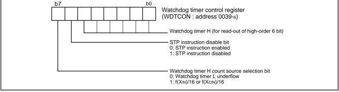
Fig. 48 Structure of Watchdog timer control register
