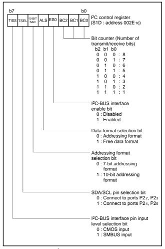
Fig. 31 Structure of I<sup>2</sup>C control register
