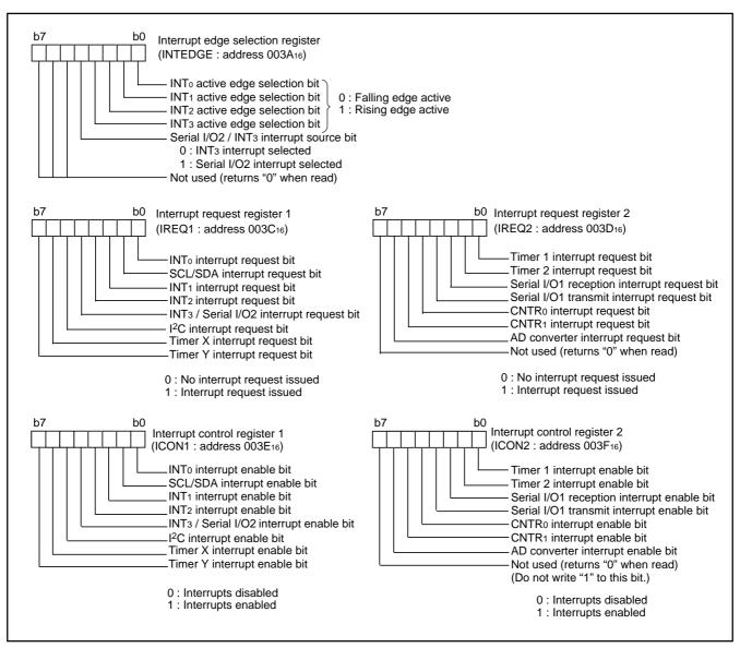
Fig. 14 Structure of interrupt-related registers
