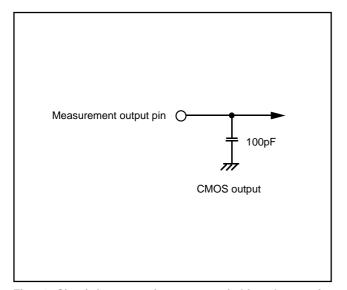
Fig. 79 Circuit for measuring output switching characteristics (1)
