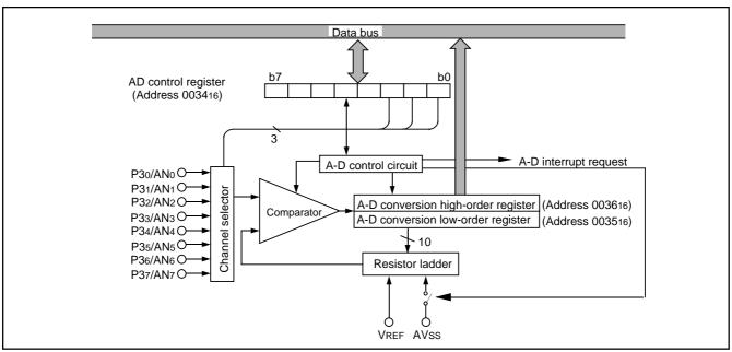
Fig. 46 Block diagram of A-D converter
