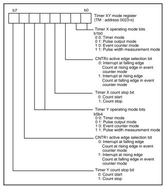
Fig. 15 Structure of timer XY mode register
