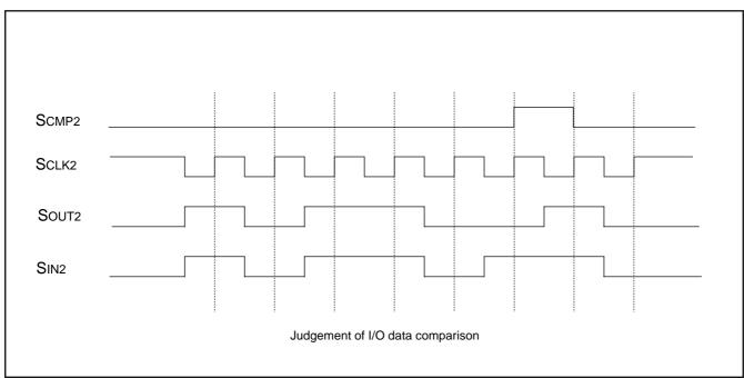
Fig. 26 ScMP2 output operation
