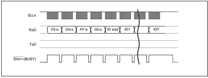
Fig. 73 Timing for ID check
