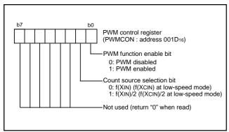
Fig. 42 Structure of PWM control register
