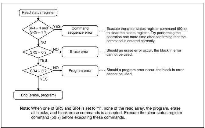
Fig. 62 Full status check flowchart and remedial procedure for errors
