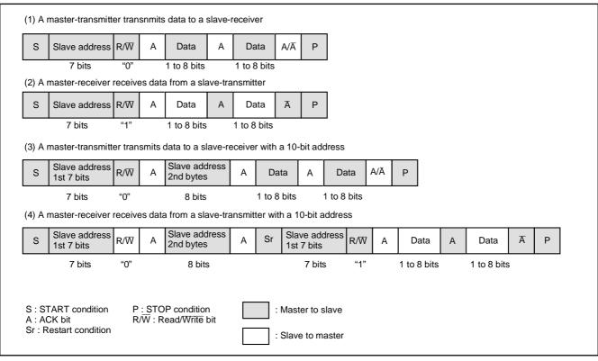
Fig. 39 Address data communication format
