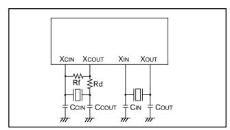
Fig. 52 Ceramic resonator circuit
