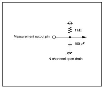
Fig. 80 Circuit for measuring output switching characteristics (2)
