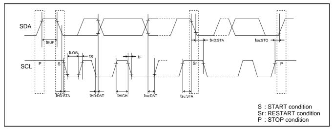
Fig. 78 Timing diagram of multi-master I<sup>2</sup>C-BUS
