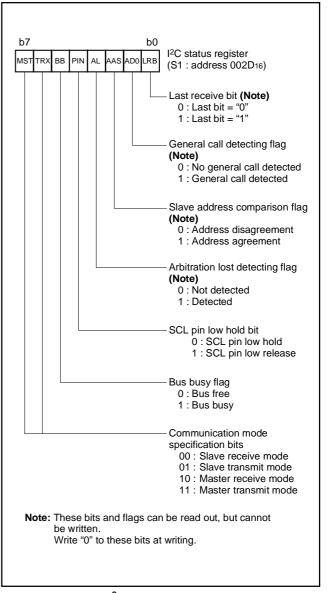
Fig. 32 Structure of I<sup>2</sup>C status register
