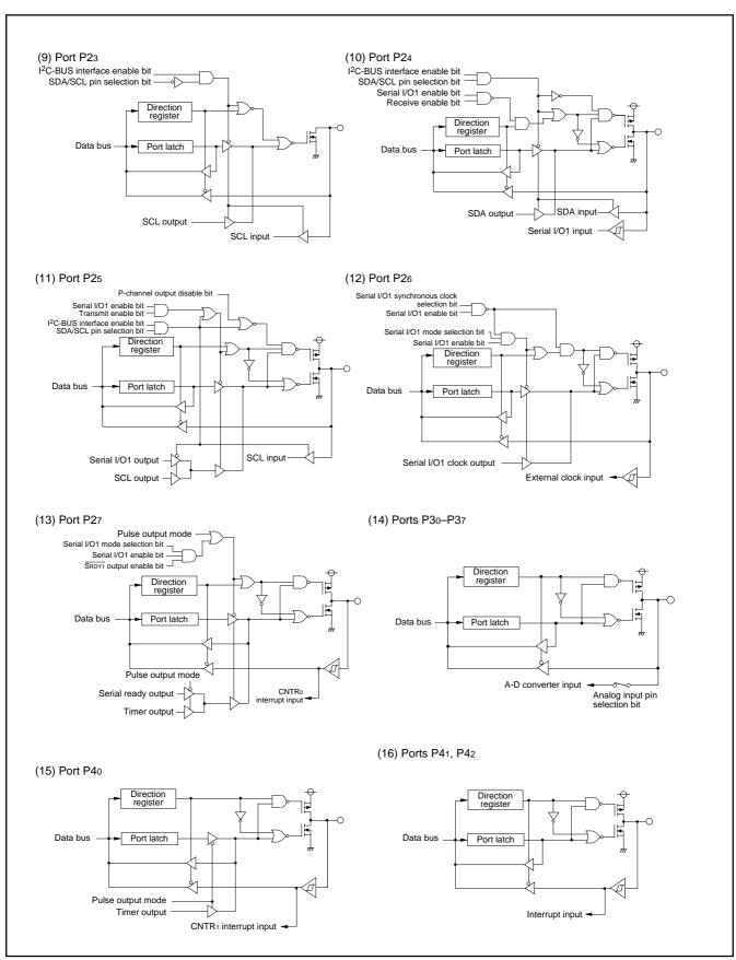
Fig. 11 Port block diagram (2)
