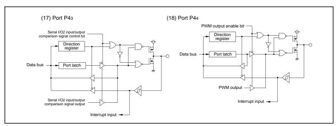
Fig. 12 Port block diagram (3)
