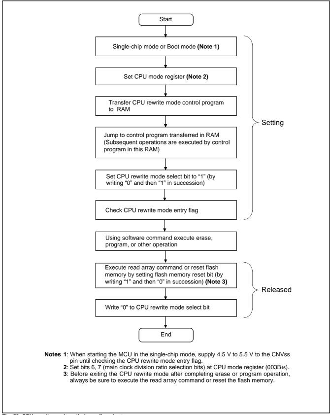
Fig. 59 CPU rewrite mode set/release flowchart
