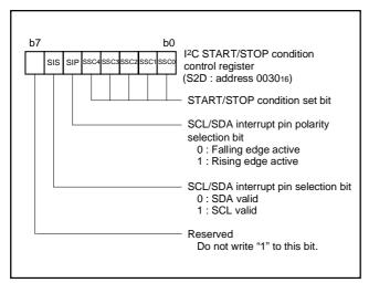
Fig. 38 Structure of I<sup>2</sup>C START/STOP condition control register
