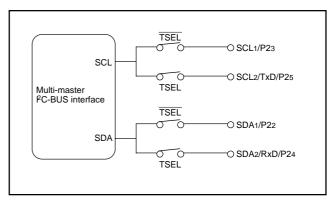
Fig. 30 SDA/SCL pin selection bit
