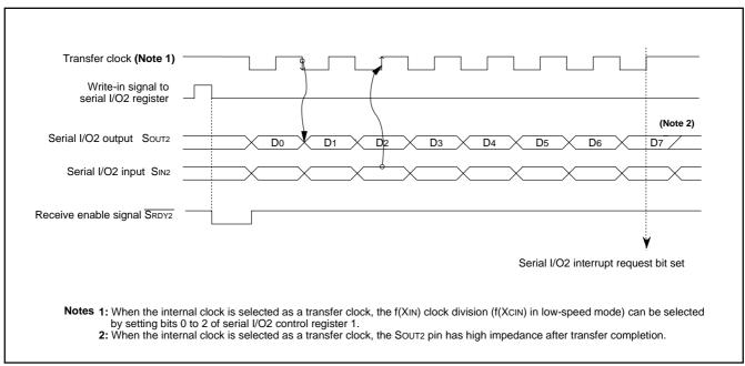
Fig. 25 Timing chart of Serial I/O2
