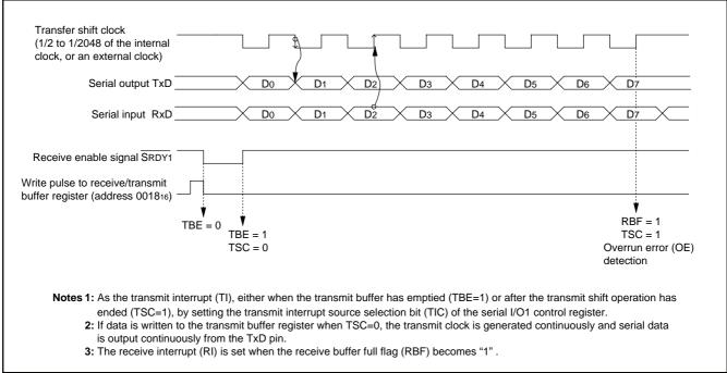
Fig. 19 Operation of clock synchronous serial I/O1 function
