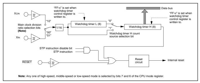
Fig. 47 Block diagram of Watchdog timer
