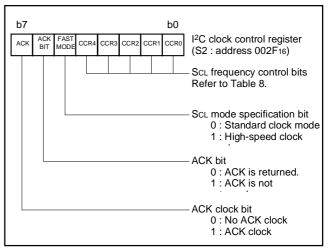
Fig. 29 Structure of I<sup>2</sup>C clock control register
