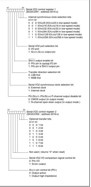
Fig. 23 Structure of Serial I/O2 control registers 1, 2
