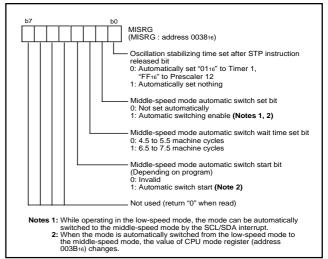
Fig. 54 Structure of MISRG
