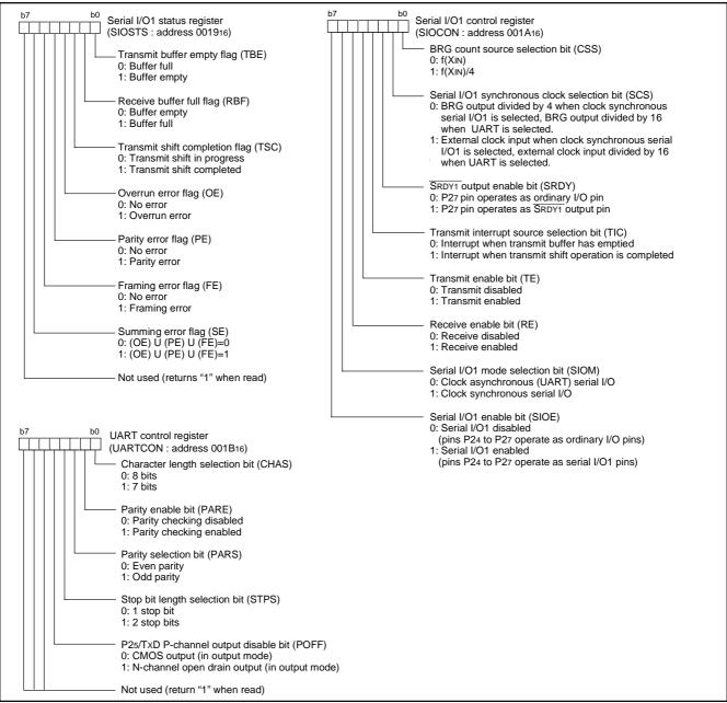
Fig. 22 Structure of serial I/O1 control registers
