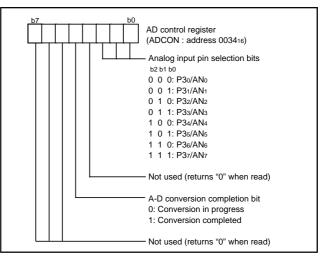
Fig. 44 Structure of AD control register
