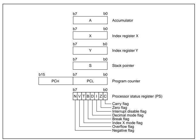
Fig. 5 740 Family CPU register structure
