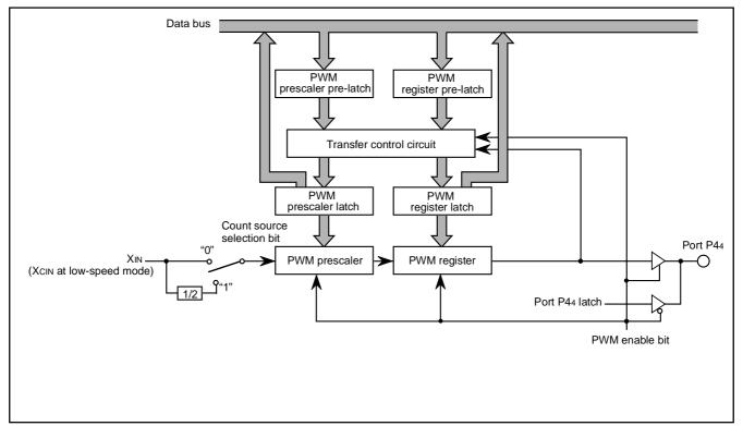
Fig. 41 Block diagram of PWM function
