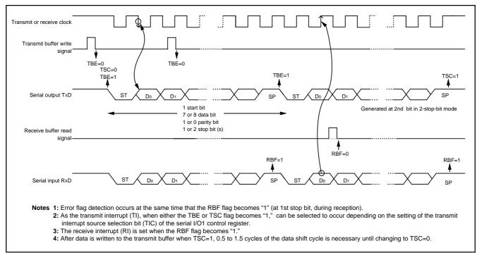
Fig. 21 Operation of UART serial I/O1 function
