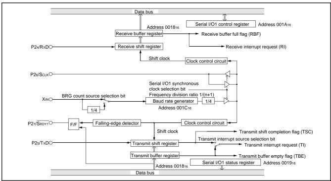
Fig. 18 Block diagram of clock synchronous serial I/O1
