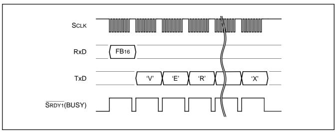
Fig. 72 Timing for version information output
