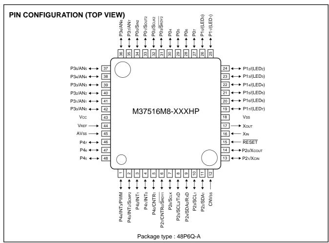
Fig. 1 M37516F8HP pin configuration
