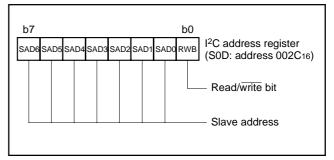
Fig. 28 Structure of I<sup>2</sup>C address register
