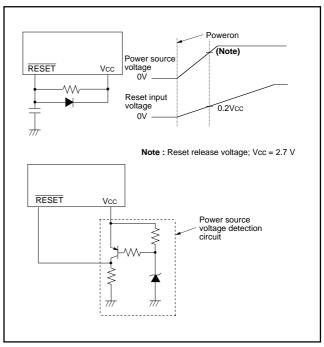
Fig. 48 Reset circuit example
