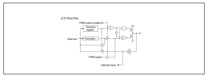
Fig. 15 Port block diagram (3) (spec. H)
