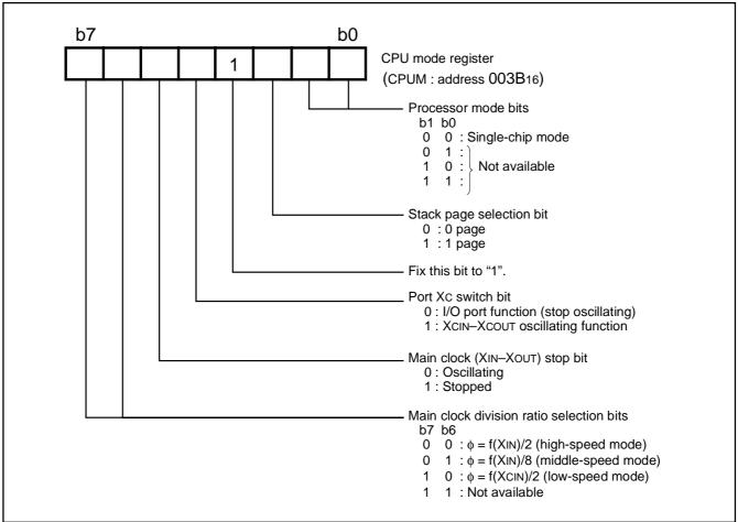
Fig. 9 Structure of CPU mode register
