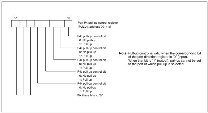
Fig. 20 Structure of port registers (2) (spec. A)
