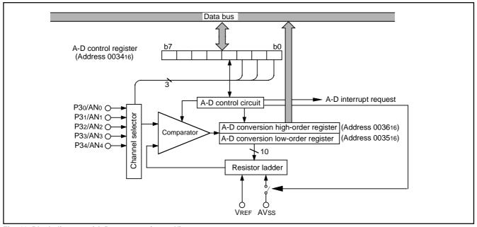
Fig. 41 Block diagram of A-D converter (spec. H)
