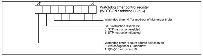
Fig. 47 Structure of Watchdog timer control register
