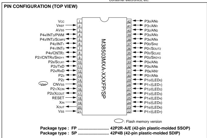
Fig. 2 M38503MXA-XXXFP/SP pin configuration (spec. A)
