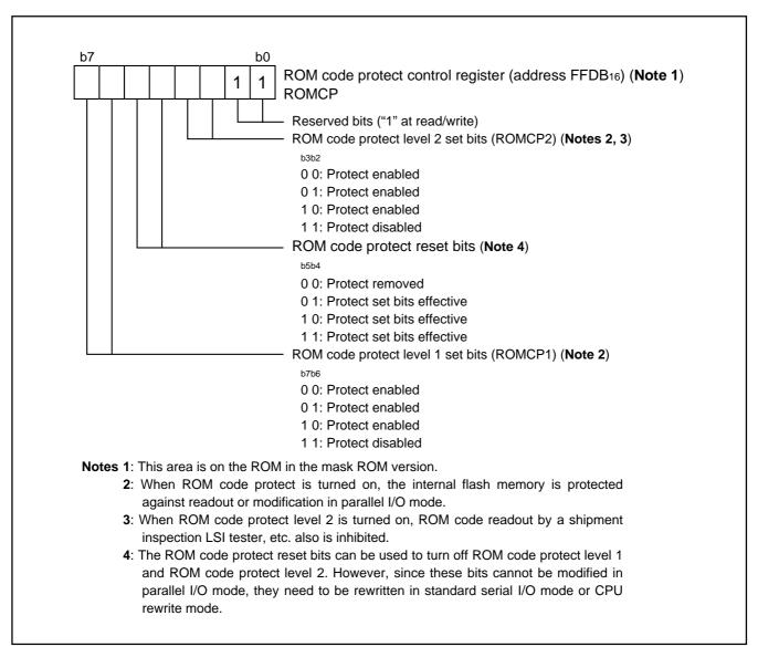
Fig. 63 Structure of ROM code protect control
