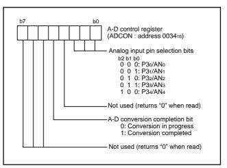
Fig. 39 Structure of A-D control register (spec. H)
