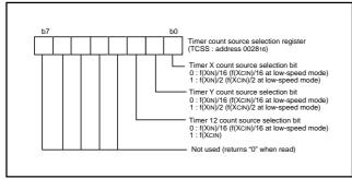
Fig. 24 Structure of timer count source selection register
