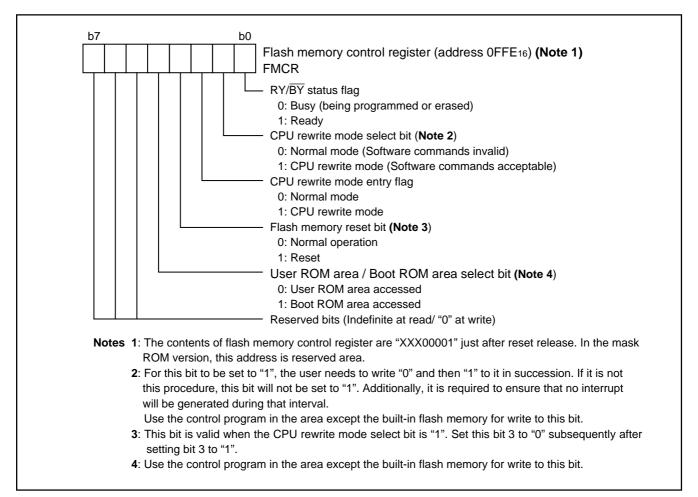
Fig.58 Structure of flash memory control register
