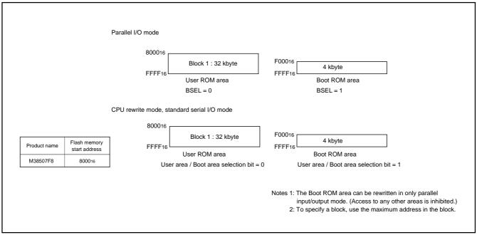
Fig. 57 Block diagram of built-in flash memory
