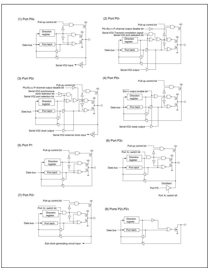
Fig. 16 Port block diagram (1) (spec. A)
