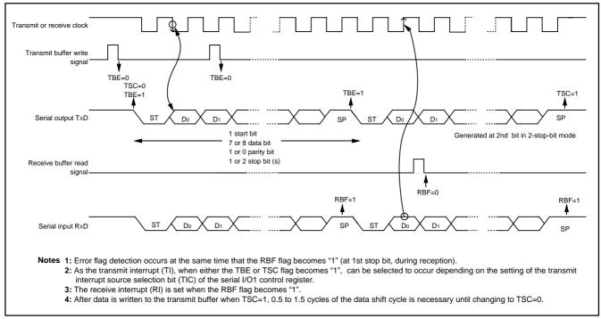
Fig. 29 Operation of UART serial I/O1 function
