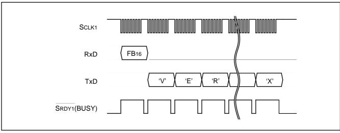
Fig. 72 Timing for version information output
