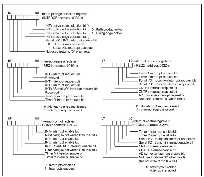
Fig. 22 Structure of interrupt-related registers
