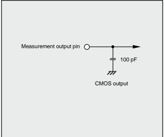
Fig. 78 Circuit for measuring output switching characteristics
