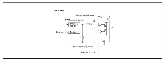
Fig. 18 Port block diagram (3) (spec. A)
