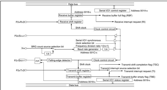
Fig. 26 Block diagram of clock synchronous serial I/O1
