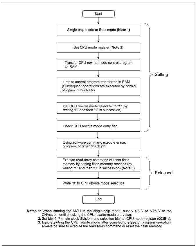
Fig. 59 CPU rewrite mode set/release flowchart
