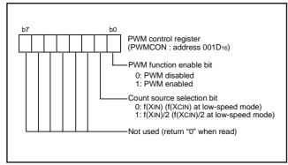
Fig. 37 Structure of PWM control register
