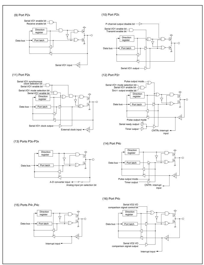
Fig. 14 Port block diagram (2) (spec. H)
