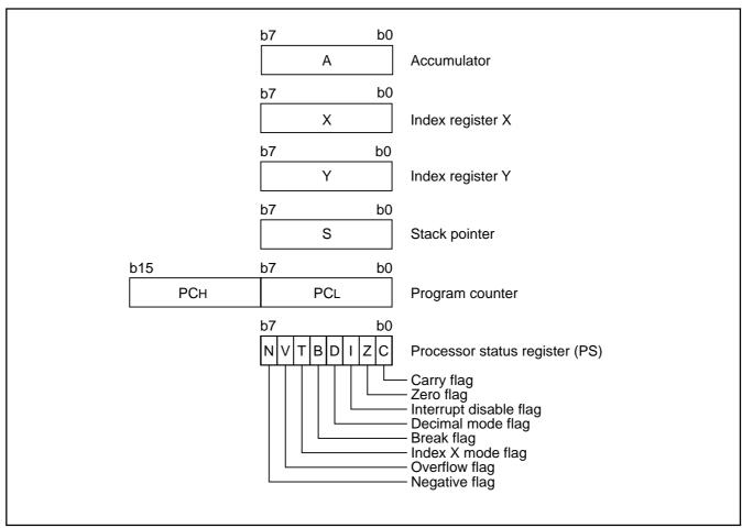
Fig. 7 740 Family CPU register structure
