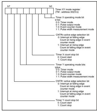
Fig. 23 Structure of timer XY mode register
