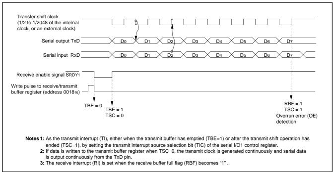
Fig. 27 Operation of clock synchronous serial I/O1 function
