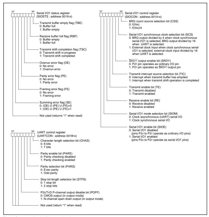
Fig. 30 Structure of serial I/O1 control registers
