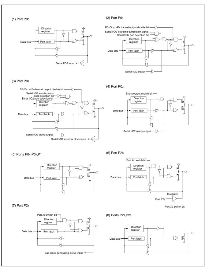
Fig. 13 Port block diagram (1) (spec. H)
