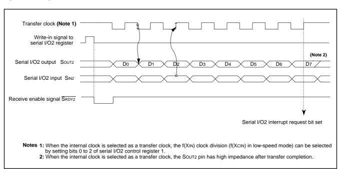
Fig. 33 Timing chart of Serial I/O2
