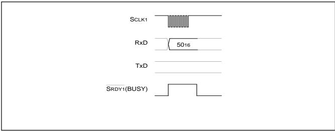
Fig. 68 Timing for clear status register
