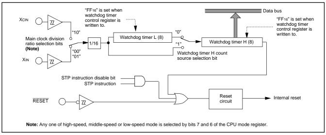
Fig. 46 Block diagram of Watchdog timer
