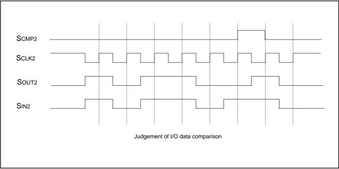
Fig. 34 ScMP2 output operation
