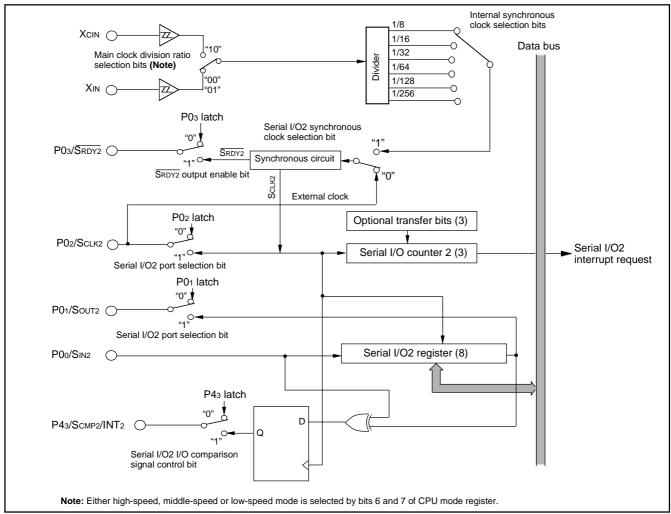
Fig. 32 Block diagram of Serial I/O2
