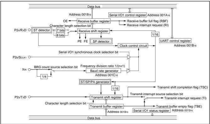
Fig. 28 Block diagram of UART serial I/O1
