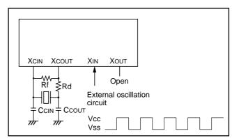
Fig. 53 External clock input circuit
