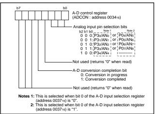
Fig. 42 Structure of A-D control register (spec. A)
