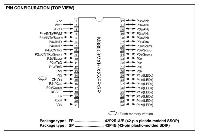
Fig. 1 M38503MXH-XXXFP/SP pin configuration (spec. H)
