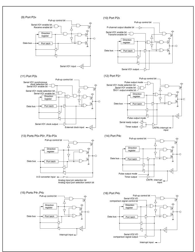
Fig. 17 Port block diagram (2) (spec. A)
