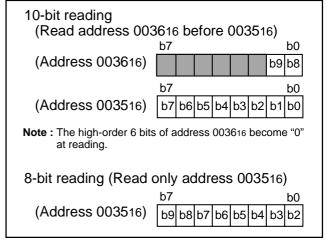
Fig. 44 Structure of A-D conversion registers (spec. A)
