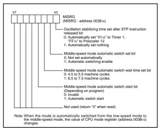
Fig. 54 Structure of MISRG
