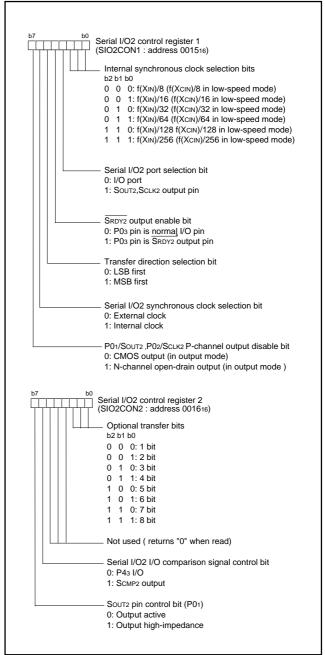
Fig. 31 Structure of Serial I/O2 control registers 1, 2
