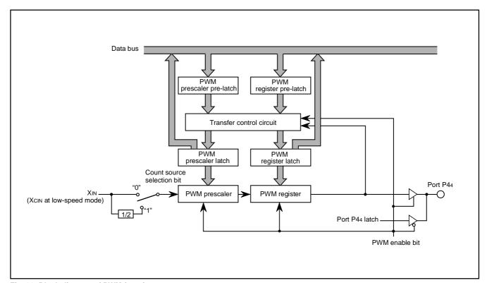
Fig. 36 Block diagram of PWM function
