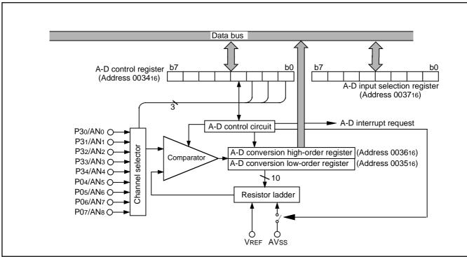
Fig. 45 Block diagram of A-D converter (spec. A)
