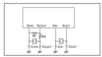
Fig. 52 Ceramic resonator circuit
