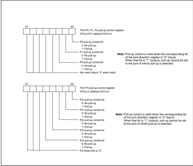
Fig. 19 Structure of port registers (1) (spec. A)
