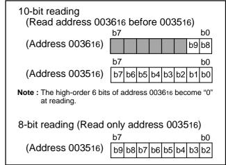
Fig. 40 Structure of A-D conversion registers (spec. H)
