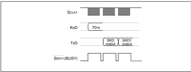
Fig. 67 Timing for reading status register
