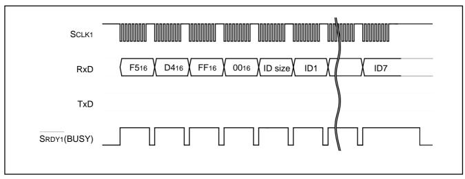
Fig. 73 Timing for ID check
