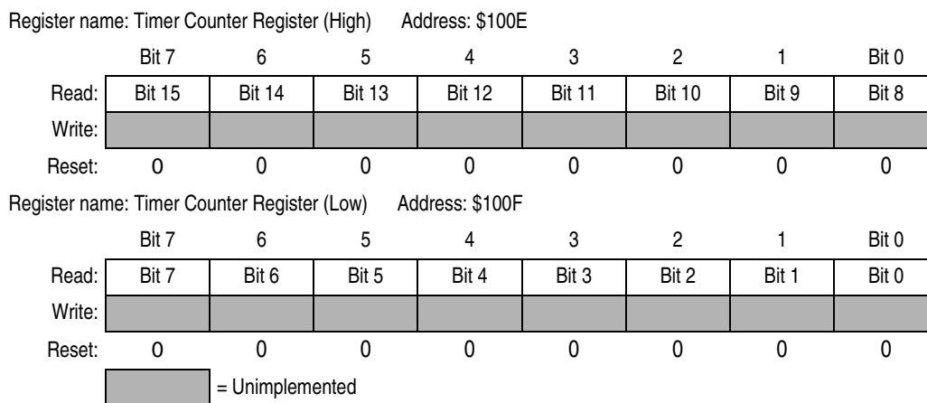
Figure 9-15. Timer Counter Register (TCNT)
