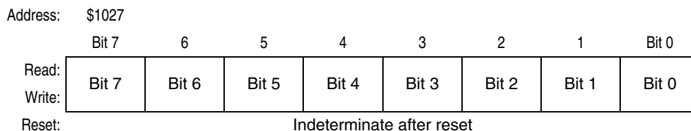
Figure 9-26. Pulse Accumulator Count Register (PACNT)
