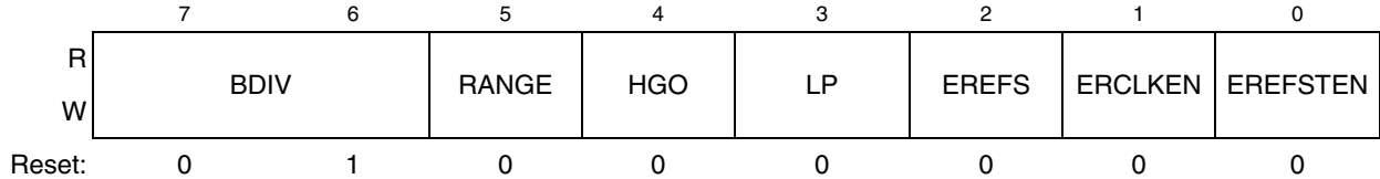
Figure 10-4. ICS Control Register 2 (ICSC2)
