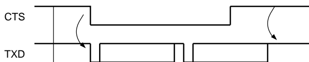
Figure 21-28. Transmitter Behavior when Operating with Hardware Handshaking
