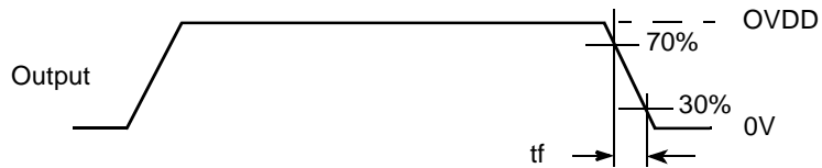
Figure 7. Definition of Timing for Standard and Fast-Mode
