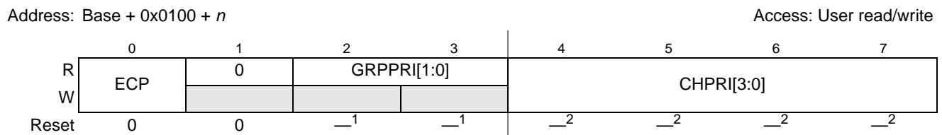
Figure 9-21. DMA Channel n Priority Register (DCHPRI n )
