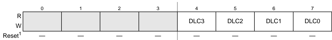
Figure 22-29. Data Length Register (DLR)—Extended Identifier Mapping
