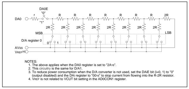
Figure 19.3 D/A Converter Equivalent Circuit
