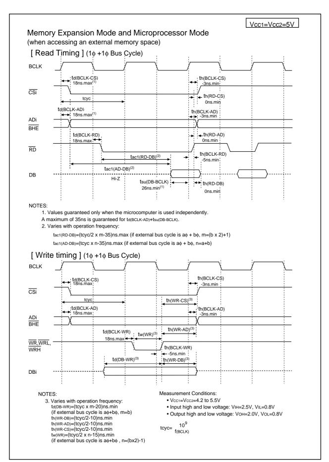
Figure 26.3 Vcc1=Vcc2=5V Timing Diagram (1)
