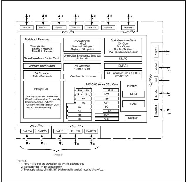
Figure 1.1 M32C/84 Group (M32C/84, M32C/84T) Block Diagram
