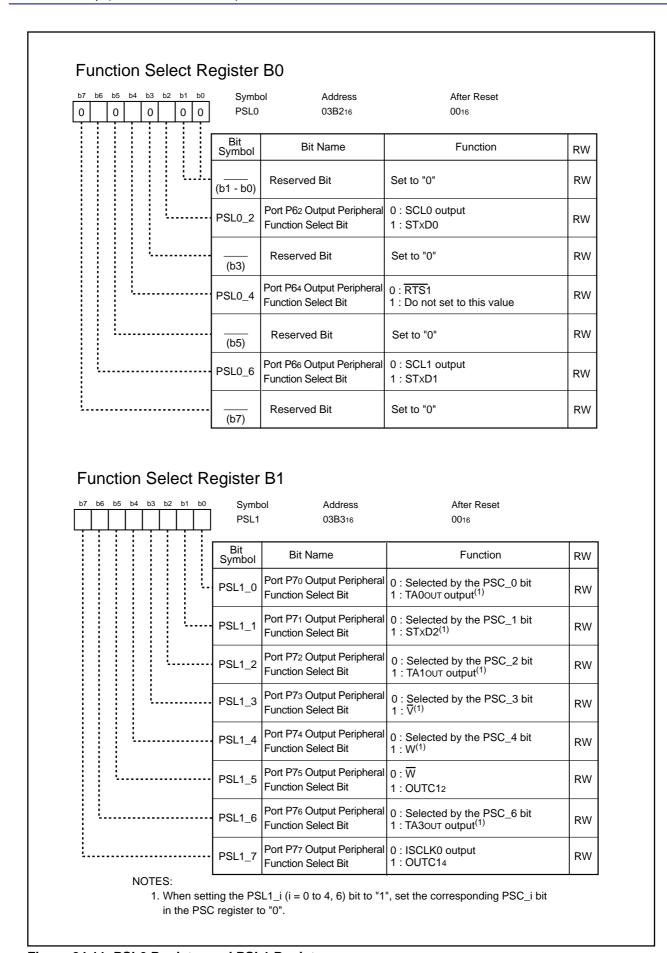
Figure 24.11 PSL0 Register and PSL1 Register
