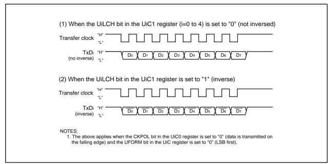
Figure 17.13 Serial Data Logic Inverse
