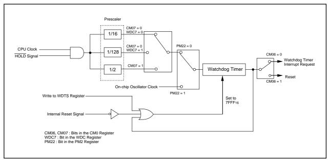
Figure 12.1 Watchdog Timer Block Diagram
