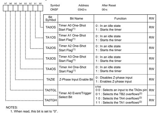
Figure 15.6 UDF Register and ONSF Register
