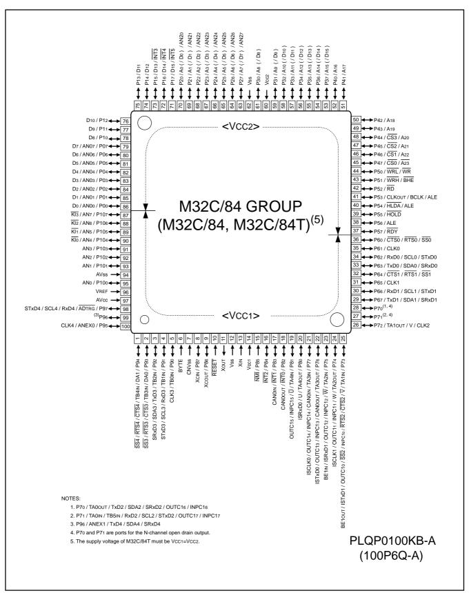
Figure 1.5 Pin Assignment for 100-Pin Package
