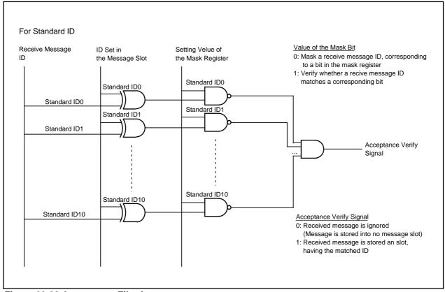
Figure 23.28 Acceptance Filtering
