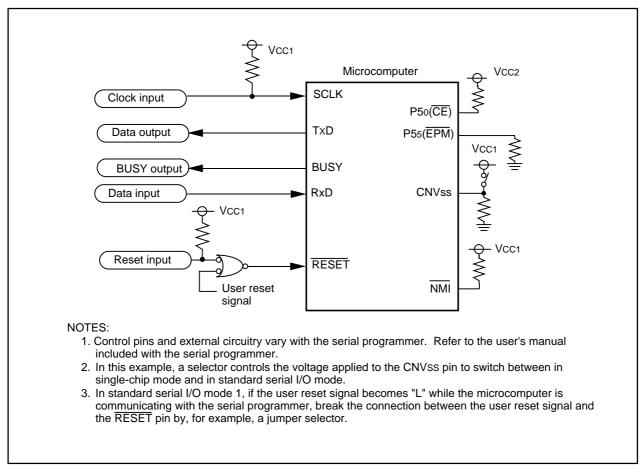
Figure 25.17 Circuit Application in Standard Serial I/O Mode 1
