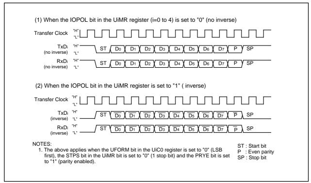
Figure 17.18 TxD and RxD I/O Polarity Inverse
