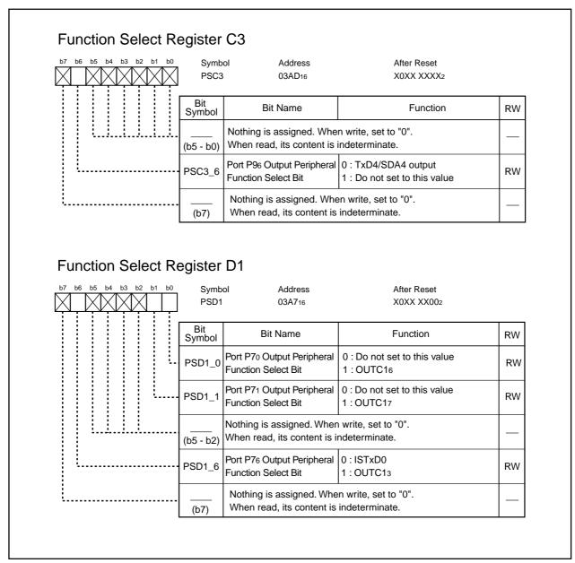
Figure 24.14 PSC3 Register and PSD1 Register
