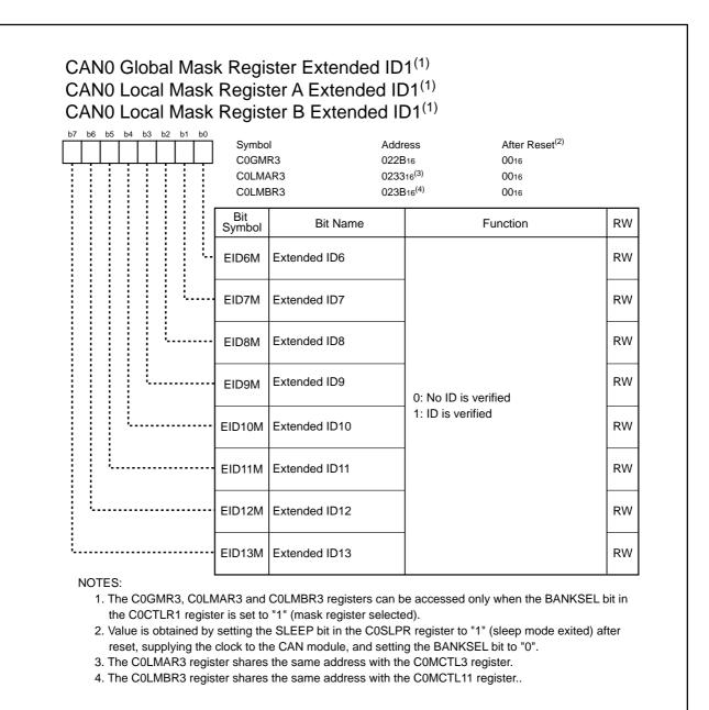
Figure 23.25 C0GMR3, C0LMAR3 and C0LMBR3 Registers
