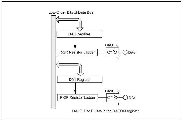
Figure 19.1 D/A Converter
