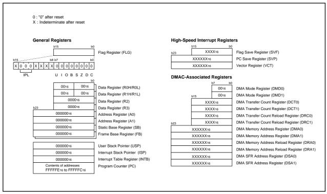
Figure 5.4 CPU Register States after Reset
