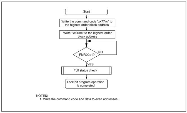
Figure 25.11 Lock Bit Program Command
