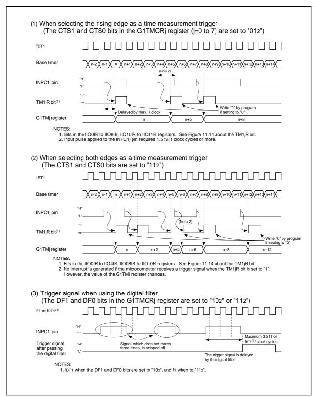
Figure 22.14 Time Measurement Function (2)
