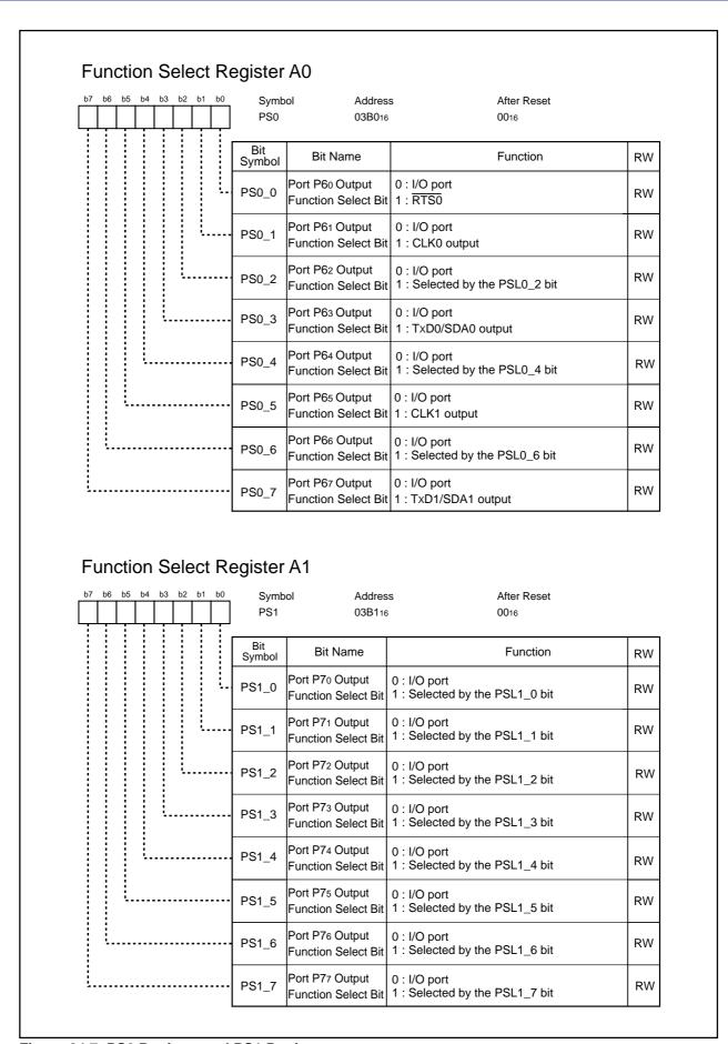
Figure 24.7 PS0 Register and PS1 Register
