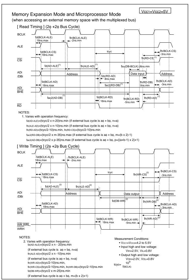
Figure 26.4 Vcc1=Vcc2=5V Timing Diagram (2)
