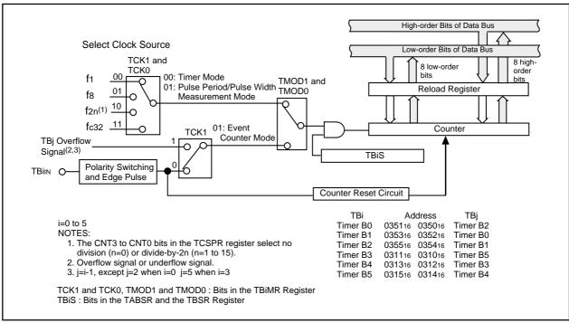
Figure 15.16 Timer B Block Diagram
