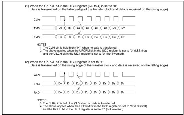
Figure 17.11 Transfer Clock Polarity
