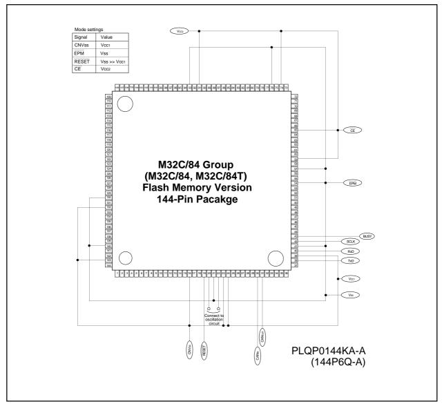
Figure 25.16 Pin Connections in Standard Serial I/O Mode (3)
