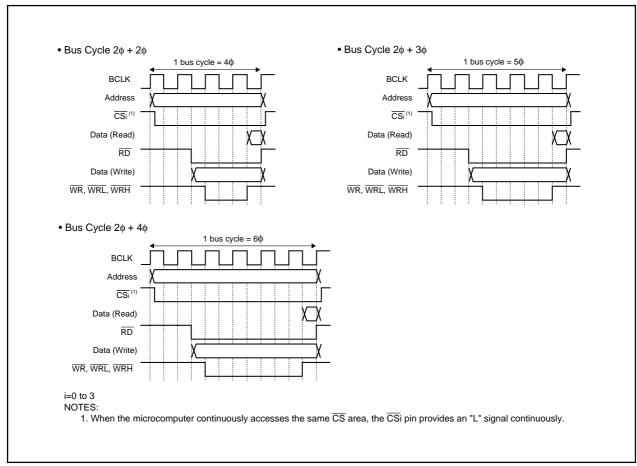
Figure 8.5 Bus Cycle with Separate Bus (2)
