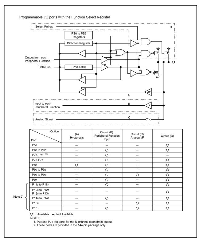
Figure 24.3 Programmable I/O Ports (3)
