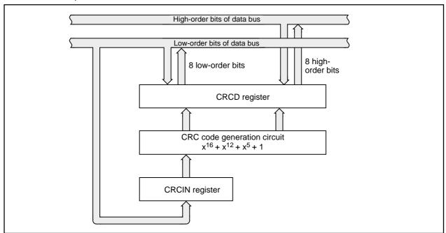
Figure 20.1 CRC Calculation Block Diagram
