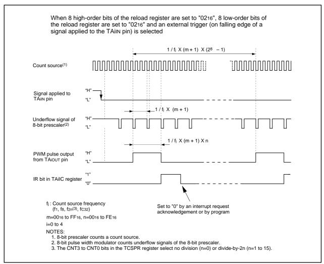
Figure 15.15 8-bit Pulse Width Modulator Operation
