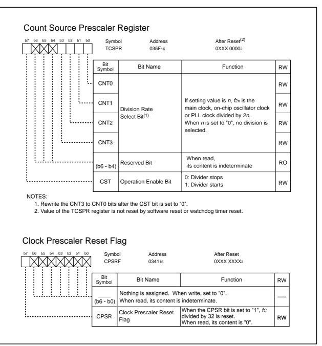
Figure 9.6 TCSPR and CPSRF Registers
