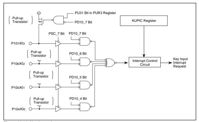
Figure 11.11 Key Input Interrupt
