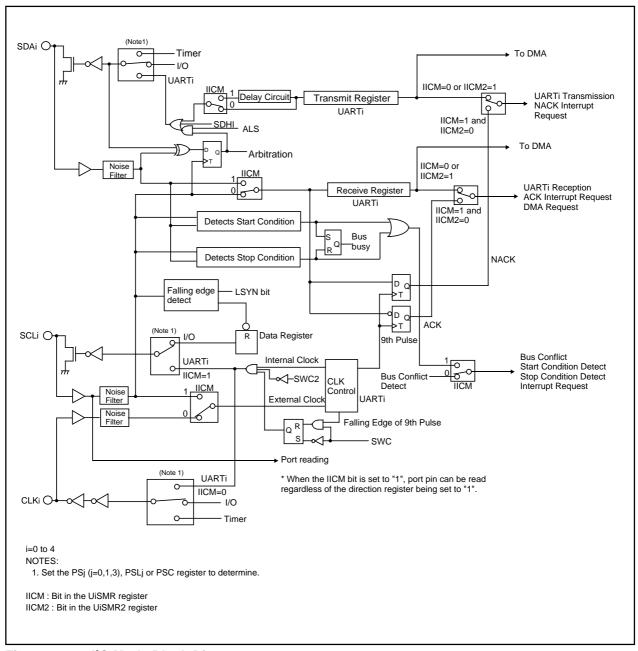
Figure 17.19 I<sup>2</sup>C Mode Block Diagram
