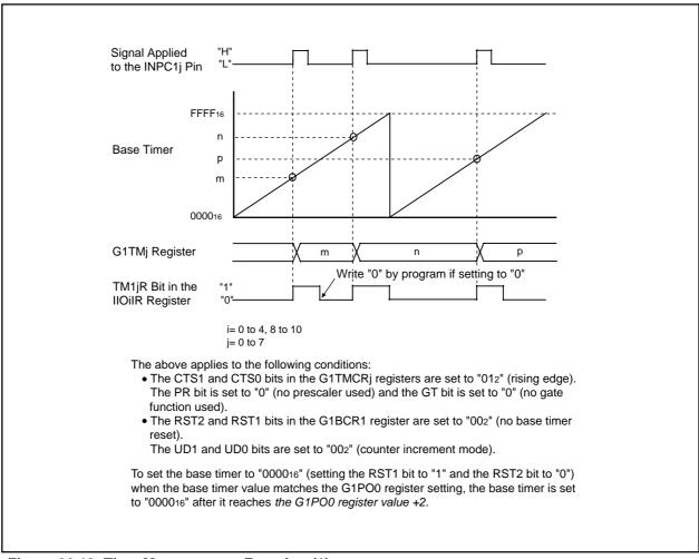
Figure 22.13 Time Measurement Function (1)
