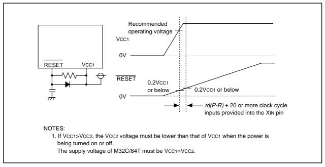
Figure 5.1 Reset Circuit
