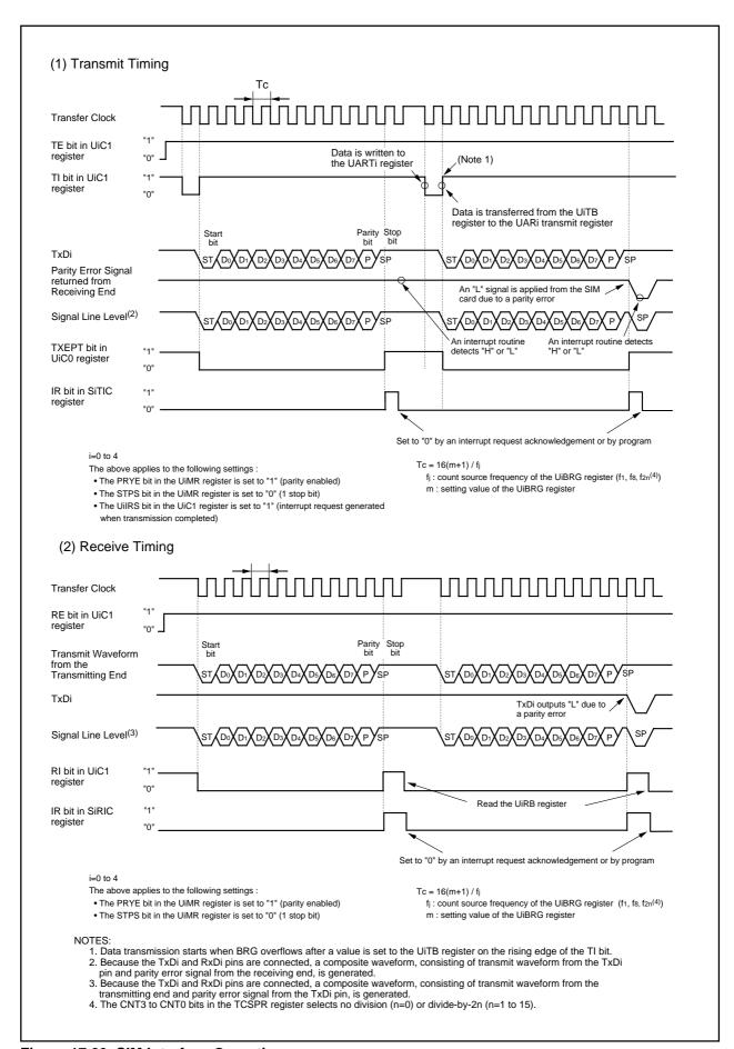
Figure 17.29 SIM Interface Operation
