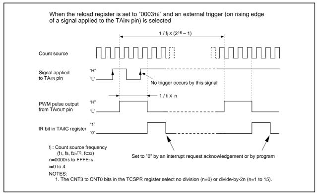
Figure 15.14 16-bit Pulse Width Modulator Operation
