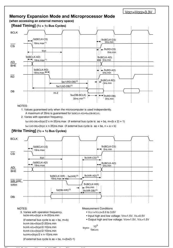
Figure 26.7 Vcc1=Vcc2=3.3V Timing Diagram (1)
