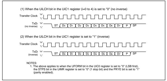
Figure 17.17 Serial Data Logic Inverse
