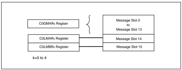
Figure 23.27 Mask Registers and Message Slots
