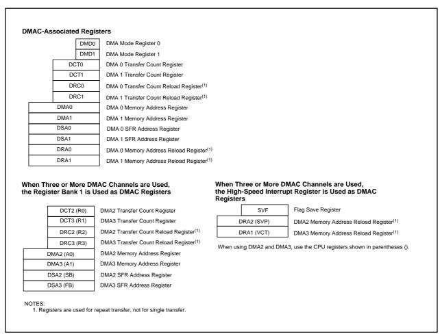
Figure 13.1 Register Mapping for DMAC
