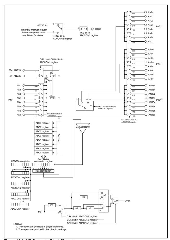
Figure 18.1 A/D Converter Block Diagram
