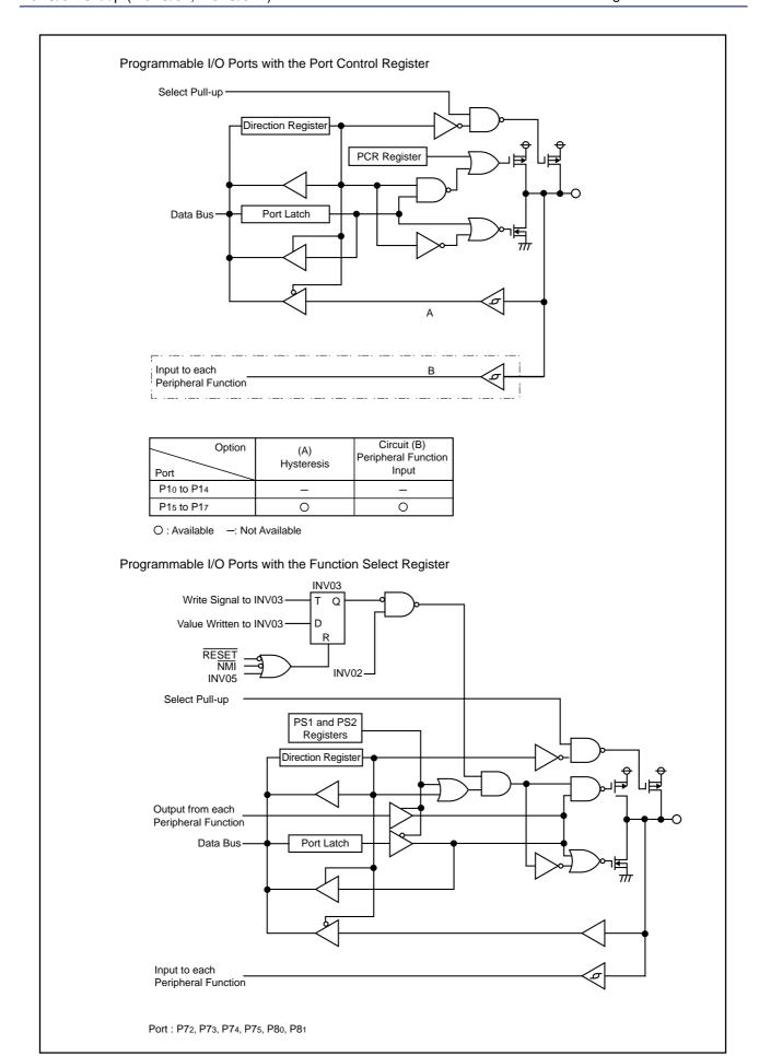
Figure 24.2 Programmable I/O Ports (2)
