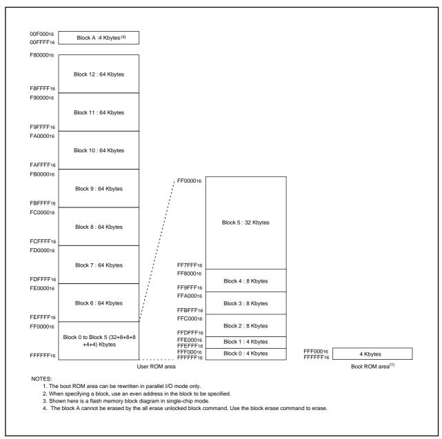
Figure 25.1 Flash Memory Block Diagram
