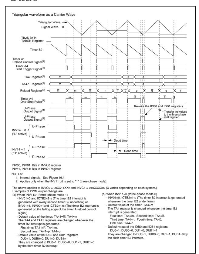
Figure 16.8 Triangular Wave Modulation Operation
