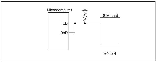
Figure 17.30 SIM Interface Connection
