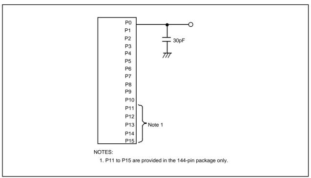
Figure 26.2 P0 to P15 Measurement Circuit
