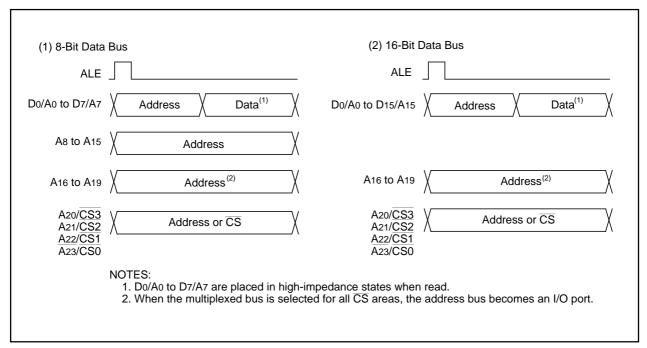
Figure 8.10 ALE Signal and Address/Data Bus
