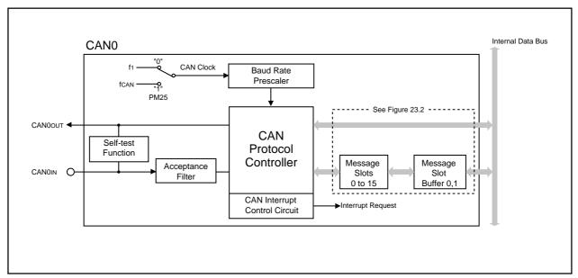
Figure 23.1 CAN Module Block Diagram
