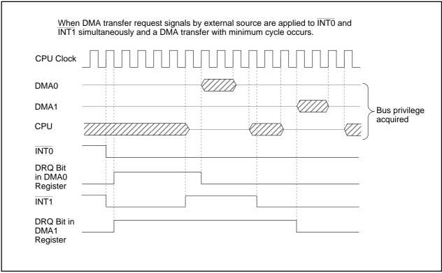
Figure 13.7 DMA Transfer by External Source
