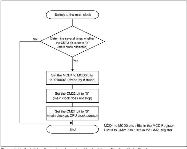
Figure 9.11 Switching Procedure from On-chip Oscillator Clock to Main Clock
