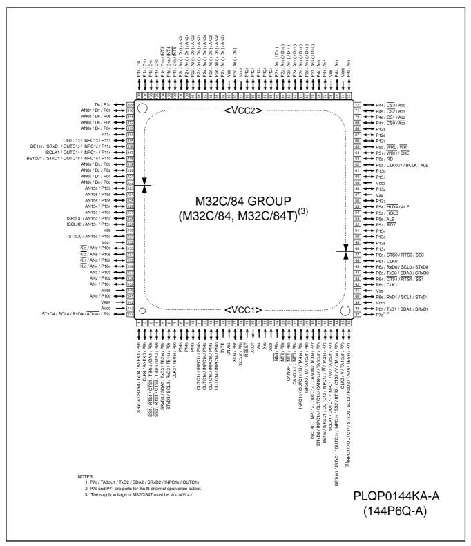
Figure 1.3 Pin Assignment for 144-Pin Package
