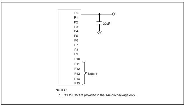
Figure 26.12 P0 to P15 Measurement Circuit
