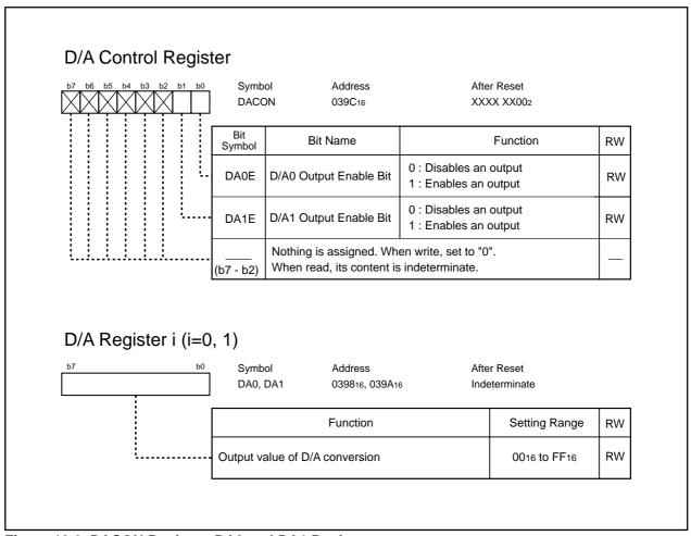
Figure 19.2 DACON Register, DA0 and DA1 Registers
