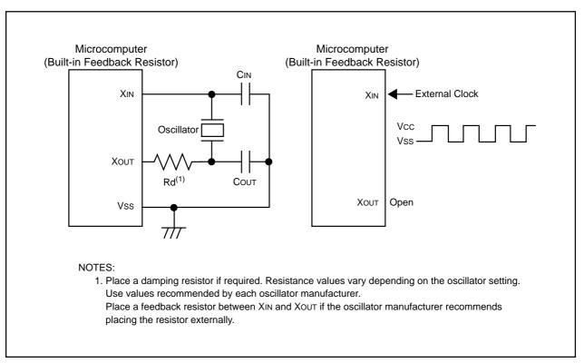
Figure 9.9 Main Clock Circuit Connection
