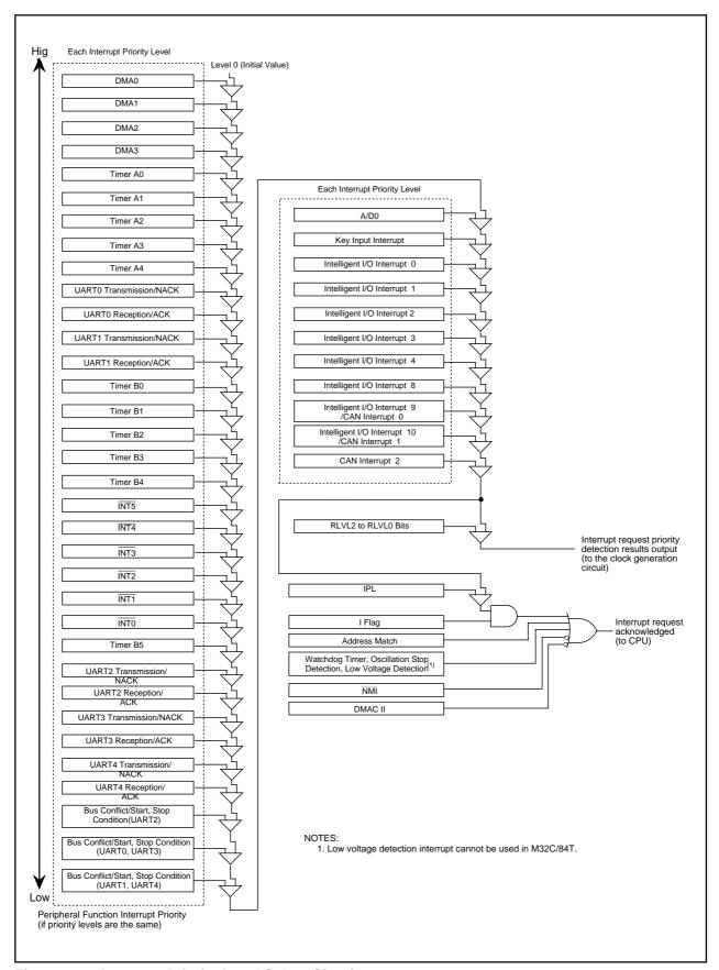
Figure 11.9 Interrupt Priority Level Select Circuit
