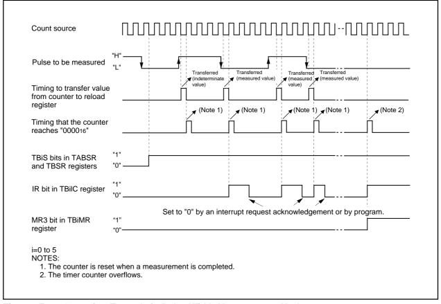
Figure 15.24 Operation Example in Pulse Width Measurement Mode
