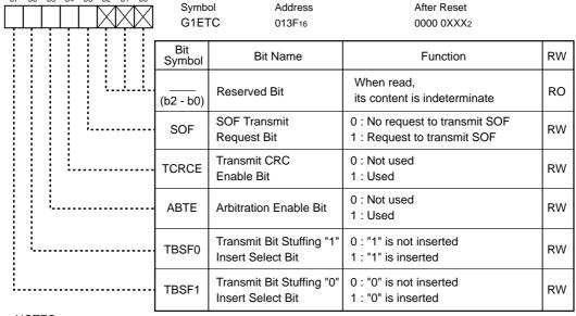
Figure 22.24 G0ETC and G1ETC Registers
