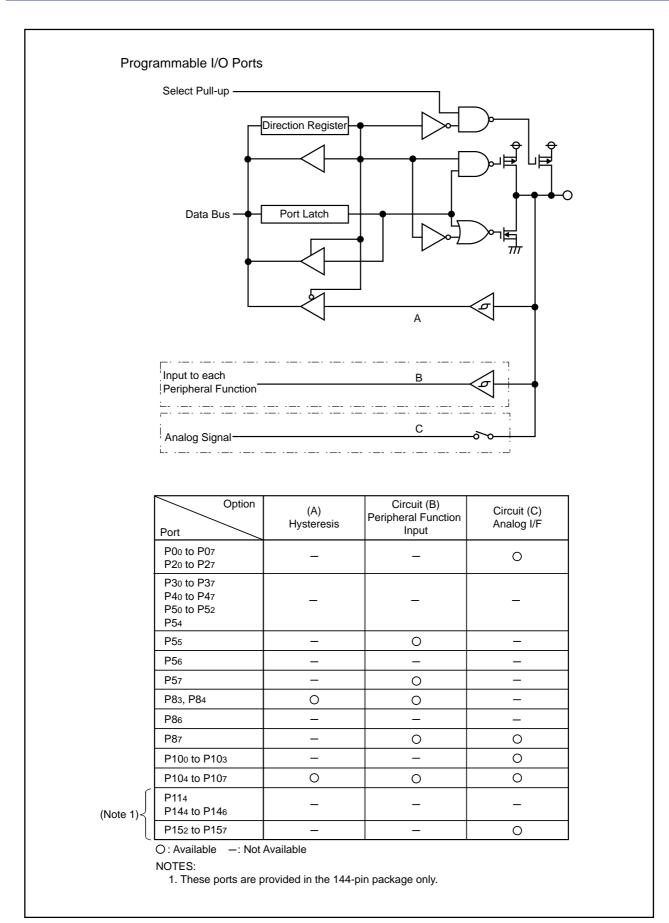
Figure 24.1 Programmable I/O Ports (1)
