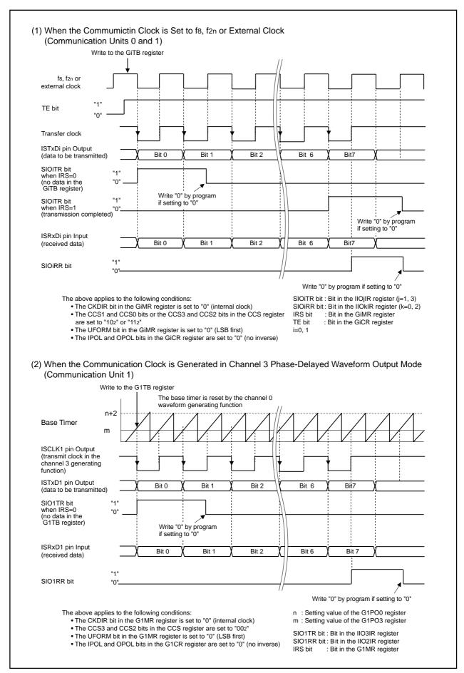
Figure 22.30 Transmit and Receive Operation
