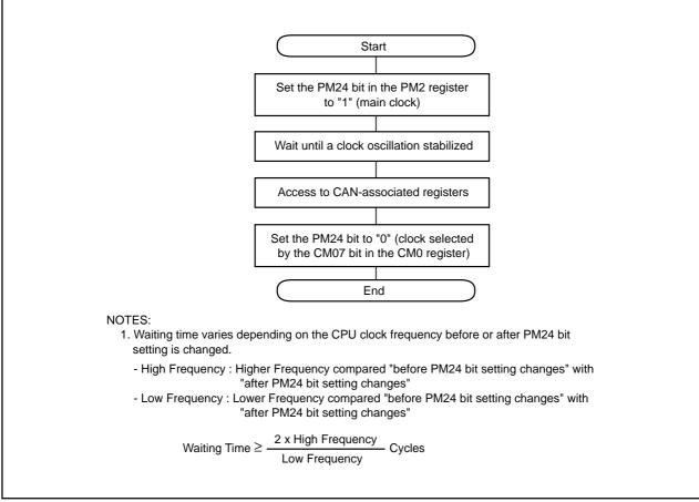
Figure 23.36 Accessing Procedure for CAN-Associated Registers
