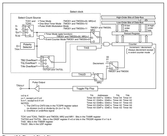
Figure 15.3 Timer A Block Diagram
