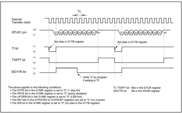
Figure 22.31 Transmit Operation
