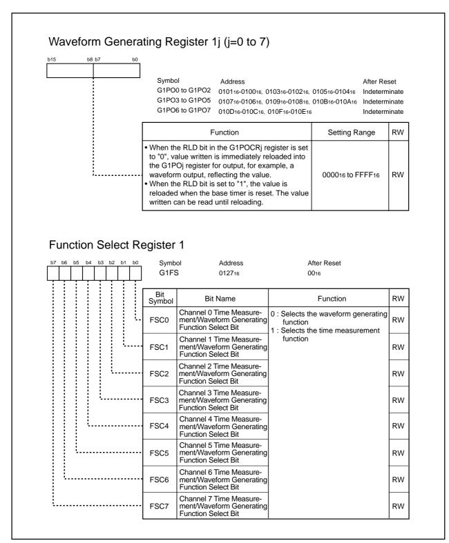
Figure 22.7 G1PO0 to G1PO7 Registers and G1FS Register
