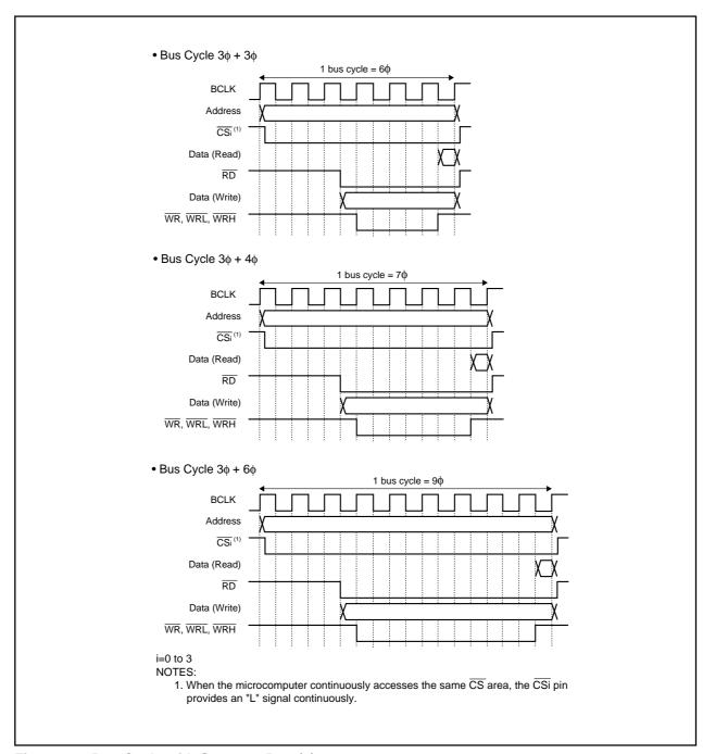
Figure 8.6 Bus Cycle with Separate Bus (3)
