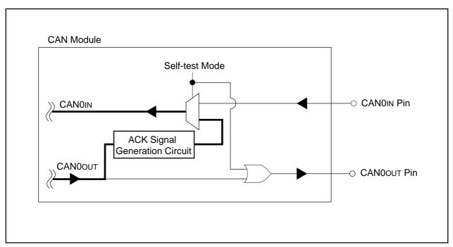
Figure 23.19 Self-Test Mode
