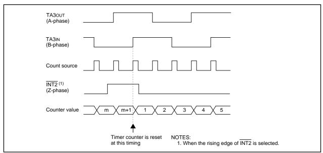
Figure 15.11 Counter Reset Timing
