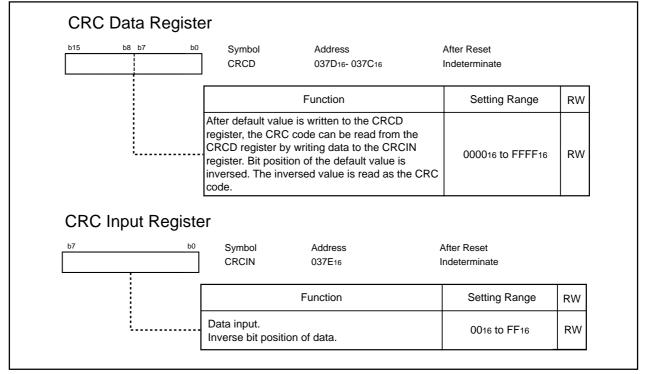
Figure 20.2 CRCD Register and CRCIN Register
