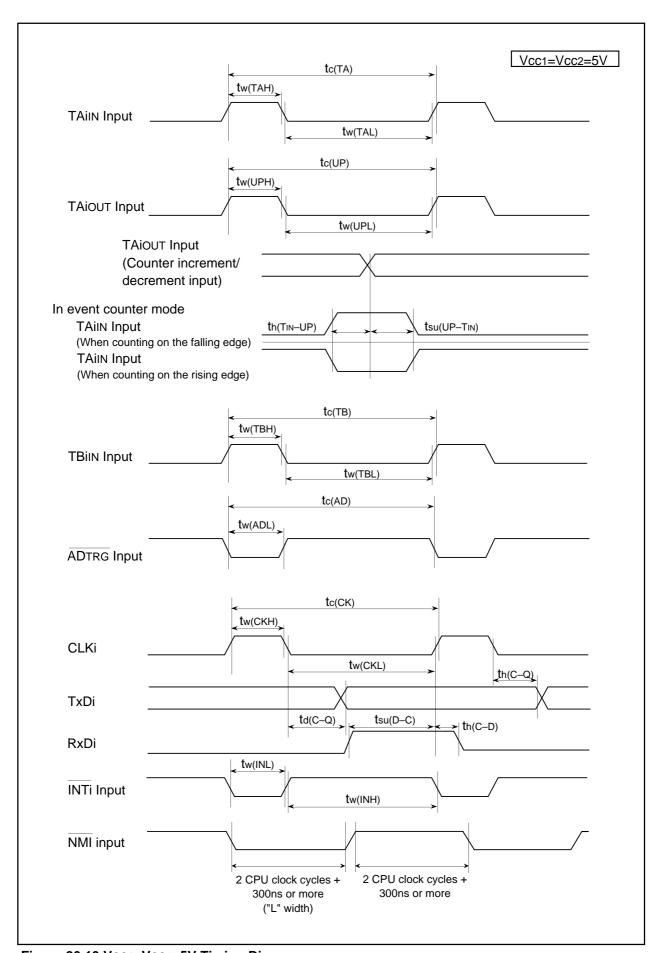
Figure 26.13 VCC1=VCC2=5V Timing Diagram
