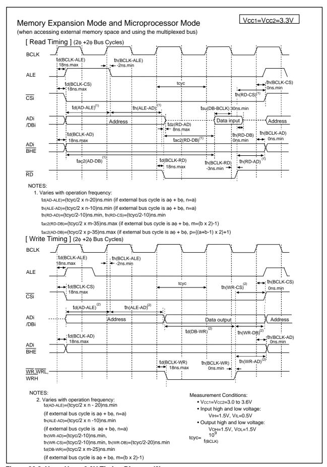
Figure 26.8 Vcc1=Vcc2=3.3V Timing Diagram (2)
