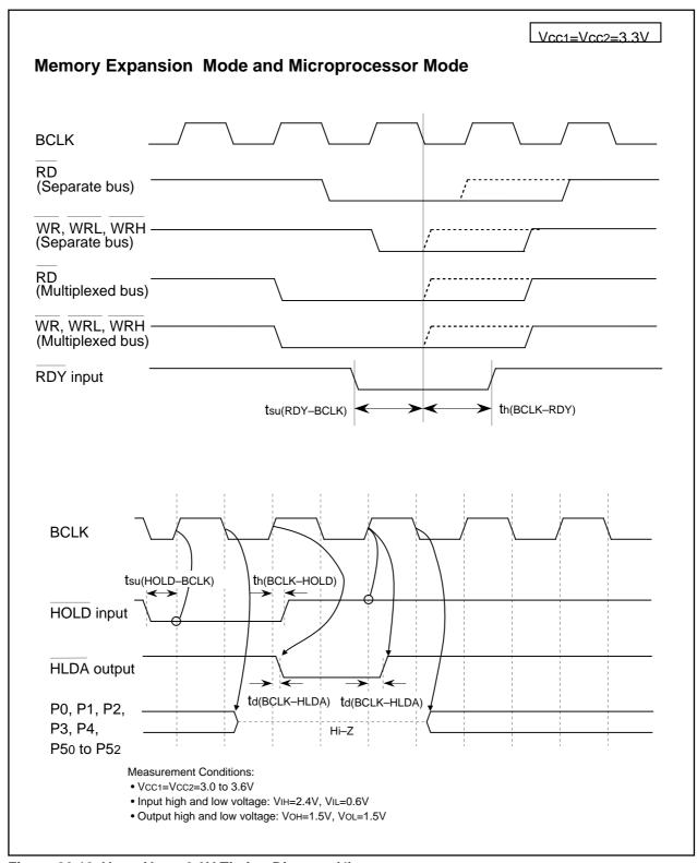
Figure 26.10 Vcc1=Vcc2=3.3V Timing Diagram (4)
