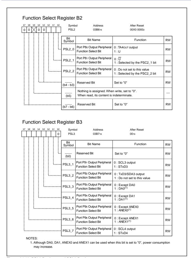
Figure 24.12 PSL2 Register and PSL3 Register
