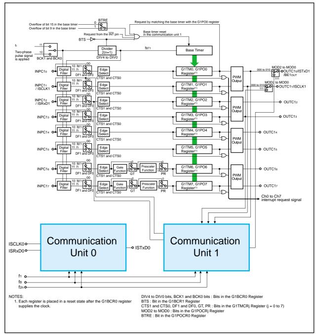
Figure 22.1 Intelligent I/O Block Diagram
