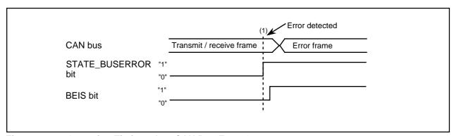
Figure 23.40 Operation Timing when CAN Bus Error Occurs
