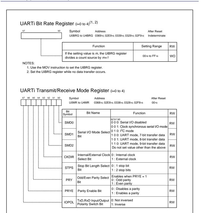
Figure 17.3 U0BRG to U4BRG Registers and U0MR to U4MR Registers
