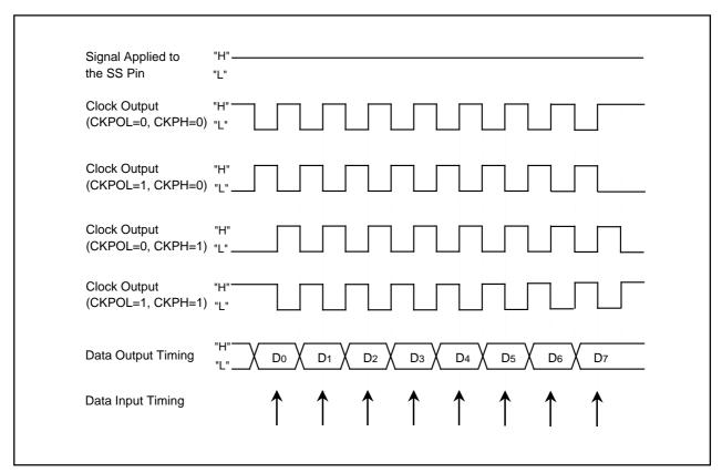
Figure 17.24 Transmit and Receive Timing in Master Mode (Internal Clock)
