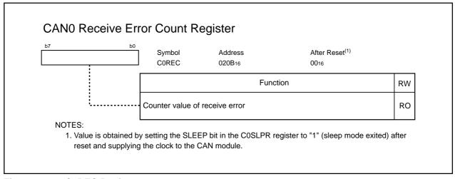
Figure 23.12 COREC Register
