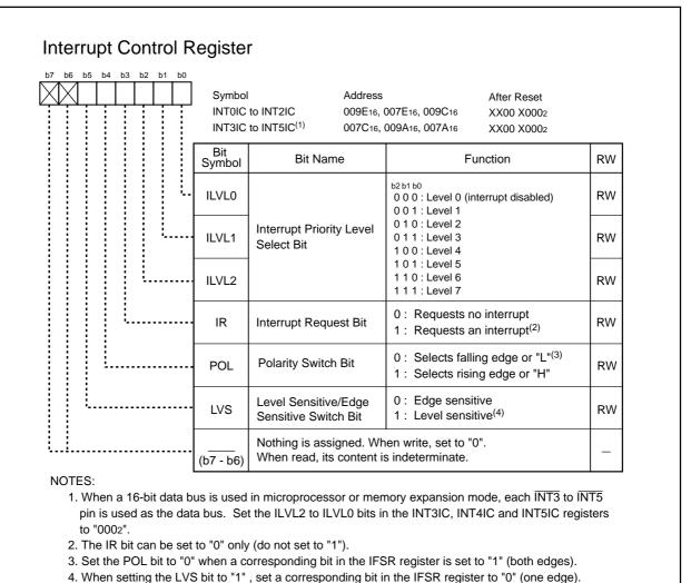
Figure 11.4 Interrupt Control Register (2)
