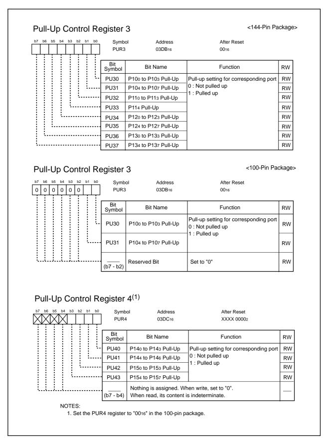
Figure 24.16 PUR3 Register and PUR4 Register
