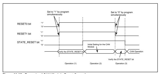
Figure 23.37 Example of CAN Module Reset Operation
