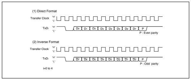
Figure 17.32 SIM Interface Format
