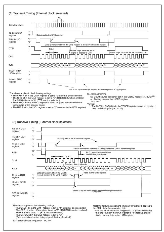
Figure 17.10 Transmit and Receive Operation
