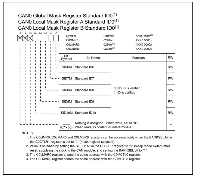
Figure 23.22 C0GMR0, C0LMAR0 and C0LMBR0 Registers
