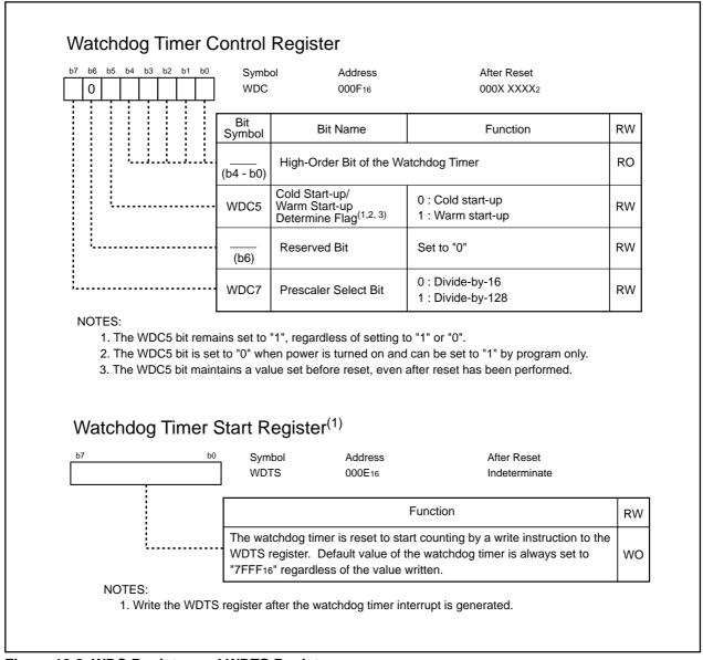
Figure 12.2 WDC Register and WDTS Register
