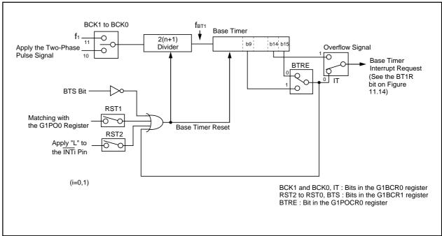
Figure 22.9 Base Timer Block Diagram
