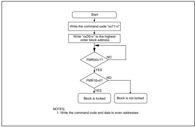
Figure 25.12 Read Lock Bit Status Command
