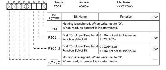
Figure 24.13 PSC Register and PSC2 Register
