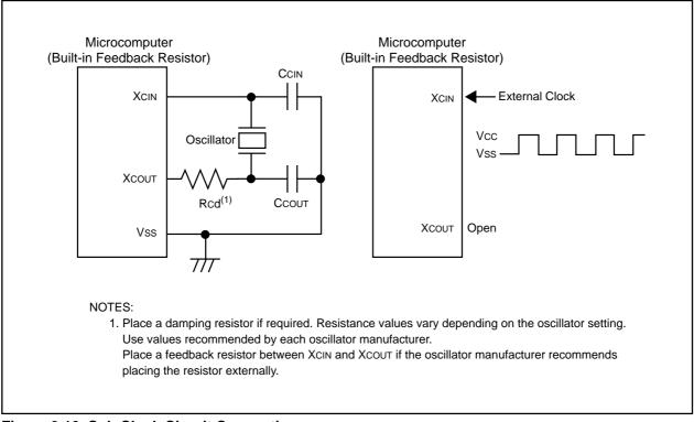
Figure 9.10 Sub Clock Circuit Connection
