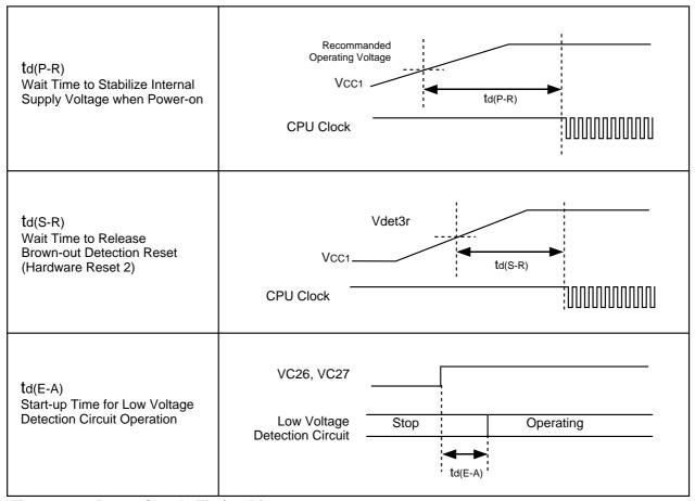
Figure 26.1 Power Supply Timing Diagram
