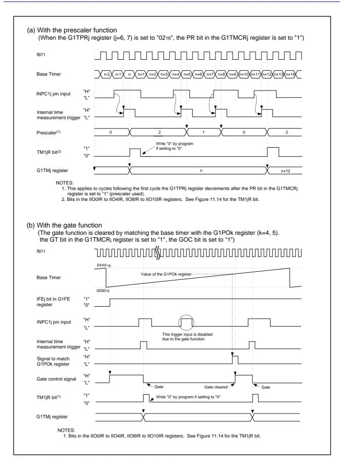
Figure 22.15 Prescaler Function and Gate Function
