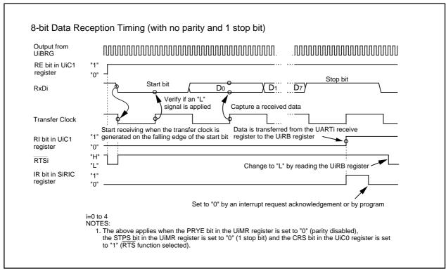
Figure 17.15 Receive Operation
