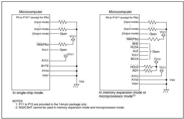
Figure 24.19 Unassigned Pin Handling
