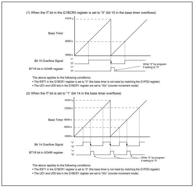
Figure 22.10 Counter Increment Mode
