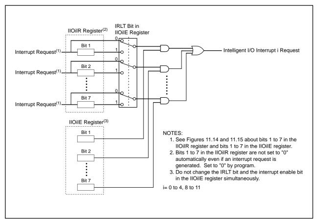
Figure 11.13 Intelligent I/O Interrupt and CAN Interrupt
