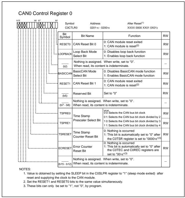
Figure 23.3 C0CTLR0 and C1CTLR0 Registers
