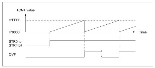
Figure 10-15 Free-Running Counter Operation
