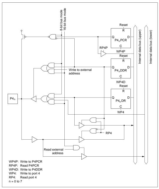
Figure C-1 Port 4 Block Diagram
