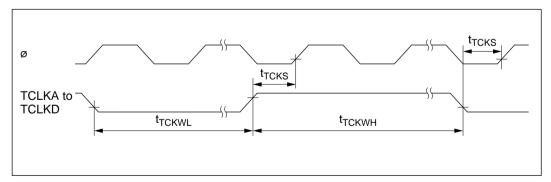
Figure 18-22 ITU Clock Input Timing
