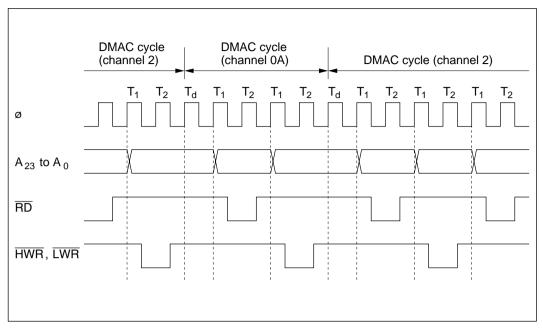
Figure 8-20 Timing of Multiple-Channel Operations in Different Groups
