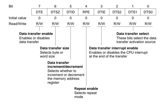
The DTCRs are initialized to H'00 by a reset and in standby mode.
