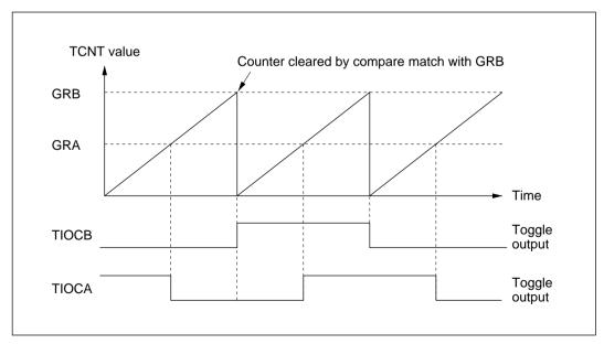
Figure 10-21 Toggle Output (Example)
