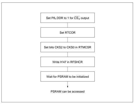
Figure 7-18 Setup Procedure for Pseudo-Static RAM
