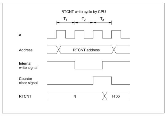
Figure 7-20 Contention between RTCNT Write and Clear
