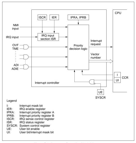
Figure 5-1 Interrupt Controller Block Diagram
