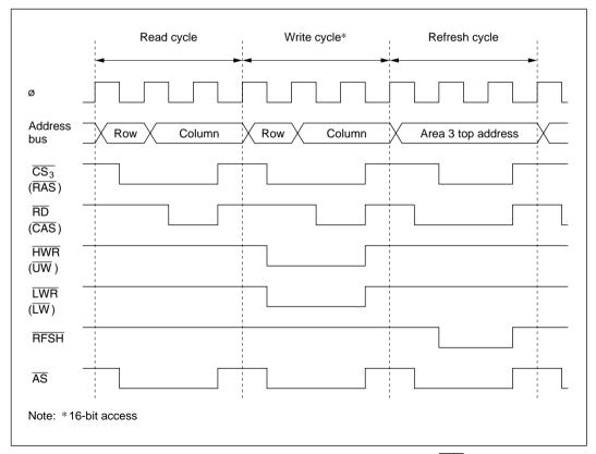
Figure 7-5 DRAM Control Signal Output Timing (1)  $(2\overline{WE} \text{ Mode})$
