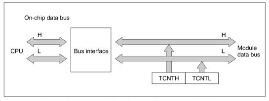
Figure 10-7 Access to Timer Counter (CPU Reads TCNT, Word)
