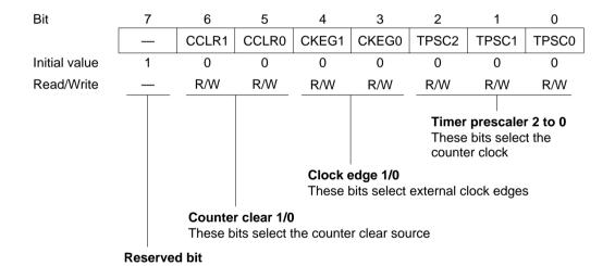
Each TCR is an 8-bit readable/writable register that selects the timer counter clock source, selects the edge or edges of external clock sources, and selects how the counter is cleared.
