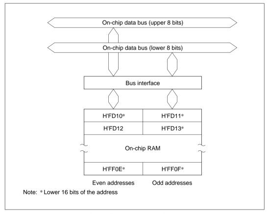
Figure 15-1 RAM Block Diagram
