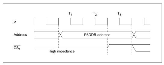
Figure 6-21 DDR Write Timing
