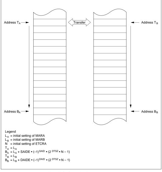
Figure 8-8 Operation in Normal Mode
