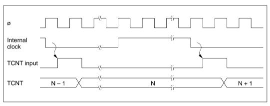
Figure 10-17 Count Timing for Internal Clock Sources
