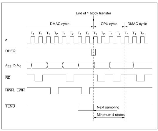
Figure 8-18 Timing of DMAC Activation by Falling Edge of DREQ in Block Transfer Mode
