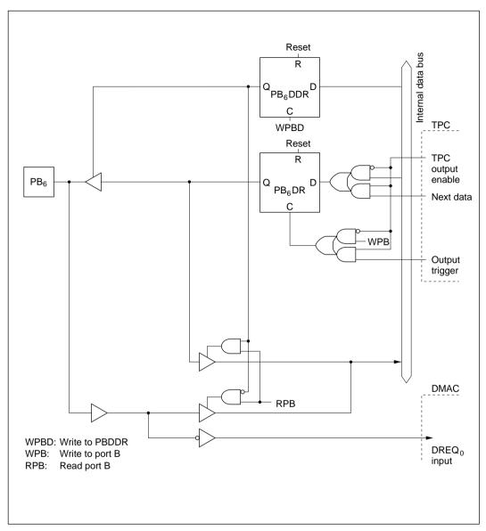
Figure C-8 (c) Port B Block Diagram (Pin  $PB_6$ )
