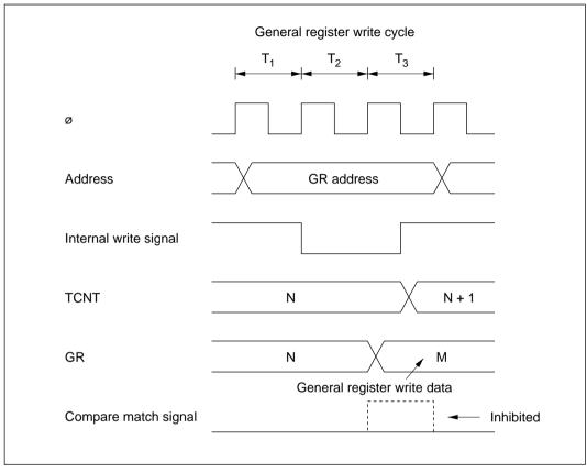
Figure 10-64 Contention between General Register Write and Compare Match
