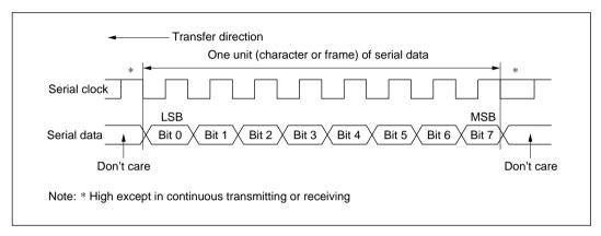
Figure 13-14 Data Format in Synchronous Communication
