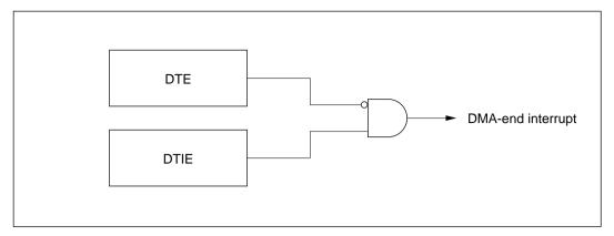
Figure 8-26 DMA-End Interrupt Logic
