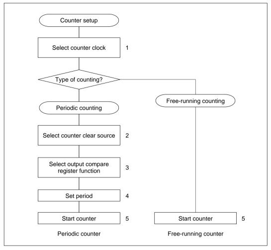
Figure 10-14 Counter Setup Procedure (Example)
