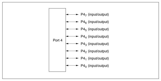
Figure 9-2 Pin Functions in 8-Bit Bus Mode (Port 4)
