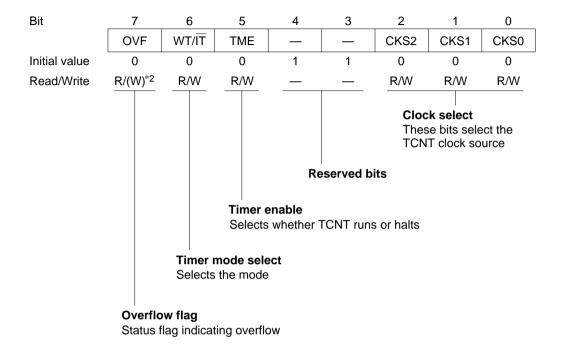
Bits 7 to 5 are initialized to 0 by a reset and in standby mode. Bits 2 to 0 are initialized to 0 by a reset. In software standby mode bits 2 to 0 are not initialized, but retain their previous values.
