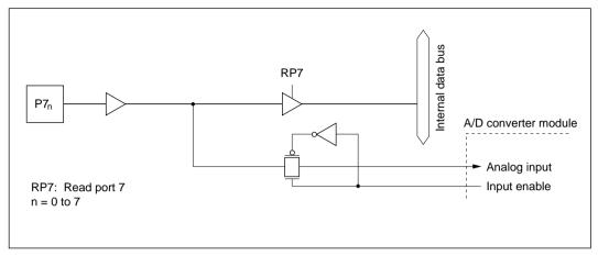
Figure C-4 Port 7 Block Diagram (Pin P7<sub>n</sub>)
