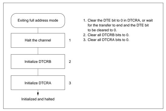
Figure 8-24 Procedure for Exiting Full Address Mode (Example)
