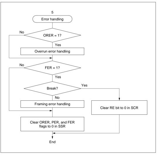
Figure 13-12 Sample Flowchart for Receiving Multiprocessor Serial Data (2)
