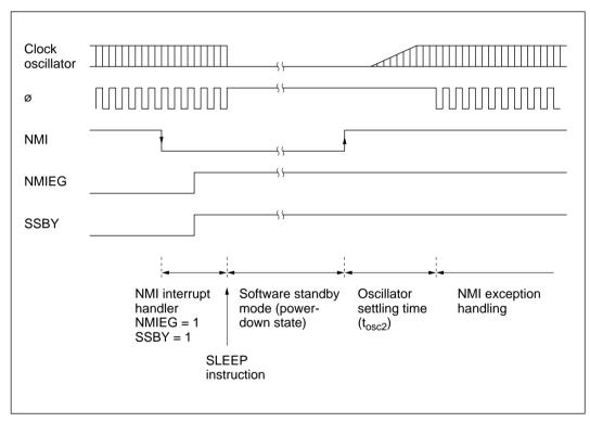
Figure 17-1 NMI Timing for Software Standby Mode (Example)
