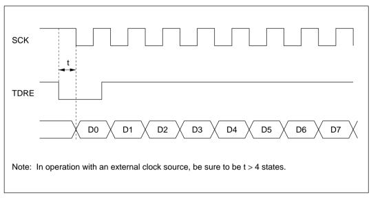
Figure 13-22 Synchronous Transmission Using DMAC (Example)
