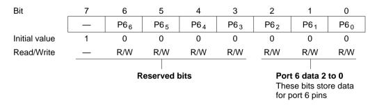
When a bit in P6DDR is set to 1, if port 6 is read the value of the corresponding P6DR bit is returned directly. When a bit in P6DDR is cleared to 0, if port 6 is read the corresponding pin level is read. In this case bit 7 reads 1 and bits 6 to 3 have undetermined values. Bits 7 to 3 are reserved. Bits 6 to 3 can be written and read, but they cannot be used for port input or output. Bit 7 cannot be modified and always reads 1.
