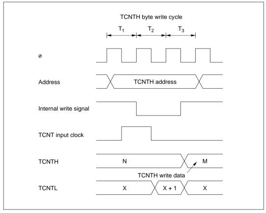
Figure 10-63 Contention between TCNT Byte Write and Increment
