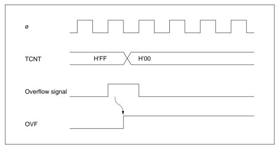
Figure 12-6 Timing of Setting of OVF
