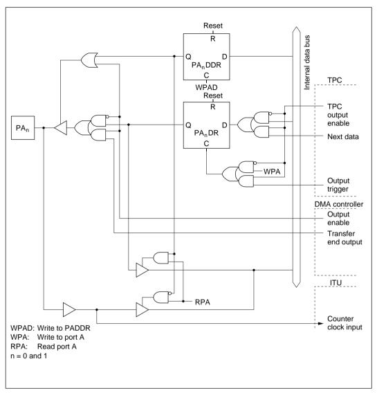
Figure C-7 (a) Port A Block Diagram (Pins PA<sub>0</sub>, PA<sub>1</sub>)
