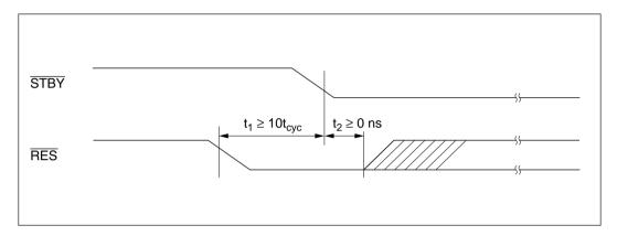
(2) To retain RAM contents with the RAME bit cleared to 0 in SYSCR, RES does not have to be driven low as in (1).
