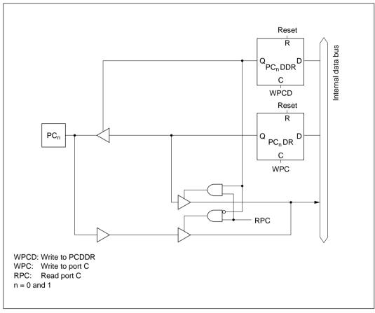
Figure C-9 (a) Port C Block Diagram (Pins PC<sub>0</sub>, PC<sub>1</sub>)
