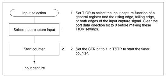
Figure 10-23 Setup Procedure for Input Capture (Example)
