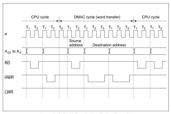
Figure 8-13 DMA Transfer Bus Timing (Example)
