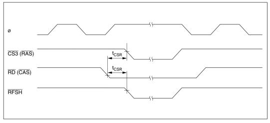
Figure 18-9 DRAM Bus Timing (Self-Refresh Mode)  $-2\overline{WE}\ Mode --$
