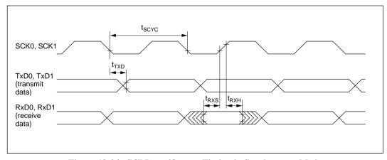
Figure 18-24 SCI Input/Output Timing in Synchronous Mode
