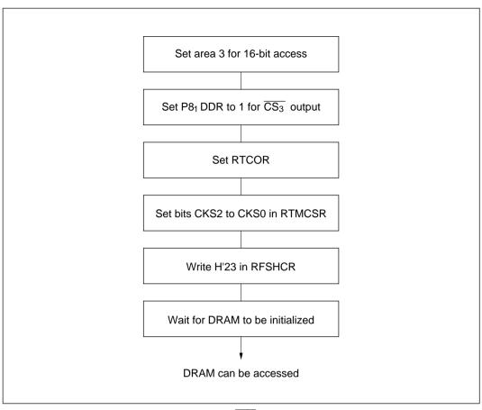
Figure 7-8 Setup Procedure for 2WE 1-Mbit DRAM (1-Mbyte Mode)
