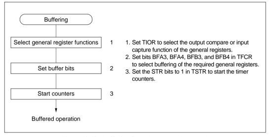
Figure 10-48 Buffering Setup Procedure (Example)
