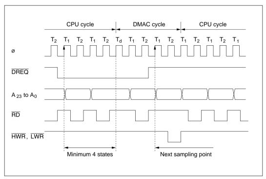
Figure 8-17 Timing of DMAC Activation by Low DREQ Level in Normal Mode
