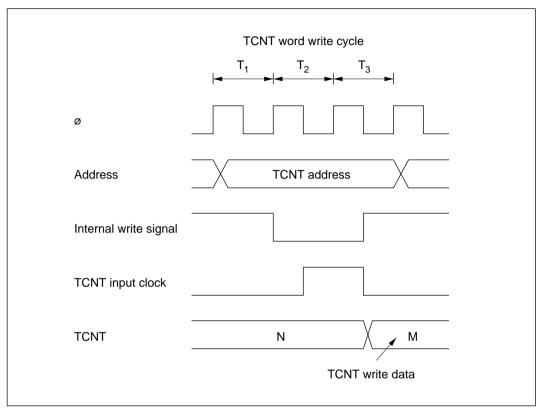
Figure 10-62 Contention between TCNT Word Write and Increment
