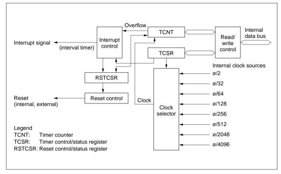
Figure 12-1 WDT Block Diagram
