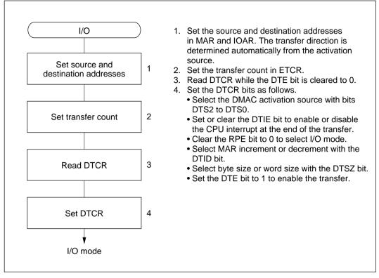
Figure 8-3 I/O Mode Setup Procedure (Example)
