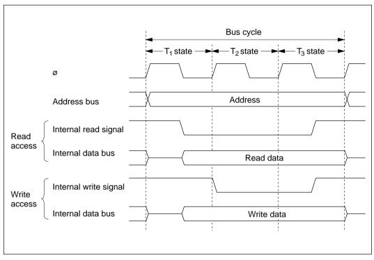
Figure 2-17 Access Cycle for On-Chip Supporting Modules
