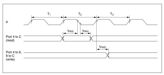
Figure 18-20 TPC and I/O Port Input/Output Timing
