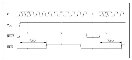
Figure 18-19 Oscillator Settling Timing
