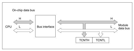
Figure 10-8 Access to Timer Counter (CPU Writes to TCNT, Upper Byte)
