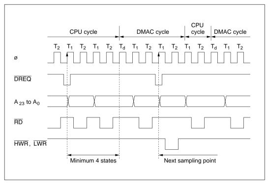
Figure 8-16 Timing of DMAC Activation by Falling Edge of DREQ in Normal Mode
