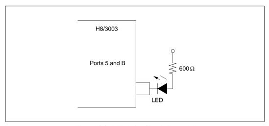
Figure 18-2 LED Drive Circuit (Example)
