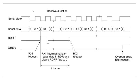
Figure 13-19 Example of SCI Receive Operation
