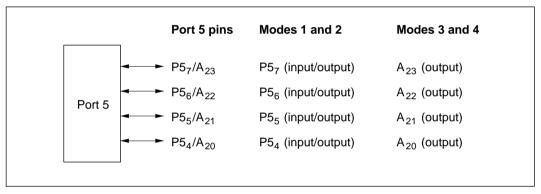
Figure 9-4 Port 5 Pin Configuration
