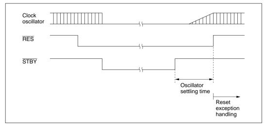
Figure 17-2 Hardware Standby Mode Timing
