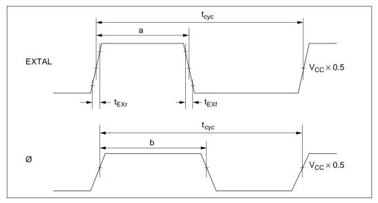
Figure 16-6 External Clock Input Timing
