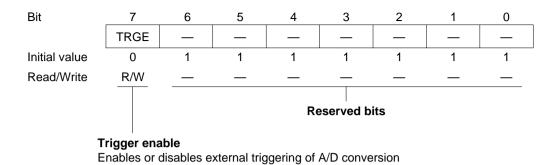
ADCR is an 8-bit readable/writable register that enables or disables external triggering of A/D conversion. ADCR is initialized to H'7F by a reset and in standby mode.
