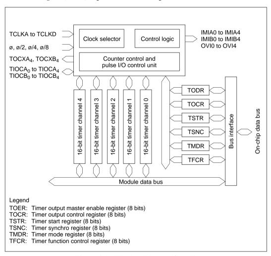
Figure 10-1 ITU Block Diagram (Overall)
