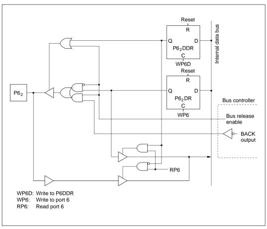
Figure C-3 (c) Port 6 Block Diagram (Pin P6<sub>2</sub>)
