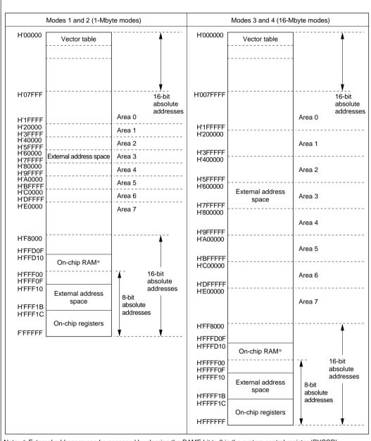
Note: \* External addresses can be accessed by clearing the RAME bit to 0 in the system control register (SYSCR).
