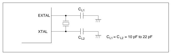
Figure 16-2 Connection of Crystal Resonator (Example)
