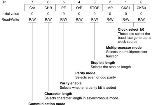
Selects asynchronous or synchronous mode
