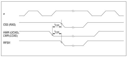
Figure 18-12 DRAM Bus Timing (Self-Refresh Mode)  $-2\overline{\text{CAS}} \text{ Mode} --$
