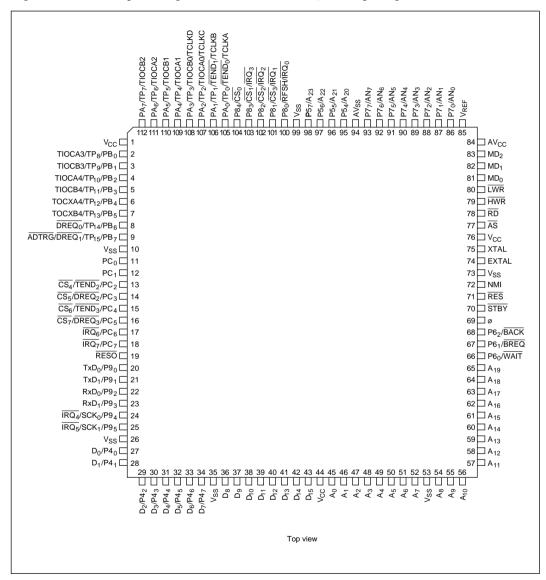
Figure 1-2 Pin Arrangement (QFP-112, Top View)
