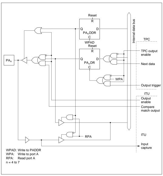
Figure C-7 (c) Port A Block Diagram (Pins PA<sub>4</sub> to PA<sub>7</sub>)
