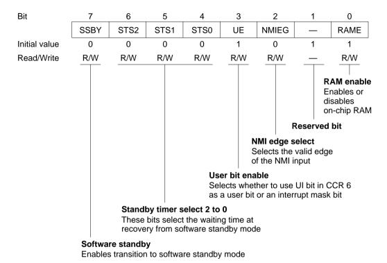
**Bit 7—Software Standby (SSBY):** Enables transition to software standby mode. (For further information about software standby mode see section 17, Power-Down State.)
