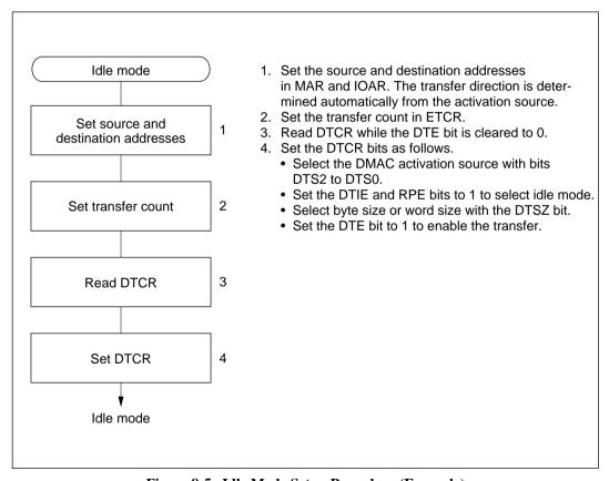
Figure 8-5 Idle Mode Setup Procedure (Example)
