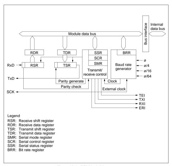
Figure 13-1 SCI Block Diagram
