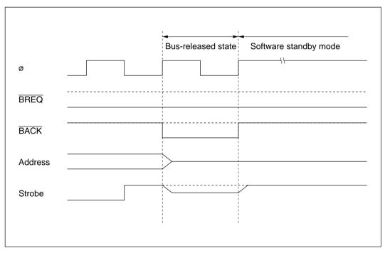
Figure 7-24 Contention between Bus-Released State and Software Standby Mode
