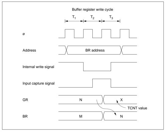
Figure 10-69 Contention between Buffer Register Write and Input Capture
