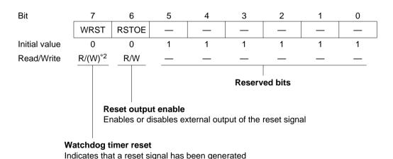
Bits 7 and 6 are initialized by input of a reset signal at the  $\overline{RES}$  pin. They are not initialized by reset signals generated by watchdog timer overflow.
