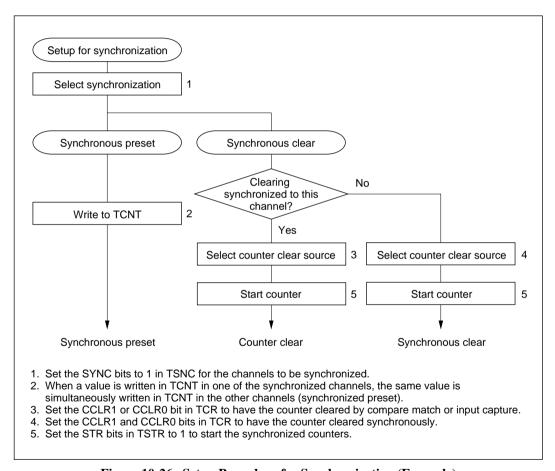
Figure 10-26 Setup Procedure for Synchronization (Example)
