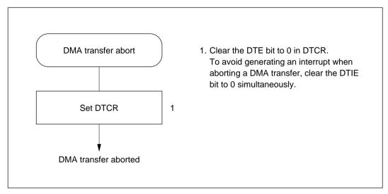
Figure 8-23 Procedure for Aborting a DMA Transfer
