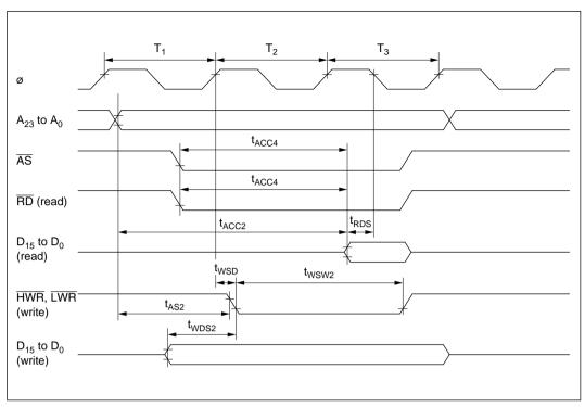
Figure 18-5 Basic Bus Cycle: Three-State Access
