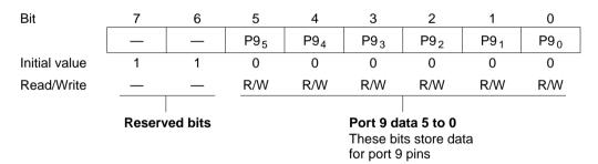
When a bit in P9DDR is set to 1, if port 9 is read the value of the corresponding P9DR bit is returned directly. When a bit in P9DDR is cleared to 0, if port 9 is read the corresponding pin level is read.
