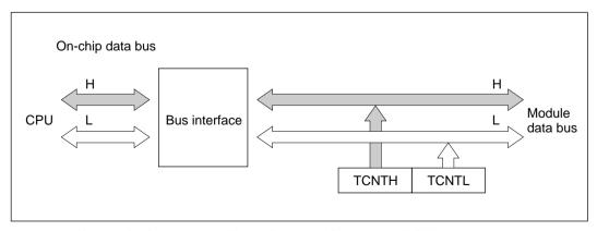
Figure 10-10 Access to Timer Counter (CPU Reads TCNT, Upper Byte)
