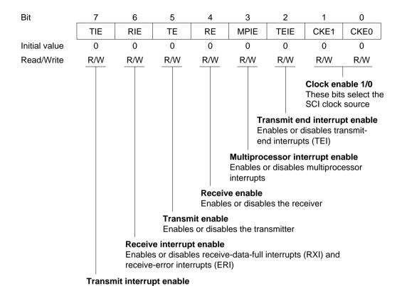
The CPU can always read and write SCR. SCR is initialized to H'00 by a reset and in standby mode.
