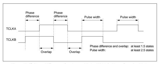
Figure 10-45 Phase Difference, Overlap, and Pulse Width in Phase Counting Mode
