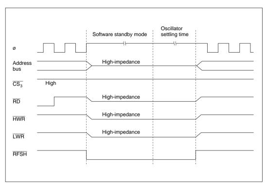
Figure 7-16 Signal Output Timing in Self-Refresh Mode (PSRAME = 1, DRAME = 0)
