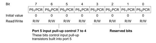
In modes 1 and 2, when a P5DDR bit is cleared to 0 (selecting generic input), if the corresponding bit from P5<sub>7</sub>PCR to P5<sub>4</sub>PCR is set to 1, the input pull-up transistor is turned on.
