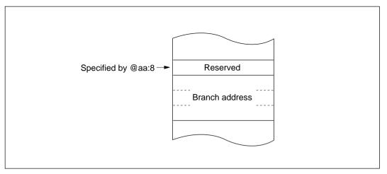
Figure 2-10 Memory-Indirect Branch Address Specification
