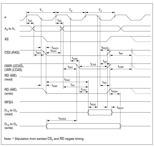
Figure 18-10 DRAM Bus Timing (Read/Write): Three-State Access  $-2\overline{\text{CAS}}$  Mode -
