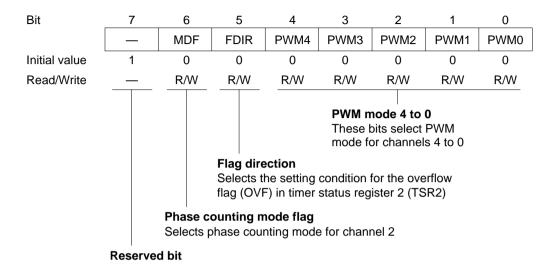
TMDR is initialized to H'80 by a reset and in standby mode.
