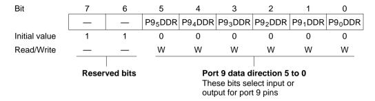
A pin in port 9 becomes an output pin if the corresponding P9DDR bit is set to 1, and an input pin if this bit is cleared to 0.
