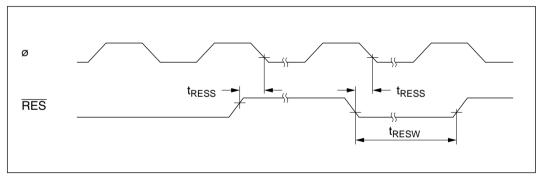
Figure 18-15 Reset Input Timing
