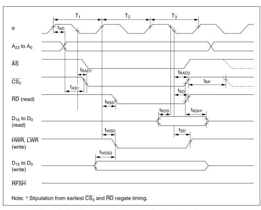
Figure 18-13 PSRAM Bus Timing (Read/Write): Three-State Access
