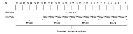
An MAR functions as a source or destination address register depending on how the DMAC is activated: as a destination address register if activation is by a receive-data-full interrupt from the serial communication interface (SCI), and as a source address register otherwise.
