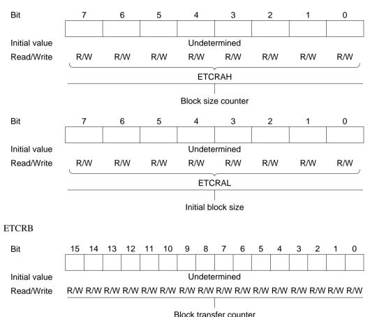
In block transfer mode, ETCRAH functions as an 8-bit block size counter. ETCRAL holds the initial block size. ETCRAH is decremented by 1 each time one byte or word is transferred. When the count reaches H'00, ETCRAH is reloaded from ETCRAL. Blocks consisting of an arbitrary number of bytes or words can be transferred repeatedly by setting the same initial block size value in ETCRAH and ETCRAL.
