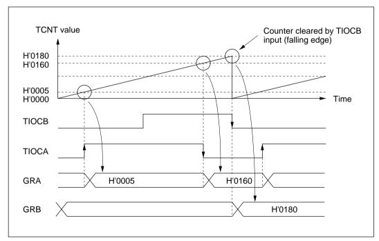
Figure 10-24 Input Capture (Example)
