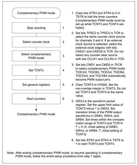
Figure 10-33 Setup Procedure for Complementary PWM Mode (Example)
