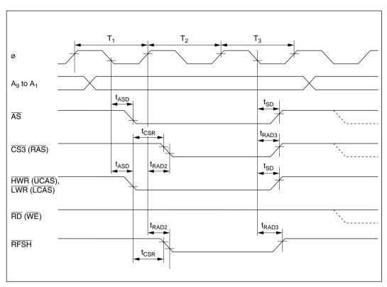
Figure 18-11 DRAM Bus Timing (Refresh Cycle): Three-State Access
