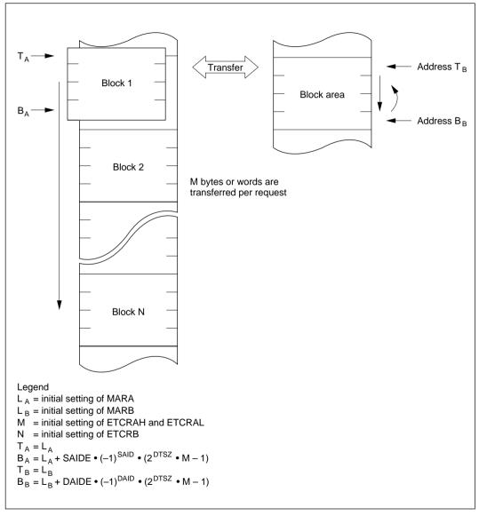
Figure 8-10 Operation in Block Transfer Mode
