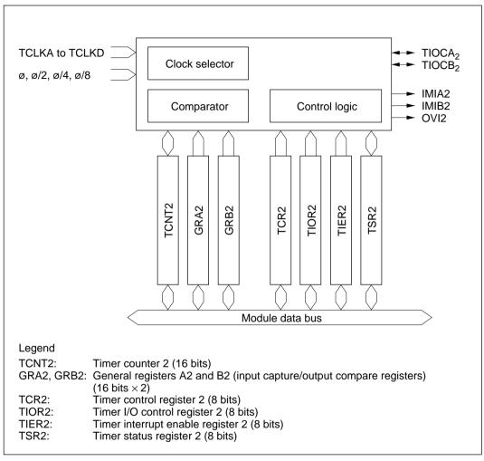
Figure 10-3 Block Diagram of Channel 2
