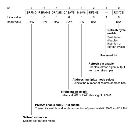
RFSHCR is initialized to H'02 by a reset and in hardware standby mode.
