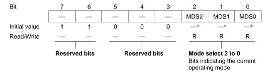
Note: \* Determined by pins MD<sub>2</sub> to MD<sub>0</sub>.
