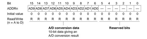
The four A/D data registers (ADDRA to ADDRD) are 16-bit read-only registers that store the results of A/D conversion.
