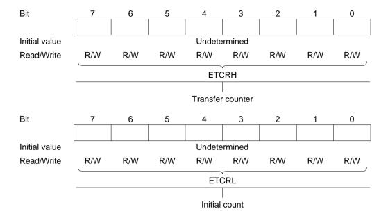
In repeat mode, ETCRH functions as an 8-bit transfer counter and ETCRL holds the initial transfer count. ETCRH is decremented by 1 each time one transfer is executed. When ETCRH reaches H'00, the value in ETCRL is reloaded into ETCRH and the same operation is repeated.
