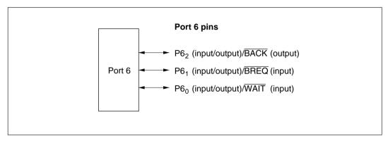
Figure 9-7 Port 6 Pin Configuration
