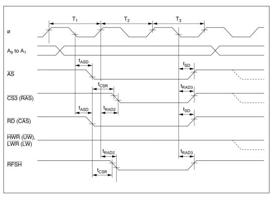
Figure 18-8 DRAM Bus Timing (Refresh Cycle): Three-State Access  $-2\overline{\text{WE}}$  Mode -
