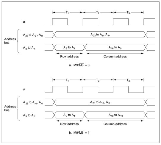
Figure 7-4 Multiplexed Address Output (Example without Wait States)
