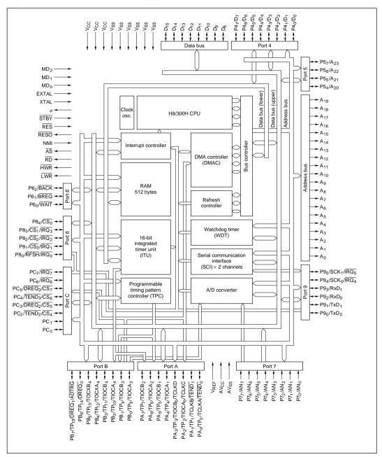
Figure 1-1 Block Diagram
