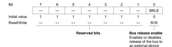
BRCR is initialized to HFE by a reset and in hardware standby mode. It is not initialized in software standby mode.
