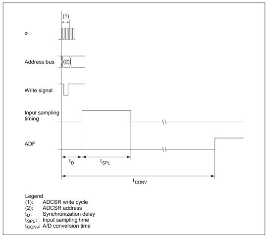
Figure 14-5 A/D Conversion Timing
