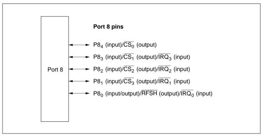
Figure 9-9 Port 8 Pin Configuration
