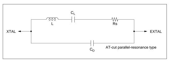
Figure 16-3 Crystal Resonator Equivalent Circuit
