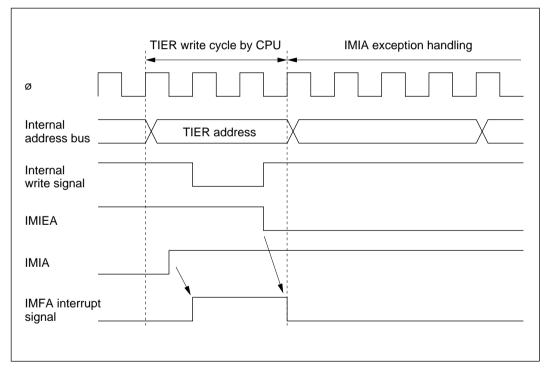
Figure 5-8 Contention between Interrupt and Interrupt-Disabling Instruction
