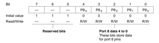
When a bit in P8DDR is set to 1, if port 8 is read the value of the corresponding P8DR bit is returned directly. When a bit in P8DDR is cleared to 0, if port 8 is read the corresponding pin level is read.
