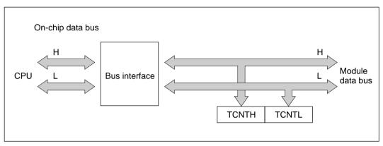
Figure 10-6 Access to Timer Counter (CPU Writes to TCNT, Word)
