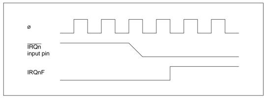
Figure 5-3 Timing of Setting of IROnF
