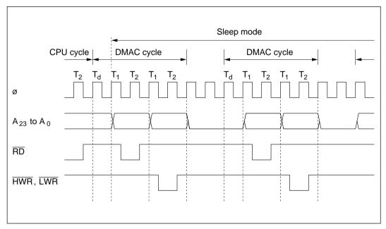
Figure 8-25 Timing of Cycle-Steal Transfer in Sleep Mode
