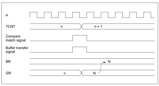
Figure 10-50 Compare Match and Buffer Transfer Timing (Example)
