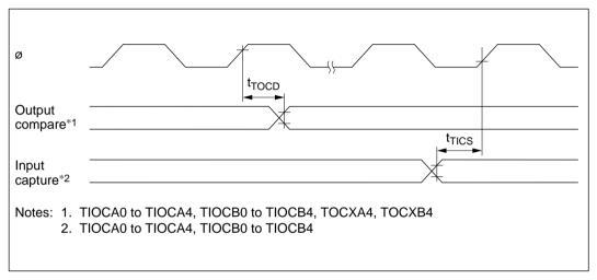
Figure 18-21 ITU Input/Output Timing
