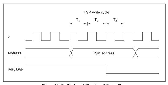
Figure 10-60 Timing of Clearing of Status Flags
