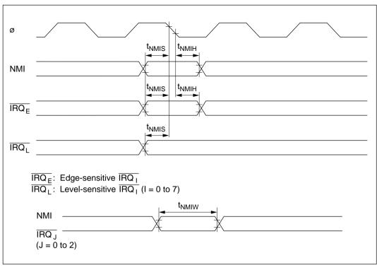
Figure 18-17 Interrupt Input Timing
