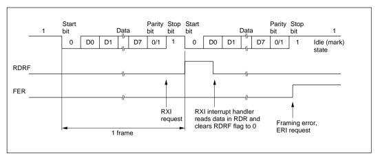
Figure 13-8 Example of SCI Receive Operation (8-Bit Data with Parity and One Stop Bit)
