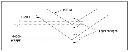
Figure 10-41 Changing a General Register Setting by Buffer Transfer (Caution 2)
