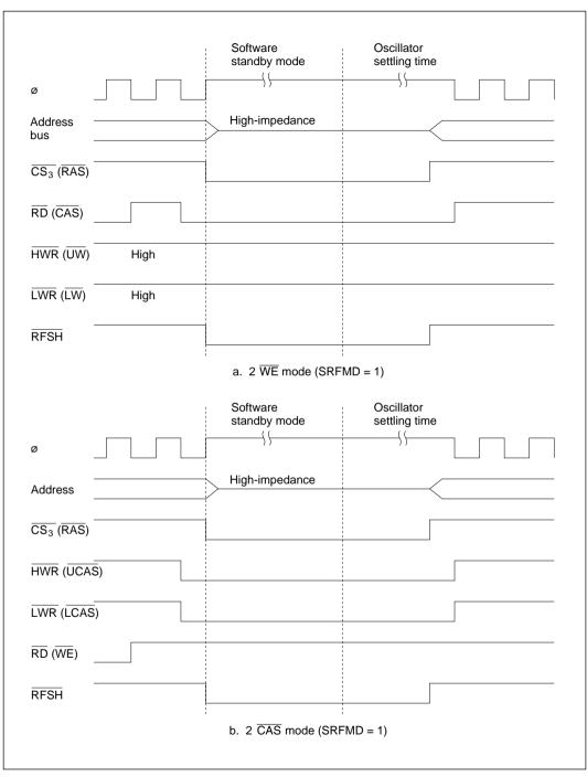
Figure 7-6 Signal Output Timing in Self-Refresh Mode (PSRAME = 0, DRAME = 1)
