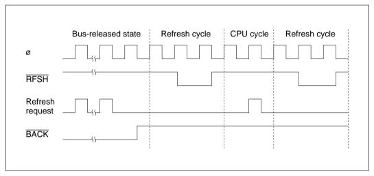
Figure 7-23 Refresh Cycles when Bus is Released
