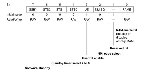
One function of SYSCR is to enable or disable access to the on-chip RAM. The on-chip RAM is enabled or disabled by the RAME bit in SYSCR. For details about the other bits, see section 3.3, System Control Register.
