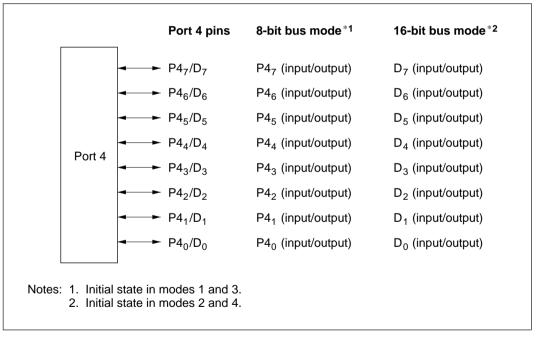
Figure 9-1 Port 4 Pin Configuration
