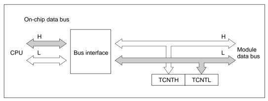
Figure 10-9 Access to Timer Counter (CPU Writes to TCNT, Lower Byte)
