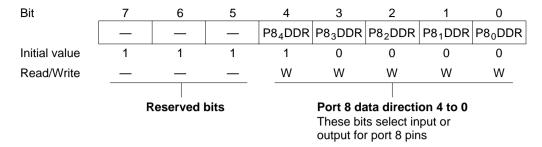
When bits in P8DDR bit are set to 1,  $P8_4$  to  $P8_1$  become  $\overline{CS_0}$  to  $\overline{CS_3}$  output pins and  $P8_0$  becomes a generic output pin. When bits in P8DDR are cleared to 0, the corresponding pins become input pins.
