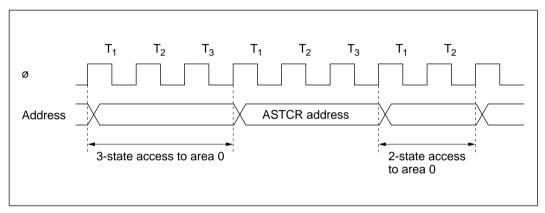
Figure 6-20 ASTCR Write Timing
