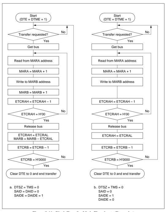
Figure 8-11 Block Transfer Mode Flowcharts (Examples)
