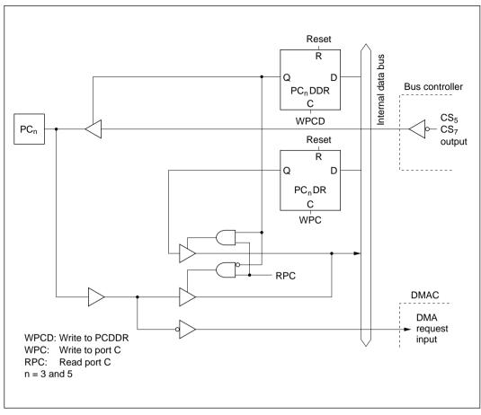
$Figure \ C-9 \ (c) \quad Port \ C \ Block \ Diagram \ (Pins \ PC_3, PC_5)$
