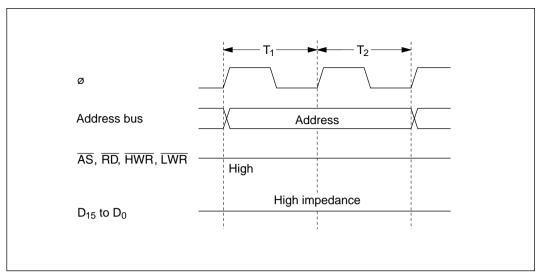
Figure 2-16 Pin States during On-Chip Memory Access
