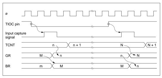
Figure 10-52 Input Capture and Buffer Transfer Timing (Example)
