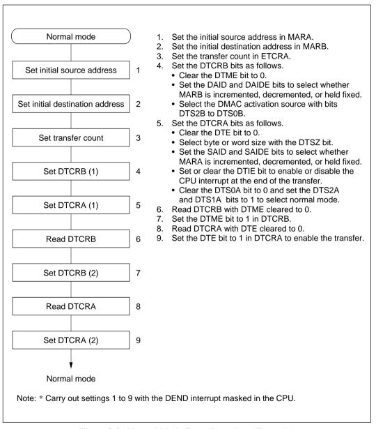
Figure 8-9 Normal Mode Setup Procedure (Example)
