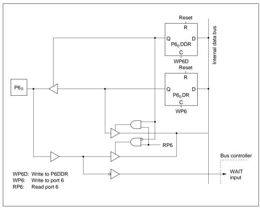
Figure C-3 (a) Port 6 Block Diagram (Pin  $P6_0$ )
