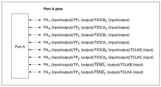
Figure 9-11 Port A Pin Configuration
