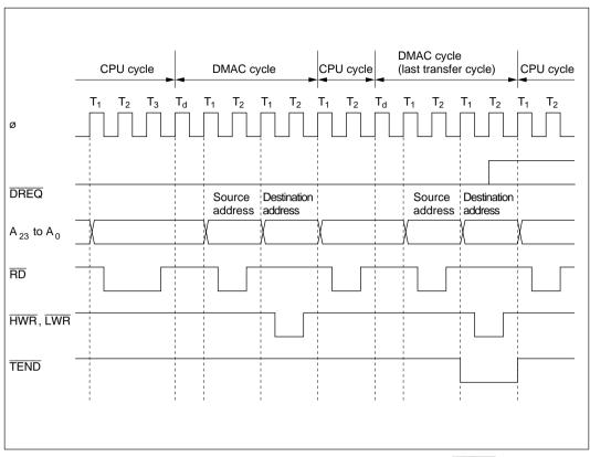
Figure 8-14 Bus Timing of DMA Transfer Requested by Low DREQ Input
