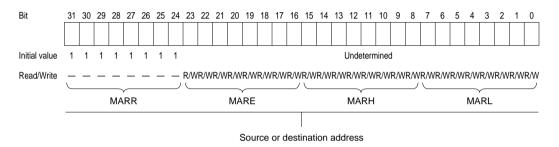
The MAR value is incremented or decremented each time one byte or word is transferred, automatically updating the source or destination memory address. For details, see section 8.3.4, Data Transfer Control Registers (DTCR).
