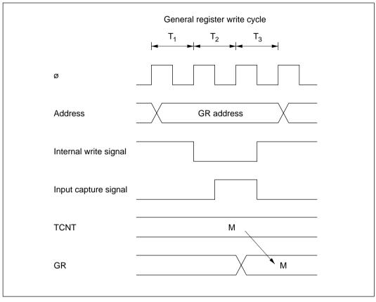
Figure 10-68 Contention between General Register Write and Input Capture
