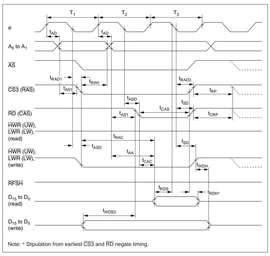
Figure 18-7 DRAM Bus Timing (Read/Write): Three-State Access
