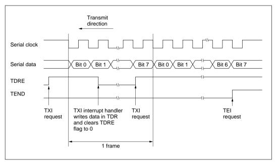
Figure 13-17 Example of SCI Transmit Operation
