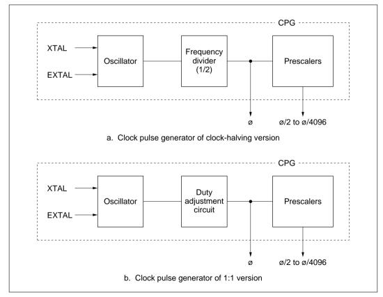
Figure 16-1 Block Diagram of Clock Pulse Generator
