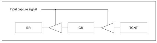
Figure 10-47 Input Capture Buffering
