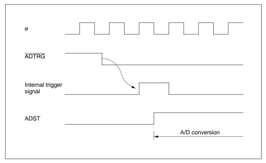
Figure 14-6 External Trigger Input Timing
