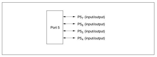
Figure 9-5 Pin Functions in Modes 1 and 2 (Port 5)
