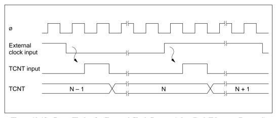
Figure 10-18 Count Timing for External Clock Sources (when Both Edges are Detected)
