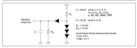
Figure 18-3 Output Load Circuit
