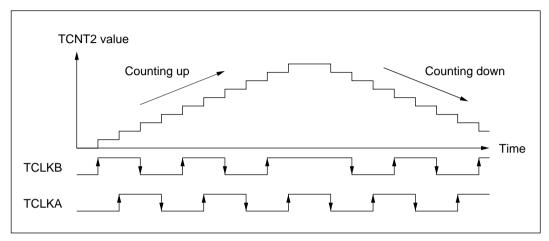
Figure 10-44 Operation in Phase Counting Mode (Example)
