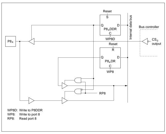
Figure C-5 (c) Port 8 Block Diagram (Pin  $P8_4$ )
