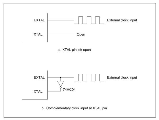
Figure 16-5 External Clock Input (Examples)
