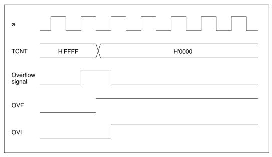
Figure 10-59 Timing of Setting of OVF
