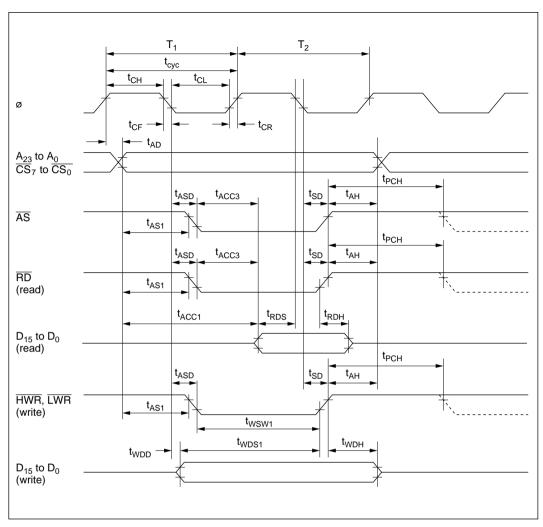
Figure 18-4 Basic Bus Cycle: Two-State Access
