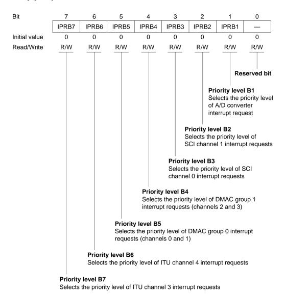
IPRB is initialized to H'00 by a reset and in hardware standby mode.
