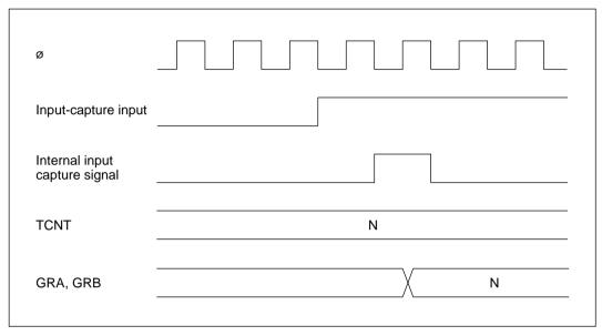
Figure 10-25 Input Capture Signal Timing
