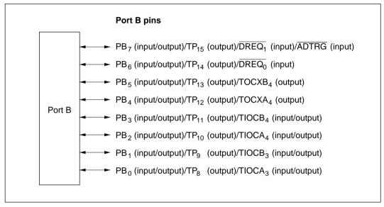
Figure 9-12 Port B Pin Configuration
