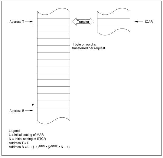
Figure 8-2 Operation in I/O Mode
