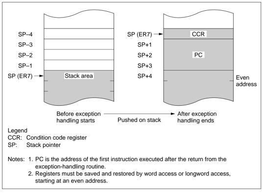
Figure 2-14 Stack Structure after Exception Handling
