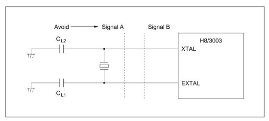
Figure 16-4 Example of Incorrect Board Design
