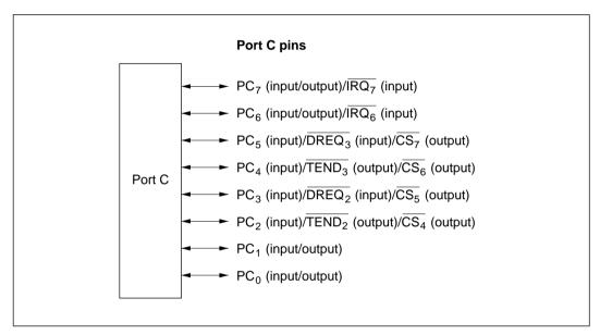
Figure 9-13 Port C Pin Configuration
