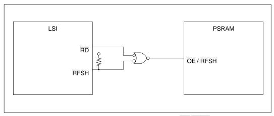
Figure 7-17 Interconnection to Pseudo-Static RAM with OE/RFSH Signal (Example)
