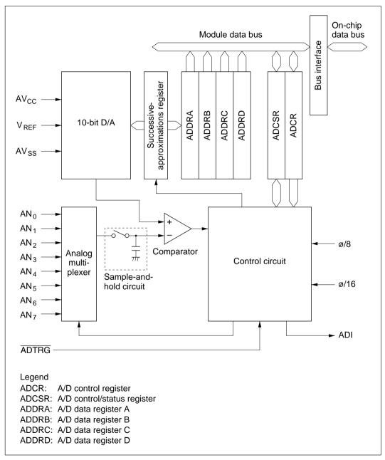
Figure 14-1 A/D Converter Block Diagram
