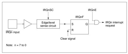
Figure 5-2 Block Diagram of Interrupts IRQ<sub>0</sub> to IRQ<sub>7</sub>
