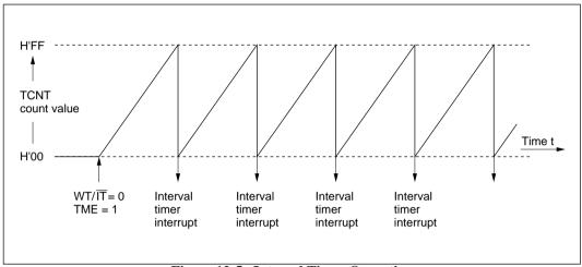
Figure 12-5 Interval Timer Operation
