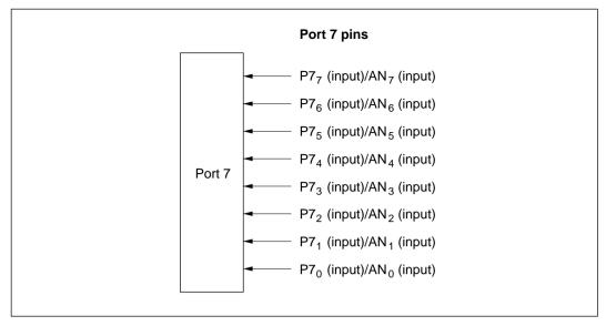
Figure 9-8 Port 7 Pin Configuration
