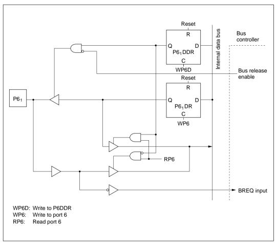
Figure C-3 (b) Port 6 Block Diagram (Pin P6<sub>1</sub>)
