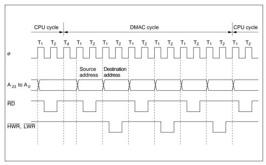
Figure 8-15 Burst DMA Bus Timing
