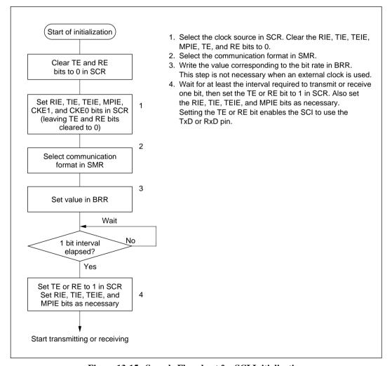
Figure 13-15 Sample Flowchart for SCI Initialization
