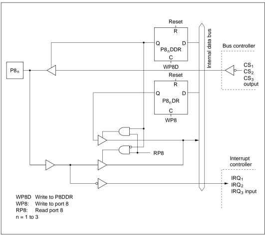
Figure C-5 (b) Port 8 Block Diagram (Pins P8<sub>1</sub>, P8<sub>2</sub>, P8<sub>3</sub>)
