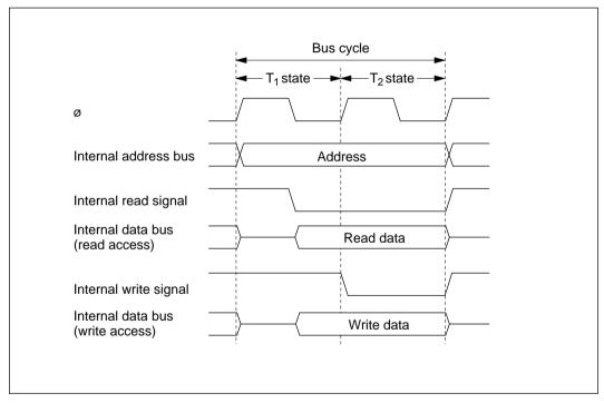
Figure 2-15 On-Chip Memory Access Cycle
