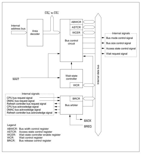
Figure 6-1 Block Diagram of Bus Controller
