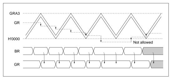
Figure 10-39 Changing a General Register Setting by Buffer Transfer (Example 1)
