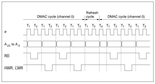
Figure 8-21 Bus Timing of Refresh Controller and DMAC
