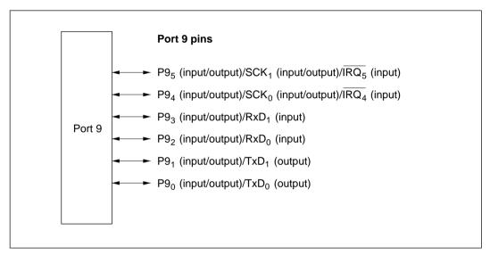
Figure 9-10 Port 9 Pin Configuration
