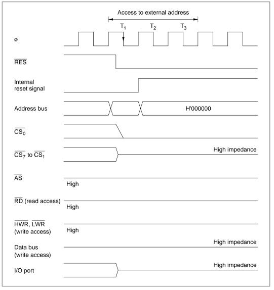
Figure D-1 Reset during Memory Access (Reset during T<sub>1</sub> State)
