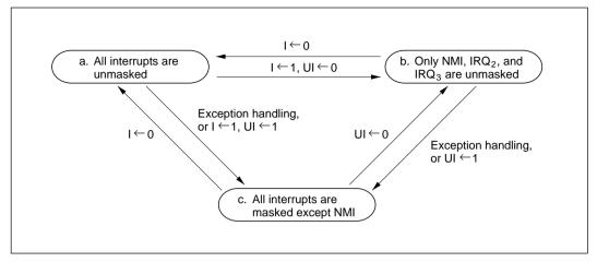
Figure 5-5 Interrupt Masking State Transitions (Example)
