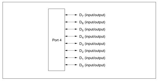
Figure 9-3 Pin Functions in 16-Bit Bus Mode (Port 4)
