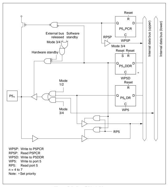
Figure C-2 Port 5 Block Diagram
