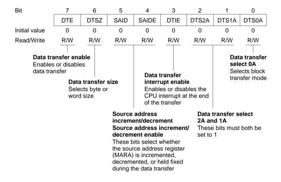
DTCRA is initialized to H'00 by a reset and in standby mode.
