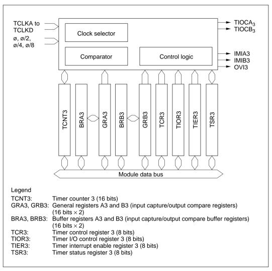
Figure 10-4 Block Diagram of Channel 3
