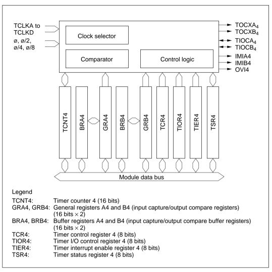
Figure 10-5 Block Diagram of Channel 4
