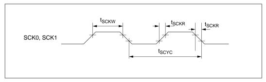
Figure 18-23 SCK Input Clock Timing
