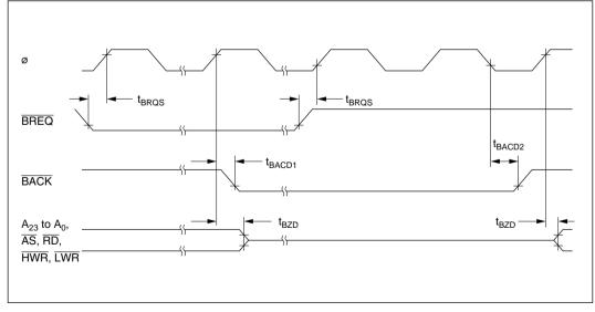
Figure 18-18 Bus-Release Mode Timing
