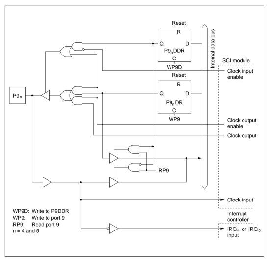
Figure C-6 (c) Port 9 Block Diagram (Pins P9<sub>4</sub>, P9<sub>5</sub>)
