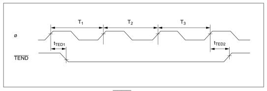
Figure 18-26 DMAC TEND Output Timing/3 State Access
