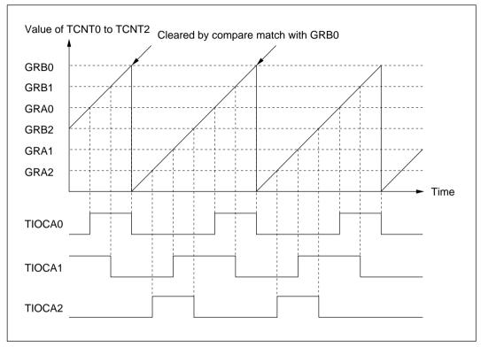
Figure 10-27 Synchronization (Example)
