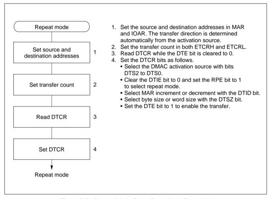
Figure 8-7 Repeat Mode Setup Procedure (Example)
