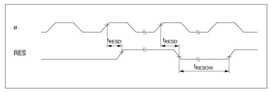
Figure 18-16 Reset Output Timing
