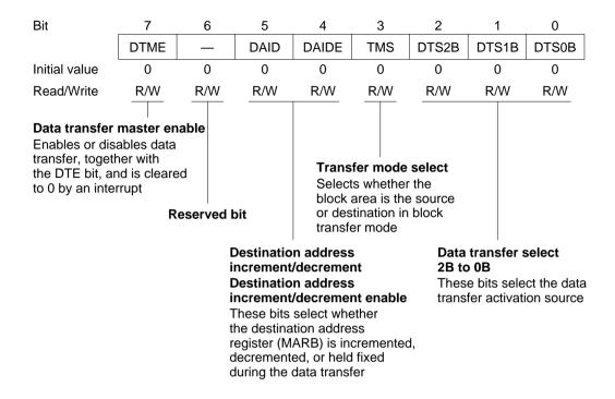
DTCRB is initialized to H'00 by a reset and in standby mode.
