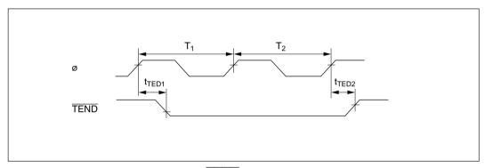
Figure 18-25 DMAC  $\overline{\text{TEND}}$  Output Timing/2 State Access
