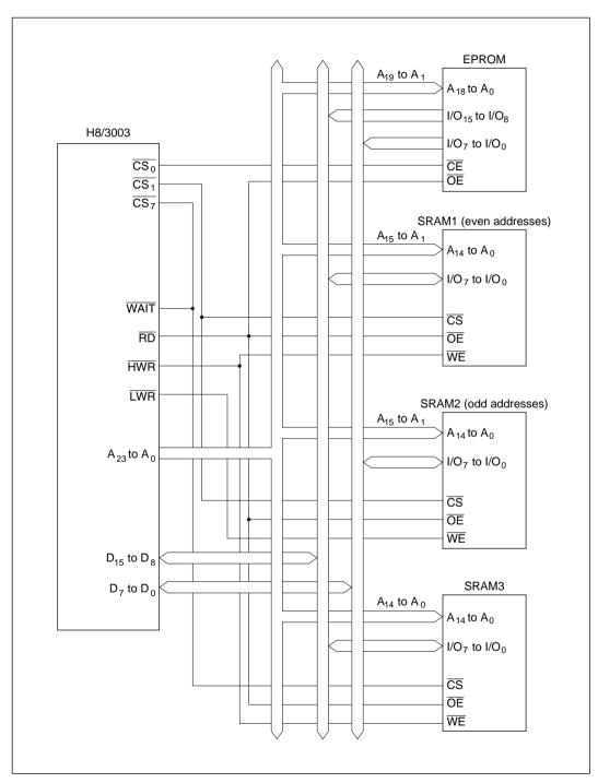
Figure 6-18 Interconnections between H8/3003 and Memory (Example)
