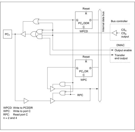
Figure C-9 (b) Port C Block Diagram (Pins PC<sub>2</sub>, PC<sub>4</sub>)
