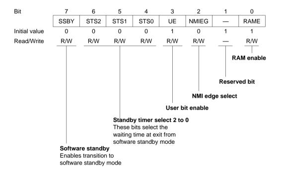
SYSCR is an 8-bit readable/writable register. Bit 7 (SSBY) and bits 6 to 4 (STS2 to STS0) control the power-down state. For information on the other SYSCR bits, see section 3.3, System Control Register.
