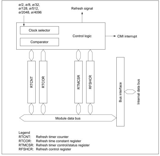
Figure 7-1 Block Diagram of Refresh Controller
