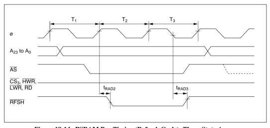
Figure 18-14 PSRAM Bus Timing (Refresh Cycle): Three-State Access
