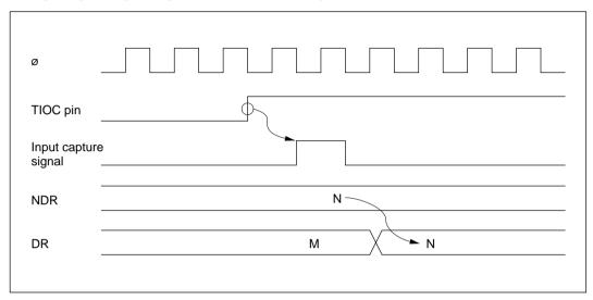
Figure 11-8 TPC Output Triggering by Input Capture (Example)
