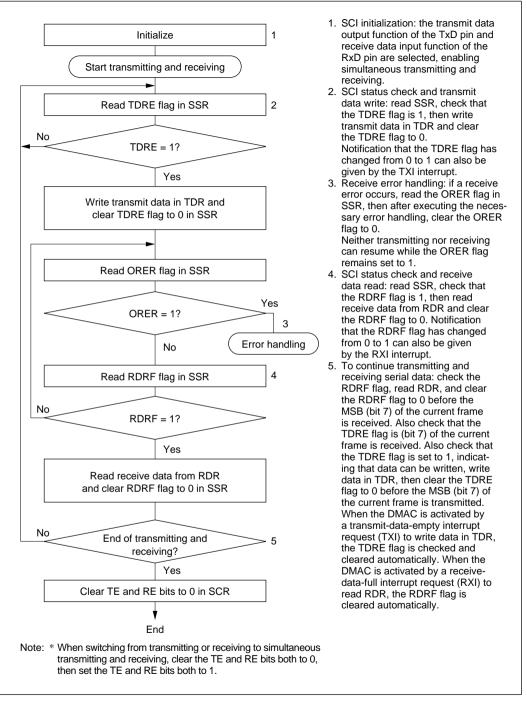
Figure 13-20 Sample Flowchart for Serial Transmitting
