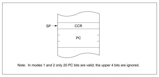
Figure 4-5 Stack after Completion of Exception Handling
