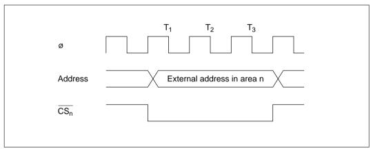
Figure 6-3  $\overline{CS_n}$  Output Timing
