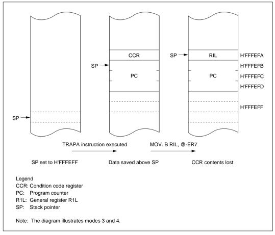
Figure 4-6 Operation when SP Value is Odd
