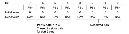
When a bit in P5DDR is set to 1, if port 5 is read the value of the corresponding P5DR bit is returned directly, regardless of the actual state of the pin. When a bit in P5DDR is cleared to 0, if port 5 is read the corresponding pin level is read.
