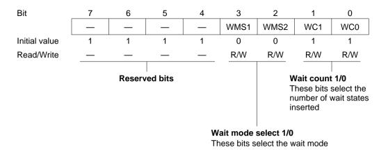
WCR is initialized to H'F3 by a reset and in hardware standby mode. It is not initialized in software standby mode.
