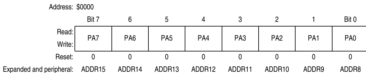
Figure 6-1. Port A Data Register (PORTA)
