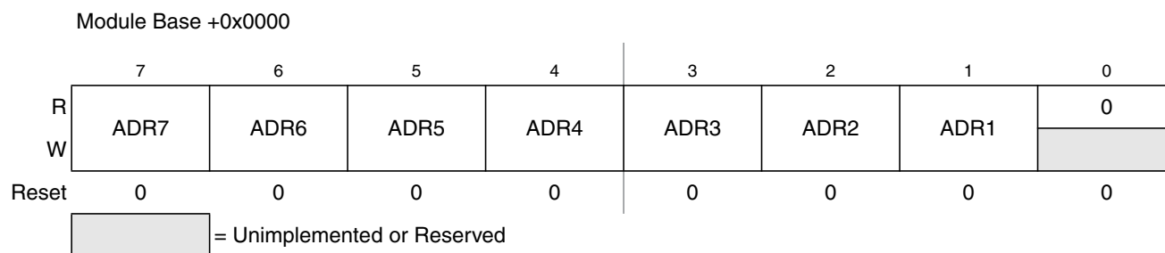
Figure 15-3. IIC Bus Address Register (IBAD)
