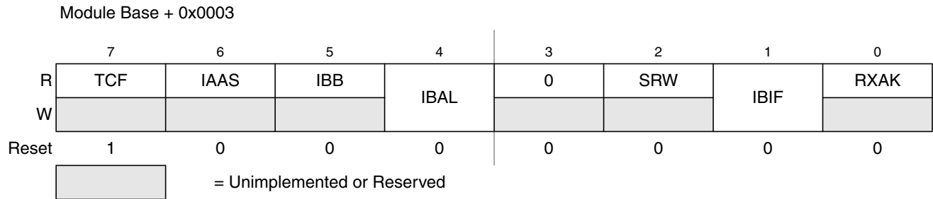
Figure 15-7. IIC Bus Status Register (IBSR)
