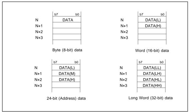
Figure 1.8.2 Data arrangement in memory
