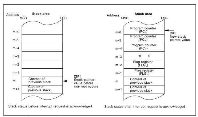
Figure 5.3.2 Stack status before and after an interrupt request is acknowledged
