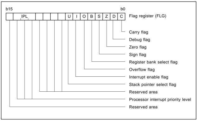
Figure 1.4.1 Configuration of flag register (FLG)
