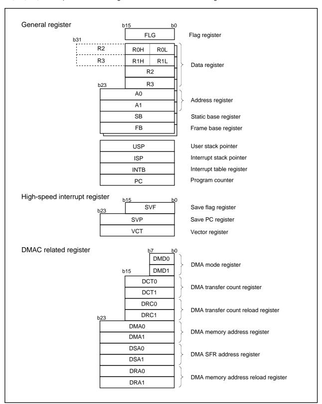
Figure 1.3.1 CPU register configuration
