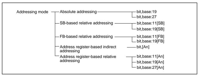
Figure 1.7.4 Addressing modes used for memory bit specification
