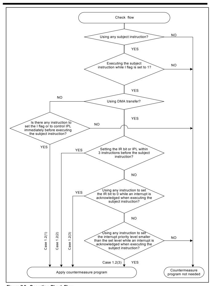
Figure 7.2 Operation Check Flow
