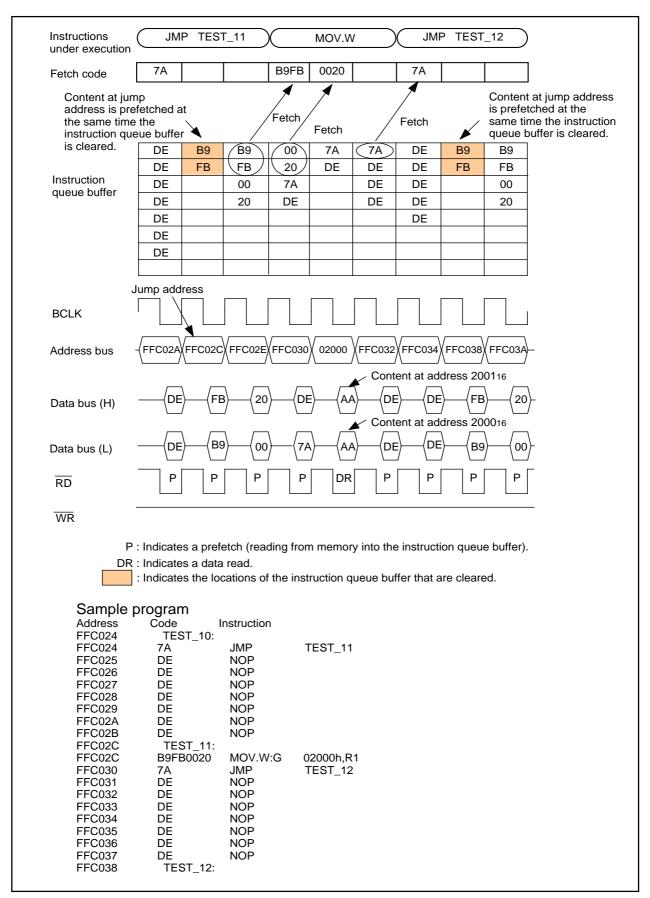
Figure 6.1.3. When executing an instruction to read from even addresses starting from an even address (Program area: 16-bit bus without wait state; Data area: 16-bit bus without wait state)
