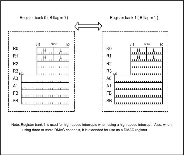
Figure 1.5.1 Configuration of register banks
