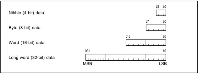
Figure 1.8.1 Data arrangement in register
