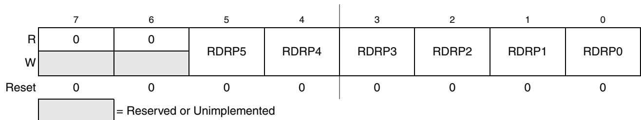
Figure 3-20. Port P Reduced Drive Register (RDRP)
